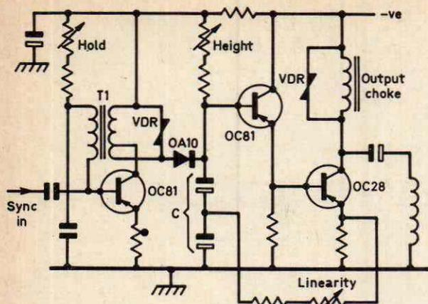
Fig. 3: Practical field timebase circuit using a blocking oscillator stage. Note the tapping on T1 primary, explained in the text.
