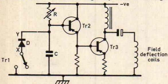
Fig. 1: Basic direct-coupled sawtooth-generator field timebase circuit with oscillator stage Tr1 shown as a switch.
