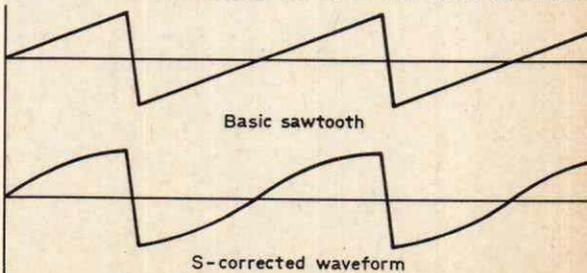
Fig. 7: Illustrating S-correction of line scanning.
