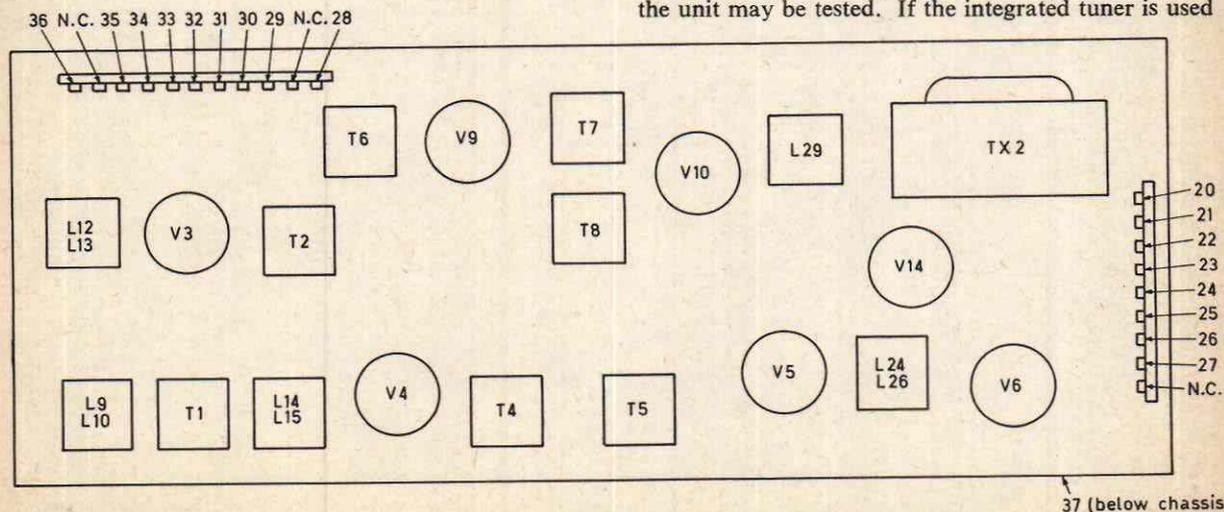
Fig. 1: Top layout of the panel, showing the tag connections.
