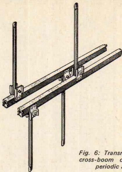
Fig. 6: Transmission-line cross-boom of the log-periodic aerial.
