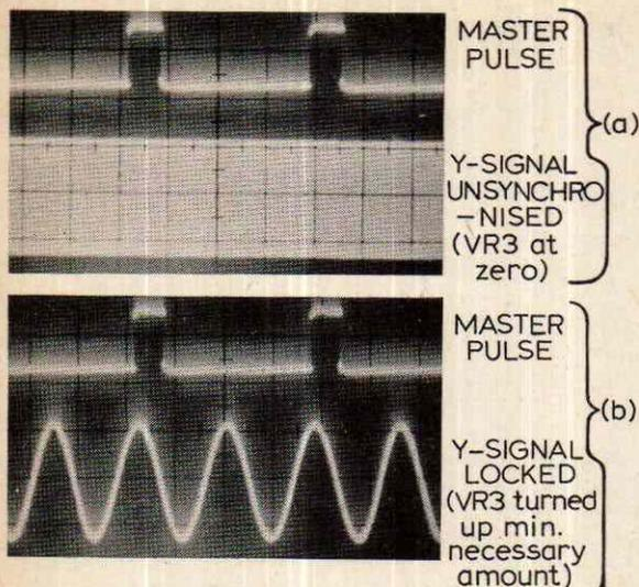
Note that master pulse here shortened to terminate with negative going zero transition of signal (S4 to negative sync polarity)
