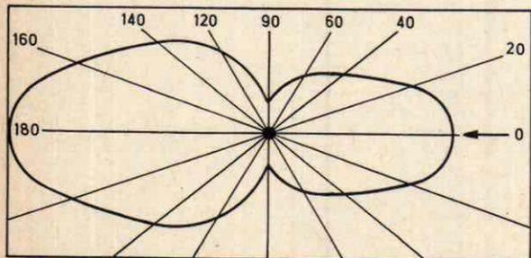
Fig. 5: Wrong design can cause a yagi to "back-fire" at certain frequencies within the bandwidth with a resulting impairment to the front-to-back ratio.
