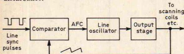
Fig. 5: Block diagram showing the basic operation of a flywheel line timebase.
