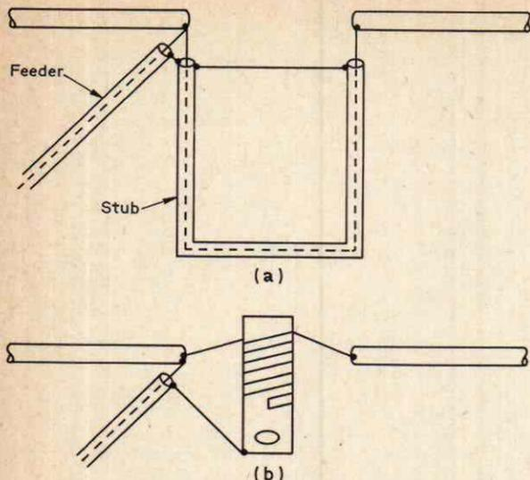
Fig. 4: Development of the J-Beam inverse balun: (a) shows the basic matching stub principle which gives a 75-ohm coax feed from the relatively higher terminal impedance of a skeleton slot radiator while (b) shows how J-Beam simulate the principle by means of a wound component.
