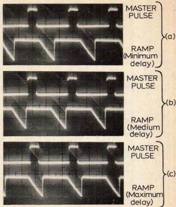
sive sync lock ranges overlap and an unlocked state is no longer possible. As the relative frequencies are changed cycles add or subtract abruptly without lock ever being lost. This automatic synchronisation persists up to signal repetition frequencies in the MHz range.
