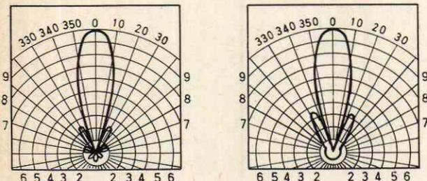
Fig. 1 (left): Horizontal polar diagram of 18-element yagi (including reflector system). This has a front-to-back ratio of about 26dB.
