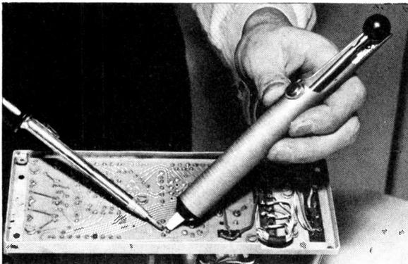
*The Picard "Abiko" desoldering gun in use.*
