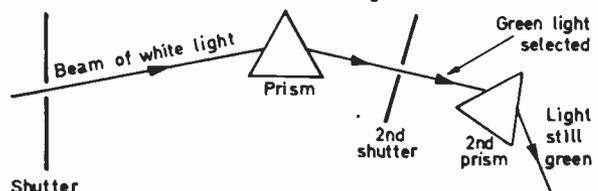
Fig. 2: Newton's second experiment. Once the white light had been separated into colours by a prism it could not be separated further by using another prism. This proved that the colours obtained were not something added to the white light by the glass of the prism.
