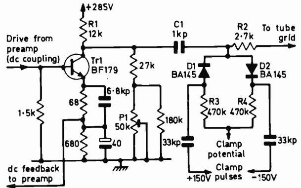
Fig. 5: Transistor colour-difference output stage with diode clamp. A similar circuit is used in the Korting chassis.
