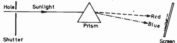
Fig. 1: Newton's first experiment. Sunlight had to be used as no artificial light then known was bright enough. The image on the screen was the shape of the hole in the shutter but with coloured edges.
