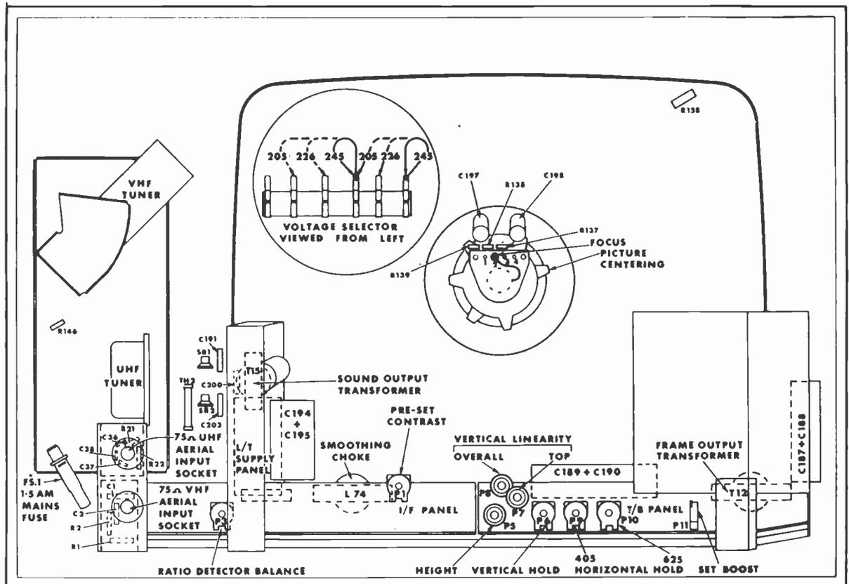
Fig. 1: Rear view of the receiver with the cabinet back removed.
