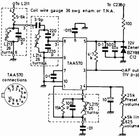
Fig. 6: Recommended circuit for use with the alternative sound i.c. type TAA570.
