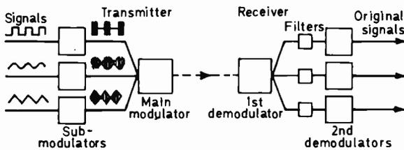
Fig. 9: Principle of frequency multiplexing. Each signal is modulated on to a separate subcarrier, each subcarrier being at a different frequency. The subcarriers are then added together and modulated on to a carrier for transmission. At the receiver the carrier is demodulated and the subcarriers separated by filters and then separately demodulated to give the original separate signals.
