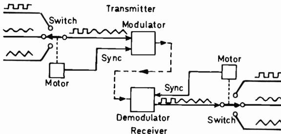
Fig. 10: Principle of time multiplexing. The transmitter and receiver contained synchronised switches. A portion of each waveform is transmitted in turn and in the receiver switched into the correct channel. Provided the switching frequency is higher than the frequency at which changes in the signals occur no information is lost.
