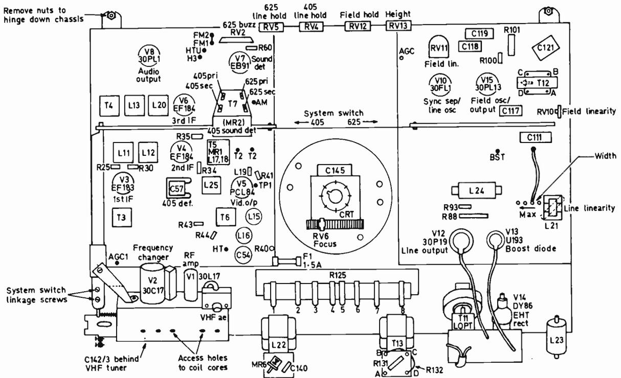
Fig. 1: Rear chassis layout showing components mentioned in the text.
