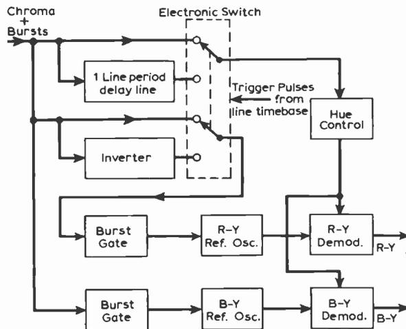
*Fig. 1: The chroma signal decoding system used in the Sony Model KV1320.*
