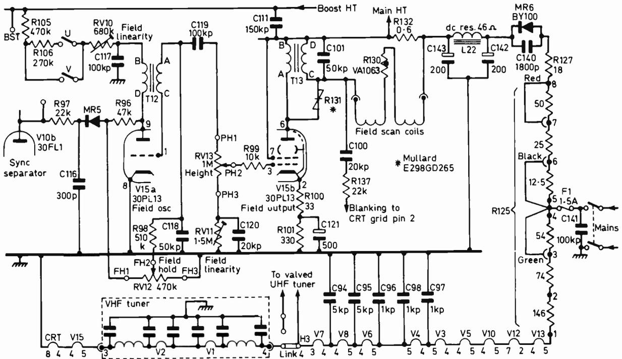
Fig. 2: The field timebase and power supply circuits of the Ekco Model T402. Minor component value variations in the blocking oscillator (V15a) and sync feed circuits may be found in some chassis. C117 charges slowly from the boost rail to give the field timebase waveform. C118, R98 and RV12 control the speed.
