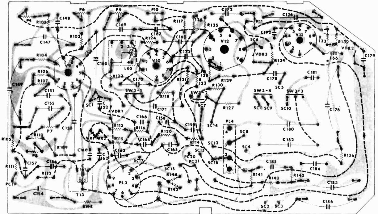
Fig. 2: Layout of the timebase printed board viewed from the tin-dip side.
