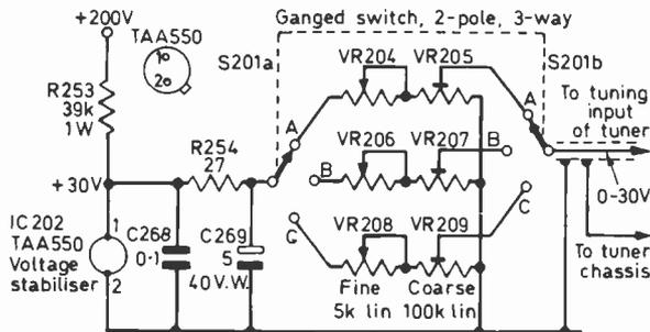
Fig. 1: Tuning arrangements for a varicap tuner.
