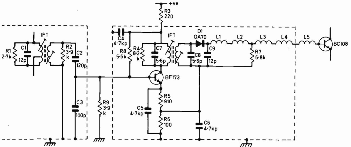
Fig. 2: Representative final vision i.f. stage (Philips 210 chassis). The potential developed at the junction of R5 and R6 provides forward bias for the BC108 video phase splitter, the positive-going output from the detector diode D1 being superimposed on this. Component functions and fault conditions with their associated symptoms are summarised in Table 1 below.
