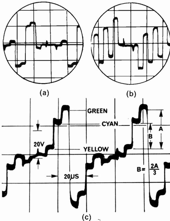
Fig. 6: Colour-difference grid drive signals for the standard colour-bar test pattern, (a) R—Y, (b) B—Y and (c) G—Y. The dimensions given on (c) indicate one way of setting up the G—Y matrix correctly.
