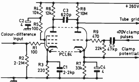
*Fig. 1: Pentode colour-difference output stage with triode clamp. With colour-difference drive each shadowmask tube grid is driven by a stage like this.*
