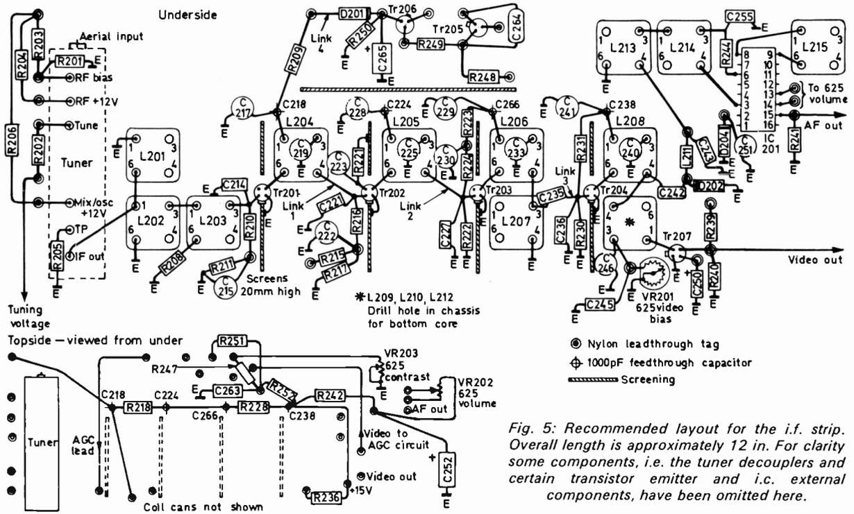
Fig. 5: Recommended layout for the i.f. strip. Overall length is approximately 12 in. For clarity some components, i.e. the tuner decouplers and certain transistor emitter and i.c. external components, have been omitted here.
