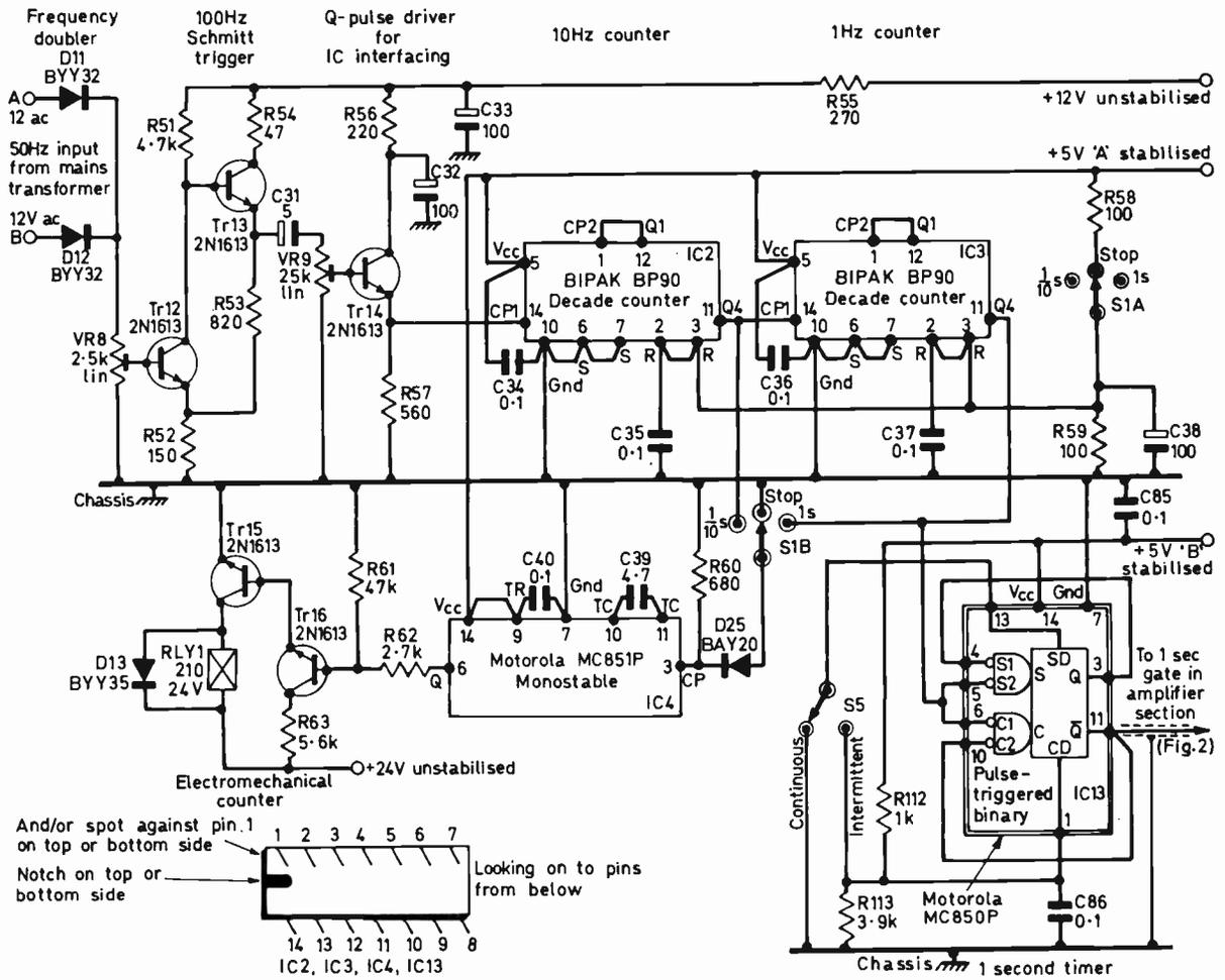
Fig. 3: Circuit of the time counter section of the frequency meter.
