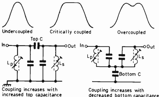
Fig. 4: The three possible bandpass response shapes and two possible types of bandpass circuit.
