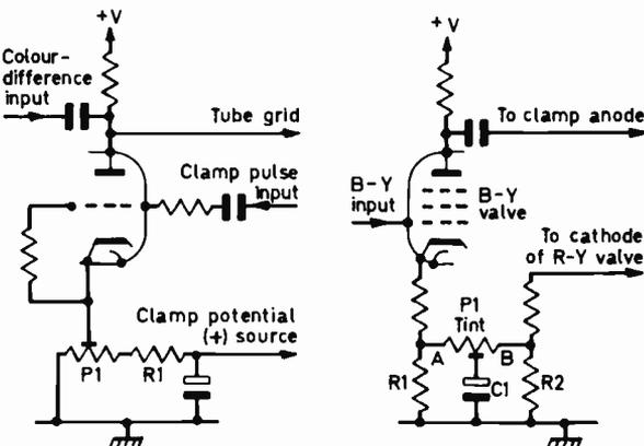
Fig. 3 (left): Clamp stage with preset clamp potential.
