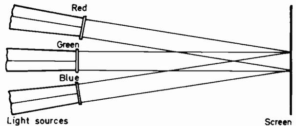
Fig. 4: Additive colour mixing. Sources of red, blue and green light are all directed to the same spot on the screen. The colour seen at this spot on the screen will depend on the proportions of the three primary colours used. Because the lights are added in parallel this is known as additive colour mixing.
