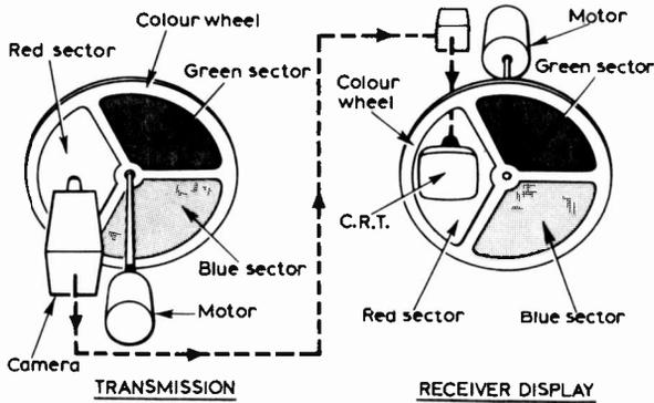
Fig. 6: Principle of early sequential colour systems. The colour wheel was common to all the early sequential colour systems and was the factor which contributed to their downfall. Synchronising difficulties, the high speed of the wheel in line-sequential systems and the non-compatibility doomed such systems to extinction.
