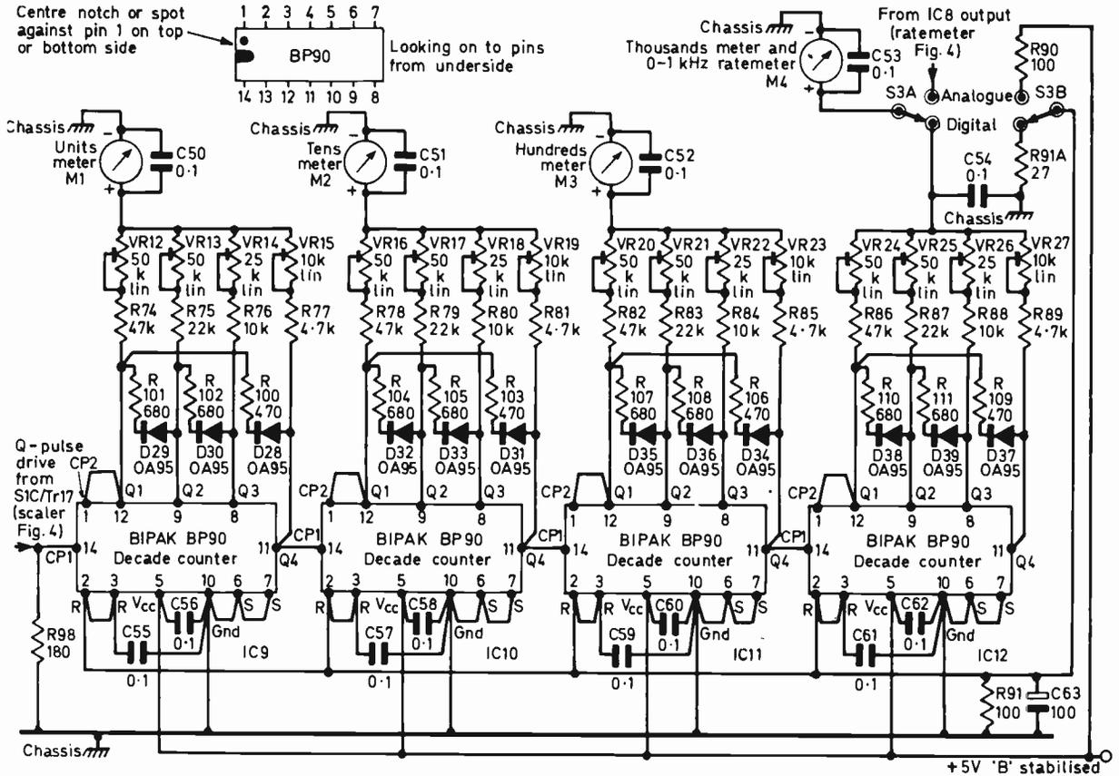
Fig. 5: Circuit of the frequency counter section of the meter.
