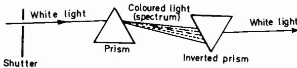
Fig. 3: Newton's third experiment. This showed that the white light split into its component colours by one prism could be reassembled by another prism.
