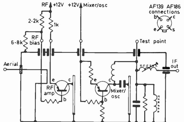
Fig. 2: Basic d.c. and signal paths in a typical "surplus" u.h.f. tuner using germanium transistors. The values of the external resistors are for guidance only and may require slight adjustment for optimum noise performance.
