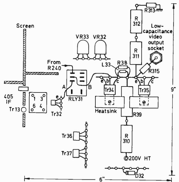
Fig. 3 (right): Suggested layout—as used in the prototype.
