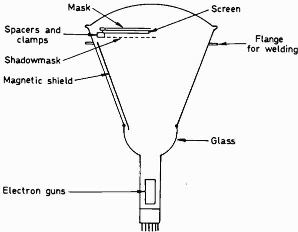
*Fig. 2: The early shadowmask tube. The glass face of the tube was not the screen but simply a transparent cover sealed to a metal ring on which were mounted the phosphor-dot screen and the shadowmask. This assembly was in turn welded to a metal cone to which the stem carrying the guns was sealed. The whole tube was adapted from the 16in. metal-cone tube used for black-and-white television for a considerable time (the same as the monochrome tube made in the UK at the time by English Electric).*
