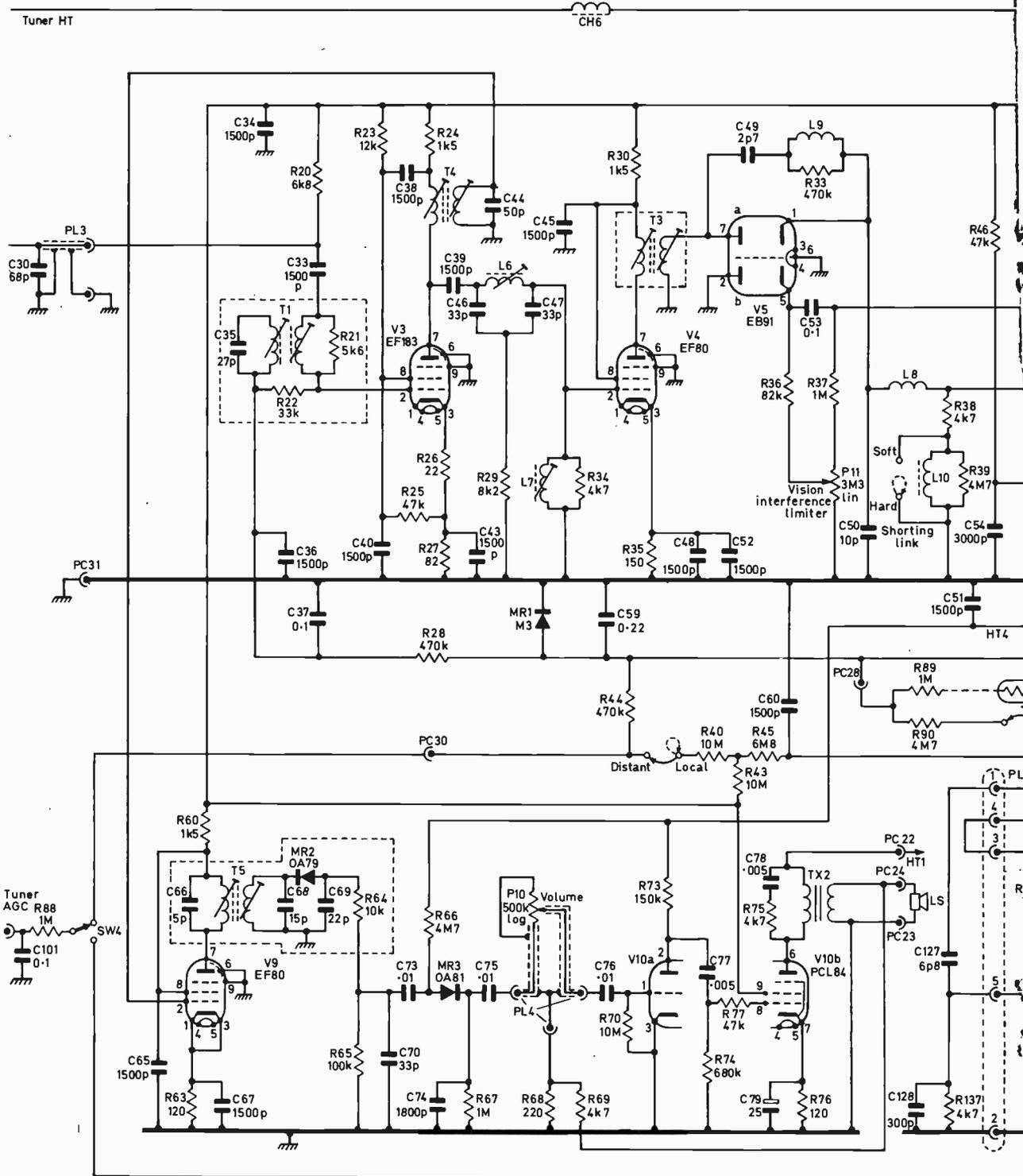
Fig. 1: Circuit diagram, Sobell ST282 series 625-line convertible models. CH6 is only present when a push-button
