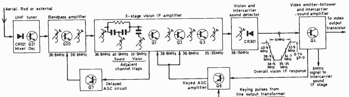
Fig. 1: Block diagram of the vision receiver sections of the Crown 7TV105 portable model.
