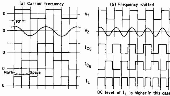
Fig. 3: Quadrature detector waveforms.
