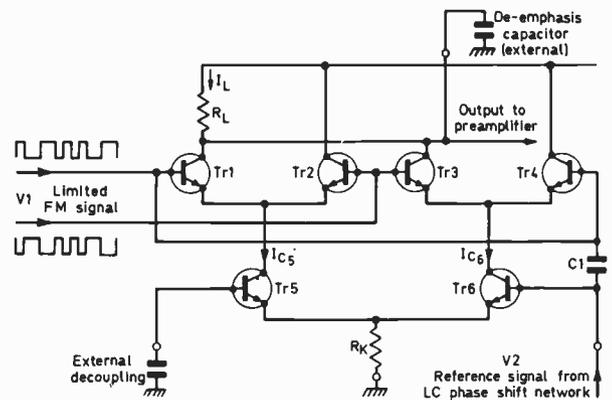
Fig. 2: The quadrature detector circuit. The external LC phase-shift network is driven by the signal fed to it via C1. The sine-wave signal from the phase-shift network drives Tr6 base and by emitter-follower action appears across its emitter resistor  $R_k$ . Thus Tr6 is driven at its base and Tr5 is driven at its emitter by the same basic waveform. This of course amounts to paraphase drive and Tr5 and Tr6 provide antiphase squarewave outputs.
