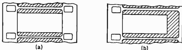
Fig. 2: Making the most of the 16mm. gauge. (a) Double-perforated 16mm. film—shaded area indicates loss of picture area when projected on a 1-85:1 cinema screen. (b) Single-perforated 16mm. film with sound track omitted, showing (shaded) the additional area available for photographing a 1-65:1 frame for television or a 1-85:1 frame for cinema release.
