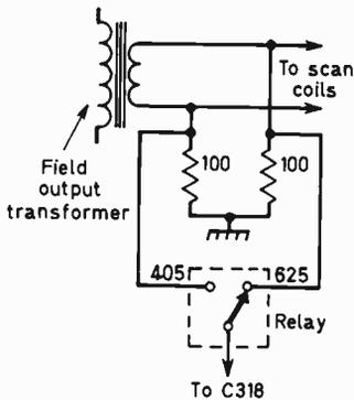
Fig. 2 (left): Because of the switched drive to the c.r.t. it is necessary to invert the polarity of the field blanking pulses on the two systems. The arrangement shown here provides the necessary blanking pulse inversion.
