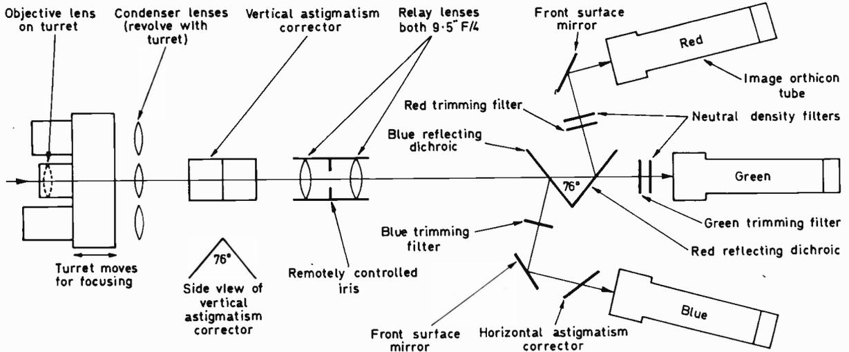
Fig. 4: The optical system used in the three-tube colour television camera developed by RCA.
