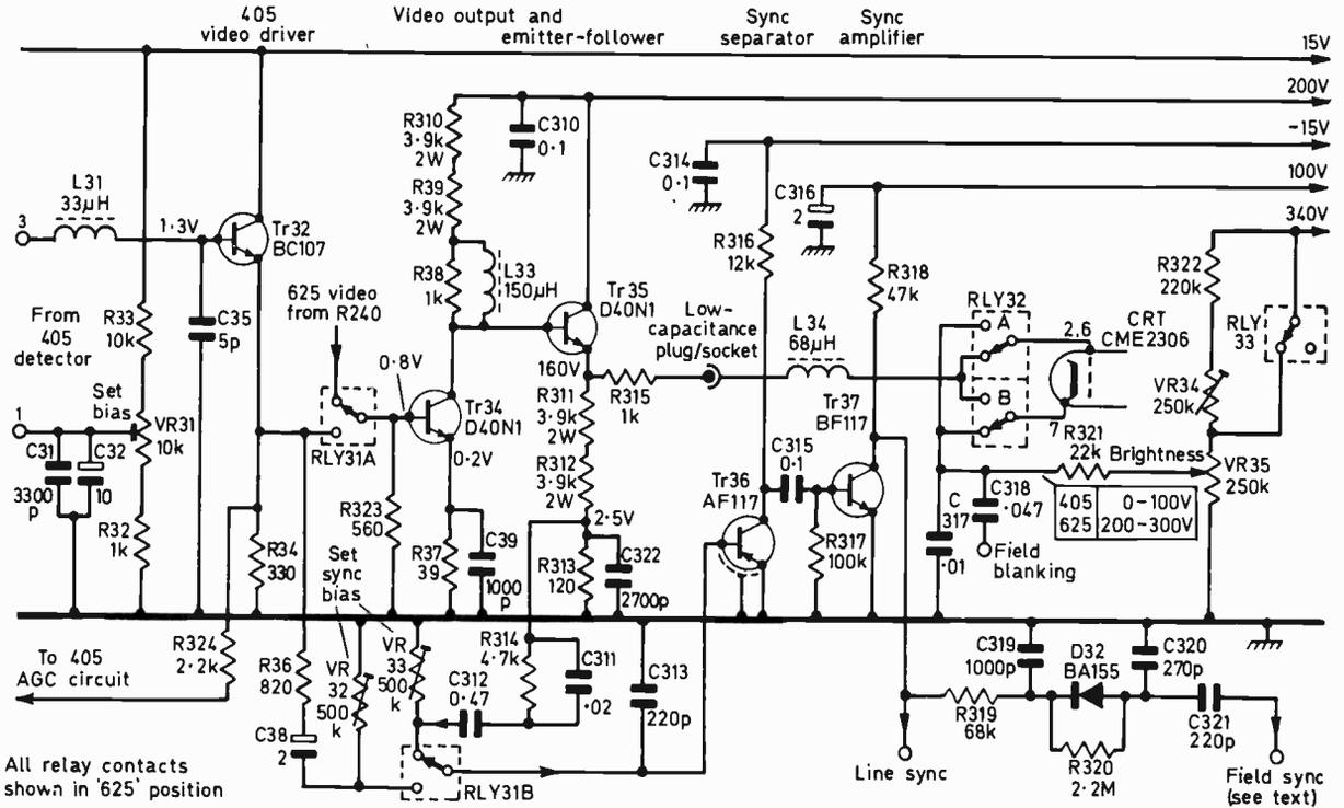
Fig. 1: The video and sync circuits. All relay contacts are shown in the 625-line position. The approximate voltages shown were measured with no signal, the line timebase operational and the video bias presets correctly adjusted, using a meter with an impedance of  $10k\Omega/V$ .
