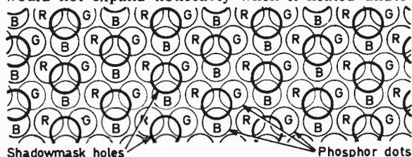
Fig. 1: Alignment of the holes in the shadowmask with the groups of phosphor dots on the screen.
