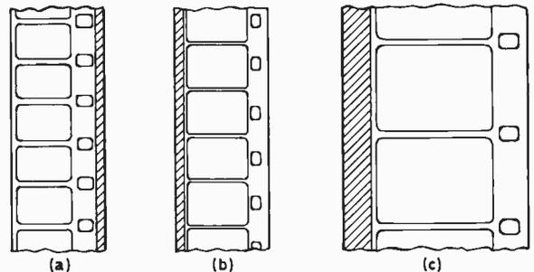
Fig. 1: Comparative picture areas—to same scale—of (a) standard 8mm. film, (b) super-8mm. and (c) 16mm. film, all with sound tracks on the prints. Super-8 has 52% greater area than standard 8.
