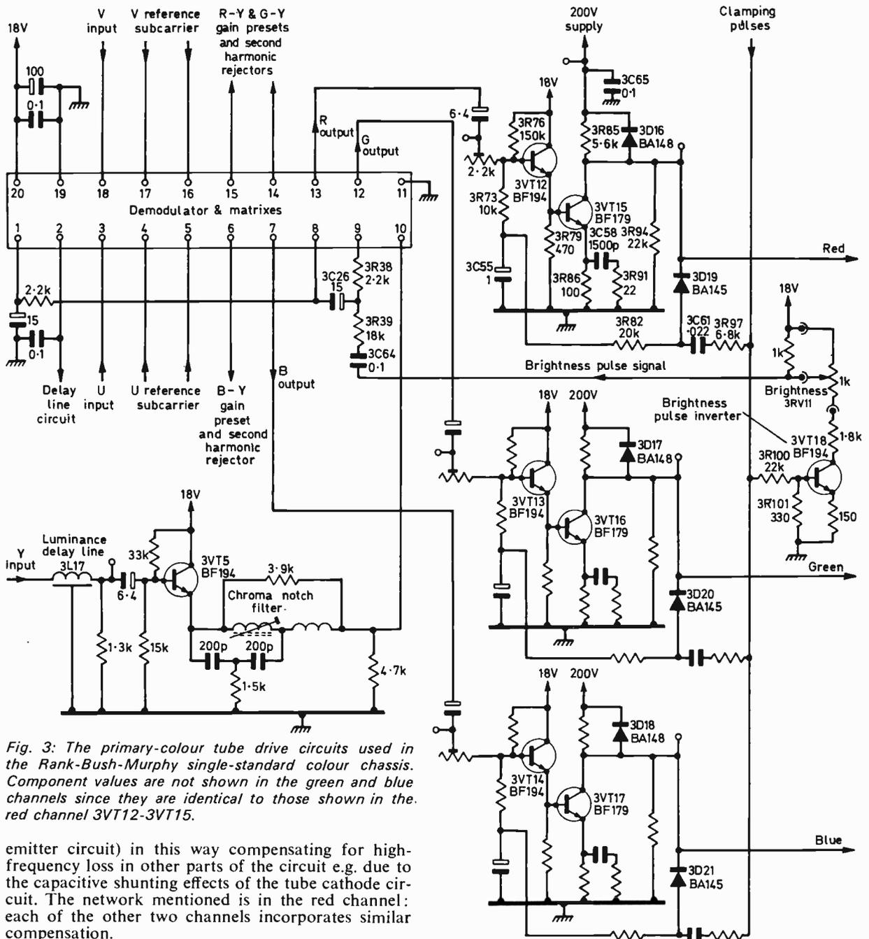
Fig. 3: The primary-colour tube drive circuits used in the Rank-Bush-Murphy single-standard colour chassis. Component values are not shown in the green and blue channels since they are identical to those shown in the red channel 3VT12-3VT15.
