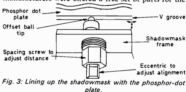
*Fig. 3: Lining up the shadowmask with the phosphor-dot plate.*
