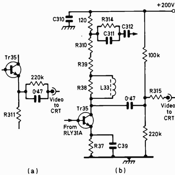
Fig. 4: Optional modifications to the basic circuit. (a) Circuit to reduce aircraft flutter. (b) A.C. coupling to the c.r.t., with the emitter-follower Tr35 omitted.
