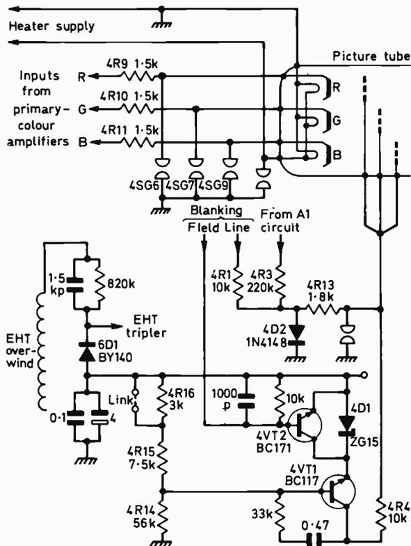
Fig. 1: The picture tube grid clamping, beam current limiting and line and field flyback blanking arrangements.
