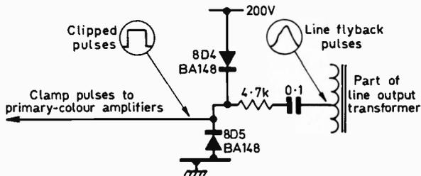
Fig. 2: Method by which the clamping pulses are obtained by clipping the line flyback pulses.
