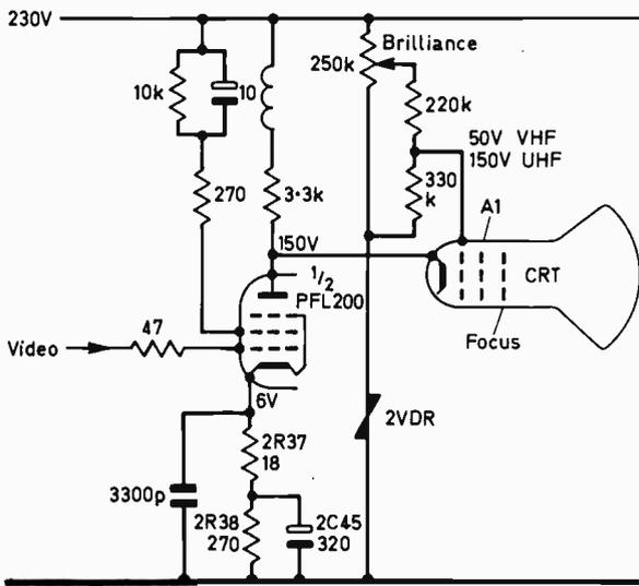
Fig. 4: Video output stage used in the Bush-Murphy TV161U-V1910U series. 2VDR provides switch-off spot suppression: as the h.t. falls on switch-off its resistance rapidly falls thereby quickly reducing the c.r.t. grid voltage.
