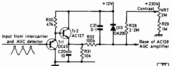
Fig. 5: The original sync tip a.g.c. circuit used in the Constructors' 625-line Receiver.
