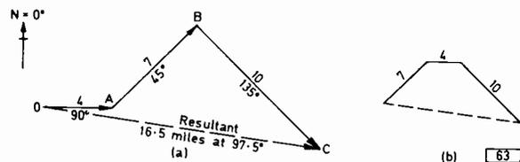
Fig. 1: Simple map reading (a) drawn in the form of a vector diagram. Note that precisely the same answer will be obtained if the vectors are drawn in a different order, as shown for example at (b).
