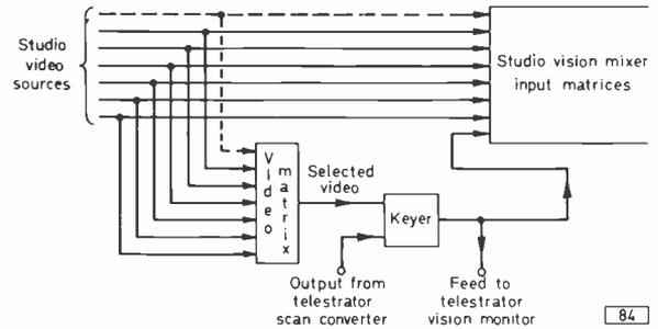
Fig. 4: How the Telestrator output is used with the studio system.
