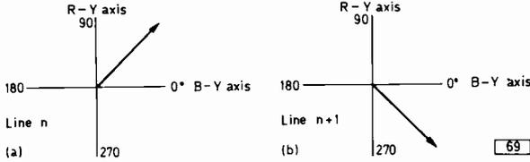
Fig. 7: The phase angle of the chrominance subcarrier on two successive lines for a magenta hue.
