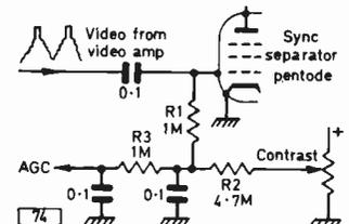
Fig. 2: Typical mean-level vision a.g.c. circuit. The negative potential developed at the grid of the sync separator is used as the a.g.c. source.
