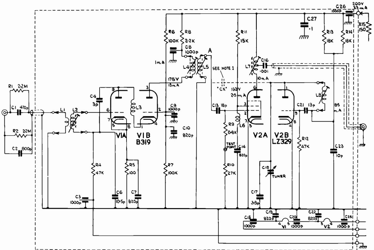
Fig. 3: Circuit of the turret tuner. Note 1: Capacitor CX consists of stray capacitance supplemented on Ban 1 III by a loop around L8 connected to point A.
