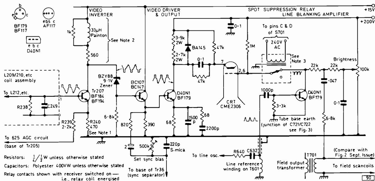
Fig. 6: Video circuit for single-standard (625 lines) operation. Notes: (1) R240 470Ω in this circuit. (2) Additional components in Tr207 collector lead. (3) Spot suppression relay—same type as in Fig. 5.
