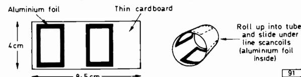
Fig. 7: Line linearity sleeve construction.
