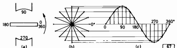
Fig. 5: Electronic vectors are assumed to be rotating anticlockwise. We stop them at a given instant in time in order to compare their amplitudes and phases.
