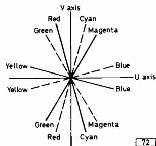
Fig. 10: A true vector diagram showing the phase angles and amplitudes of the chrominance subcarrier on successive lines for the primary and complementary colours.
