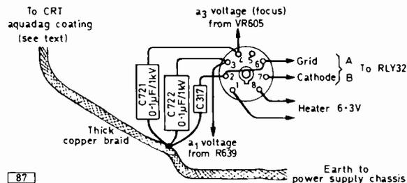
Fig. 3: CRT base connections (CME2306/A59-16W).
