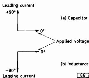
Fig. 4(a): Vector diagram equivalent to Fig. 3: it's much easier to draw! (b) Conditions when a sine-wave voltage is applied to an inductor instead of a capacitor.
