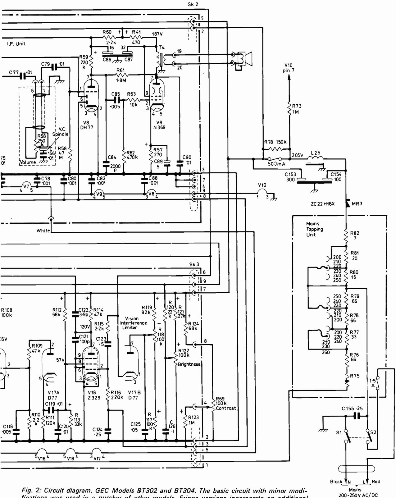
Fig. 2: Circuit diagram, GEC Models BT302 and BT304. The basic circuit with minor modifications was used in a number of other models. Fringe versions incorporate an additional common i.f. stage.
