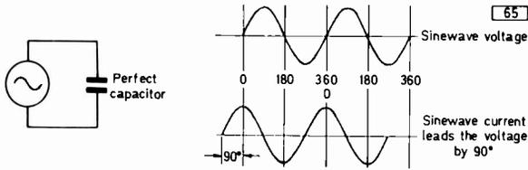
Fig. 3: A sinewave voltage applied to a perfect capacitor causes a current which leads the voltage by 90°.
