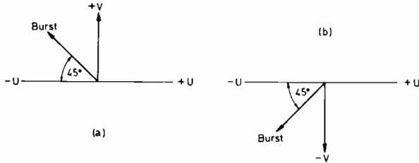
Fig. 2: How the phase of the V component of the chroma signal is inverted on alternate lines in the PAL system—(a) odd lines, (b) even lines with inverted V. The bursts swing about the  $-U$  axis on alternate lines.
