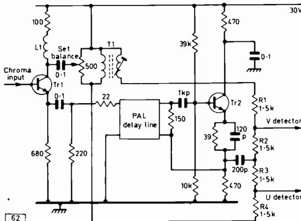
Fig. 7: In this circuit a resistive add and subtract network (R1-R4) is used in conjunction with a post delay line amplifier stage.
