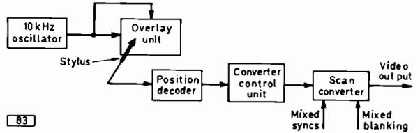
Fig. 3: Simplified block diagram of the Telestrator system.
