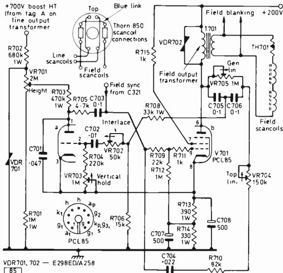
Fig. 1: Suggested field timebase circuit.
