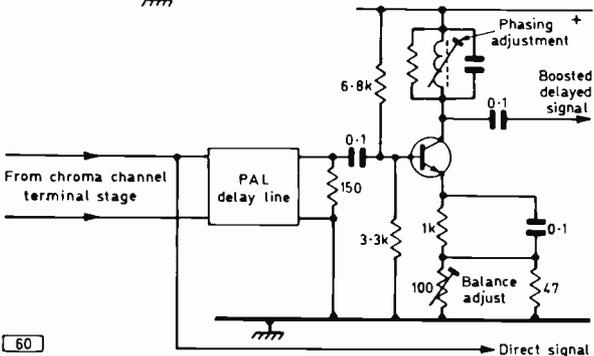
Fig. 5 (below): Circuit in which a post delay line amplifier is used to make good the insertion loss introduced by the delay line.
