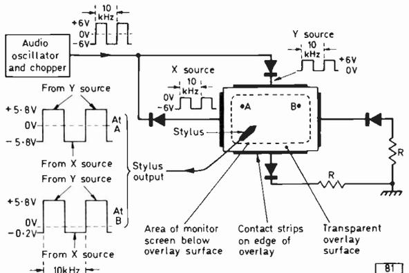
Fig. 1: Telestrator position detector.
