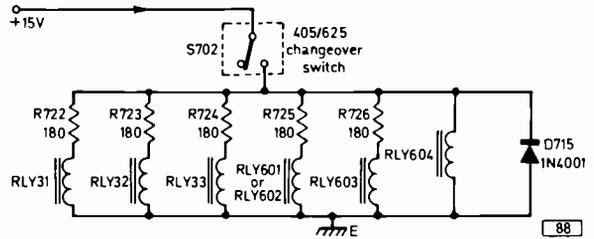
Fig. 4: Relay coil wiring.
