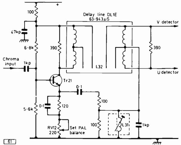
Fig. 6: With more recent types of delay line the summing networks are contained in the delay line housing.
