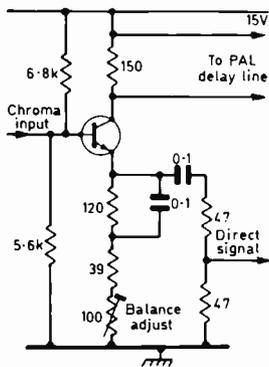
Fig. 4: It is more common to drive the delay line from the collector of the delay line driver stage and to tap the direct signal from its emitter circuit.
