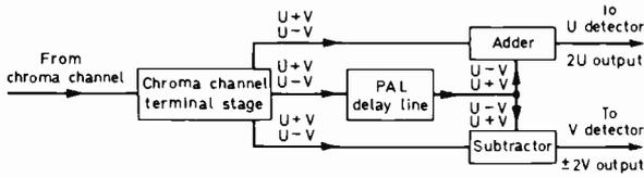
Fig. 1: Block diagram showing how the U and V signals are separated in a PAL decoder by using add and subtract matrix networks and a PAL delay line.
