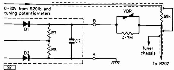
Fig. 8: Correct a.f.c. circuit connections.
