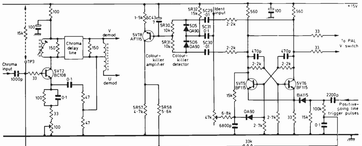
Fig. 1: The colour-killer circuit used in the Bush-Murphy dual-standard colour chassis.
