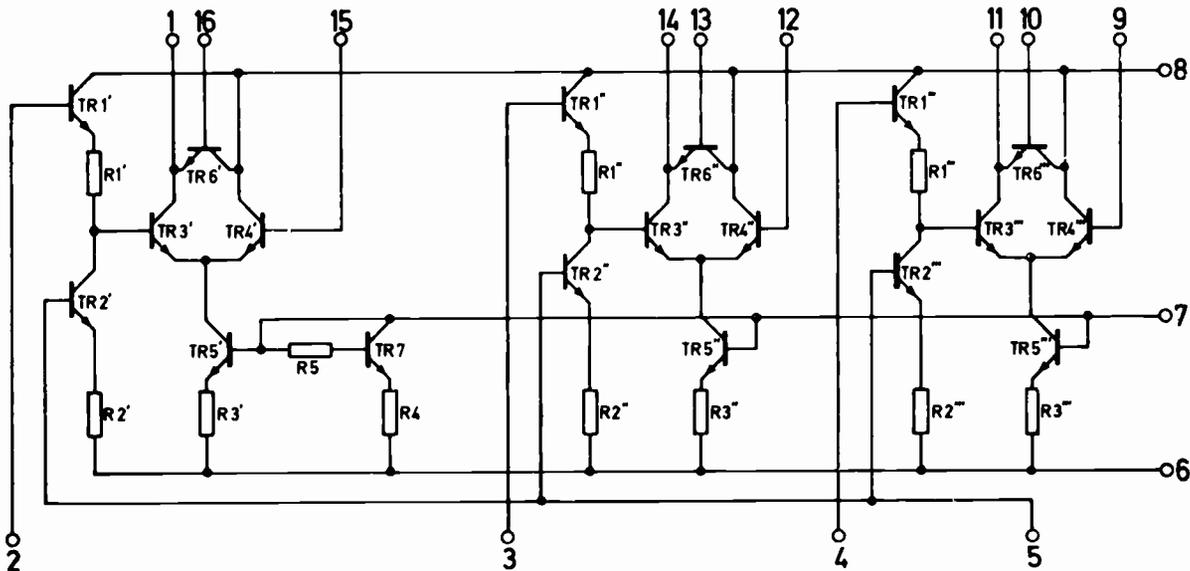
Fig. 2: Internal circuit of the TBA530Q i.c.
