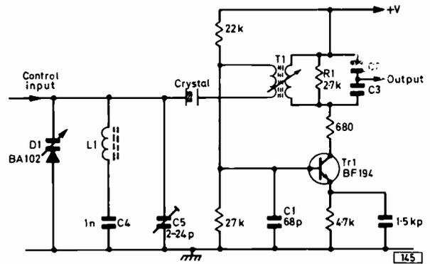
Fig. 4: The reference oscillator circuit used in the Philips G8 single-standard chassis. The crystal is in the feedback circuit.
