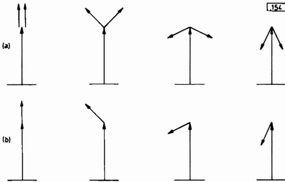
Fig. 6: A double-sideband signal (a) and a single-sideband signal (b) with the lower sideband removed.
