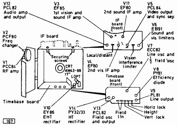
Fig. 5: Chassis layout, 506T series.
