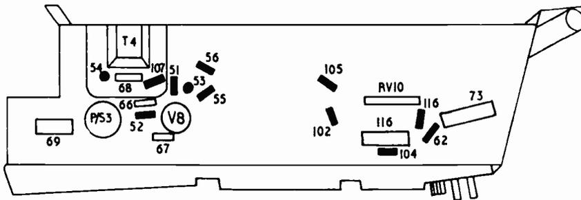
Fig. 1: View of top chassis from above (resistors shown solid black).
