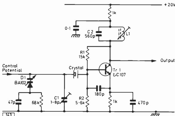
Fig. 2: Typical crystal-controlled reference oscillator circuit (Baird 700 series).
