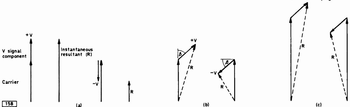
Fig. 10: Imperfect demodulators are not immune to quadrature crosstalk or phase errors in the subcarrier. (a) Correct signal phase. (b) With phase error  $\beta$  the resultant is changed as shown here. (c) Using a larger amplitude reference carrier the effect of the errors shown at (b) is reduced.
