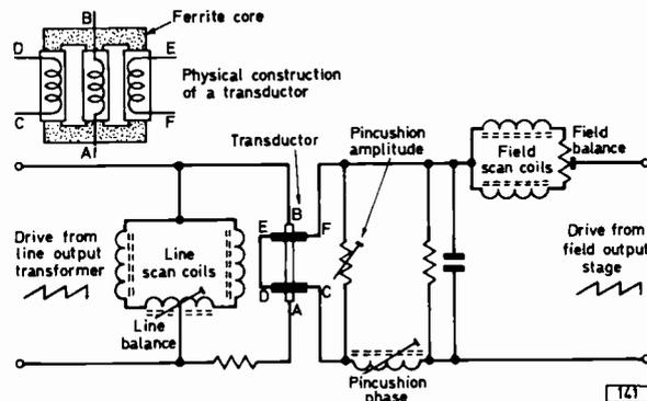
Fig. 6: Simplified  $90^\circ$  pincushion correction circuit.
