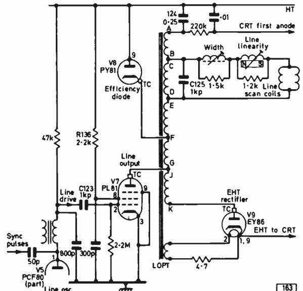
Fig. 1: Line output stage, Models 306T and 308T.
