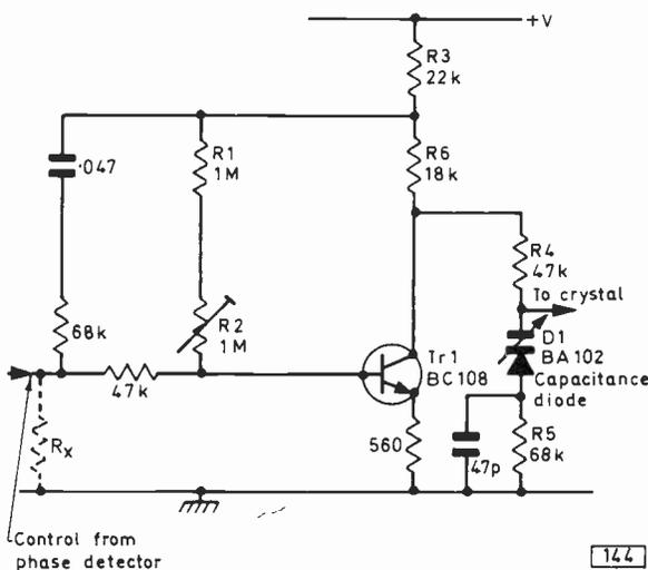
Fig. 3: D.C. amplifier which operates between the phase detector and the crystal oscillator circuits.
