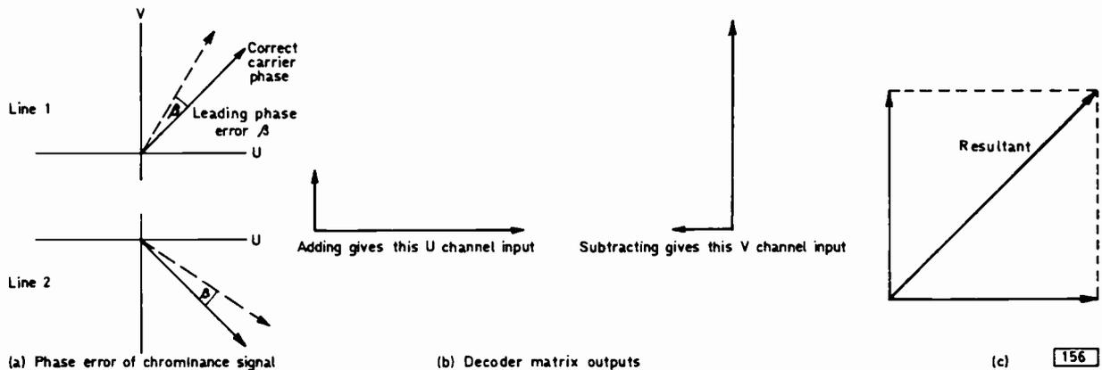
Fig. 8: Phase distortion of the chrominance signal is cancelled in a delay line PAL decoder provided the demodulation axes are scrupulously accurate. The resultant decoder output shown at (c) is at correct phase (hue), but only if demodulation is correctly on axis: saturation is slightly reduced.
