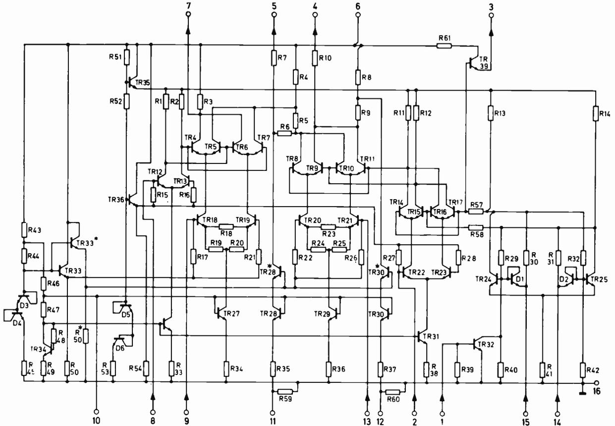
Fig. 4: Internal circuit of the TBA520Q chrominance demodulator, G-Y matrix and V switch i.c.
