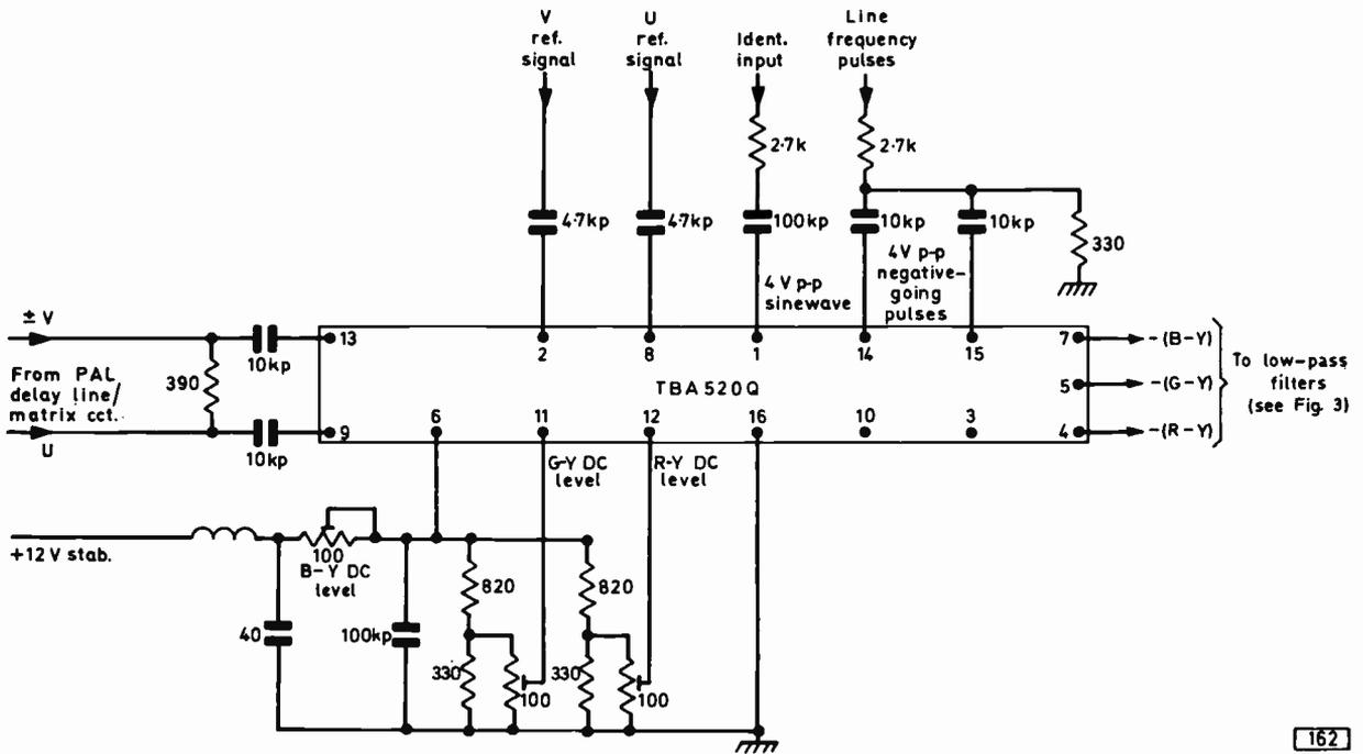
Fig. 5: External connections to the TBA520Q i.c. as used in the Philips G8 chassis.
