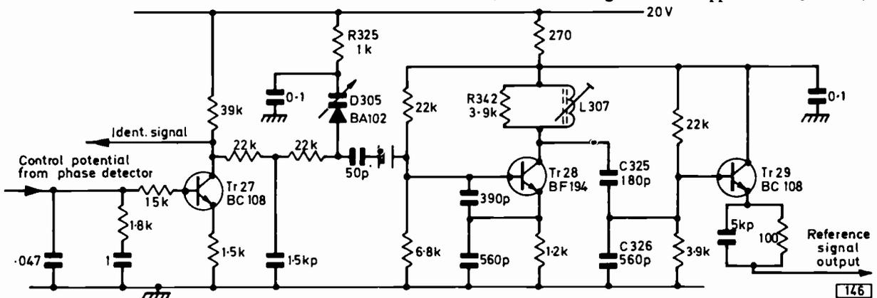
Fig. 5: D.C. amplifier, reference oscillator and buffer amplifier circuits used in GEC dual-standard models.
