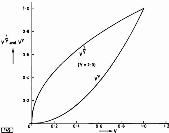
Fig. 1: How the gamma correction applied at the transmitter (top curve) compensates for the characteristics of the c.r.t. (lower curve). For simplicity it has been assumed that gamma is 2: in practice it is normally in the range 2.7–3.
