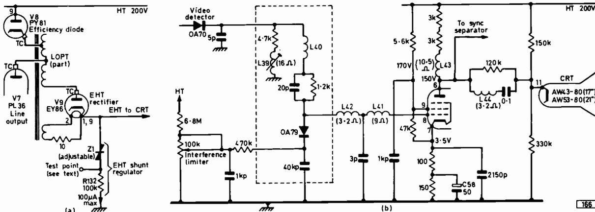
Fig. 4: E.H.T. circuit (a) and video output stage (b), Models 406T and 408T. D.C. resistances are approximate.
