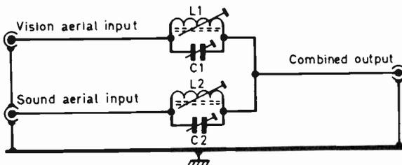
Fig. 1: Diplexer for channel F2.
