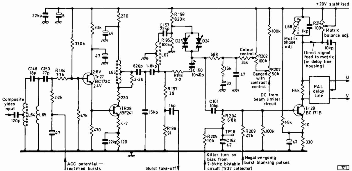
Fig. 1: The chrominance amplifier circuitry of the ITT/KB CVC5 chassis.
