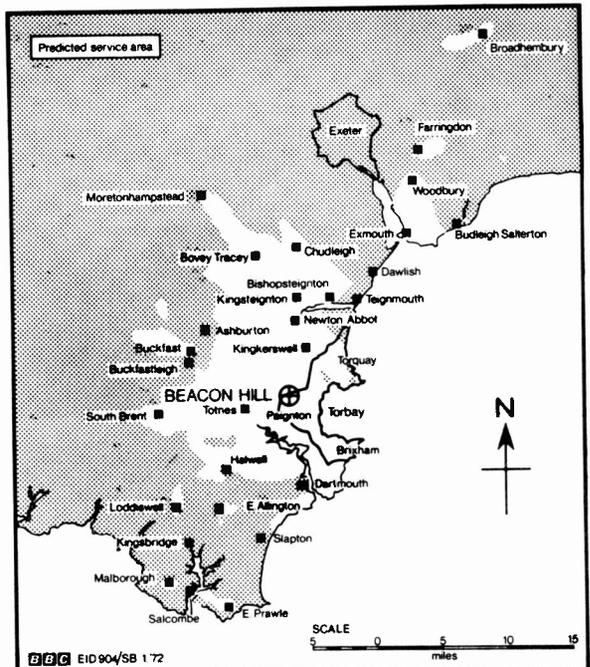
The unshaded portion of the above map shows the expected service area. Channels: Fourth 53, BBC-1 57, ITV 60, BBC-2 63. Polarisation horizontal, receiving aerial group C, maximum e.r.f. 100kW. Map courtesy BBC Engineering Information Service.
