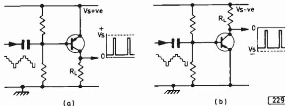
Fig. 1: A video signal with negative-going sync pulses is required to drive a pnp transistor used as a sync separator. Whether the transistor is fed from a positive or a negative rail we get an output consisting of positive-going sync pulses.
