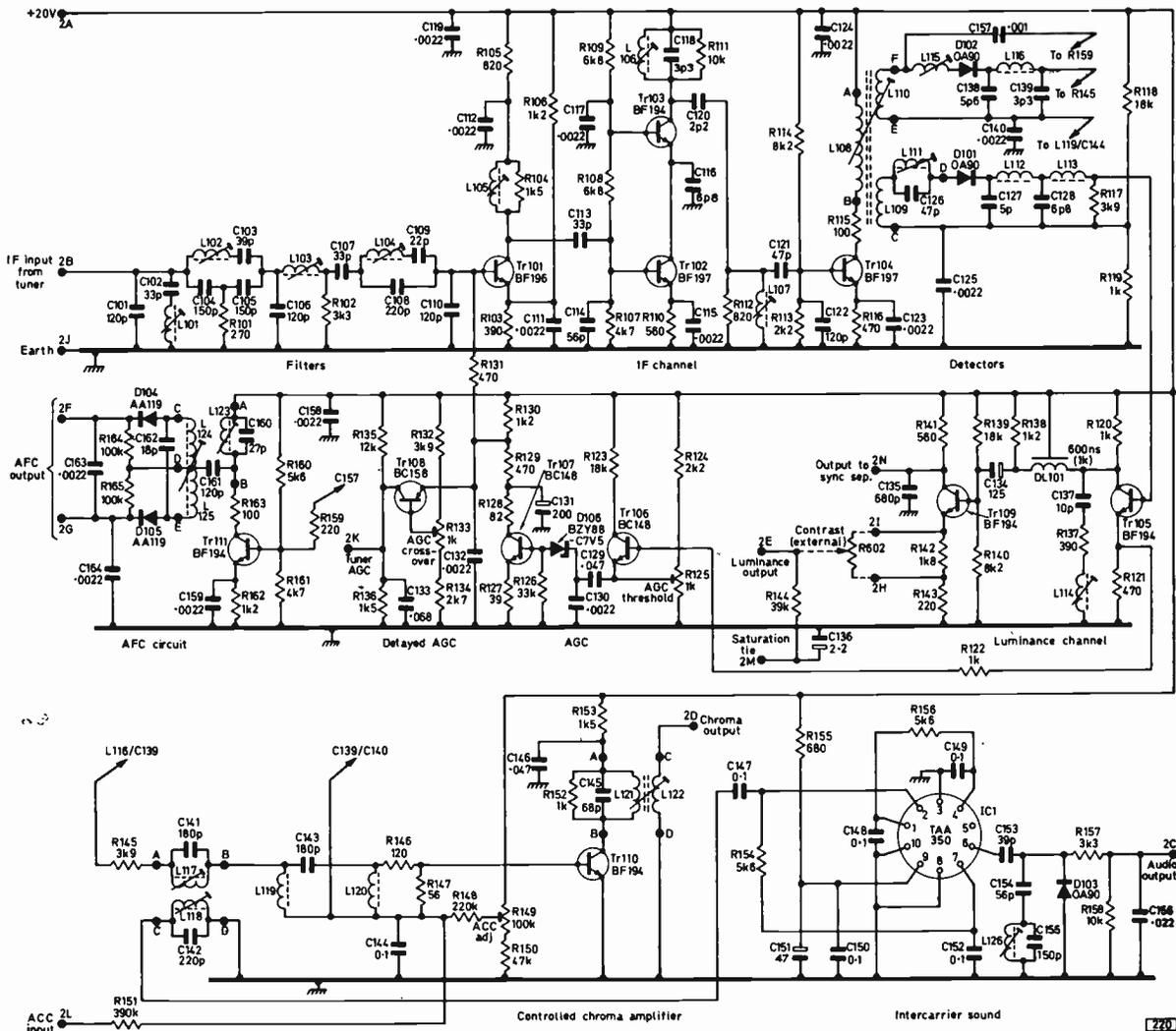
Fig. 7: Complete circuit diagram of the i.f. strip for the Television colour receiver. The strip incorporates the luminance channel, the a.g.c. circuits, the a.f.c. circuit, the intercarrier sound channel and the first chrominance amplifier. C138 may be 5pF.
