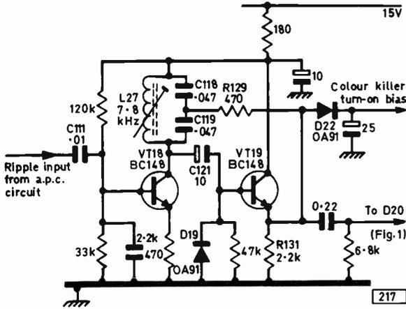
Fig. 2: The V switching must be synchronised and for this purpose the ident circuit shown here (Pye 691 chassis) generates a 7.8kHz sinewave from the phase swings of the transmitted burst signal.
