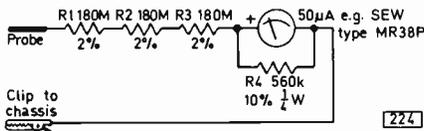
*Fig. 3: Suggested e.h.t. meter circuit*
