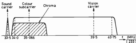
Fig. 1: The i.f. signal distribution (note that the actual transmitted signal is reversed—the sound carrier is at vision carrier plus 6MHz; reversal occurs as the result of the action of the mixer stage in the tuner).
