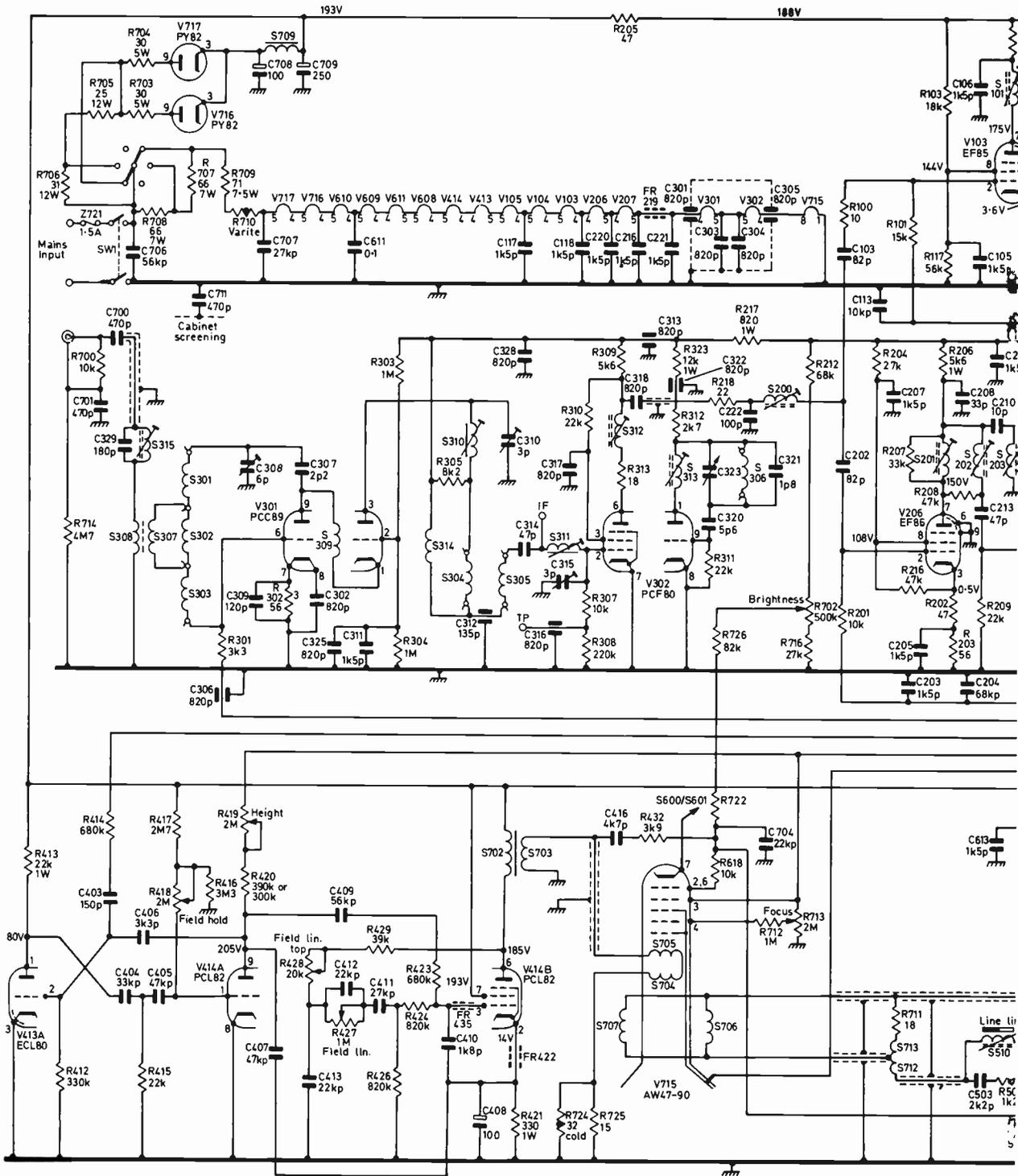
Fig. 3: Circuit diagram, Philips Model 19TG108U. Voltages shown measured using a 20,000 Ω/V meter.
