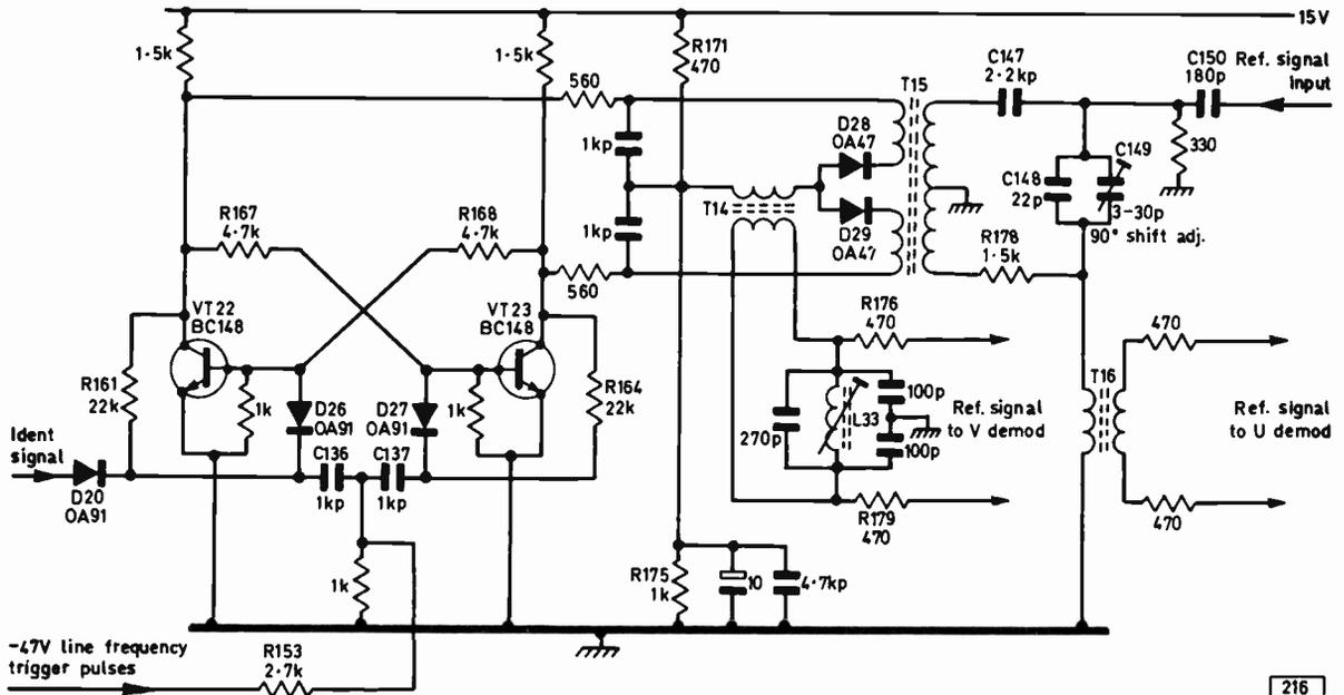
Fig. 1: Typical PAL V switch circuit (T15 with D28 and D29) and its controlling bistable circuit (VT22 and VT23) which provides antiphase squarewave outputs to switch the diodes D28 and D29 alternately on and off. In this circuit (Pye 691 chassis) it is the reference signal to the V demodulator that is switched line by line.
