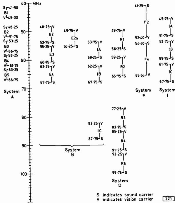
**System A:** 405 lines, positive vision modulation, a.m. sound. (UK, Eire.)
