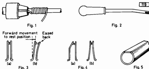
Fig. 1: Using a wheelbrace to wind a spring. The end is anchored securely in the chuck and the wire kept taut and pulled backwards to ensure close turns.
