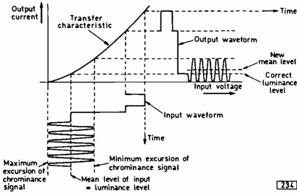
Fig. 2: With a common luminance and chrominance signal detector the non-linear transfer characteristic of the diode produces the form of distortion shown here.
