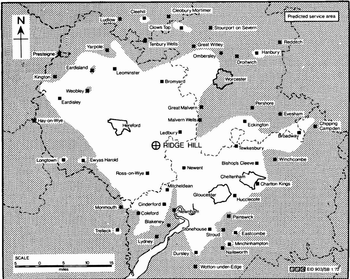
The expected area of the Ridge Hill u.h.f. services is indicated by the unshaded part of the above map. Channels are BBC-1 22, ITV 25, BBC-2 28, fourth 32. Polarisation is horizontal, receiving aerial group A, maximum e.r.p. 100kW. Map courtesy BBC Engineering Information Service.
