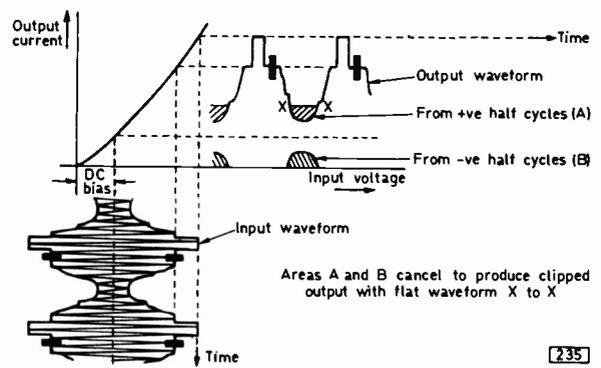
Fig. 3: This shows why applying d.c. bias to a common luminance/chrominance detector diode will not give a linear detection characteristic.
