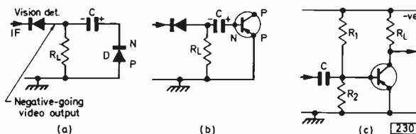
Fig. 2: Basic sync separator action. (a) Capacitor charged via diode D. (b) The np base-emitter junction of the transistor is equivalent to diode D in (a). (c) Basic pnp transistor sync separator circuit. The key to the operation of a transistor sync separator is the time-constant of its base circuit: this is arranged so that the transistor is cut off during the picture information but is driven into saturation by the sync pulses.
