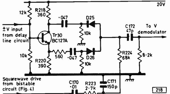
Fig. 3: The PAL V switch used in the ITT-KB CVC5 chassis uses a pair of switching diodes (D25 and D26) in conjunction with a transistor phase splitter (Tr30). In this chassis it is the signal feed to the V demodulator that is inverted on alternate lines.
