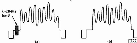
Fig. 1: The same composite video waveform at the video detector as displayed (a) by an oscilloscope with a 6MHz bandwidth, using a low-capacitance r.f. probe, and (b) by a cheap oscilloscope with a 3MHz bandwidth connected without a probe. Note the failure to resolve the 4.43MHz burst in (b).
