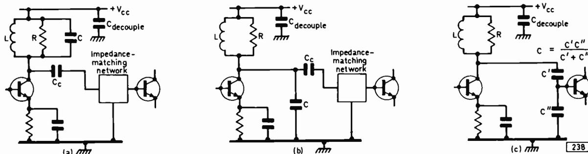
Fig. 6: Impedance matching by using tapped tuned circuit capacitance (d.c. biasing arrangements not shown).
