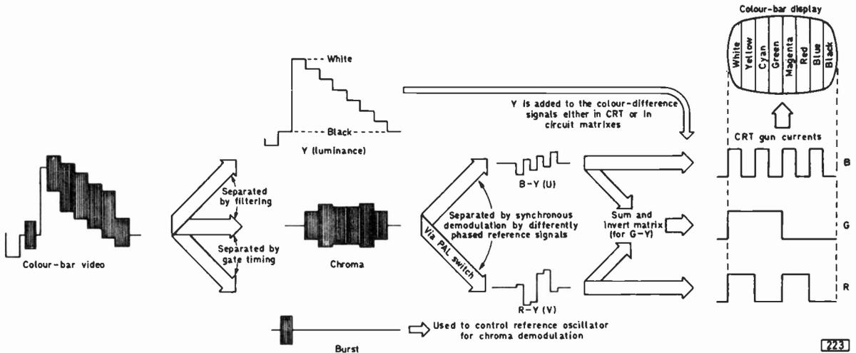
Fig. 2: Simplified representation of the processes in which the composite video signal is decoded to give a colour display. Factors glossed over here include the use of a delay line for initial U and V signal separation and the coefficients in the basic colour equations.
