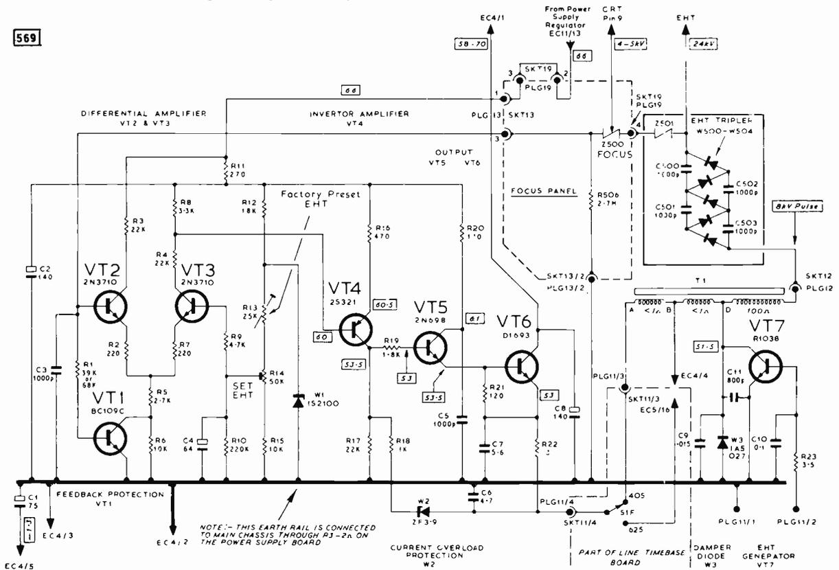
Fig. 4: The e.h.t. generator, regulator and focus circuit. Note that EC4/2 connects to the main chassis via EC10/18 and R3 on the power supply board.
