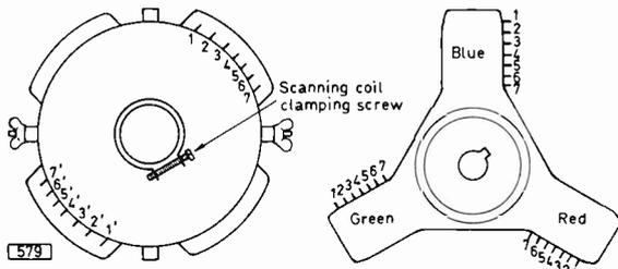
Fig. 4 (left): Connection numbering and interconnections required for all deflection units. Interconnections to be made: field, 5 to 4, 5' to 4', 3 to 6' and 6 to 3', with input from 4F on the timebase panel to 3 and return from 3' and 6 to R427 on the convergence panel at 5M and 5N (see Fig. 3, page 17, November issue); line, 1 to 2, with input to 1 from 5B and return from 2' and 1' to L402 via 5D and 5C on convergence board.
