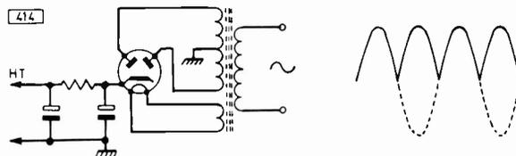
Fig. 1 (left): Basic full-wave power circuit, with valve rectifier.
