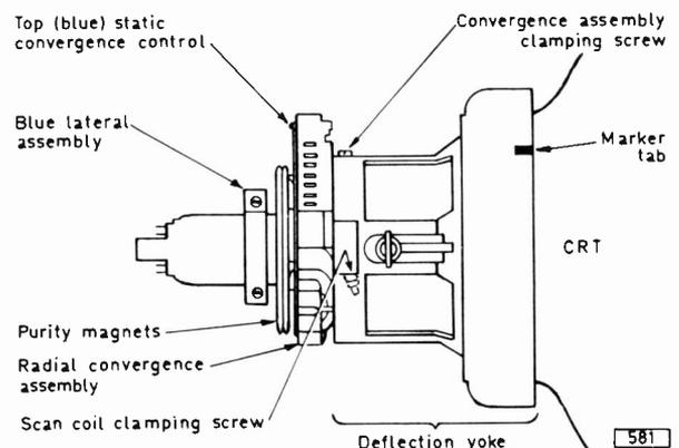
Fig. 1: General arrangement of the tube neck components using the AT1022 type deflection yoke. Note that on this series the marker tab is red; on AT1027 and AT1029 assemblies with convergence "rider" units (see text) the tab is blue.
