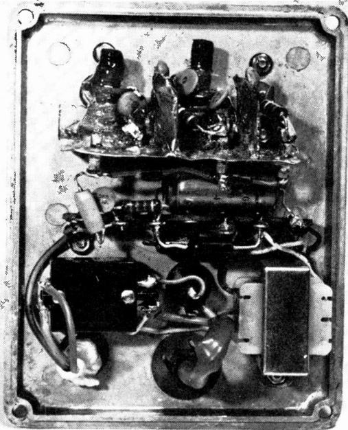
Internal view of the prototype preamplifier.
