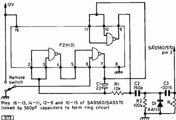
Fig. 4: Use of an FZ101 i.c. as a clock pulse generator to apply remote control to the Siemens touch-tuning i.c.s.
