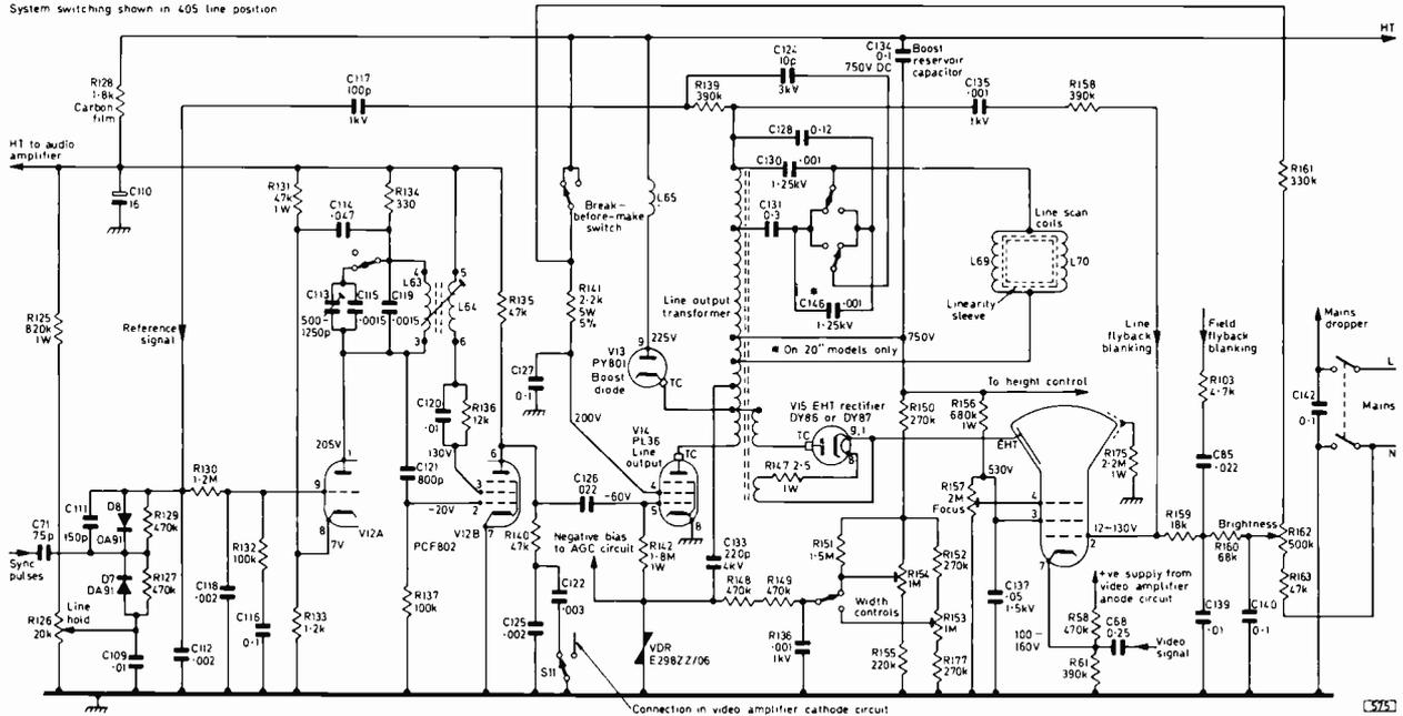
Fig. 1: Line timebase and c.r.t. circuit, STC VC52 chassis. The same basic circuit with only minor component value changes was used from the VC2 chassis on. In earlier chassis the arrangement of S11 is slightly different and the S-correction capacitor C130 is 0.0022 $\mu$ F (3kV).
