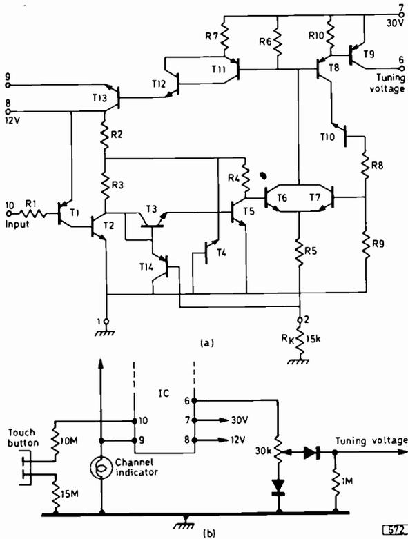
Fig. 3: (a) One of the switch channels of the Siemens SAS560/SAS570 bipolar touch-tuning i.c. series. (b) External connections to the i.c.
