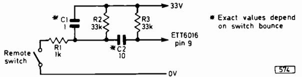
Fig. 5: Circuit for applying remote control to the Emihus ETT6016 m.o.s. touch-tuning i.c.
