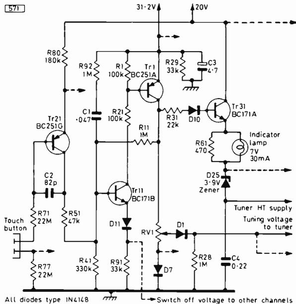
Fig. 2: Circuit of one of the six touch-button controlled switch channels in the tuner control unit used with the ITT CVC7 chassis (fitted in the KB Feathertouch 100 colour receiver).
