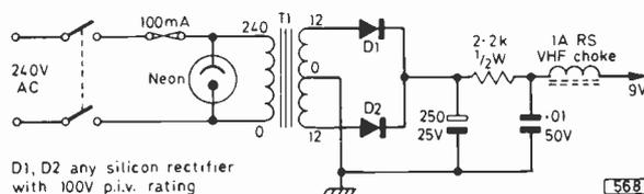
Fig. 2: A full-wave mains power supply was used (T1 is an Eagle miniature mains transformer with 240V primary and 12-0-12V secondary at 100mA). A half-wave circuit could be used if more convenient.
