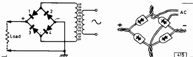
Fig. 3 (left): Basic bridge rectifier circuit. Rectifiers 1 and 4 conduct on one half cycle of the input, rectifiers 2 and 3 conducting on the other half cycle.
