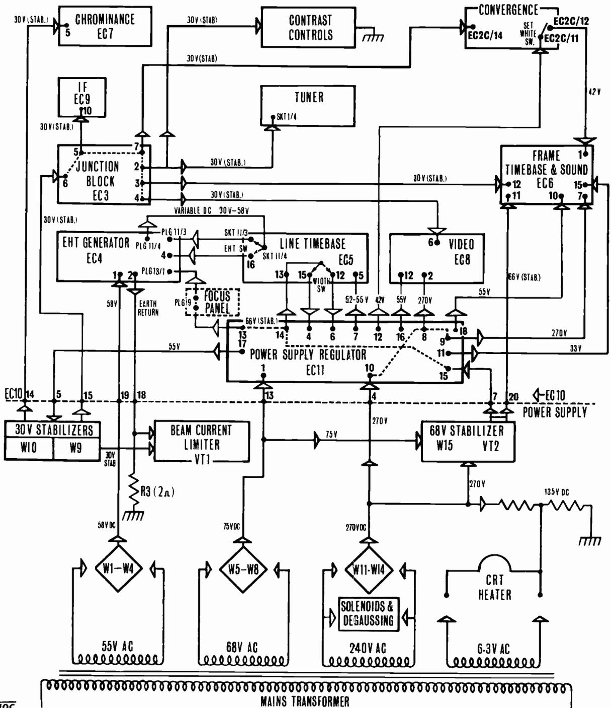
Fig. 6: Power distribution. The voltages shown are nominal.
