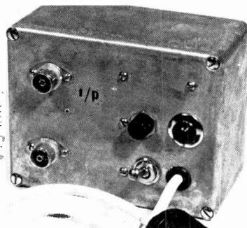
The prototype is housed in an Eddystone diecast box.
