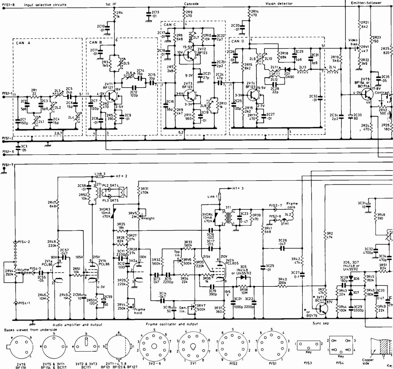
Fig. 1: Circuit diagram, Bush TV181S/Murphy V2016 series. Models include the Bush
