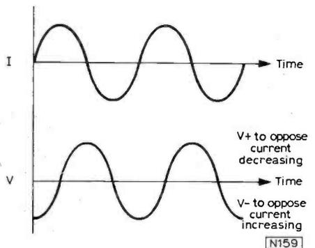
Fig. 9: Relative phase of the current and induced e.m.f. in an inductor.
