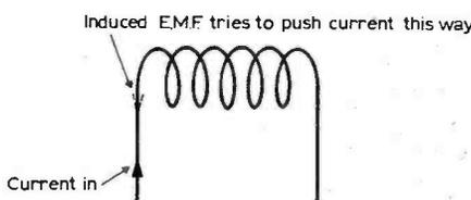
Fig. 7: The induced e.m.f. opposes the direction of current flow which caused it.
