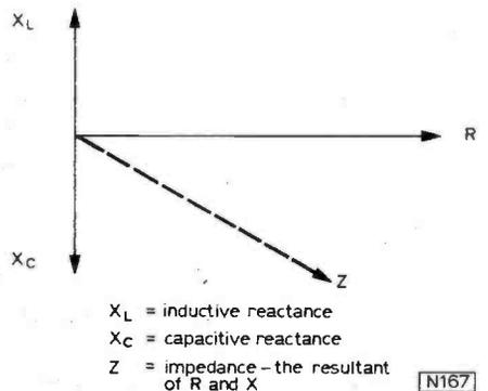
Fig. 17: Phasor diagrams are often plotted in Resistance ( $R$ ), Reactance ( $X$ ) and Impedance ( $Z$ ).
