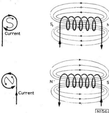
Fig. 6: Magnetic fields around an inductor. (Conventional current flow).
