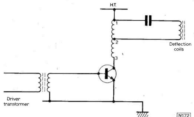
Fig. 2: The basic line output transformer circuit.
