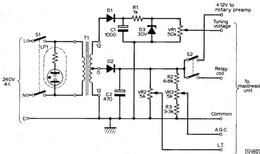
Fig. 3: Circuit diagram of the Power and Control Unit.
