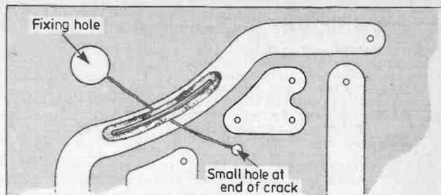
Fig. 4: Board cracks often radiate from a fixing hole and break nearby tracks. Repair with a wire bridge and drill a small hole at the end of the crack to prevent it spreading.
