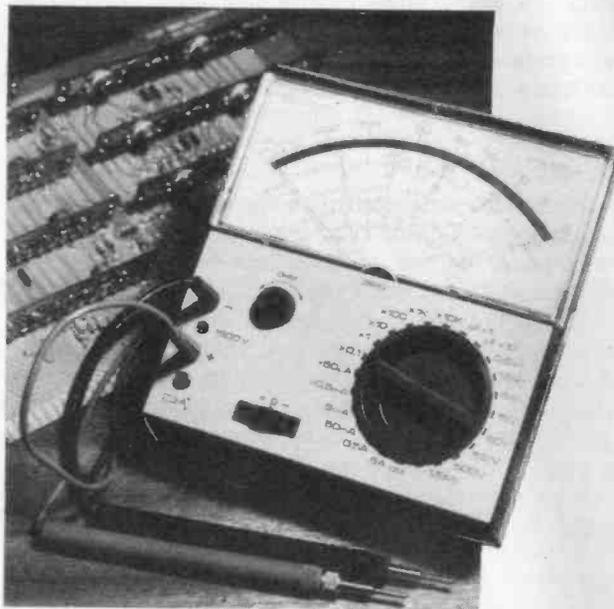
Six decade resistance ranges are provided with mid scale readings of  $5\Omega$  to  $500\text{k}\Omega$ . The range of measurements is from  $0.05\Omega$  to  $50\text{M}\Omega$ . It is unusual to find the two low resistance ranges on an instrument of this type but they are very useful when making up low value resistors from resistance wire (e.g. Power amplifier emitter resistors), or for measuring the resistance of connecting leads.
