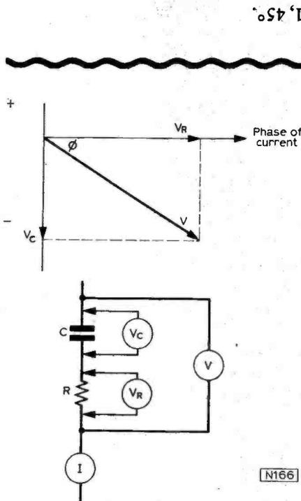
Fig. 16: Relative phase of current and voltages in a CR circuit.
