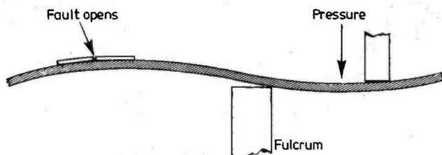
Fig. 2: Pressure on one part of a board may affect a fault in another part due to rocking action over a support which acts as a fulcrum.
