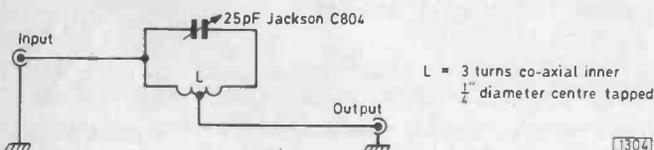
Fig. 1: Band III notch filter being used by Hugh Cocks.
