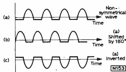
Fig. 3: For a wave which is not symmetrical, 180° phase shift is NOT the same as inversion.
