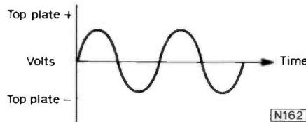
Fig. 12: An alternating voltage applied to a capacitor produces an alternating charge between the plates.
