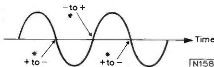
Fig. 8: The current changes most rapidly when it is reversing its direction.
