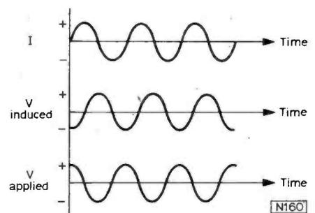
Fig. 10: Relative phase of the current, induced voltage and applied voltage in an inductor.
