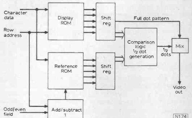
Fig. 38: A basic circuit for character rounding.
