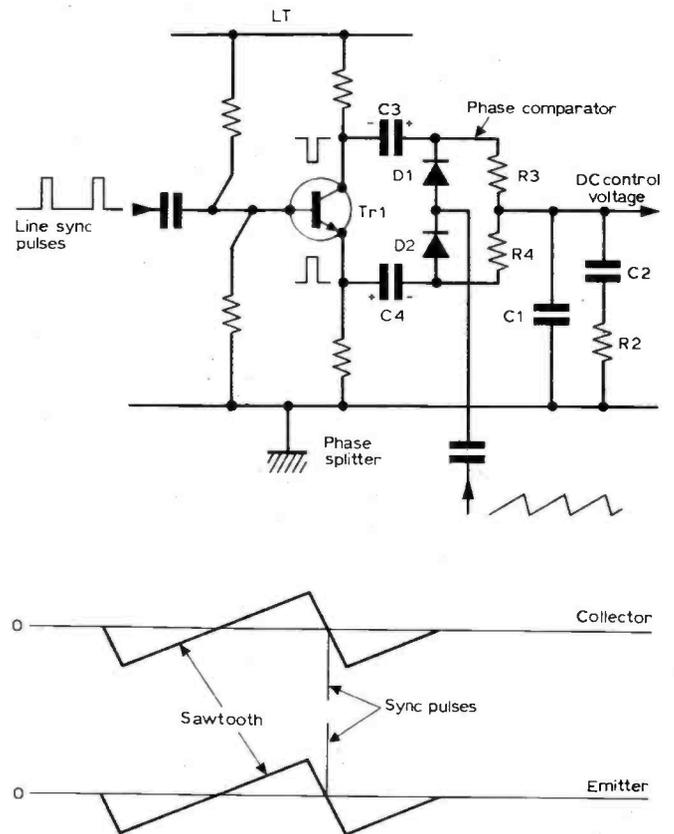
Fig. 5: A simple flywheel phase comparator circuit with pulse timings at the transistor collector and emitter.
