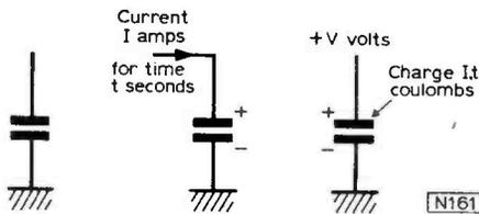
Fig. 11: The energy of the electric charge is stored as an ELECTRIC FIELD between the capacitor plates, just as a magnet stores energy in a magnetic field.
