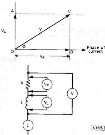
Fig. 15: Relative phase of current and voltages across the various parts of a circuit containing resistance and inductance.
