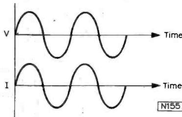
Fig. 5: Phase relationship of current and voltage in a circuit containing pure resistance only.
