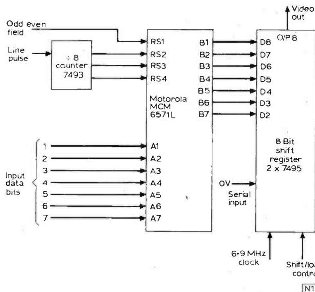
Fig. 35: A character generator using the Motorola MCM6571L.
