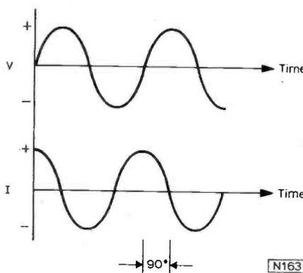
Fig. 13: The current peaks occur 90° earlier (to the left) of the voltage peaks in a capacitor.
