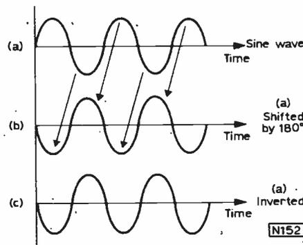
Fig. 2: Phase shifting a sinewave by 180° produces the same effect as inversion.
