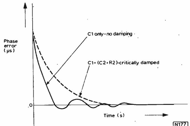
Fig. 7: Effect of the anti-hunt network. The settling time can vary from 20 lines to 20 seconds according to circuit design, and shows up when changing channels.
