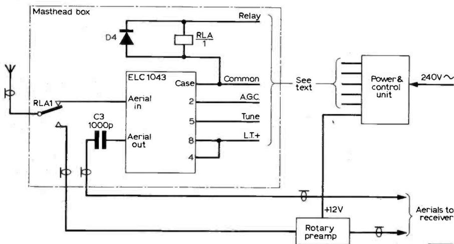
Fig. 4: Internal wiring of the masthead unit and general system connections.
