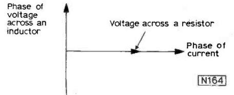
Fig. 14: In a PHASOR diagram we use angle to represent phase and length to represent magnitude of the voltage or current.
