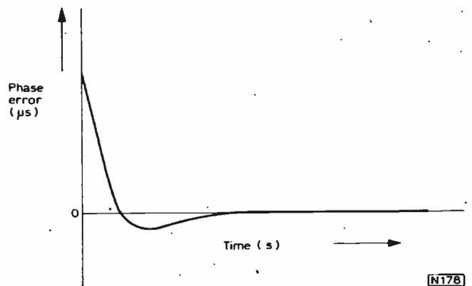
Fig. 8: For VTR operation, the shorter filter time-constant reduces settling time to about 5 lines in a well-designed circuit.
