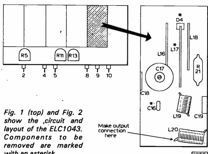
Fig. 1 (top) and Fig. 2 show the circuit and layout of the ELC1043. Components to be removed are marked with an asterisk.
