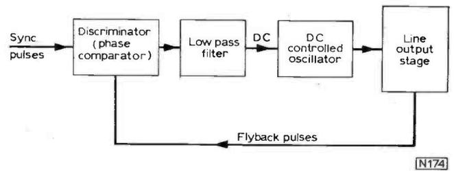
Fig. 4: A flywheel phase-locked loop.
