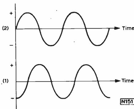
Fig. 1: Two loops rotating 90° apart will produce two sinewaves separated by ¼ cycle, a phase shift of 90°.
