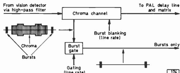
Fig. 1: Block diagram showing the burst gating action.
