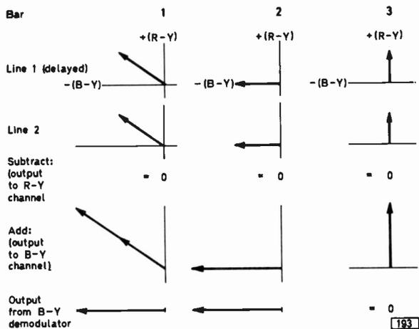
Fig. 9: When decoded an NTSC signal produces no R-Y output, only B-Y. Bar four has luminance only.
