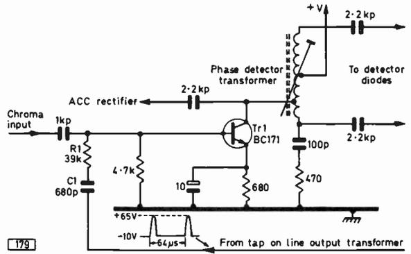
Fig. 6: The burst gate/amplifier used in the ITT-KB CVC5 single-standard colour chassis. This is gated by flyback pulses from the line output stage. The collector circuit is rather unusual in comprising a series tuned circuit, the coil driving the discriminator diodes in the normal manner.
