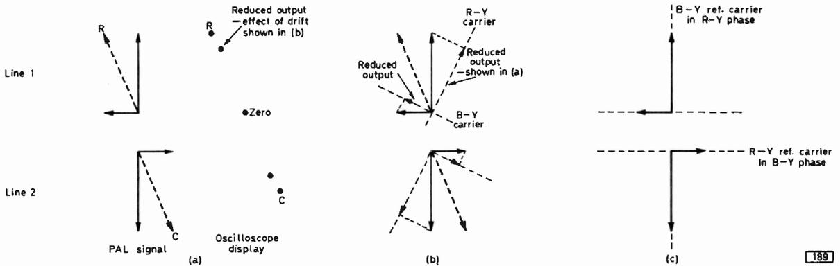
Fig. 5: The dotted lines shown in Fig. 4 (a) are produced as the reference oscillator drifts through one complete cycle. (a) Oscillator reference carriers in correct phase. (b) Both carriers here have drifted away from their correct phases, giving reduced output. (c) When both reference carriers have drifted 90° out of phase there is zero output from both demodulators: the spot is then at the centre of the screen.
