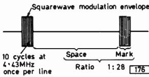
Fig. 3 (left): As the bursts occur once each line (during the back porch period) they can be considered as a 4.43MHz sinewave 100% modulated by a squarewave at line frequency.
