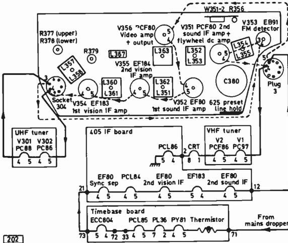
Fig. 7: Layout of the 625 convertor i.f. strip, with the complete heater chain after conversion (arrows point towards chassis).
