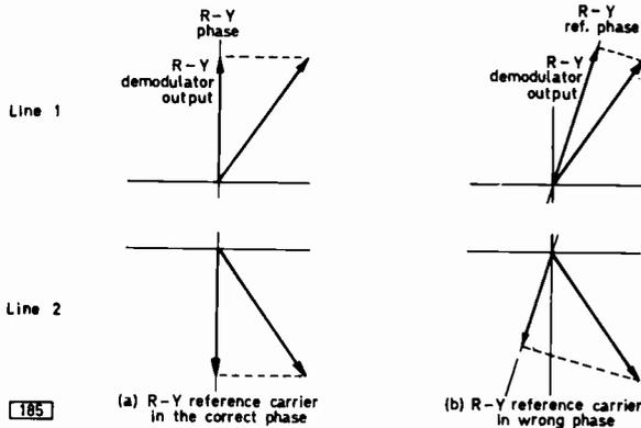
Fig. 1: With Simple PAL decoding a demodulator phase error causes different outputs on alternate lines and hence blinds on the display.
