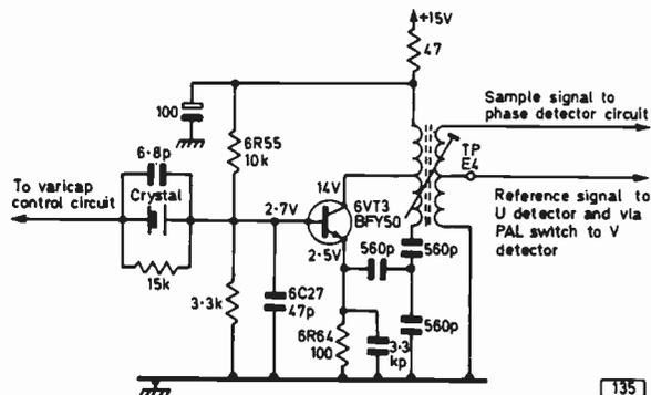
Fig. 1: The decoder reference oscillator circuit used in the Bush-Murphy dual-standard chassis.
