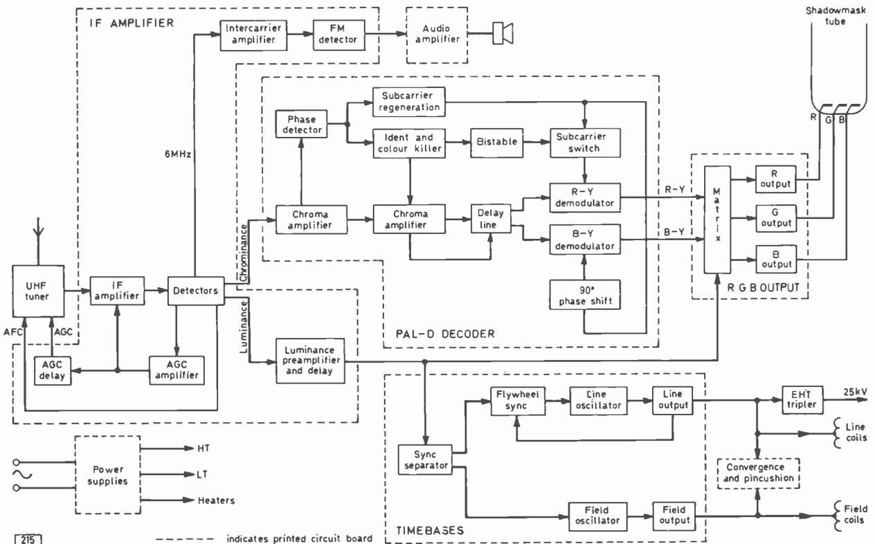
Fig. 1: Basic block diagram of the colour receiver project. Most of the components are mounted on the seven printed circuit boards indicated above. A conventional, push-button or varactor (varicap) tuner unit may be used but the latter type, which is now readily available, is recommended.
