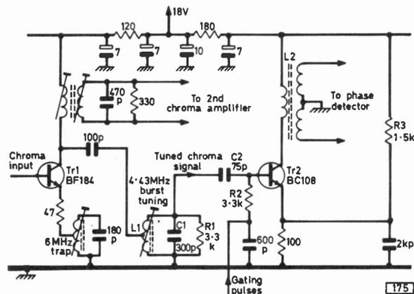
Fig. 2: Representative circuit (Decca dual-standard): Tr2 is the burst gate/amplifier which drives the phase detector transformer L2. It is fed with chroma signal from the chroma amplifier Tr1 via the tuned circuit L1, C1 and is gated on during the bursts by pulses fed via R2 from the pulse generator stage shown in Fig. 5.
