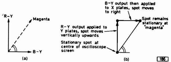
Fig. 2: (a) The R-Y and B-Y components of a magenta hue. (b) If the R-Y component is fed to the Y plates and the B-Y component to the X plates of an oscilloscope with its internal timebase stopped, the display shown here will be obtained.
