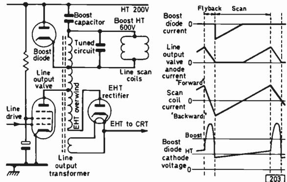
Fig. 8: Basic elements of the line output stage, with the associated waveforms.
