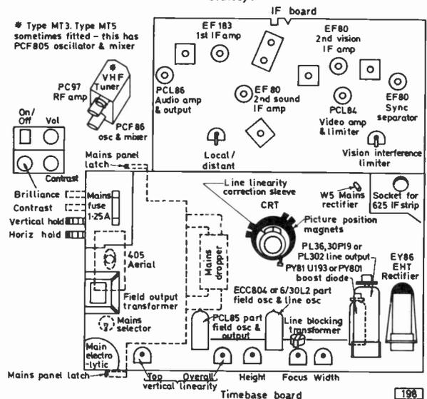
Fig. 2: Layout of the convertible Thorn 850 chassis. The heater circuit is similar to the 800. On some sets the controls, mains dropper and fuse are repositioned.
