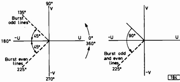
Fig. 11 (left): How the transmitted bursts swing  $\pm 45^\circ$  with respect to the  $-U$  axis on alternate lines.
