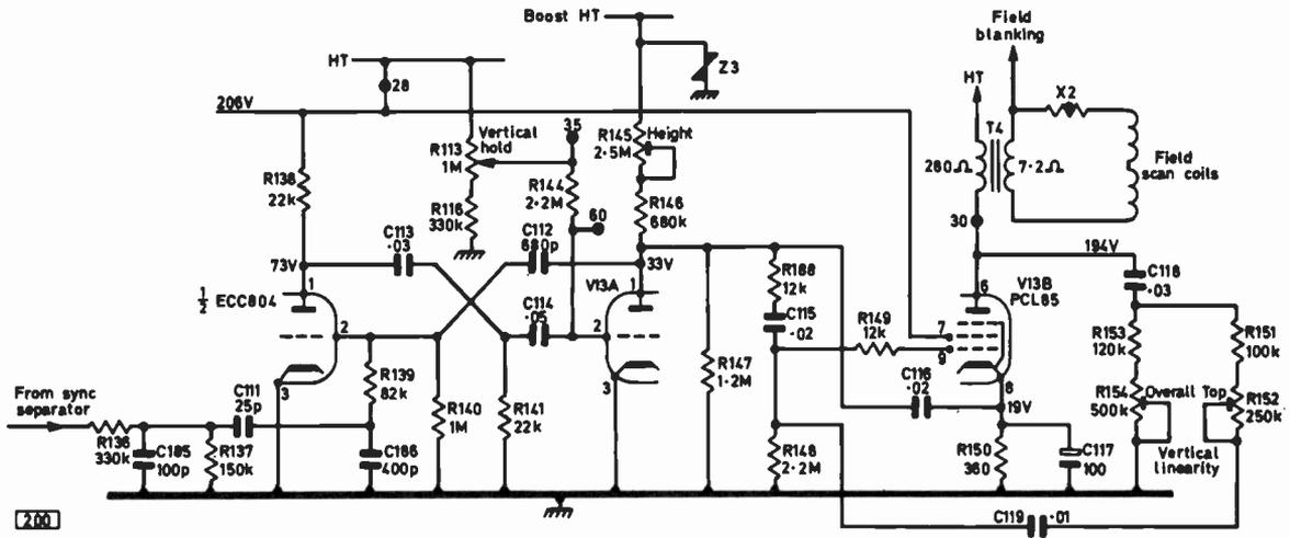
Fig. 4: The field timebase circuit. This is as used in the 850 dual-standard chassis but the earlier 800s and 850s are very similar. Early 800s had v.d.r.s (voltage dependent resistors) in series with R147 (on this circuit) and across T4 (field output transformer) primary winding.
