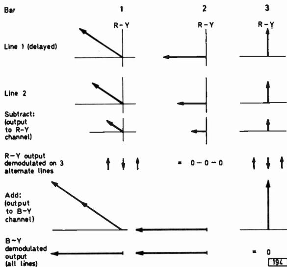
Fig. 10: Decoding the NTSC signal (with switched burst) when the direct and delayed path signals are unequal. Note the alternating outputs in bars one and three, causing blinds on the display.
