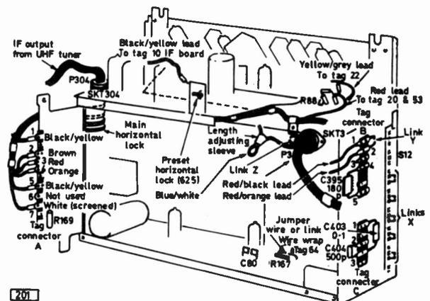
Fig. 5: Connection details for the 625 converter i.f. strip.
