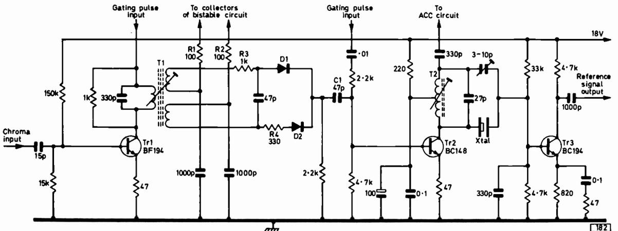
Fig. 9: The burst channel, with passive subcarrier regenerator, used in the RBM single-standard chassis.
