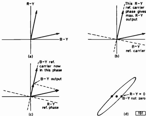
Fig. 7: Crosstalk between the R-Y and B-Y channels causes an ellipse on the X-Y display. (a) These signal components are the result of incorrect delay line amplitude adjustment. (b) This phasing corresponds to a point almost at the tip of the ellipse. (c) No R-Y output, but there is still some B-Y output so the result is an ellipse. (d) An ellipse is formed if the R-Y and B-Y outputs are not zero simultaneously.
