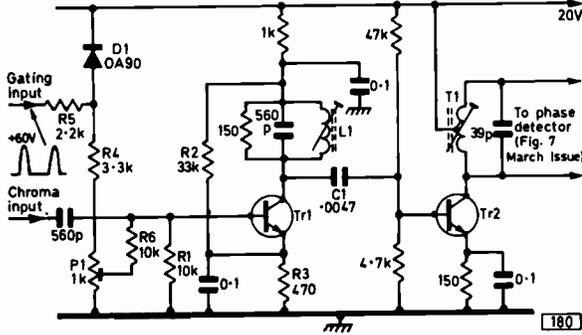
Fig. 7: Two-stage burst channel used in dual-standard Baird colour sets. Line flyback pulses clamped to the 20V l.t. rail by D1 gate the base of Tr1.
