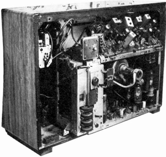
A Thorn 800 chassis: hinges at the right enable the chassis to be swung out almost 90° after removing two screws at the left, giving access to both sides.
