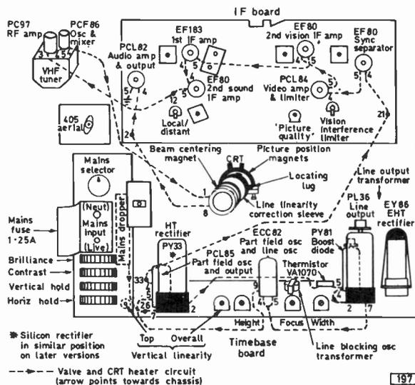
Fig. 1: Layout of the Thorn 800 chassis. The i.f. board has been tilted up and the line output stage shield removed for clarity.
