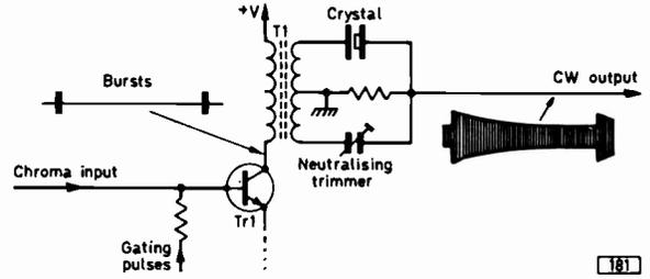
Fig. 8: The basic passive subcarrier regenerator circuit. The crystal acts as a high Q filter which removes the sidebands from the burst subcarrier to provide a 4.43MHz c.w. output.
