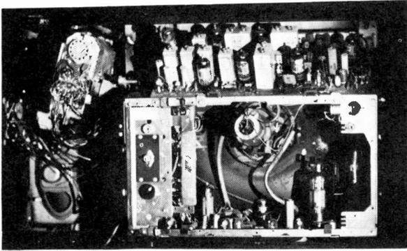
A dual-standard Thorn 850 chassis, fitted in the wide cabinet of an Ultra Bermuda model.
