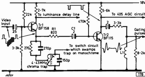
Fig. 5: The pulse generator used in Decca dual-standard models to produce the pulse to switch on the burst gate. An output with positive-going sync pulses is taken from the luminance preamplifier Tr1 and fed to the base of Tr2. As a result Tr2 produces negative-going pulses which are fed to L1. This coil rings, producing a positive-going overshoot which is coincident in time with the bursts and is used as the burst gating pulse (fed to Tr2 in Fig. 2).
