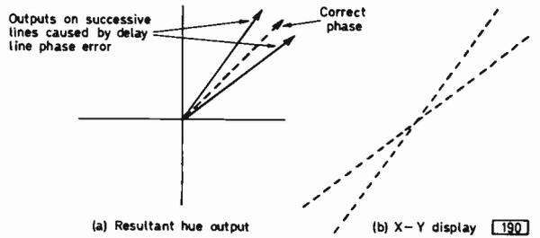
Fig. 6: A delay line phase (time) error produces different hues on successive lines and this is shown clearly on the X-Y display (b).
