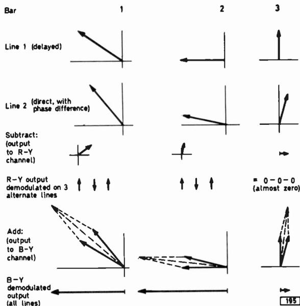
Fig. 11: The same decoding process as in Fig. 10 but this time with a phase difference between the direct and delayed path signals. Switched R-Y outputs are present on bars one and two, causing blinds.
