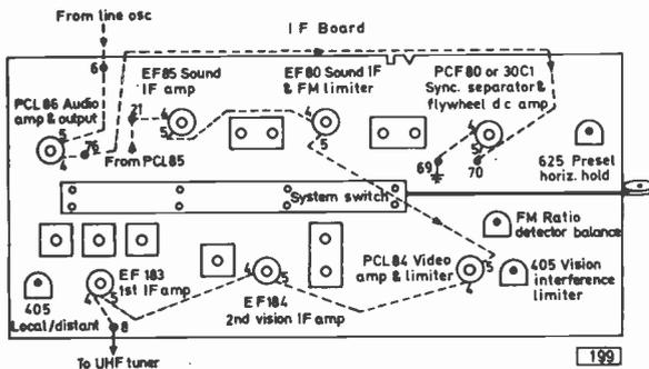
Fig. 3: Layout of the i.f. board used in the dual-standard 850 chassis. This chassis is otherwise similar to Fig. 2 except that the 625 i.f. strip socket is not required.
