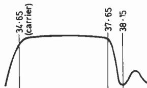
Fig. 1 (left): Typical 405-line vision i.f. response curve.
