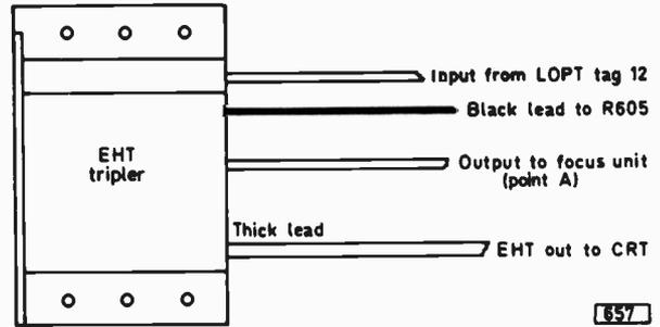
Fig. 3: Connections to the e.h.t. tripler.
