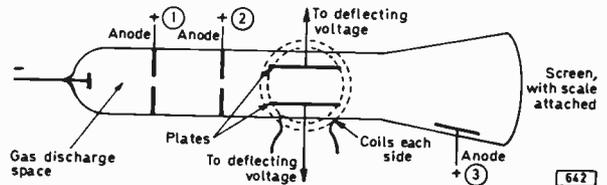
Fig. 5: Thomson's apparatus. The voltages on all anodes are equal. Electric field as before (Fig. 3). Magnetic field added so that beam is deflected back:  $Bqv = q(V/d)$ . Thus  $v = (V/dB)$ . Combining,  $q/m = (V^2/d^2B^2) \times (d/V) \times (y/lb) = Vy/dB^2lb$ .
