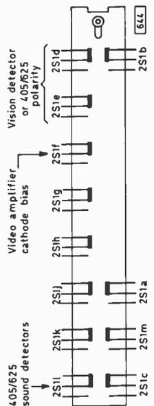
Fig. 3: I.f. panel system switch, shown in 405-line position.
