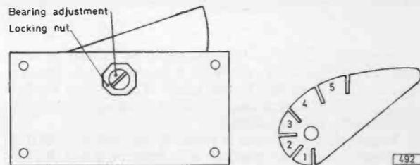
Fig. 1 (left): Gang capacitor rear view, showing the bearing adjustment screw and locking nut.
