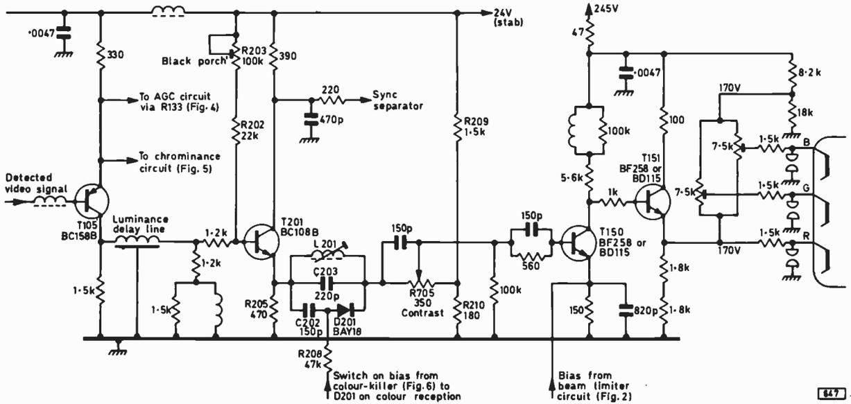
Fig. 1: Complete luminance channel circuit, which is d.c. coupled throughout.
