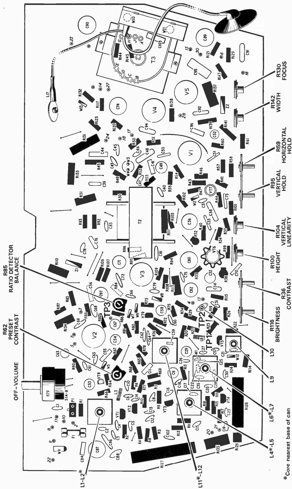
Fig. 2: Component layout on the main chassis assembly.
