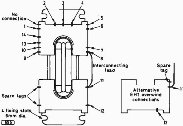
Fig. 1: Line output transformer tag identification.
