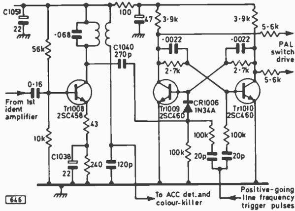
Fig. 2: Second ident stage and bistable circuit used in the decoder section of Hitachi colour sets. Poor bistable synchronisation was due to C1040 being faulty.
