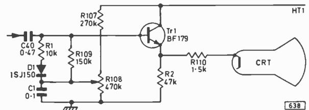
Fig. 3: Circuit finally adopted, with buffer stage Tr1. The diode (D1) is a Radiospares type 1S150: a near equivalent is the OA202.
