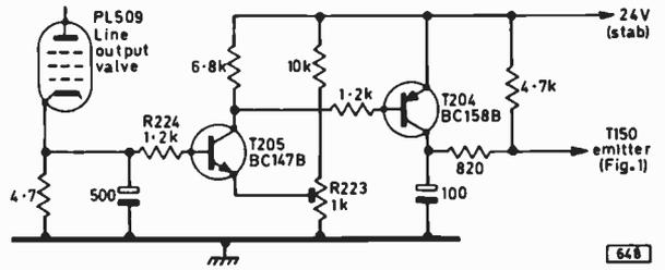
Fig. 2: The beam limiter circuit.
