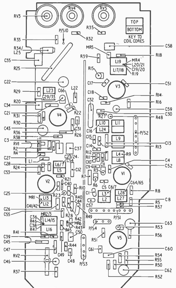
Fig. 1: Layout of the i.f. unit.
