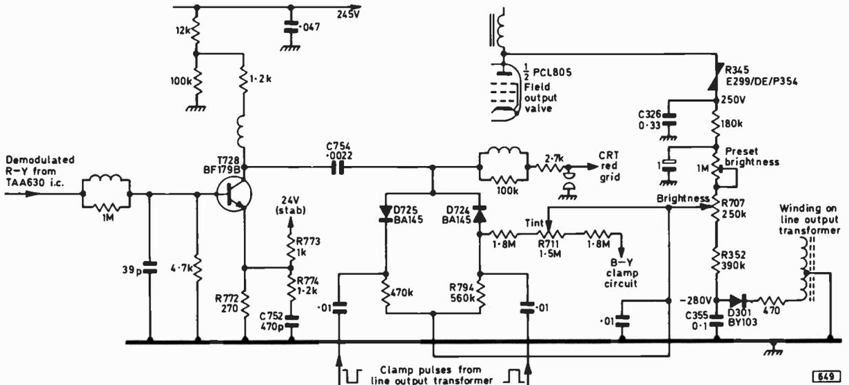
Fig. 3: Circuit of the R-Y colour-difference output stage together with the brightness and tint control arrangements. Tube protection is afforded by deriving the brightness potential from the field output valve.
