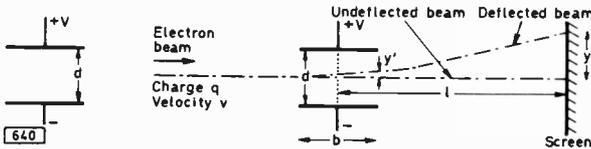
Fig. 2 (left): If  $V$  is the voltage between the plates and  $d$  the spacing between them, the electric field =  $V/d$  volts per meter, e.g. with 300V between plates 1cm (0.01m) apart, field =  $300/0.01 = 30,000V/m$ .
