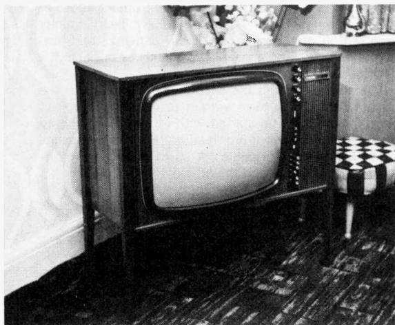
*The Philips Model G25K500, a 25in. receiver fitted with the G6 dual-standard colour chassis.*
