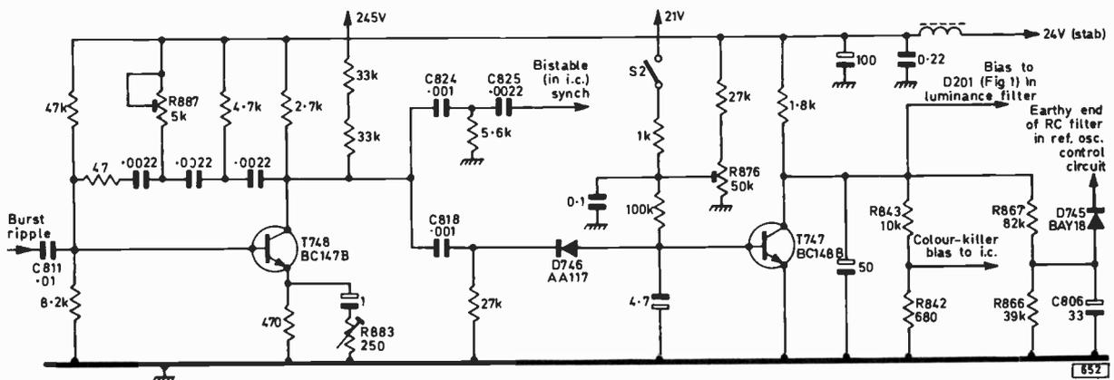
Fig. 6: The RC oscillator ident stage and colour-killer circuitry.
