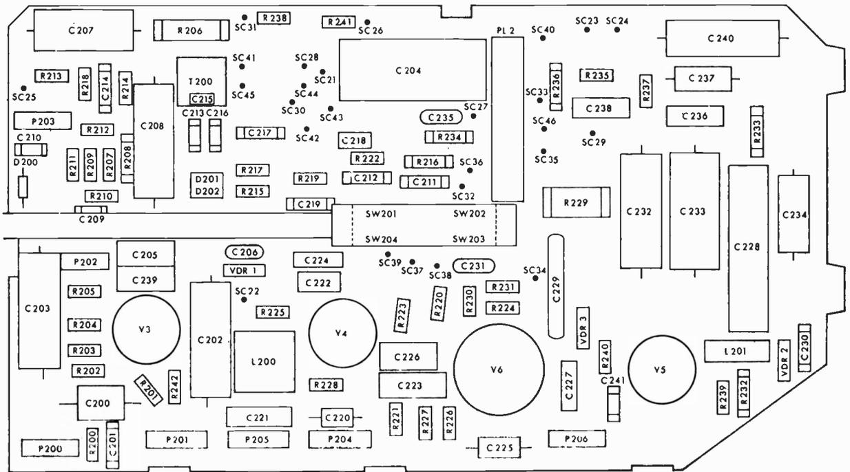
Fig. 3: Layout of the timebase printed panel, viewed from the component side.
