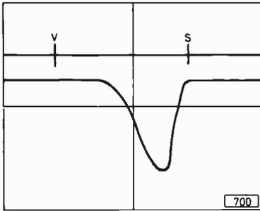
Fig. 3: Correct waveform at Tr101 base. S is the sound marker and V the vision marker. A.G.C. delay control set midway. Y amplitude 20mV/cm., X timebase speed 1msec/cm.
