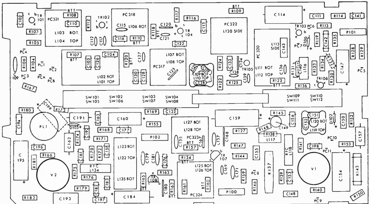
Fig. 4: Layout of the i.f. printed panel, viewed from the component side.
