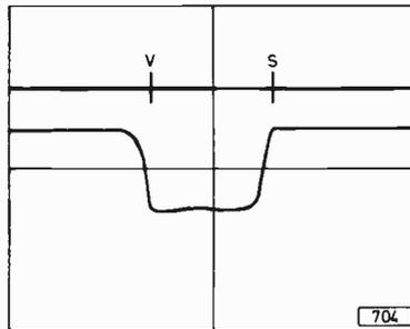
Fig. 7: Correct waveform at Tr104 collector, taken with probe placed on the body of R115 and R133 set midway. Y amplitude 200mV/cm., X timebase speed 1msec/cm.
