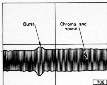
Fig. 9: Signal at Tr110 base. Y amplitude 50mV/cm., X timebase speed 10μsec/cm.
