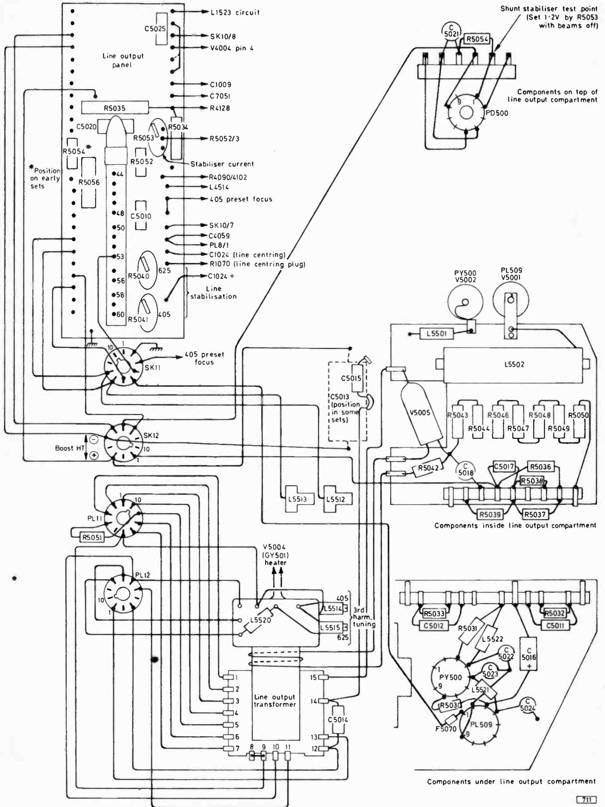
Fig. 8: Line output compartment component layout.
