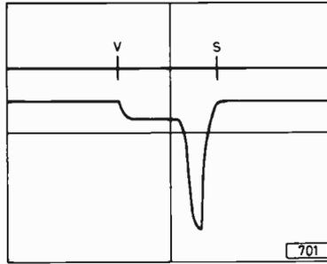
Fig. 4: Correct waveform at Tr101 collector with a.g.c. delay control set midway. Y amplitude 20mV/cm., X timebase speed 1msec/cm.
