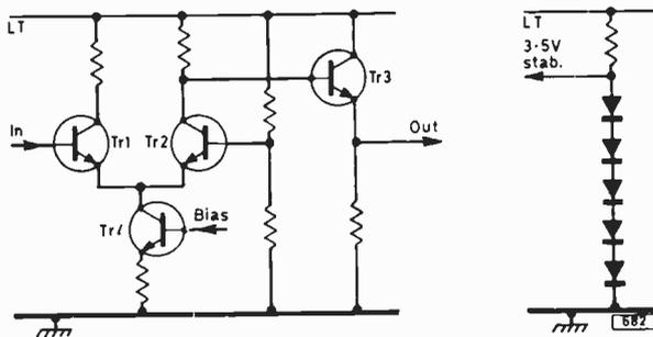
Fig. 4 (left): Typical i.c. amplifier stage: Tr1/2 form an emitter-coupled differential amplifier with the bias applied to the base of the emitter transistor Tr4 controlling the stage gain; the emitter-follower Tr3 provides matching to the following stage.
