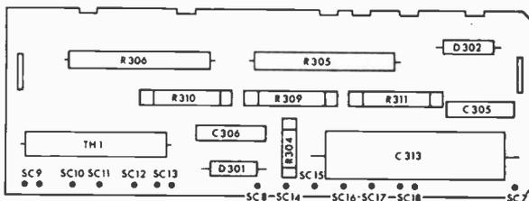
Fig. 2: Layout of the power supply panel. TH1 = TH300.
