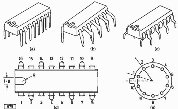
Fig. 1: I.C. encapsulations in common use. (a) DIL (dual-in-line) 16-pin package suitable for i.c. holders; (b) early QUIL (quad-in-line) configuration—pins 1 and 16 close, 2 and 15 spaced out etc.; (c) current zig-zag QUIL with pins 1 and 16 "upwards", 2 and 15 "downwards", etc.—this type can be fitted the wrong way round if the keyway position is not checked; (d) QUIL pin numbers looking down from the top; (e) 10-pin round base viewed from beneath.
