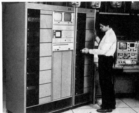
*The IVC BCR100 broadcast cassette VTR makes use of a bank of VCR100 recorders.*
