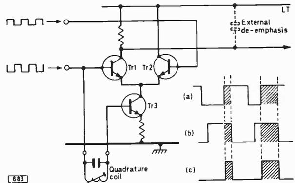
Fig. 6: Typical coincidence detector (alias synchronous demodulator) circuit. The f.m. input (a) is applied in anti-phase to the bases of Tr1 and Tr2. The input is also smoothed by the external quadrature coil to give regular phase-shifted pulses (b) which are fed to Tr3 base. Conduction occurs only when (a) and (b) overlap, producing pulses of varying width (c) at Tr1 collector. The external de-emphasis capacitor smooths these to produce the audio signal.
