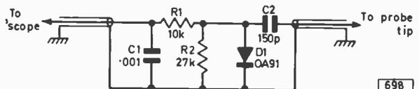
Fig. 1: Suitable demodulator probe circuit.
