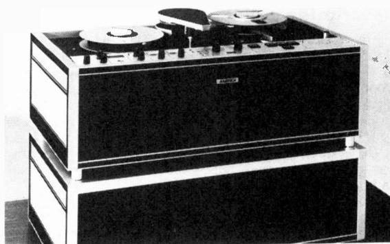
*Ampex VPR7903 1in. helical-scan VTR.*
