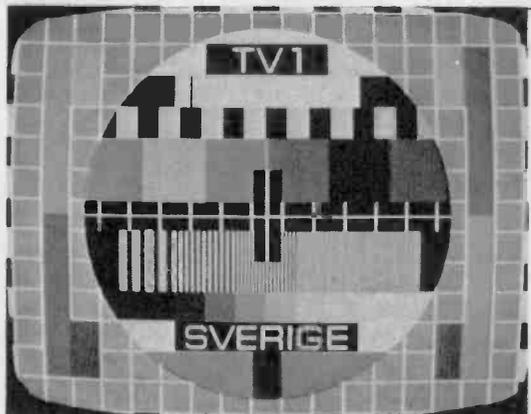
*The PM554 colour test card as used by Sweden—
