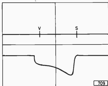
Fig. 12: Correct waveform at Tr111 collector with R133 set midway. Y amplitude 0.1V/cm., X timebase speed 1msec/cm.
