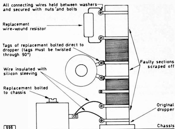
Fig. 2: Fitting replacement sections.
