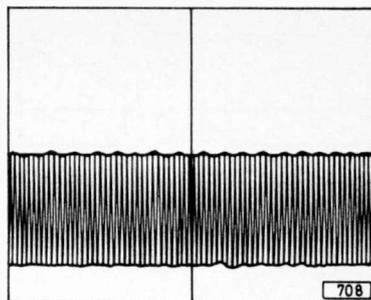
Fig. 11: Signal at pin 6 of the TAA350 intercarrier sound i.c. Y amplitude 200mV/cm., X timebase speed 20μsec/cm.
