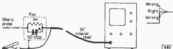
Fig. 2: This  $\times 2$  probe reduces the loading of the probe on the circuit without losing too much sensitivity. Adjust the capacitor on a squarewave for square shoulders on the 'scope screen.
