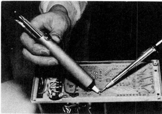
The type of desoldering gun shown here is strongly recommended for use when removing i.c.s.
