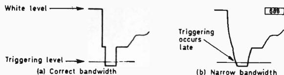
Fig. 2: Narrow bandwidth at the sync separator results in the line sync pulse being delayed when the video signal is at white level at the end of the line scan.
