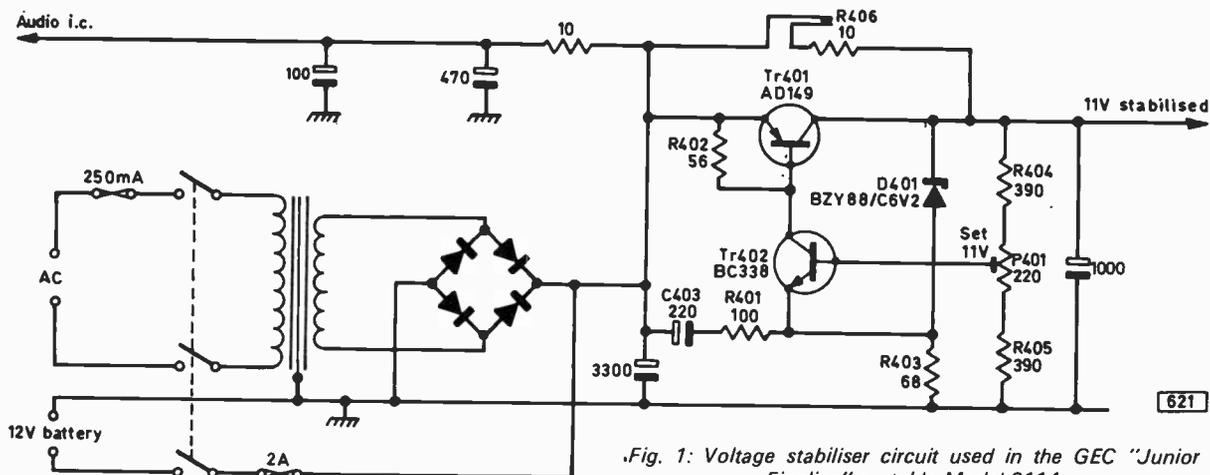
Fig. 1: Voltage stabiliser circuit used in the GEC "Junior Fineline" portable Model 2114.
