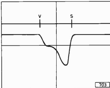
Fig. 6: Correct waveform at Tr102 collector—a.g.c. delay control set midway. Y amplitude 10mV/cm., X timebase speed 1msec/cm.
