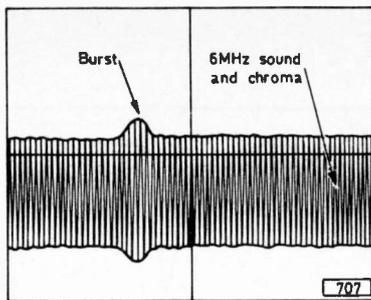
Fig. 10: Signal at pin 2 of the TAA350 intercarrier sound i.c. Y amplitude 50mV/cm., X timebase speed 10μsec/cm.
