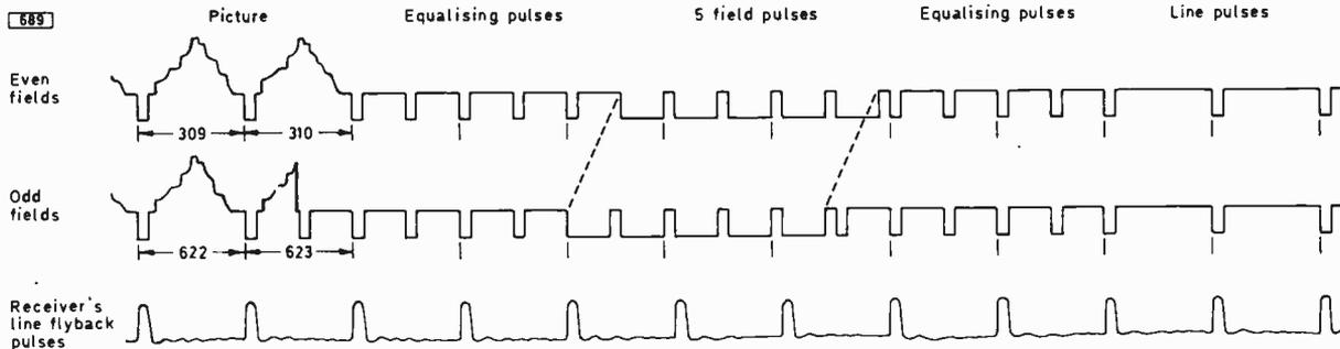
Fig. 3: The transmitted sync pulse train—625-line system. Note the half-line stagger of the field sync pulses on alternate (odd and even) fields.
