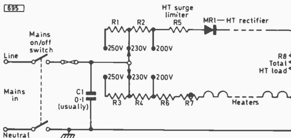
Fig. 1: Typical mains dropper circuit.
