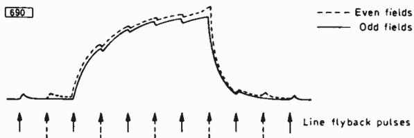
Fig. 4: Line flyback pulses picked up in the sync circuits will contribute to the composite field sync pulse. The contribution will be different on alternate fields.
