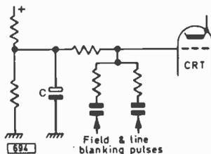
Fig. 8: A switch-off spot will be prevented by the charge retained on capacitor C after the h.t. collapses.
