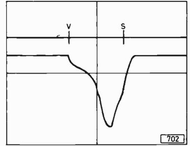
Fig. 5: Correct waveform at Tr103 collector—a.g.c. delay control set midway. Y amplitude 500mV/cm., X timebase speed 1msec/cm.
