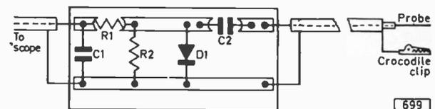
Fig. 2: Probe layout. For simplest probe tip peel back the output coaxial cable for 2in., form the chassis connection from the braiding and tin the inner conductor to make it stiff.
