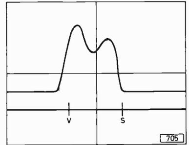
Fig. 8: Correct waveform at D101 cathode—a.g.c. delay control set midway. Y amplitude 2V/cm., X timebase speed 1msec/cm.
