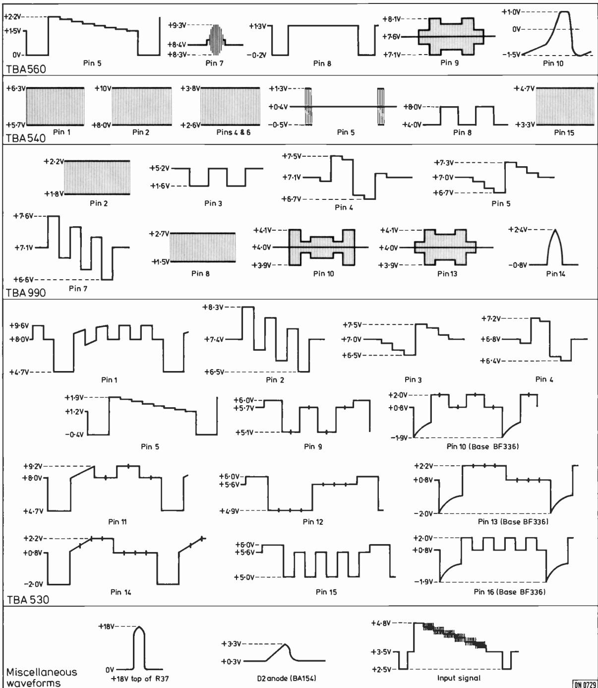
Fig. 2: Four i.c. decoder waveforms.
