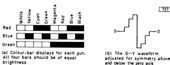
*Fig. 2: Adjusting the colour-difference drives.*
