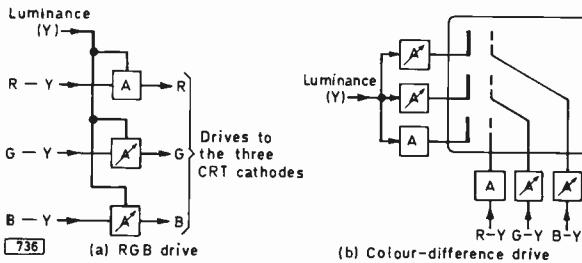
*Fig. 1: RGB (a) and colour-difference (b) c.r.t. drive techniques.*
