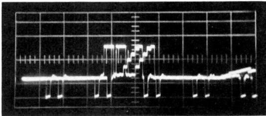
Fig. 3: The overlapping display obtained when two scans per picture are made from the delay timebase.
