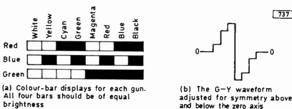
Fig. 2: Adjusting the colour-difference drives.
