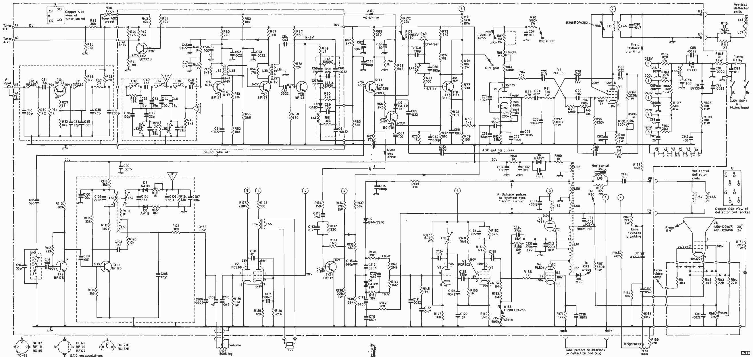
Fig. 3: Circuit of the ITT VC200 chassis. Voltages measured with a 20k $\Omega$ /V meter: (Avo Model 8). TX6, TX7 and TX8 voltages with the contrast control set midway.
