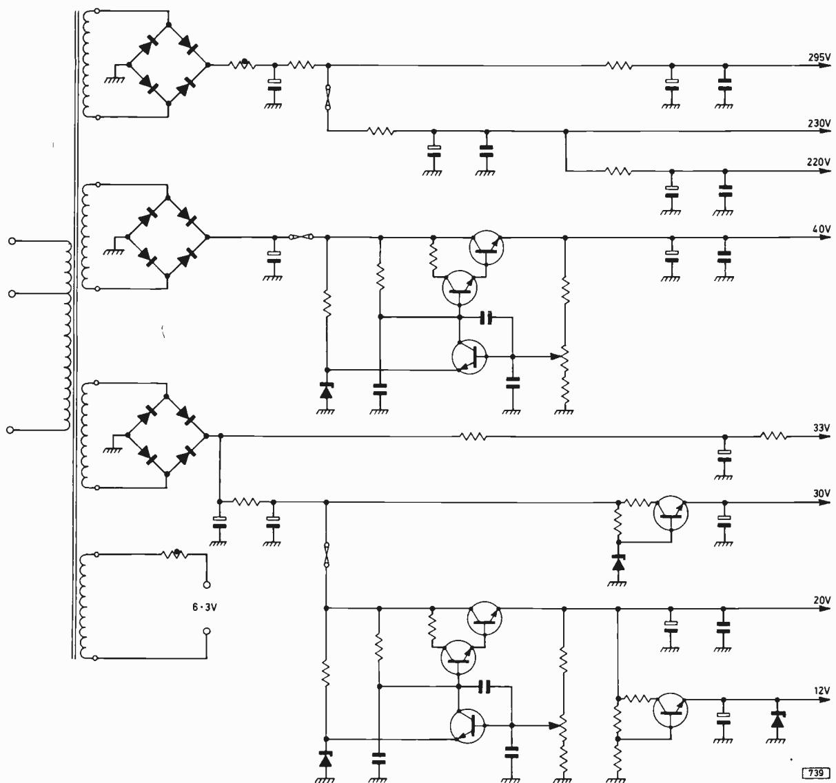
Fig. 6: Full details of this very stable power supply circuit which a reader has devised for use with the colour receiver will appear shortly.
