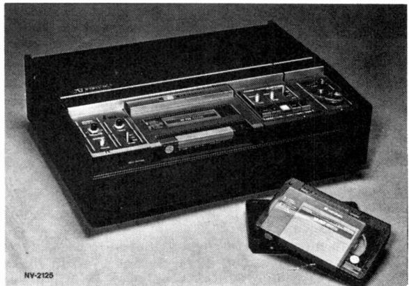
National videocassette recorder/players. Above, the NV5125 1/2 in. model; below, the NV2125 3/4 in. model. There are PAL and NTSC versions. Tuners and an r.f. unit are incorporated as standard. The video modulation system is double-sideband f.m.
