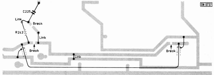
Fig. 3 (above right): This modification to the RGB board removes a bright line down the left of the screen.
