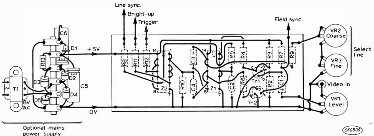
Fig. 10: Layout for the circuit shown in Fig. 9, viewed from the conductor side.
