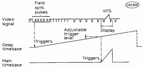
Fig. 2: Principle of using a delay-timebase oscilloscope to display single lines. This method has the disadvantages described in the text.
