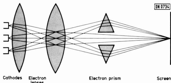
Fig. 5: Optical analogy of the Trinitron tube's electron focusing/convergence system.
