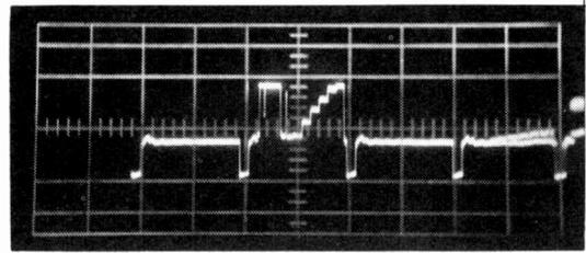
Fig. 13: The clean display obtained by use of the video test signal extractor unit.
