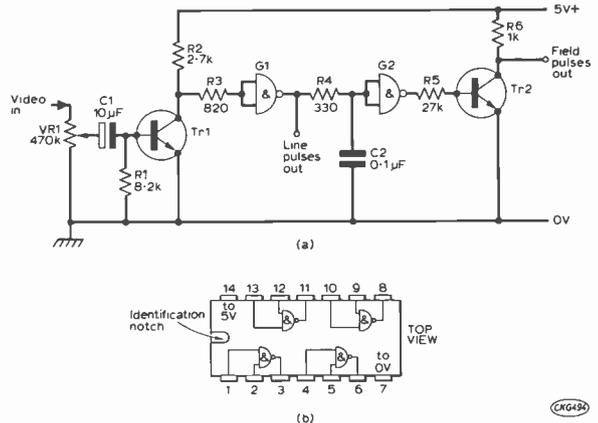
Fig. 4(a): Sync separator circuit using logic NAND gates. (b) Pin identification for the SN7400N quad 2-input NAND i.c.
