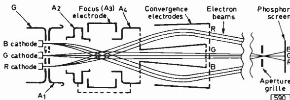
Fig. 6: More detailed depiction of the Trinitron tube's gun assembly.
