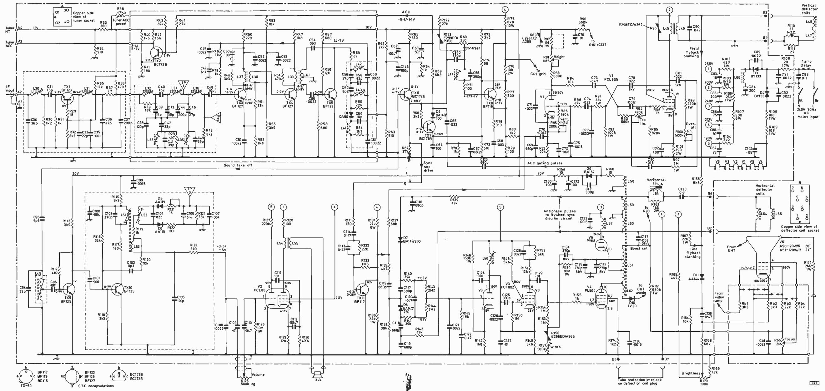
Fig. 3: Circuit of the ITT VC200 chassis. Voltages measured with a 20kΩ/V meter: (Avo Model 8), TX6, TX7 and TX8 voltages with the contrast control set midway.
