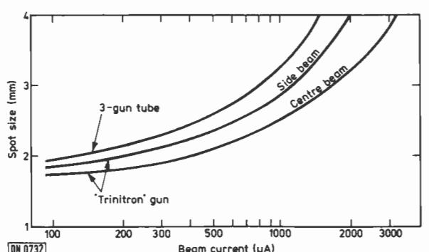
Fig. 3: Relationship between spot size and tube beam current.
