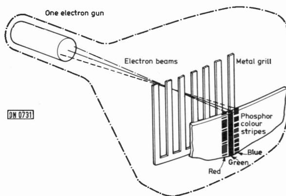
Fig. 2: Arrangement of the phosphor stripes and aperture grill of the Trinitron tube.
