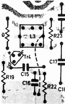
Fig. 2: (above left): Adding a link from L3 screen earth to the decoder board centre earth copper cleans up the picture.
