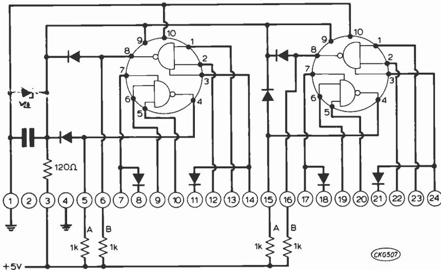
Fig. 6: Circuit of the Marconi surplus i.c. panel.
