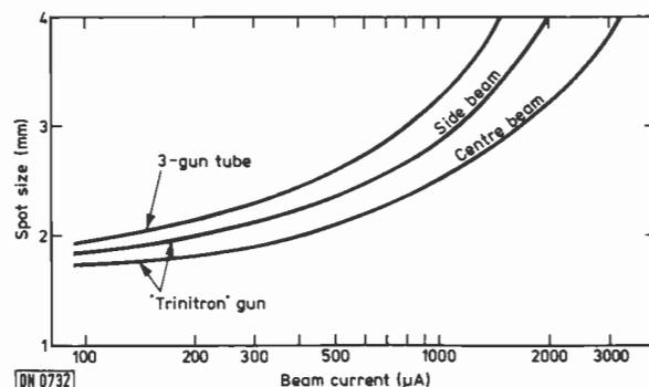
Fig. 3: Relationship between spot size and tube beam current.
