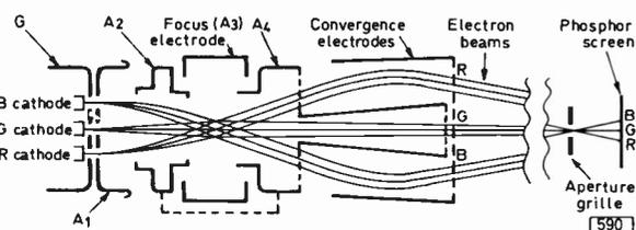
Fig. 6: More detailed depiction of the Trinitron tube's gun assembly.
