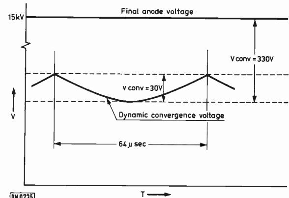
Fig. 7: The convergence potential and dynamic correction waveform applied to the deflection plates.
