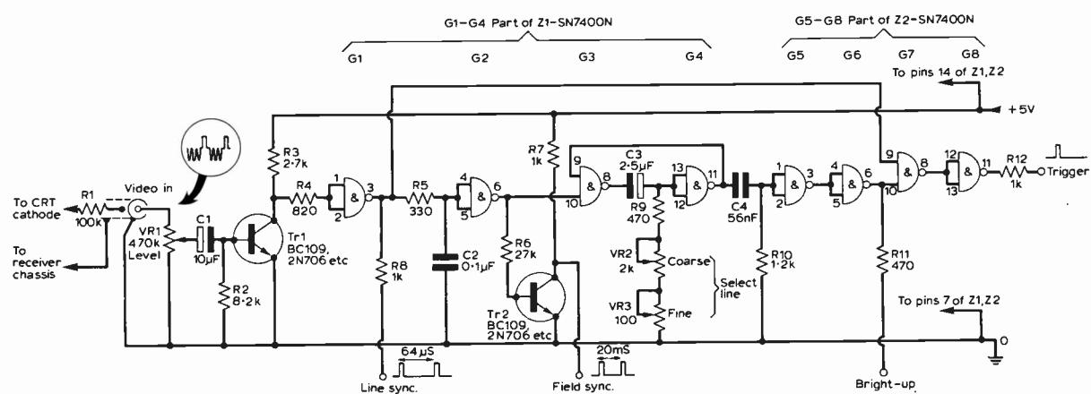
Fig. 9: Circuit of the video test signal extractor unit using two SN7400N i.c.s.
