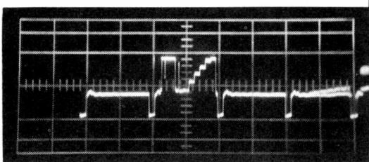
Fig. 13: The clean display obtained by use of the video test signal extractor unit.
