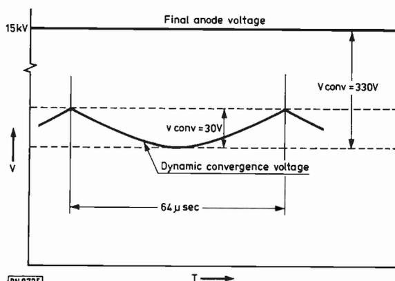
Fig. 7: The convergence potential and dynamic correction waveform applied to the deflection plates.
