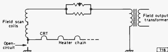
Fig. 1: Break in the lead providing a common earth for the field deflection coils and the heater chain resulted in the heater current passing through the scan coils and the secondary of the field output transformer, producing a spurious "scan".
