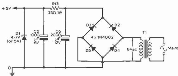
Fig. 11: 5V d.c. mains power supply suitable for the video test signal extractor unit.
