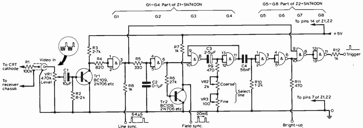
Fig. 9: Circuit of the video test signal extractor unit using two SN7400N i.c.s.
