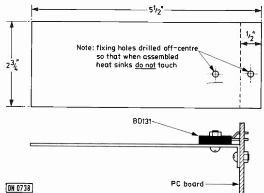
Fig. 4: Simple, effective heatsink for the BD131 field output transistors.
