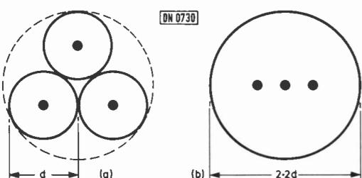
Fig. 1: Comparison between the effective electron lens diameter of the delta gun arrangement used in the shadowmask tube (a) and the single-gun system used in the Trinitron tube (b).
