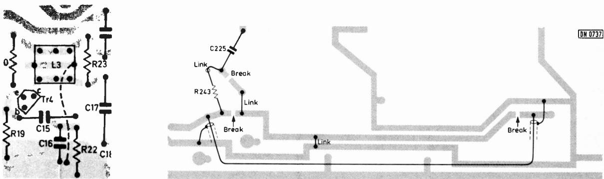
Fig. 2: (above left): Adding a link from L3 screen earth to the decoder board centre earth copper cleans up the picture.
