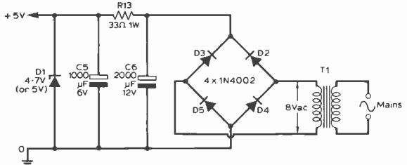
Fig. 11: 5V d.c. mains power supply suitable for the video test signal extractor unit.
