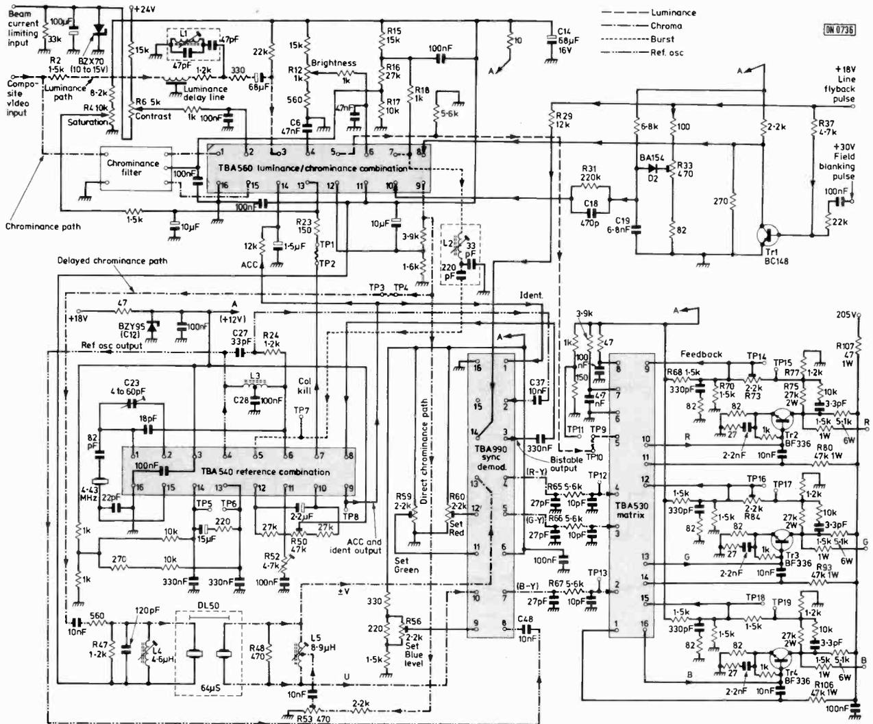
Fig. 1: Circuit of the four i.c. decoder. The gating/clamping pulses applied to pin 10 of the TBA560 are generated across C19 when the flyback pulses briefly cut off D2.
