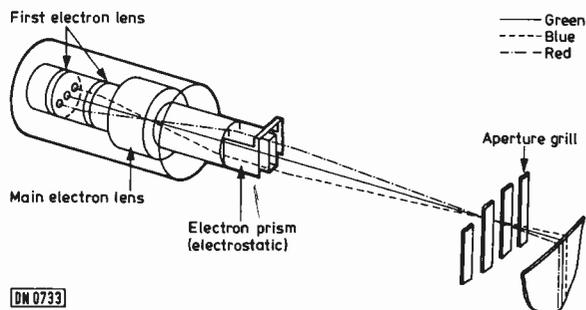
Fig. 4: The electron-optical system used in the Trinitron tube.
