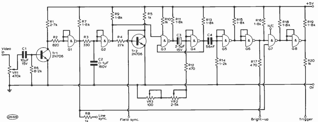
Fig. 7: Circuit of the video test signal extractor unit utilising the Marconi i.c.s. C1 should be shown as an electrolytic capacitor, polarity as in Figs. 4 and 9.
