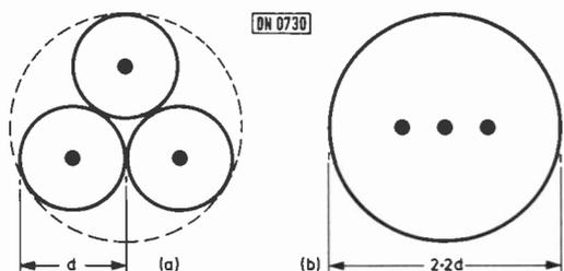
Fig. 1: Comparison between the effective electron lens diameter of the delta gun arrangement used in the shadowmask tube (a) and the single-gun system used in the Trinitron tube (b).
