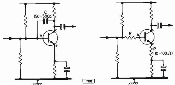
Fig. 7 (left): Placing a ceramic capacitor between the collector and base of a transistor can prevent it providing r.f. amplification.
