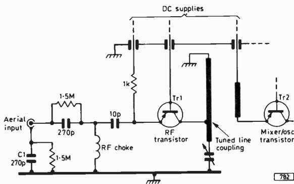
Fig. 1: Wideband RC coupled input to the tuner gives poor rejection of strong low-frequency signals picked up on both the inner conductor of the coaxial feeder and the braiding.
