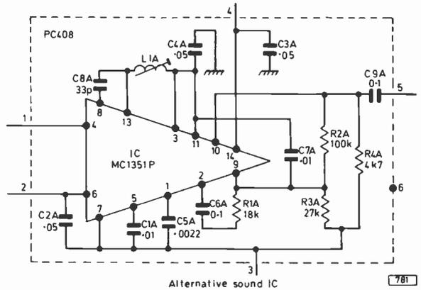
Fig. 4: Connection data and alternative intercarrier sound i.c. circuit.
