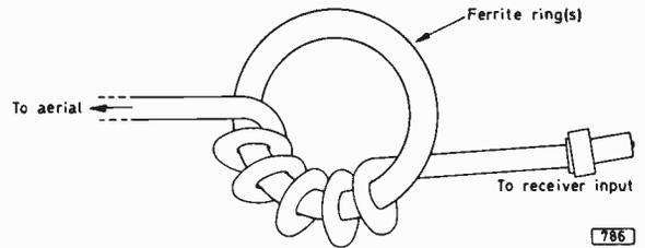
Fig. 5: Ferrite-ring filter. This introduces considerable series inductance in the coaxial feeder braiding. The number of turns required around the ferrite ring depends on the frequency of the interfering signal. Two rings placed together can further improve the efficiency, the feeder turns going around both of them.
