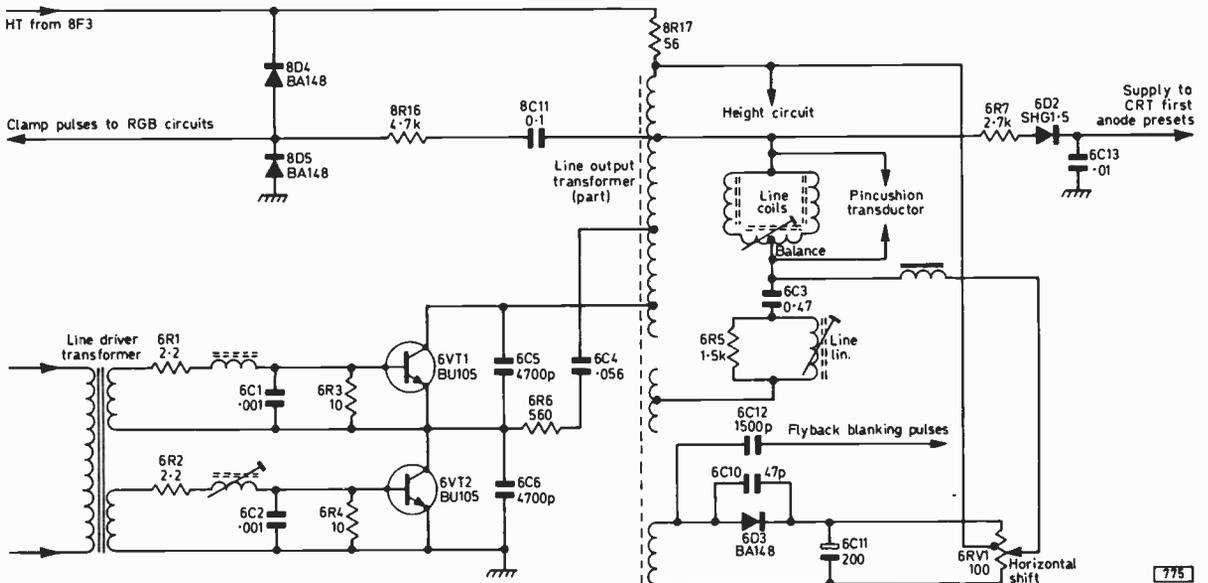
Fig. 3: Line output stage circuit (part only shown). In later production sets 6R6 and 6C4 have been deleted.
