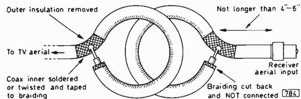
Fig. 3: The Faraday link. Tape over the joints with good (preferably plastic) insulating tape. When the optimum coupling has been found the whole link can be taped together.
