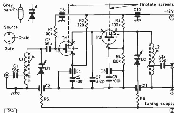
Fig. 1: Circuit of the preamplifier. Physically, C4 and C8 are at Tr1 source and Tr2 gate connection respectively—see layout. Transistor connections viewed with leads facing. The cathode end of the varicap diode is indicated by a grey band.
