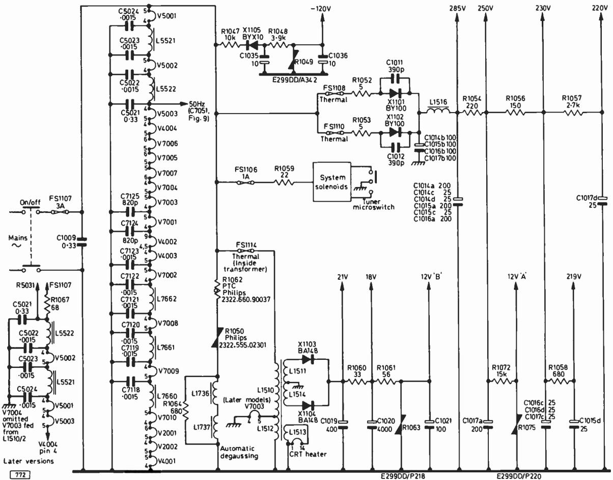
Fig. 12: The heater chain, automatic degaussing and power supply circuits, including modifications. See Fig. 13 opposite for physical layout.
