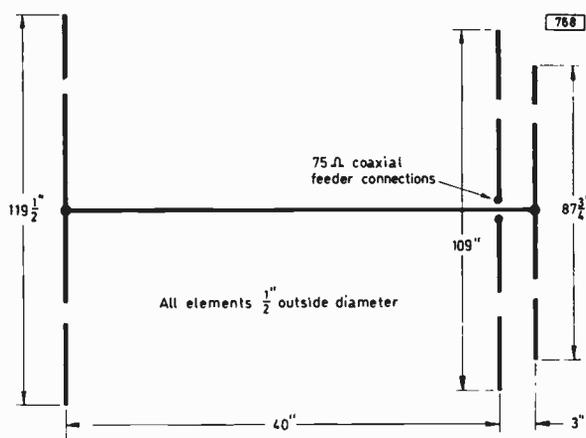
Fig. 1: A new wideband Band I array.
