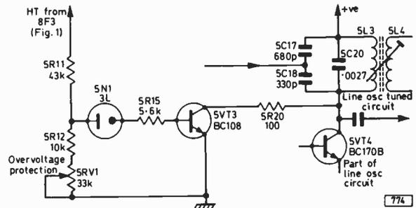
Fig. 2: The overvoltage circuit stops the line oscillator if the h.t. voltage rises excessively, resulting in no line drive and consequently no e.h.t.
