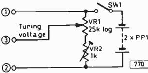
Fig. 2: Circuit of the control unit. VR1 provides channel tuning by varying the bias applied to the varicap diodes D1 and D2.
