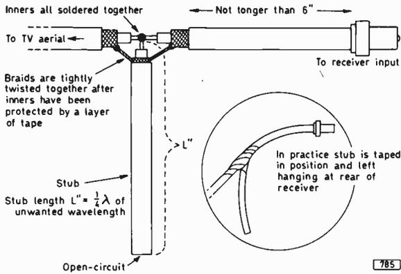
Fig. 4: Quarter-wave stub attached to the aerial input of a television set. At its resonant length the stub acts as a short-circuit across the feeder. It is critical to within  $\frac{1}{8}$  in. of the actual length cut for a particular frequency. Due allowance must be made for the velocity factor of the cable.
