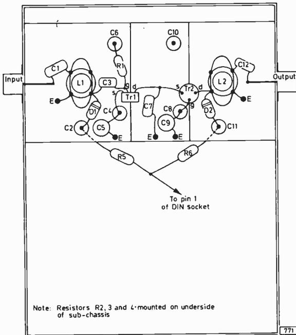
Fig. 3: Layout of the preamplifier which is housed in a diecast box.
