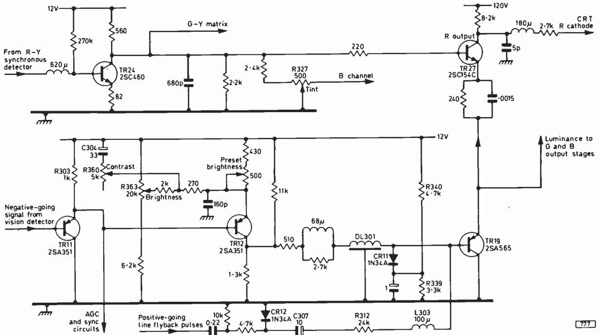
Fig. 1: Circuit of the luminance channel and one of the RGB channels in the Hitachi colour chassis. The brightness control adjusts the bias at the emitter of the second luminance transistor TR12. Since the circuit is d.c. coupled throughout this in turn varies the drive applied to the three c.r.t. cathodes.
