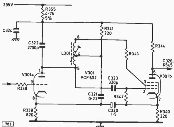
Fig. 2: Modified line oscillator circuit. L301 is the standard line oscillator coil available from Forgestone Components. Component values are shown only where they have been changed. Component ratings: R355 1W 5%; C320 40V; C321 400V; C322 5% 400V; C323 400V. Forgestone Components tell us that they can provide the components required to carry out this modification.
