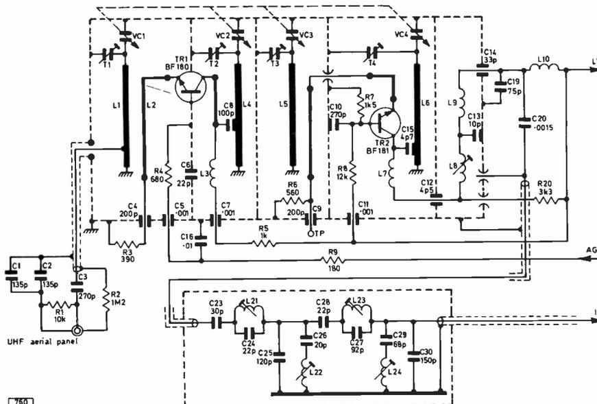
Fig. 5: Tuner and i.f. filter unit circuits.
