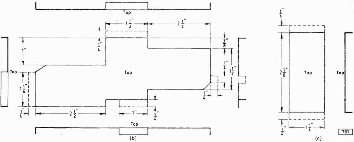
Fig. 5: (a) The performance of the i.f. strip can be improved by adding copper screening on the print side as indicated here. The soldered connections between the screens and the board must be in the positions marked above in heavy line. Transfer C116 and C117 to the print side of the board—ensure that they are mica types and mount them with the shortest possible leads. The dimensions of the two screens are shown in (b) and (c).
