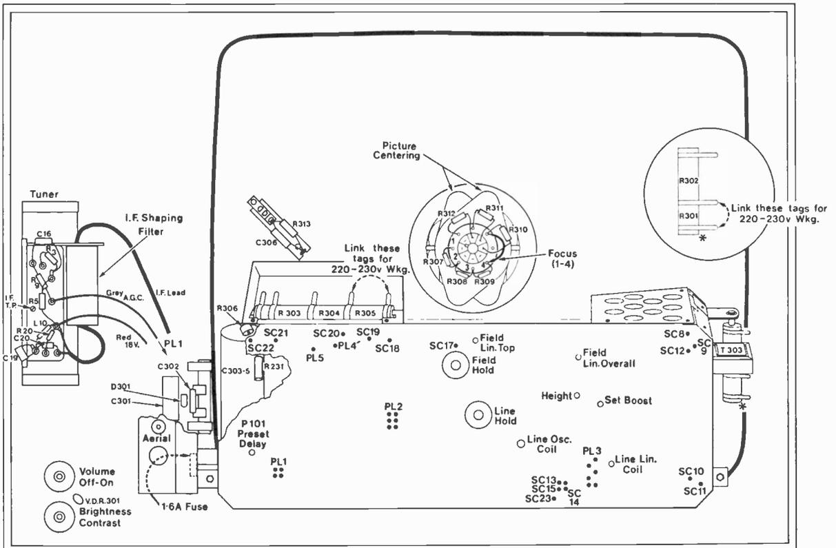
Fig. 2: Rear view (back removed), GEC Series One chassis.
