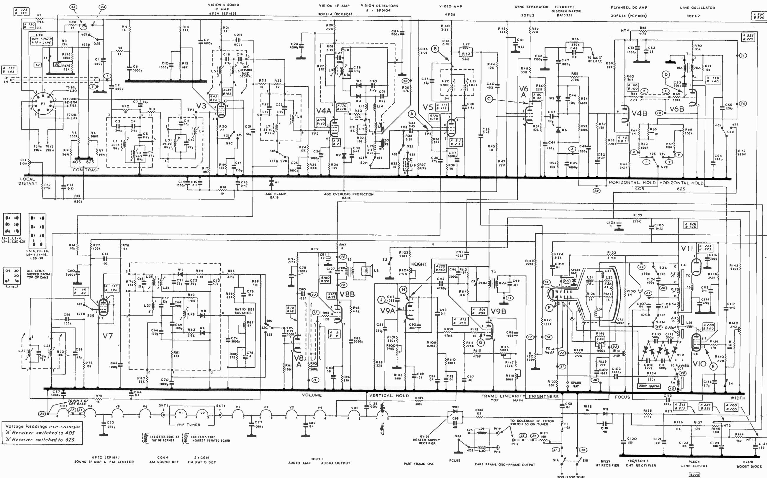
Fig. 1: Circuit diagram of the Thorn/BRC 1400 chassis, Schedule E version incorporating the modifications which will be listed next month. R137 is 226Ω in early versions in which R145 is not fitted. Voltages were measured with no signal and R11 and the contrast controls at maximum, using a 20,000Ω/V meter (AVO Model 8) except for the e.h.t.—variations of 10-20% are not to be taken as indicating a fault condition.
