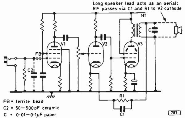
Fig. 6: Valve audio amplifier. R.F. pickup via the speaker leads results in V2 acting as a detector if the level is high enough. Pickup at the audio input can be prevented by a shunt capacitor (C2) or a ferrite bead (FB) on the grid lead. In serious cases a combination of filtering at each stage may be needed.
