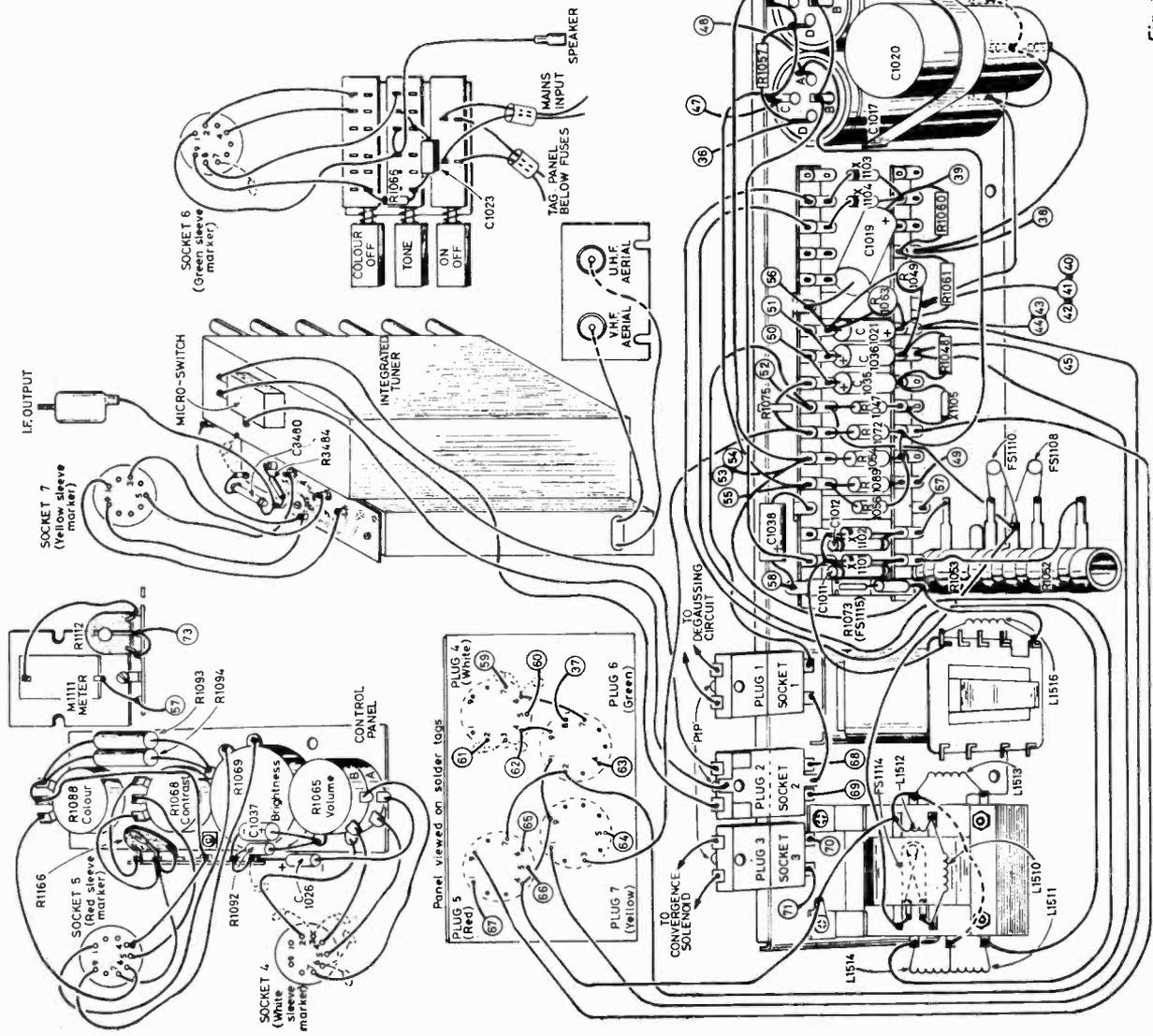
Fig. 13: Control panel and lower chassis component layout.
