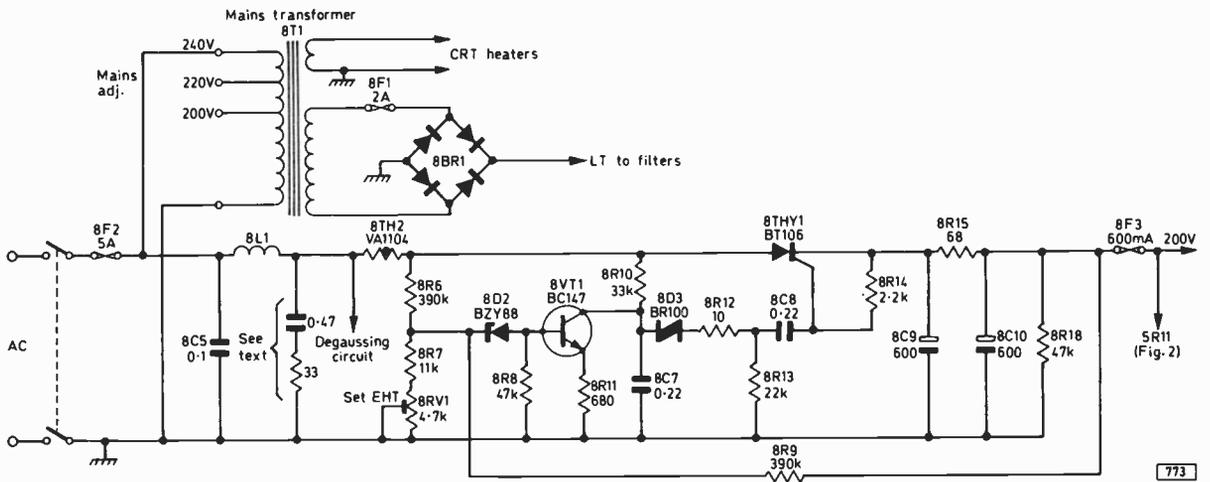
Fig. 1: Power supply circuits of the RBM single-standard colour chassis. 8R13 has been reduced to 1kΩ in current production and this modification is recommended where field jitter is experienced.
