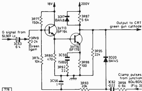
Fig. 4: The G channel. The circuits of the R and B channels are identical. The clamp pulses are also inverted and fed to the SL901 i.c. via the brightness control which thus acts on the clamping level.
