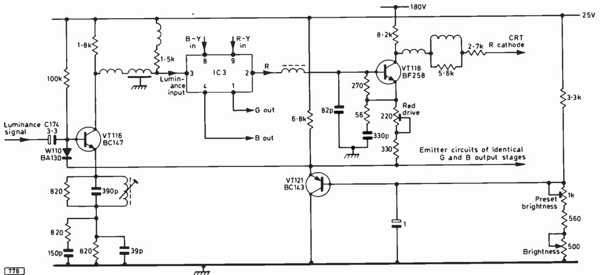
Fig. 2: The emitters for the RGB output transistors in the BRC 8000 chassis are returned to chassis via VT121 whose base bias is set by the brightness control. The cathode of the d.c. restorer diode W110 is also returned to VT121, whose emitter voltage thus determines the d.c. potential on which the luminance signal (negative-going at VT116 base) is imposed. The overall gain of the output stages, and the luminance level, are thus varied by the action of the brightness control.
