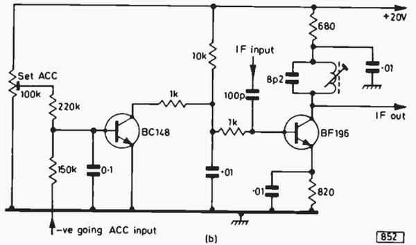
Fig. 4: (a) The original a.c.c. circuit on the RBM i.f. board. (b) Modified a.c.c. circuit to suit the input from the Mullard type decoder.
