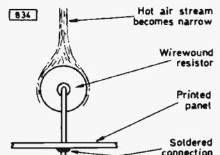
Fig. 2: The hot air stream from say a wirewound resistor does not usually spread out but on the contrary becomes narrow and of high temperature.
