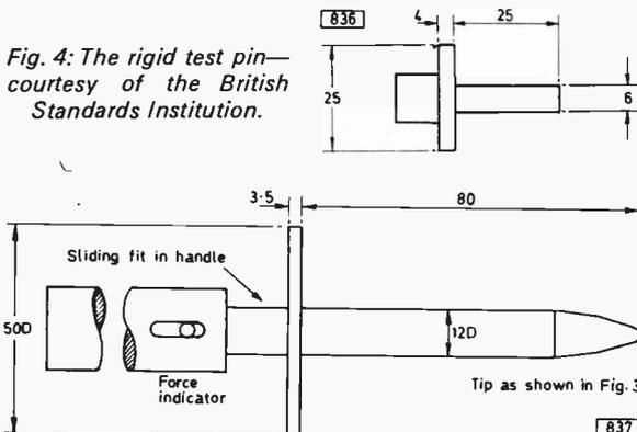
Fig. 4: The rigid test finger—courtesy of the British Standards Institution.
