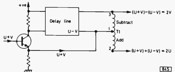
Fig. 4: Typical practical chroma delay line circuit.
