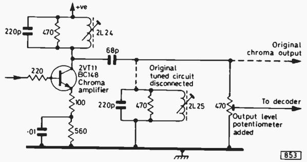
Fig. 5: Modification to the chroma amplifier on the RBM board to make it suitable for feeding the Mullard type decoder circuit.
