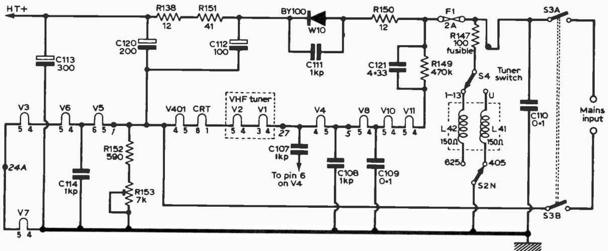
Fig. 2: Power supply circuit with capacitive (C121) heater dropper (early 960 chassis).
