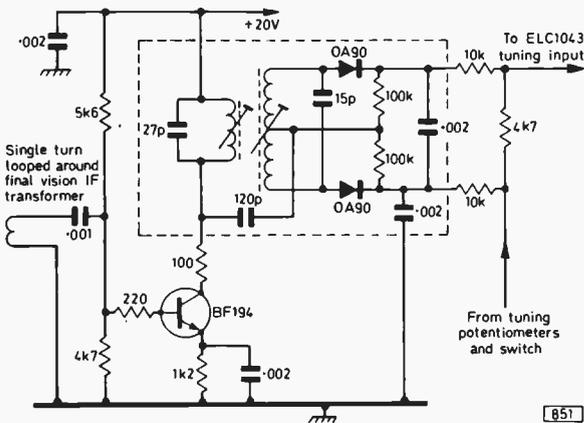
Fig. 3: A.F.C. circuit. The secondary winding consists of 12 turns of 42 s.w.g. wire, bifilar wound with one wire diameter spacing. The primary winding consists of 7 turns of 38 s.w.g. wire wound as a single layer 4.5mm. above the secondary. Use a Neosid 722/4 former and two Neosid 6/900 cores.
