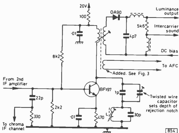
Fig. 6: Luminance i.f. output stage. The rejector *L* was redeployed as a chroma rejector to delete sound-chroma beat patterning.
