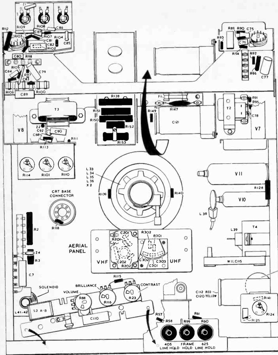
Fig. 4: Rear chassis view of the earlier version of the 960 chassis. Differences in the later version will be shown next month.
