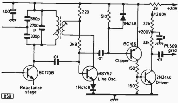
Fig. 11: Modification to the RBM line drive circuit to enable it to drive a valve line output stage.
