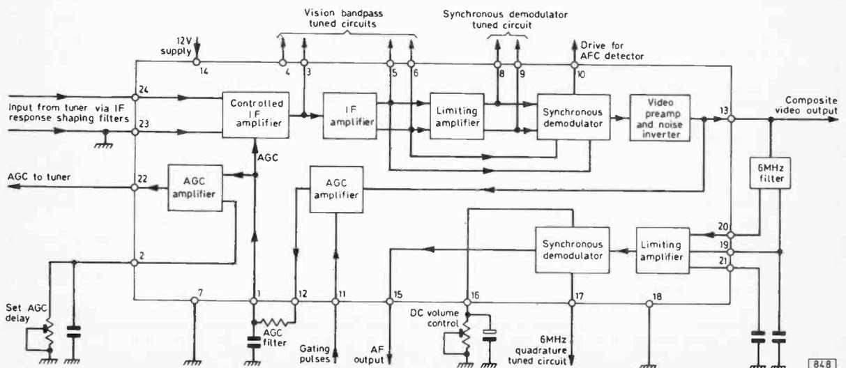
Fig. 1: Block diagram of the SL437F i.c., which provides a complete TV i.f. system.
