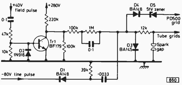
Fig. 12: Blanking and beam limiting circuits.
