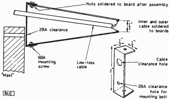
Fig. 1: Cross-section of the assembled aerial, showing the taper. The separation between the insides of the two printed boards at the front is  $\frac{1}{2}$  in.
