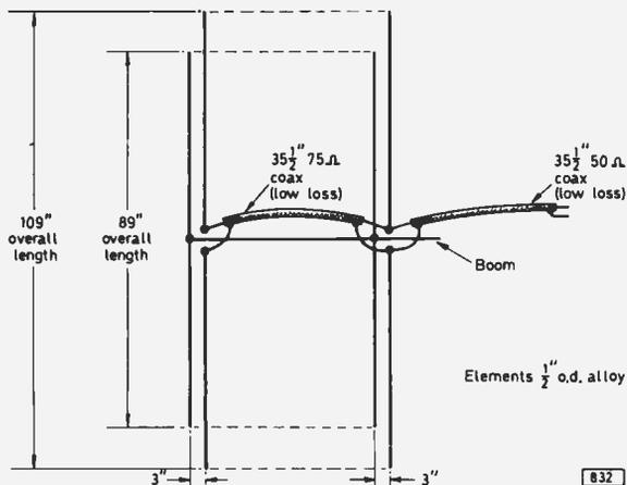
Fig. 1: Exploded view of the improved Band I omnidirectional array. The dipole assemblies are mounted at right angles to each other—see accompanying photograph.
