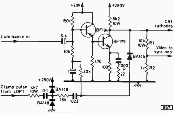
Fig. 9: One of the RGB circuits. One of these was used as shown here for initial testing (see next month), with the luminance signal applied to the input, the output fed to all three c.r.t. cathodes and R1 and R2 used to provide a feed to the sync separator. For RGB use omit R2 and connect R1 to chassis.
