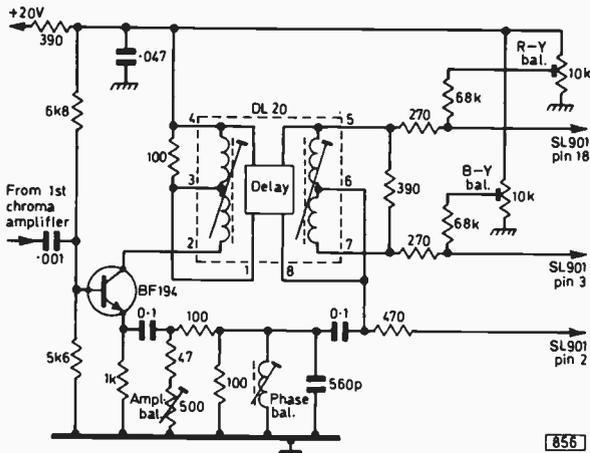
Fig. 8: Chroma delay line circuit, modified to feed the SL901 i.c.
