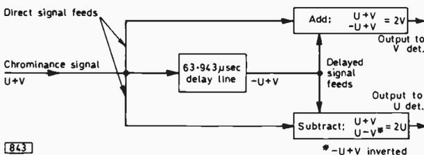
Fig. 2: How the chrominance delay line and its associated add and subtract networks in a PAL decoder separate the two transmitted colour-difference signals prior to demodulation.
