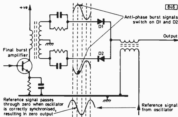
Fig. 5: The type of burst demodulator used locks the reference oscillator in quadrature with the transmitted bursts as shown here.
