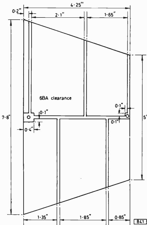
Fig. 3: The printed circuit board pattern. Two boards are required, mounted as shown in Fig. 1. Dimensions given are for a group CD aerial; for group B multiply all dimensions by 1.2 and for group A by 1.5. The width of the conducting strips is 0.1 in. Shown half scale.
