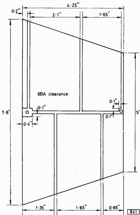
Fig. 3: The printed circuit board pattern. Two boards are required, mounted as shown in Fig. 1. Dimensions given are for a group CD aerial; for group B multiply all dimensions by 1.2 and for group A by 1.5. The width of the conducting strips is 0.1 in. Shown half scale.
