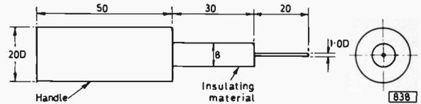
Fig. 6: Test pin—courtesy of the British Standards Institution.
