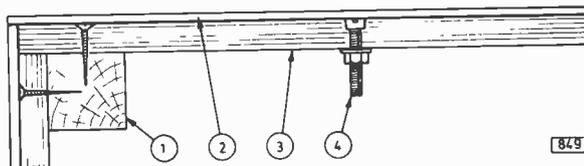
Fig. 1: Cabinet corner joint. (1) 1 x 1in. timber glued and screwed into corner. (2) Veneers fitted with top overlapping side pieces to give a neater joint. (3) Main cabinet consists of  $\frac{3}{4}$ in. plywood. (4) Bolt and locknut for chassis, transformer, etc., fitted before veneering.
