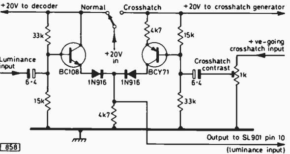
Fig. 10: Crosshatch input and switching circuit.
