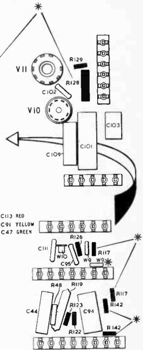
thermistor. Note that whereas the output from h.t. rectifier W10 is positive that from the heater rectifier W12 is negative. The surge limiting resistors for the two rectifiers, R149 and R150, are wound on a substantial ceramic former mounted at the top centre of the chassis along with the fusible resistor R147.
