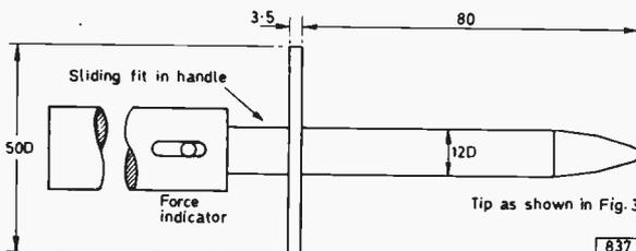
Fig. 5: The rigid test finger—courtesy of the British Standards Institution.
