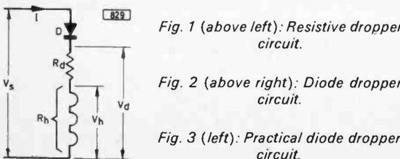
Fig. 2 (above right): Diode dropper circuit.
