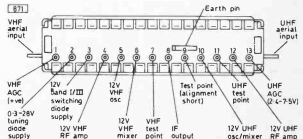
Fig. 2: ELC2000S varicap tuner pin connections. Note that the output from the u.h.f. section is coupled to the v.h.f. mixer.
