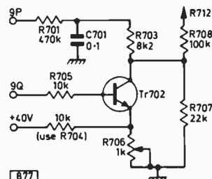
Fig. 1 (left): Modified beam limiter circuit used by W. Hill in the "Television" colour receiver.
