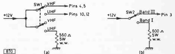
Fig. 1: Band switching arrangements for use with the Mullard ELC2000S varicap tuner. (a) U.H.F./V.H.F. switching. (b) Switching the supply to the Band I/III switching diodes. SW1 and SW2 are RS miniature toggle switches.
