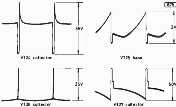
Fig. 5: Waveforms around the circuit.
