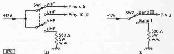
Fig. 1: Band switching arrangements for use with the Mullard ELC2000S varicap tuner. (a) U.H.F./V.H.F. switching. (b) Switching the supply to the Band I/III switching diodes. SW1 and SW2 are RS miniature toggle switches.
