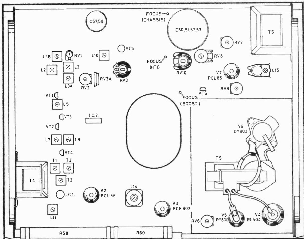
Fig. 1: Plan view of the basic 169 chassis.
