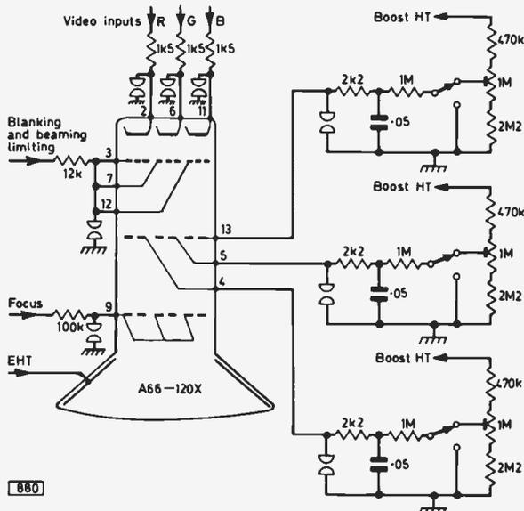
Fig. 15: The tube feed circuits.
