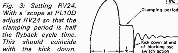
Fig. 3: Setting RV24. With a 'scope at PL10D adjust RV24 so that the clamping period is half the flyback cycle time. This should coincide with the kick down.
