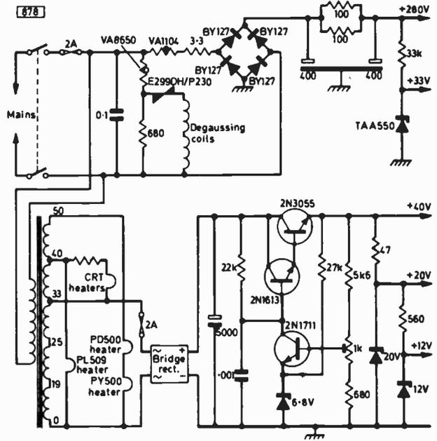
Fig. 13: Power pack circuit.
