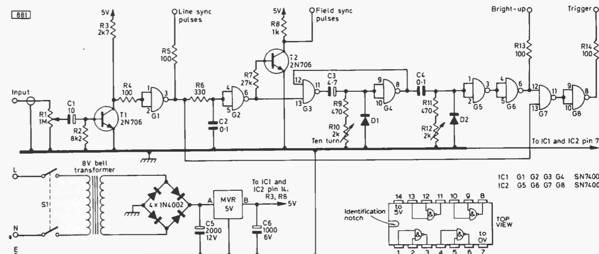
Fig. 1: Full circuit of the TTL test signal extractor unit.
