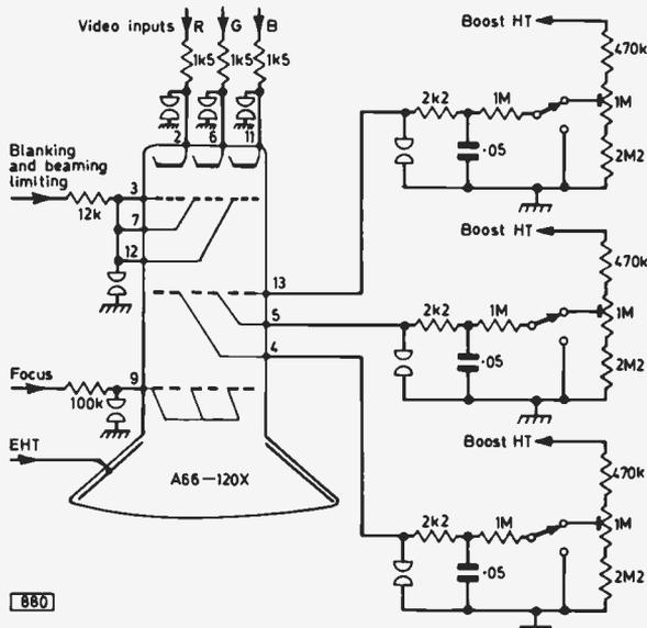
Fig. 15: The tube feed circuits.
