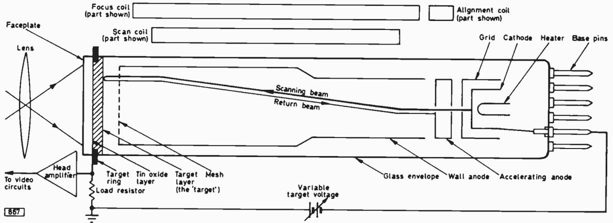
Fig. 2: Vidicon construction and basic external circuit.
