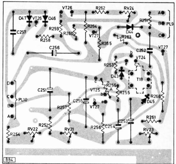
Fig. 6: Print side of the field timebase panel used in the Pye 697 chassis.
