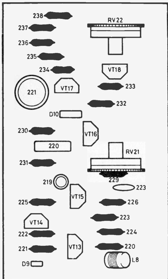
Fig. 3: Layout of the discrete component a.g.c./sync/video board used on the 569 chassis.
