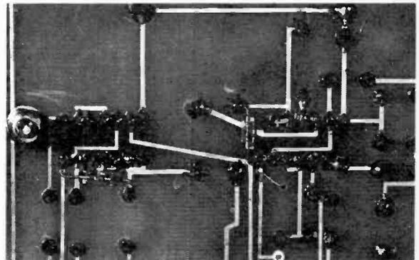
This view of the underside of the board shows the position of the gate protection diodes D1 and D2.
