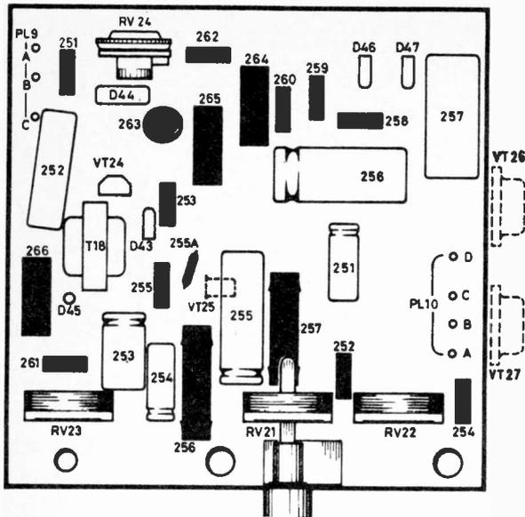
Fig. 4: Layout of the field timebase panel used in the Pye 697 chassis (component side).
