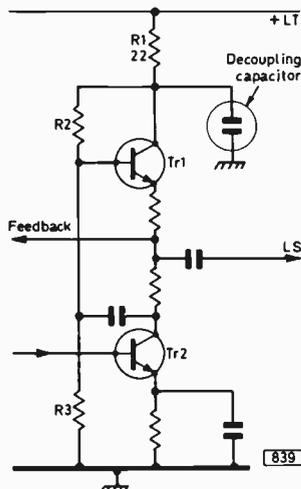
*Fig. 7: If the decoupling capacitor in the supply to this sound output stage becomes short-circuit R1 will be connected between the l.t. rail and chassis. This will produce overheating. Incidentally this particular circuit, a class A push-pull circuit with Tr1 base driven from the collector of Tr2, is not too common. A similar circuit is used in the Philips 320 chassis however. R2 and R3 set the mid-point voltage.*
