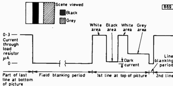
Fig. 4: Representation of the current output waveform obtained when the scene shown at the top is being viewed by a vidicon camera. The blanking periods are also shown. Note the low level of the output (peak 0.3μA).
