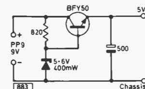
Fig. 2: Regulator for use with a PP9 battery.
