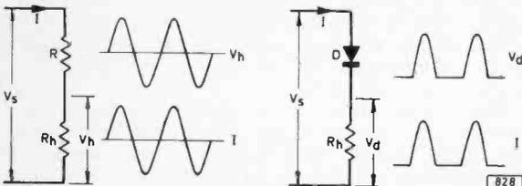
Fig. 1 (above left): Resistive dropper circuit.
