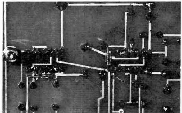
This view of the underside of the board shows the position of the gate protection diodes D1 and D2.
