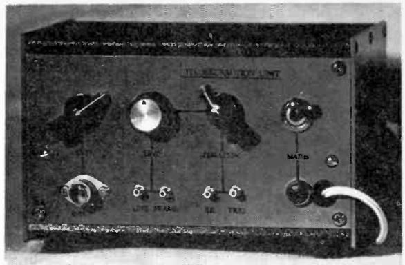
General view of the unit. Note that a round knob is used for the ten-turn potentiometer (R10).
