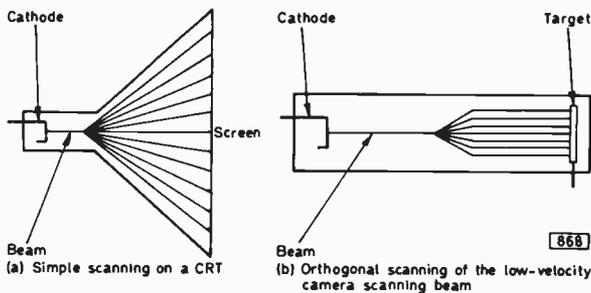
Fig. 3: Comparison between (a) normal c.r.t. scanning and (b) low-velocity beam orthogonal scanning as used with a vidicon tube.
