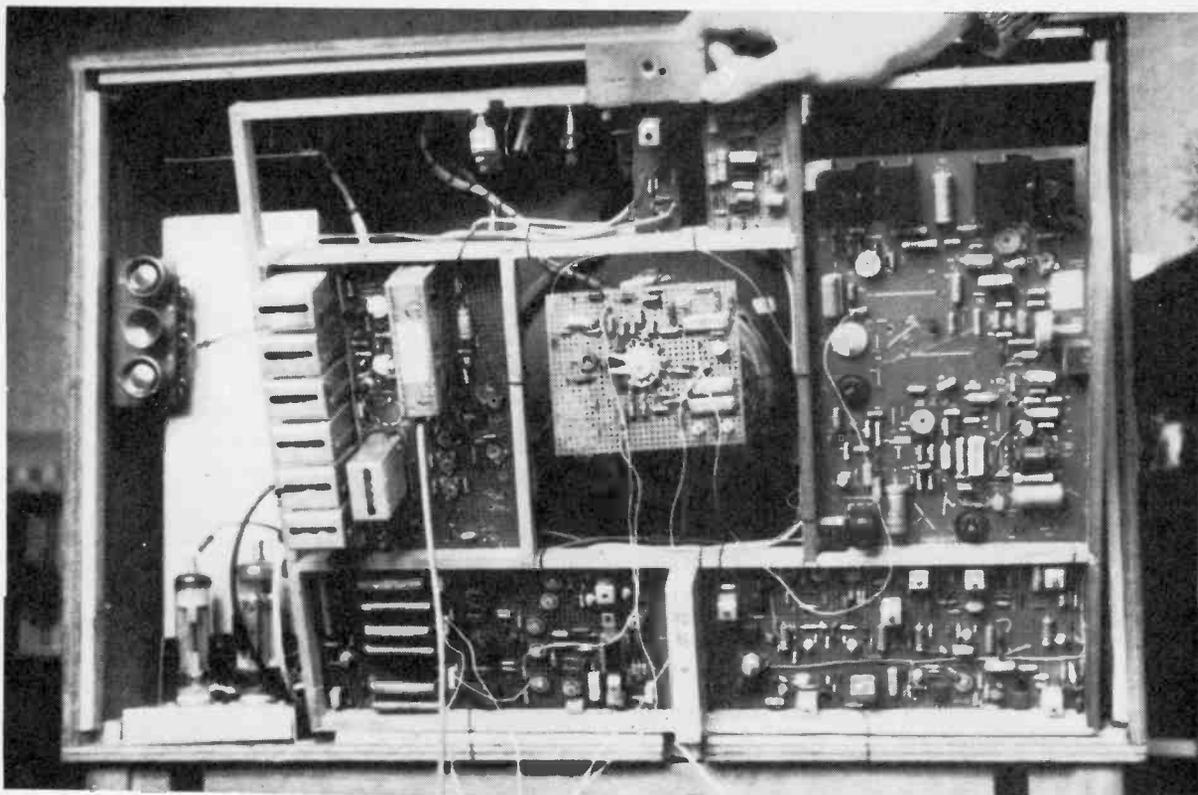
General view from rear, showing how the frame hinges down.
