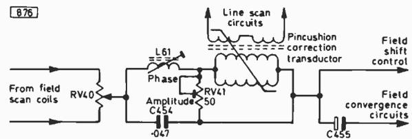
Fig. 7: Connections between the pincushion distortion correction circuit and the field scan and convergence circuits. RV41 tends to go open-circuit.
