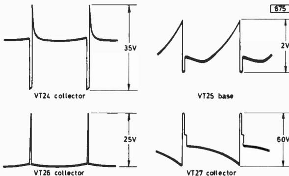
Fig. 5: Waveforms around the circuit.
