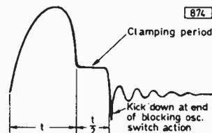
duration of the blocking oscillator flyback switch action. This setting can be done in two ways: either connect a meter from the scan coil feed (plug PL10D) to chassis and set RV24 for the meter to read 2V higher than the mid-point between l.t.+ and l.t.—, or connect a 'scope across PL10D and chassis and adjust RV24 for the end of period (c) to coincide with the kick down of the trace (this denotes the end of the oscillator flyback switch pulse, see Fig. 3).
