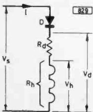
Fig. 3 (left): Practical diode dropper circuit.
