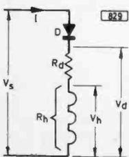
Fig. 3 (left): Practical diode dropper circuit.
