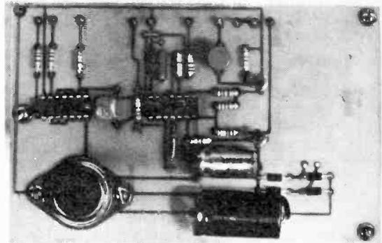
Top view of the circuit board. Reservoir/smoothing capacitor values used happened to be handy: better to use the values specified.
