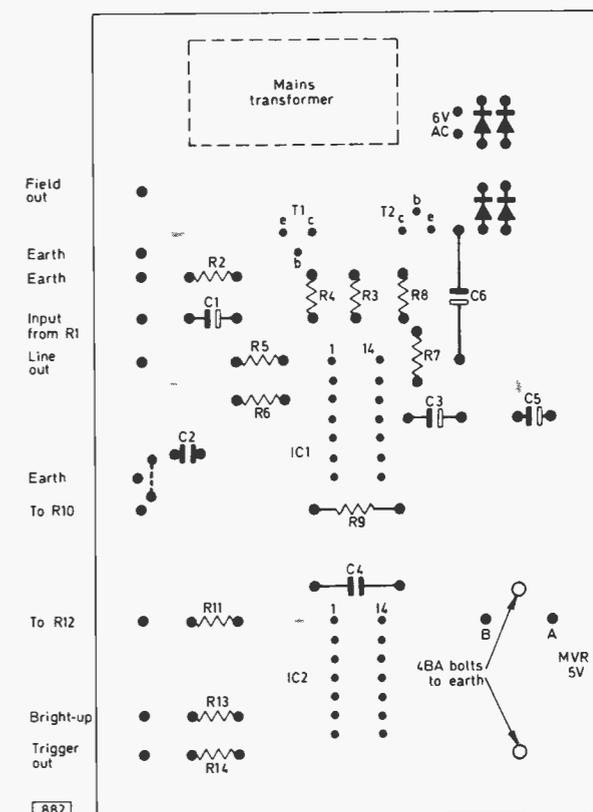
Fig. 3: Suggested board layout, viewed from the component side. D1 and D2 are mounted on the print side.
