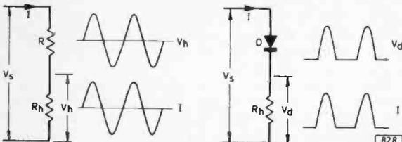
Fig. 1 (above left): Resistive dropper circuit.
