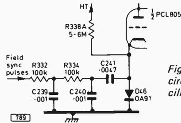
Fig. 1: Sync pulse feed circuit to the field oscillator in the ITT CVC5 colour chassis.
