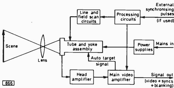
Fig. 1: Block diagram of a typical vidicon camera.
