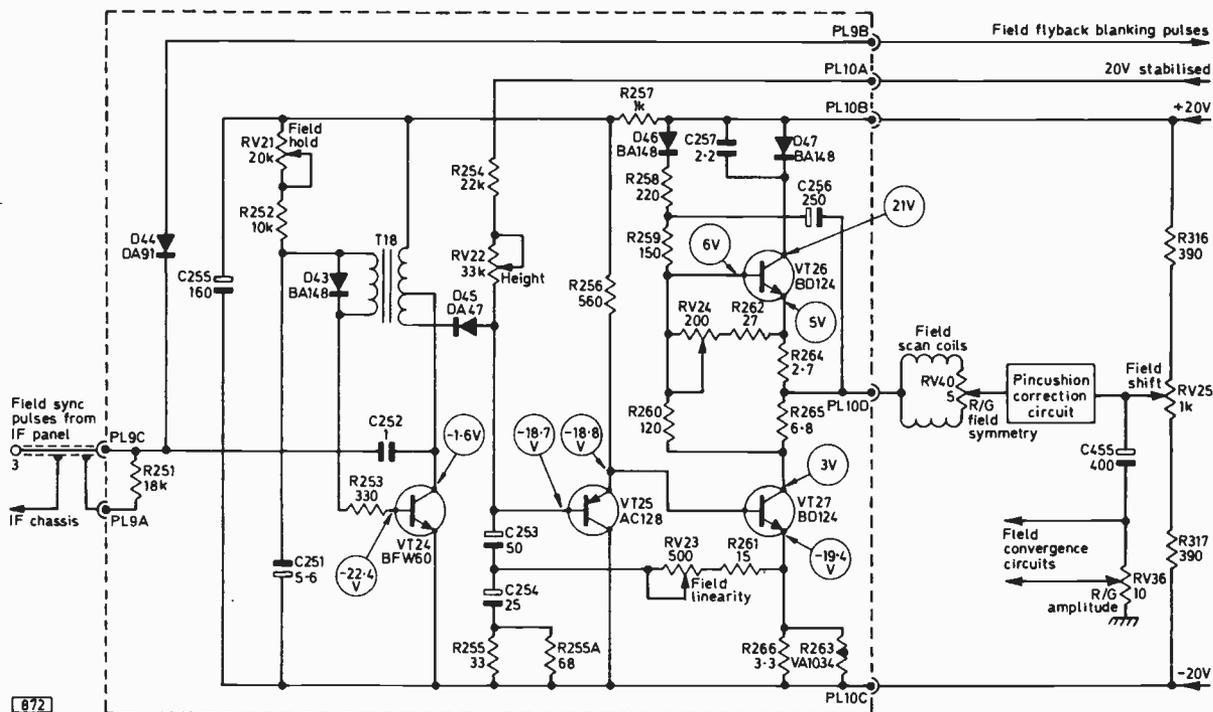
Fig. 1: Transistor field timebase circuit as used in the Pye 697 chassis.
