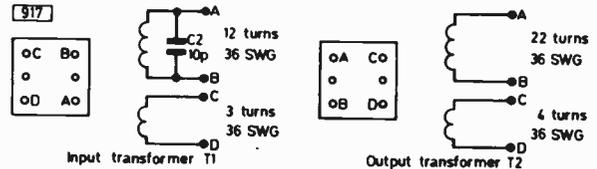
Fig. 7. I.F. transformer winding details.
