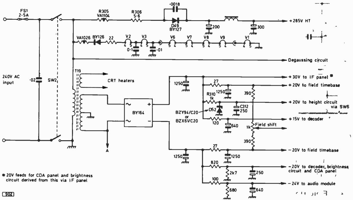
Fig. 1: The power supply circuit. Some models use an i.c. in place of the audio module; the -26.5V supply required for this is obtained from an additional 1N4002 rectifier connected to point A above.
