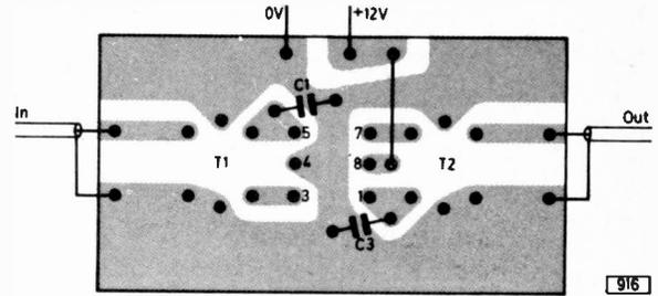
Fig. 6: Layout of the printed circuit.
