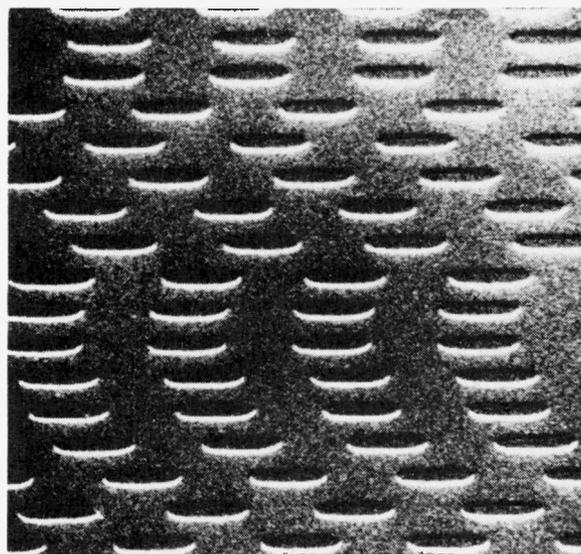
*The signal is recorded on the surface of the disc as a track of pits: this photograph shows the pits in a minute section of the surface of the disc.*
