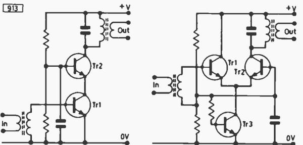
Fig. 1 (left): Cascode amplifier circuit.
