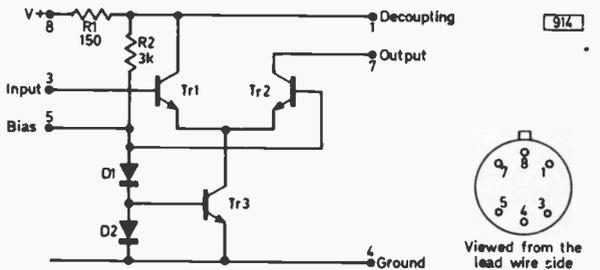
Fig. 3 (left): Circuit of the  $\mu A703$  i.c.
