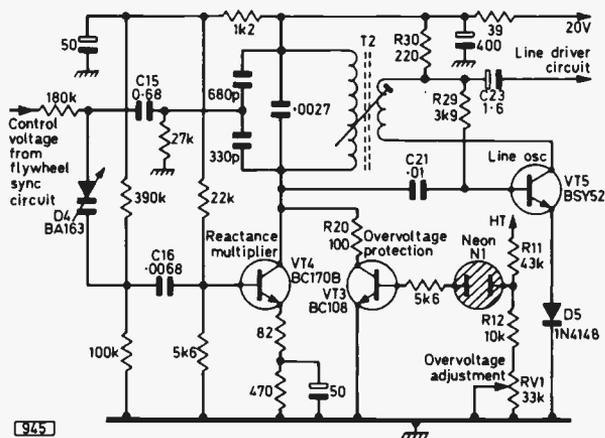
Fig. 4: Line generator circuit used in earlier versions of the RBM 90° single-standard colour chassis. The capacitance of varicap diode D4 is varied by the output from the flywheel sync discriminator circuit. Since D4 is connected in the capacitive feedback loop between the collector and base circuits of VT4 this adjusts the degree of reactive feedback. In effect VT4 acts as a reactance multiplier, amplifying the small capacitance changes in D4.
