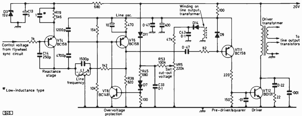
Fig. 5: Line generator and driver circuits used in later RBM 90° single-standard colour chassis.
