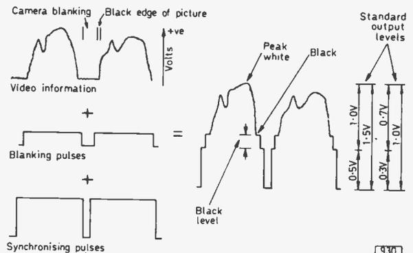
Fig. 1: Showing the make up of two successive lines of the composite camera output waveform (not to scale).
