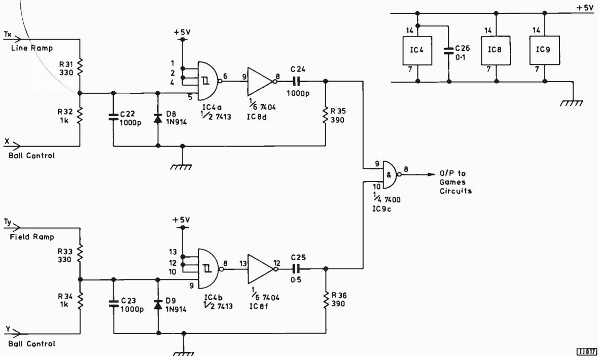
Fig. 7: Circuit diagram of the ball control system. This is built on the same board as the man circuits.
