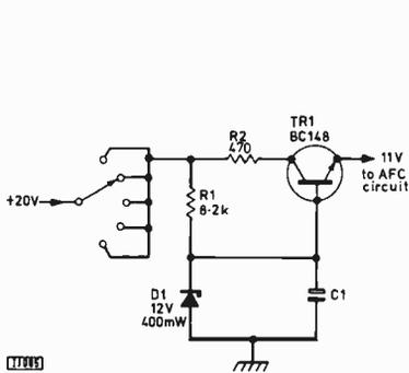
Fig. 1: Basic slow run-up regulator circuit adopted to provide electronic a.f.c. muting.
