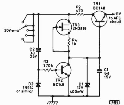
Fig. 3: An f.e.t. (TR3) can be used in place of R1: this enables smaller value electrolytics to be used.
