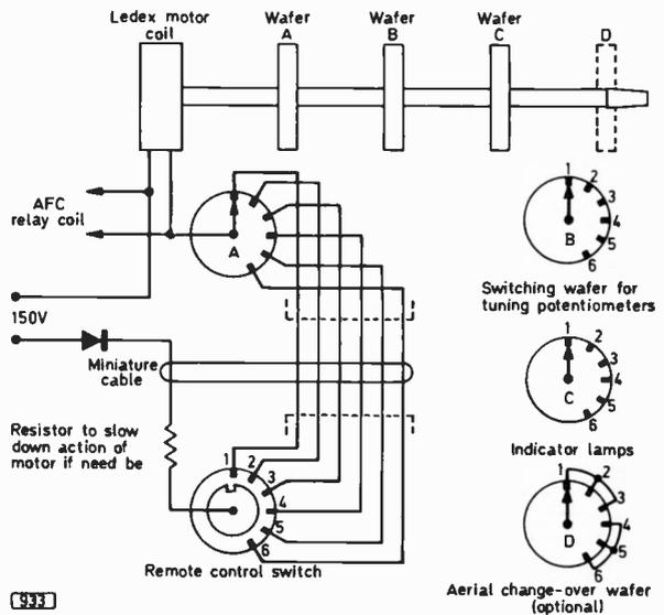
Fig. 1: Remote control system suggested by B. D. Dodd.
