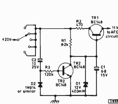
Fig. 2: Improved version—in this circuit C2 provides the delay, C1 providing smoothing.
