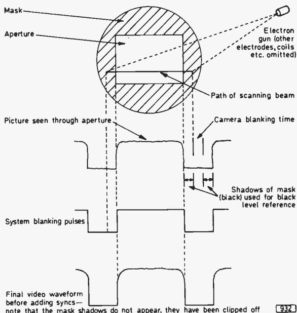
Fig. 3: One method of obtaining a black level reference.
