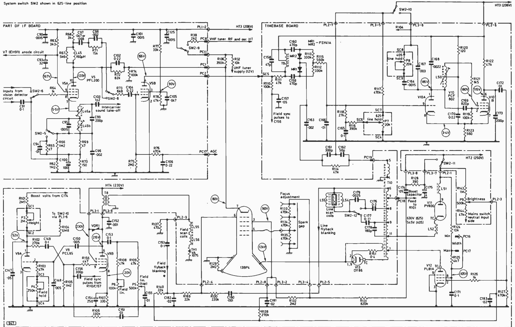
Fig. 1: The video amplifier, sync separator, timebase and c.r.t. circuit.
