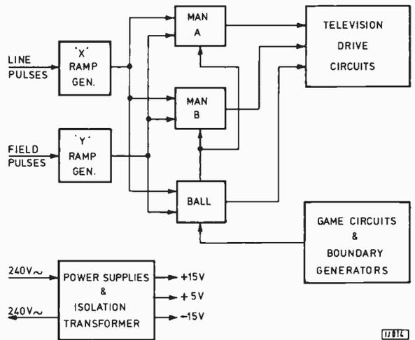
Fig. 1: Block diagram of the basic game system.
