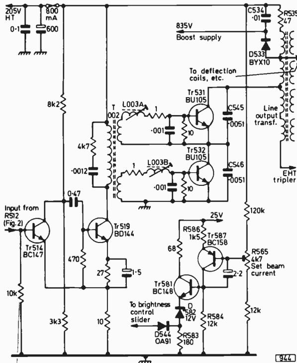
Fig. 3: Line output circuit used in later versions of the Philips G8 chassis, with two-transistor beam limiter circuit. (BY14 scan unit.)
