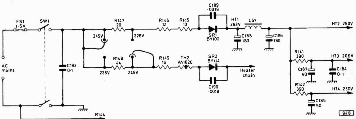
Fig. 5: Power supply circuit. H.T. voltages apply on 625 lines—they are slightly higher on 405 lines.
