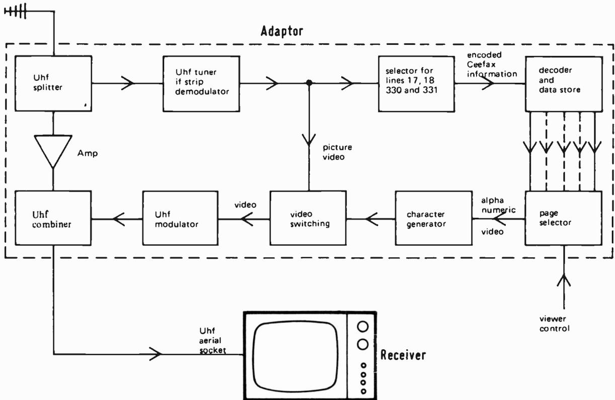
Fig. 1: Block diagram of a Ceefax adapter unit, courtesy BBC.
