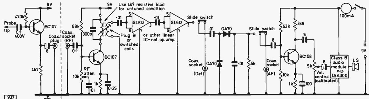
Fig. 3: A.M. signal tracer. All sections of the circuit except the class B audio module and the loudspeaker should be screened. The SL612 requires 6V at pin 2: pins 4 and 8 should be earthed and there is no connection to pin 1.
