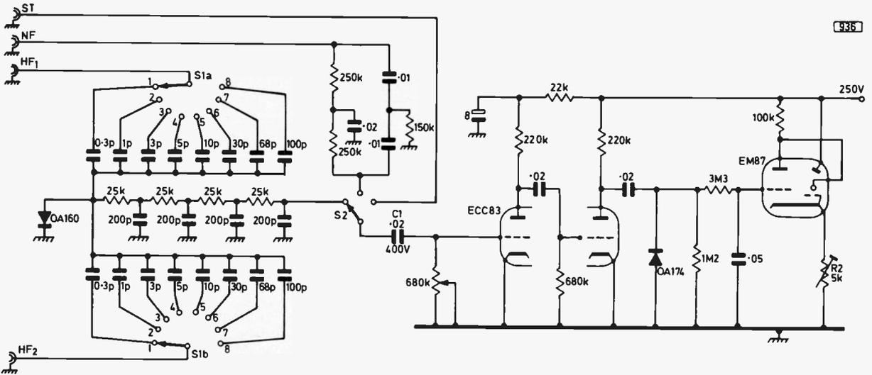
Fig. 2: Circuit (slightly modified) of the Telefunken design for a signal tracer and frequency comparator. Note that networks of capacitors like those at S1a and S1b could also be used at the ST and NF inputs—without the OA160 and 25k Ω/200pF filter.
