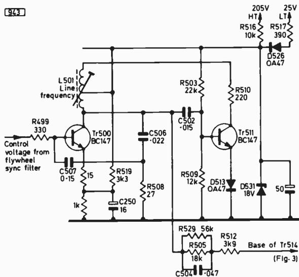
Fig. 2: The line generator circuit used in the Philips G8 chassis. The reactance transistor Tr500 tunes the lower half of the oscillator coil L501.
