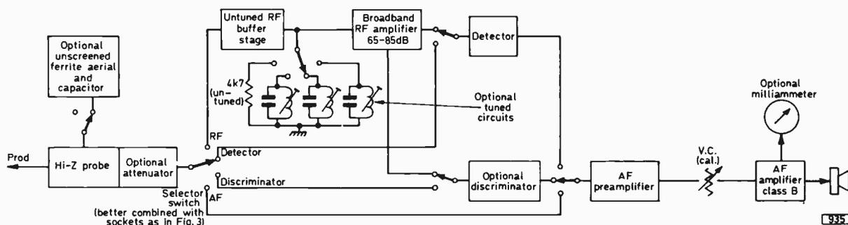
Fig. 1: Signal tracer block diagram, showing optional features that can be incorporated to increase the instrument's usefulness. The untuned r.f. buffer stage would be needed only to isolate the optional tuned circuits from the optional attenuator.
