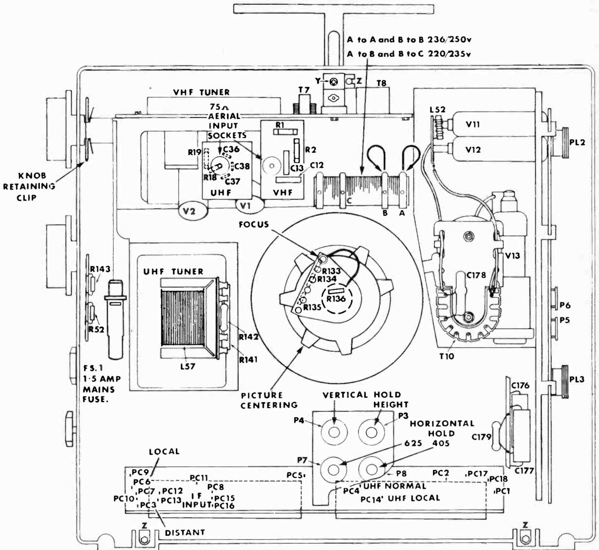
Fig. 4: Rear view of the receiver with the cabinet back removed. Screw Y and distance piece secure the handle. The three screws Z secure the chassis to the cabinet.
