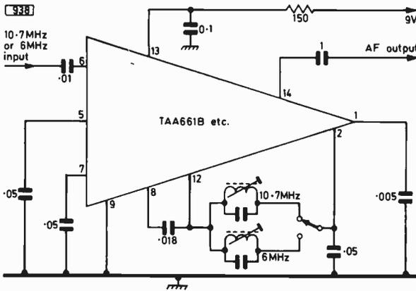
Fig. 4: Use of a coincidence (quadrature) f.m. discriminator integrated circuit.
