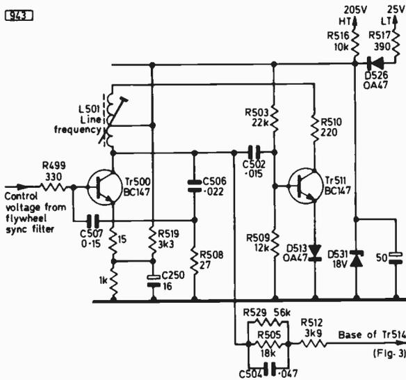
Fig. 2: The line generator circuit used in the Philips G8 chassis. The reactance transistor Tr500 tunes the lower half of the oscillator coil L501.
