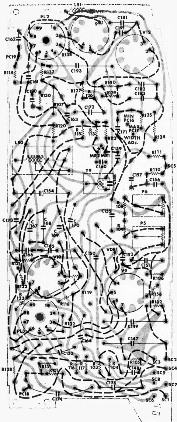
Fig. 2 (left): Layout of the timebase panel, viewed from the tin dip side (components on other side).
