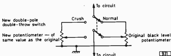
Fig. 2: Adding a black crush control.
