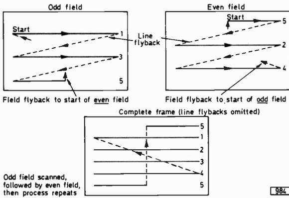
Fig. 1: 5-line, 2:1 interlaced system, showing the build up of the frame from two fields.
