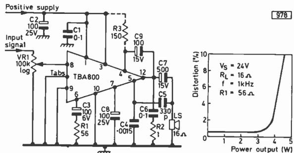
Fig. 3 (left): Alternative circuit with the loudspeaker returned to chassis—this reduces hum problems.
