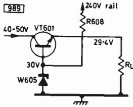
Fig. 1 (left): Operation of the series emitter-follower (VT601) which stabilises the 30V rail.
