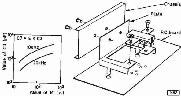
Fig. 11 (left): Value of  $C_3$  needed for use with various values of  $R_1$  when a response 3dB down at 10kHz and 20kHz is required. It is assumed that the value of  $C_7$  is five times that of  $C_3$ .
