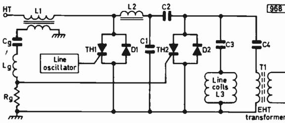
Fig. 1: Basic elements of the thyristor line timebase used with thin-neck  $110^\circ$  shadowmask tubes.
