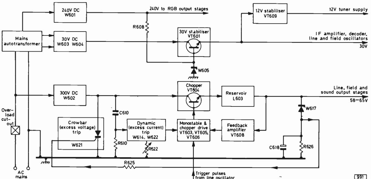
Fig. 3: Block diagram of the power supply arrangements used in the BRC/TCE 3000/3500 colour chassis.
