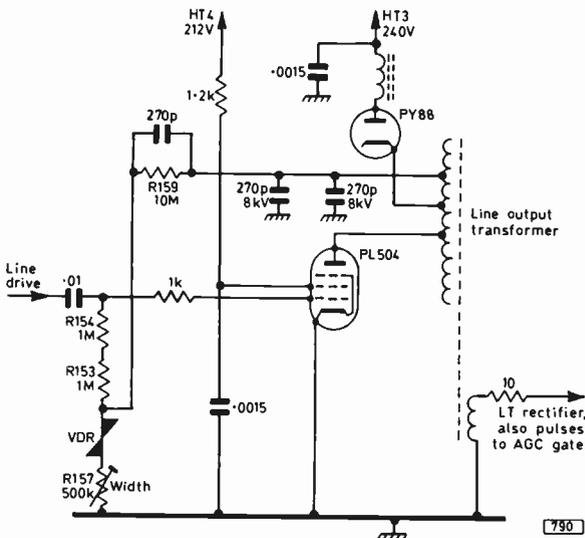
Fig. 1: ITT VC200 chassis line output stage.
