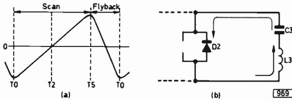
Fig. 2: (a) Output current waveform. (b) Current path during the period  $T_0$ - $T_2$ .
