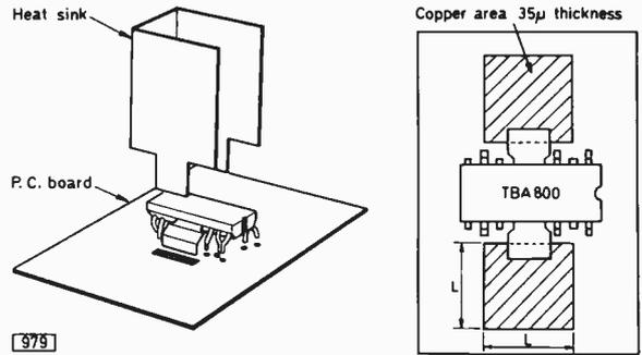
Figs. 5 and 6: Alternative heatsink arrangements for the TBA800 and TBA810S.
