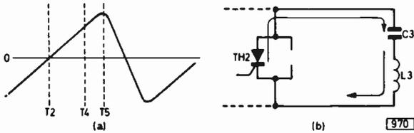
Fig. 3: Condition of the circuit between times  $T_2$  and  $T_4$ , with  $TH_2$  conducting.
