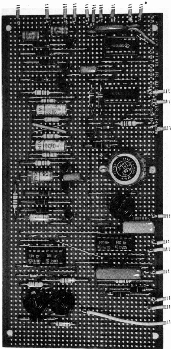
Photograph of the simple game board, showing the component side.
