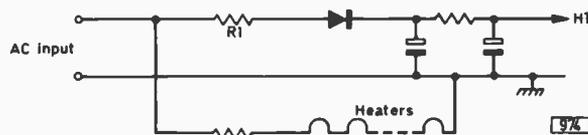
Fig. 1: A simple mains input circuit for monochrome receivers using valves.
