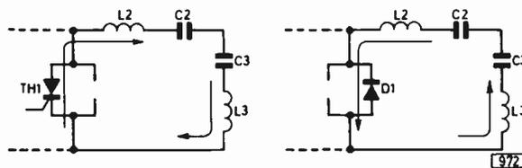
Fig. 5 (left): Between times  $T_5$  and  $T_6$   $TH_1$  conducts while  $D_2$  and  $TH_2$  are both cut off.
