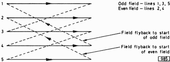
Fig. 2: An alternative method of scanning with a 5-line 2:1 interlaced system.
