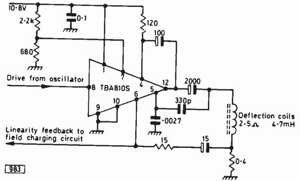
Fig. 13: Field output stage for 12-17in. monochrome receivers, using the TBA810S.
