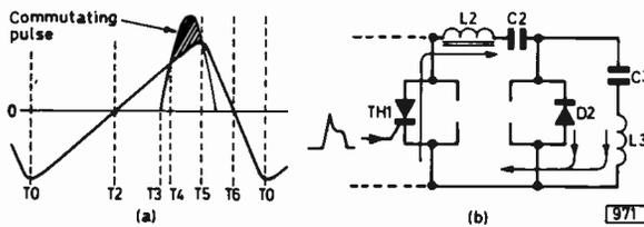
Fig. 4: Thyristor  $TH_1$  is triggered by a pulse from the line oscillator at time  $T_3$ . When the amplitude of the commutating pulse exceeds that of the scan current (time  $T_4$ )  $D_2$  switches on again and  $TH_2$  is switched off.
