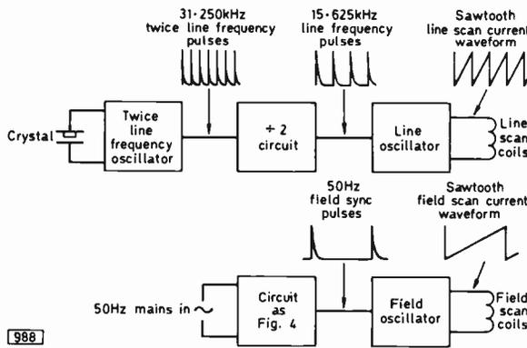
Fig. 5: Block diagram of a camera operating in the random interlace mode.
