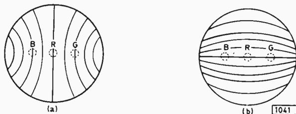
Fig. 6: The predistortion introduced by the horizontal scan coils is pincushion shaped (a), that introduced by the vertical scan coils is barrel shaped (b).
