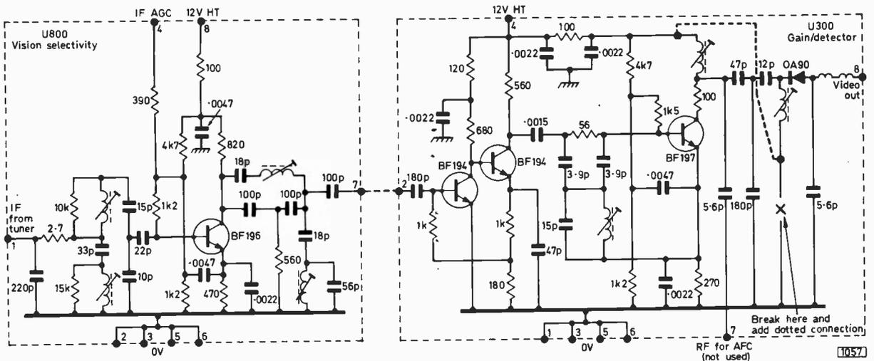
Fig. 3: Circuit of the Philips G8 i.f. strip showing the modification required to change the d.c. component of the output signal.
