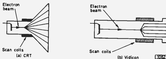
Fig. 1: Comparison between conventional c.r.t. scanning and the orthogonal scanning used with a vidicon tube.
