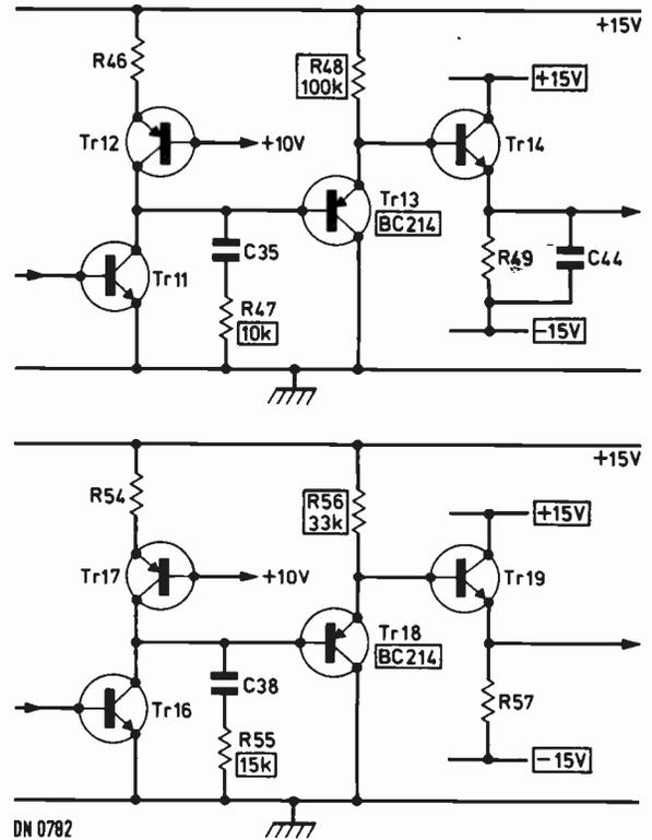
Fig. 31: Circuit diagram for the improvements to the Ramp Generators (Fig. 8). Changes to components and circuitry are shown boxed.
