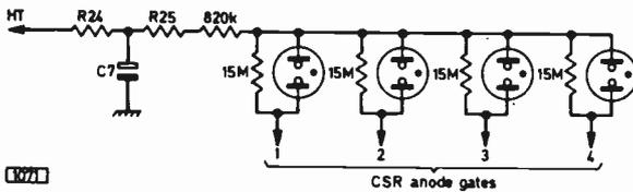
Fig. 1: Modification to the digital touch tuner unit where miniature neons are to be used instead of a numicator tube.
