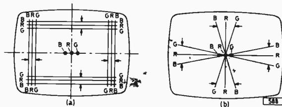
Fig. 5: Dynamic convergence is factory preset by tilting the deflection yoke: (a) if the yoke is tilted horizontally to the left the size of the green raster is increased (as indicated by the arrows) while that of the blue raster is decreased; (b) if the yoke is tilted vertically upwards the green raster is rotated in an anticlockwise direction while the blue raster is rotated in a clockwise direction.
