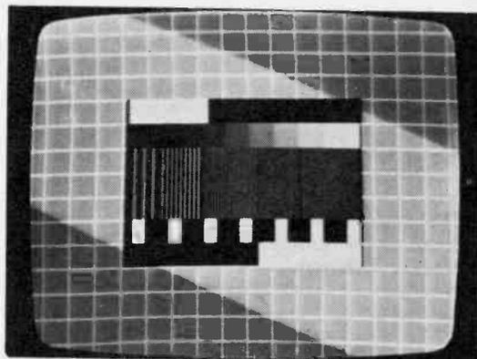
*SFB Berlin ch. E7 test card, showing effect of a focal-plane shutter camera set at 1/15th second. Photo courtesy Dieter Scheiba.*
