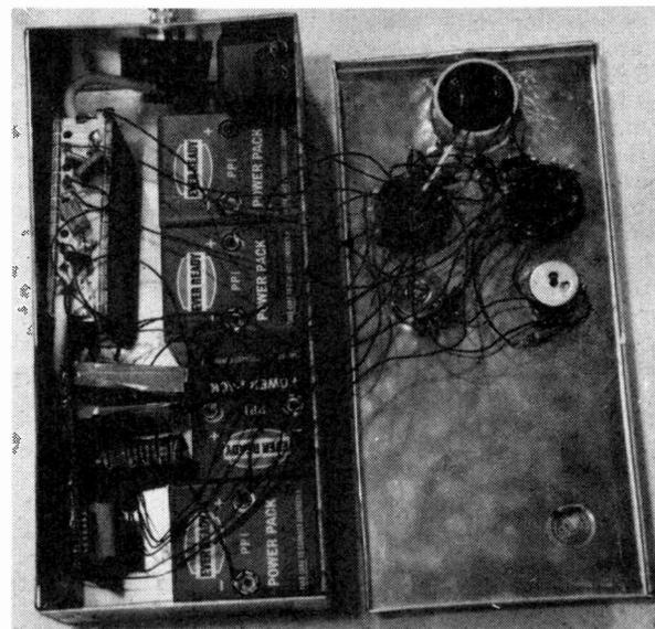
Arrangement of the interior of the Signal Strength Meter.
