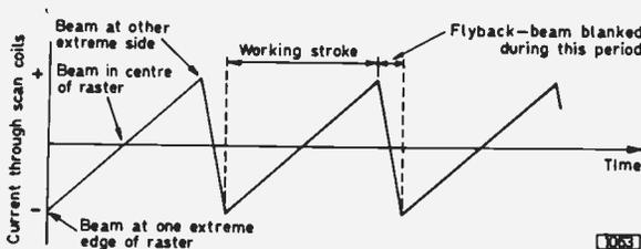
Fig. 2: The basic scanning current waveform.
