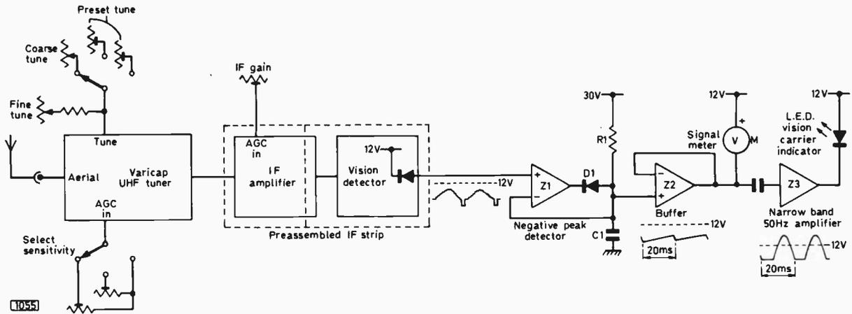
Fig. 1: Block diagram of the Signal Strength Meter.
