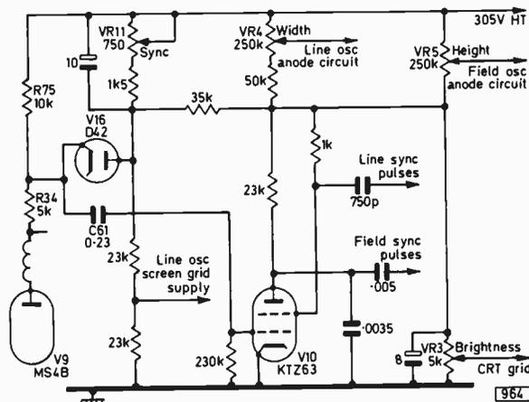
Fig. 3: The complex sync circuit used in Model 904—who thought up that lot? Blocking oscillators were used in both the field and line timebases, with the line output stage transformer coupled and the field output stage RC coupled to the deflection coils.
