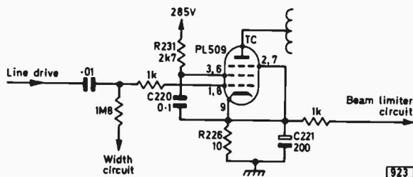
Fig. 1: Screen grid and cathode circuits of the PL509 line output stage used in the Pye group 691 chassis.
