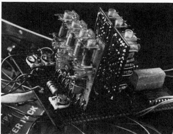
*The two i.f. modules are edge-mounted on the Veroboard.*
