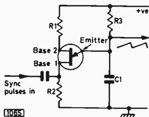
Fig. 4: The unijunction transistor sawtooth generator. This free-running oscillator can be synchronised by applying negative-going sync pulses to the transistor's base 1 connection.
