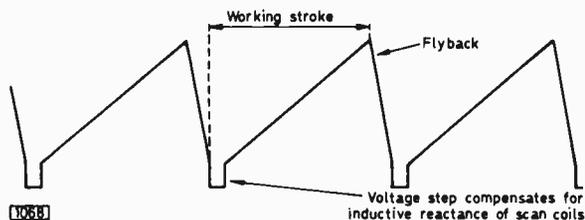
Fig. 8: Practical field scan voltage waveform.
