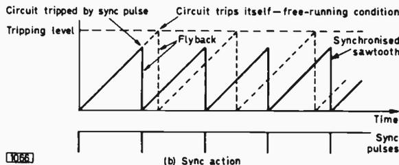
Fig. 5: Sawtooth generator waveforms. Whether the sync pulses are negative- or positive-going depends on the circuit being synchronised: they are shown negative-going here to meet the requirements of the circuit just shown (Fig. 4).
