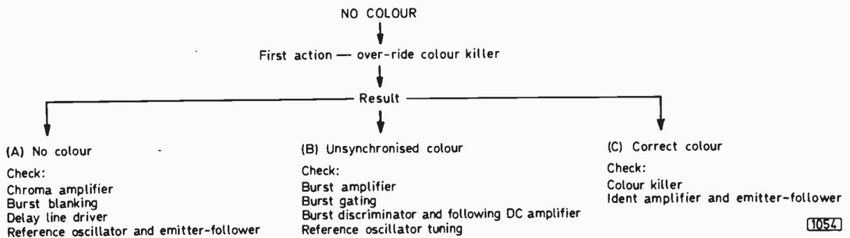
Fig. 2: Fault finding chart for the two basic decoding faults, no colour or unsynchronised colour.
