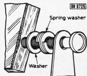
Fig. 2 (right): Detail of the assembly, showing the correct positions for the flat and spring washers.
