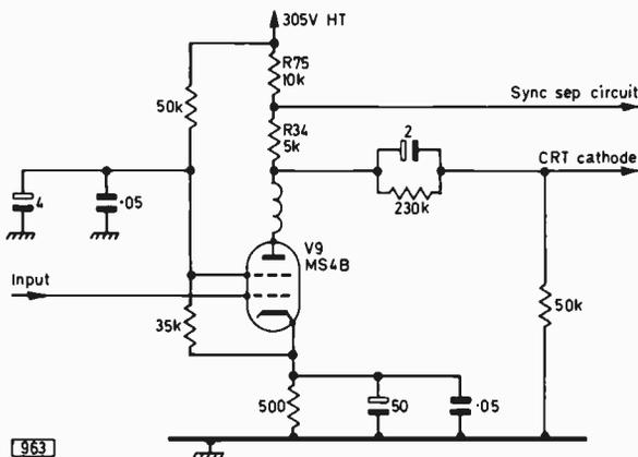
Fig. 2: The video circuit used in Model 904. The MS4B acted as vision detector and output stage. R34 was the load during the picture portion of the waveform, R75 being brought into circuit when the sync pulses arrived (see Fig. 3).
