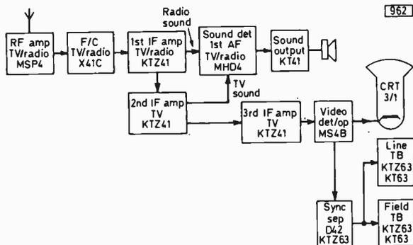
Fig. 1: Block diagram of the HMV Model 904.
