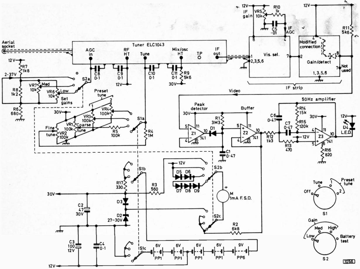
Fig. 2: Circuit diagram of the prototype meter using the Mullard ELC1043 u.h.f. tuner and Philips G8 i.f. strip. If other modules are used, the connections must, of course, be altered to suit.
