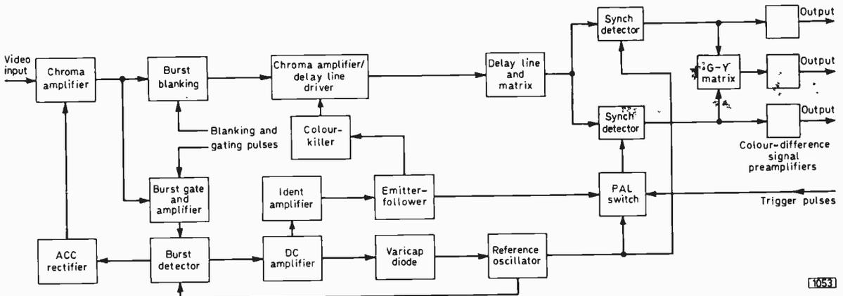
Fig. 1: Block diagram of a typical PAL-D decoder. The reference oscillator output is generally taken via an emitter-follower buffer stage (not shown above). The outputs from top to bottom are B-Y, G-Y and R-Y.
