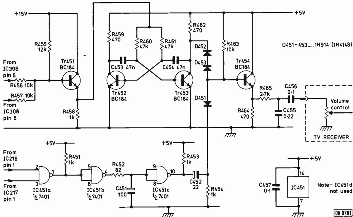
Fig. 30: This circuit produces sound effects for the Football game. The pitch of the note is controlled by the velocity of the ball by means of the summing amplifier Tr451 which varies the "aiming voltage" of the multivibrator. IC451b and c form a pulse stretching circuit for the coincidence pulses. This more sophisticated circuitry (compared with Fig. 28) is necessary because of the much shorter pulses coming from IC216 and IC217.
