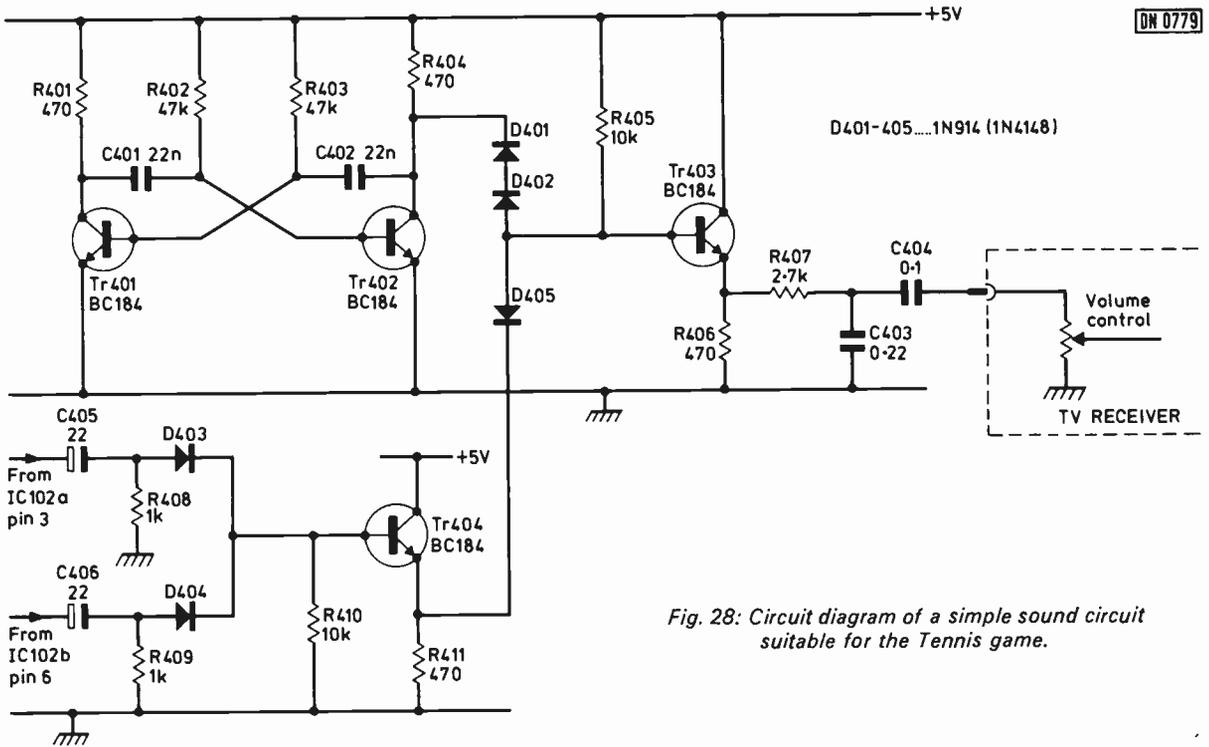
Fig. 28: Circuit diagram of a simple sound circuit suitable for the Tennis game.
