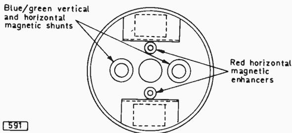
Fig. 2: Front view of the in-line electron gun assembly used in the Mitsubishi Diatron SSS range of tubes. The magnetic shunts reduce the rasters produced by the two outer beams while the enhancers increase the width of the raster produced by the centre beam.
