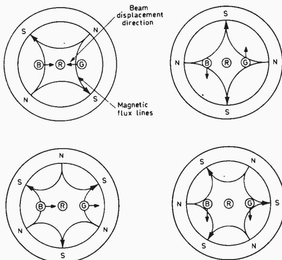
Fig. 3: Arrangement of magnets used to obtain static beam convergence—showing the beam displacements produced by the four- and six-pole fields.
