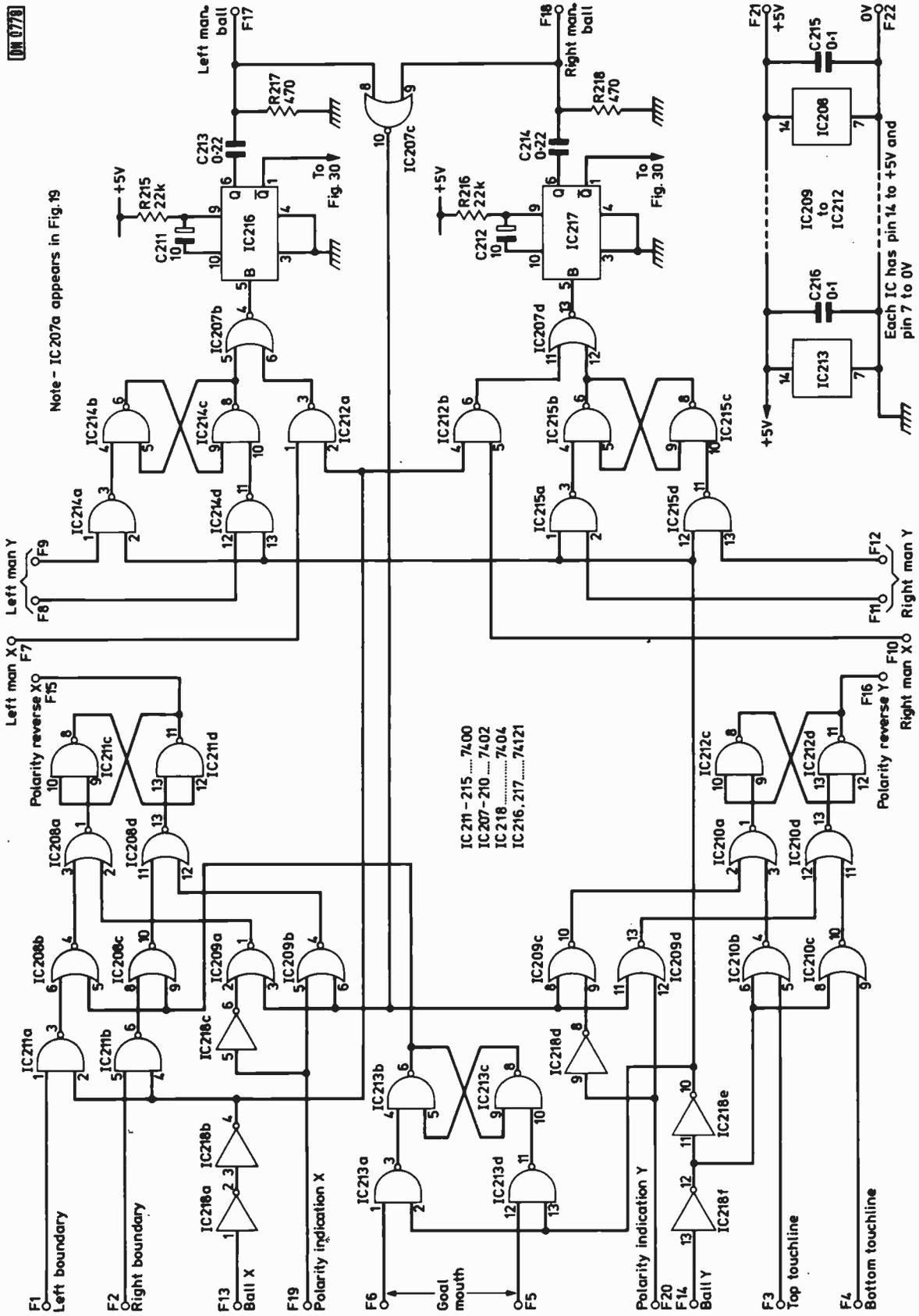
Fig. 27: Circuit diagram of the ball control logic for the Football game. This forms part of Board F, shown in Fig. 20.
