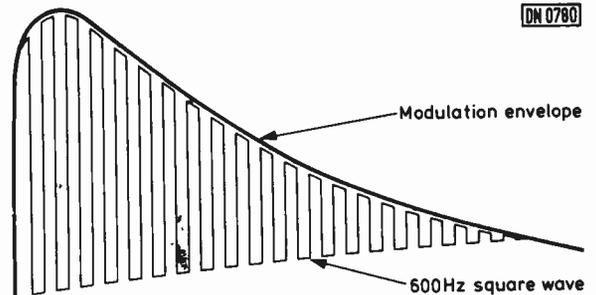
Fig. 29: Typical waveform of the sound circuit output.
