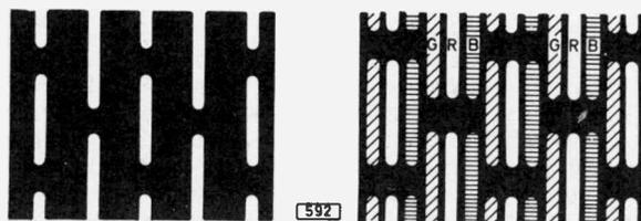
Fig. 1: Arrangement of the slits in the shadowmask (left); impression of a close-up view of the screen (right).
