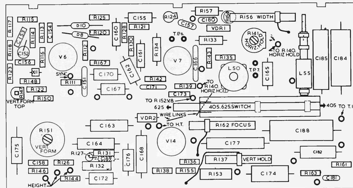
Fig. 1: Layout of the timebase printed panel, viewed from the component side.
