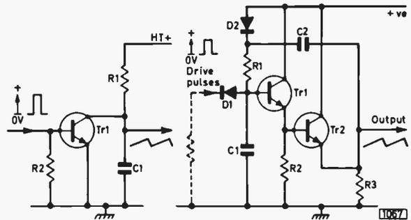
Fig. 6 (left): Driven sawtooth generator using an npn bipolar transistor as the switch.
