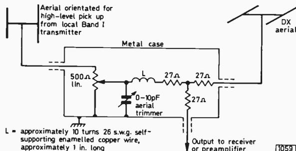
Fig. 1: Anti-phasing unit for reducing Ch. B2 interference.
