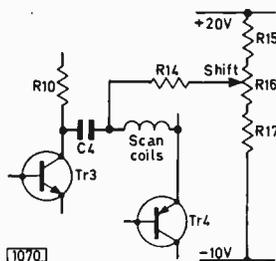
Fig. 9 (above): Practical field scan circuit.
