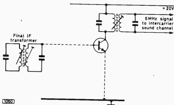
Fig. 1: Using all the components listed alongside, complete this circuit to produce a single-standard monochrome receiver detector and emitter-follower stage.
