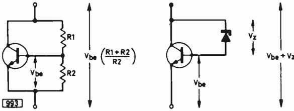
Fig. 1 (left): The  $V_{be}$  multiplier.
