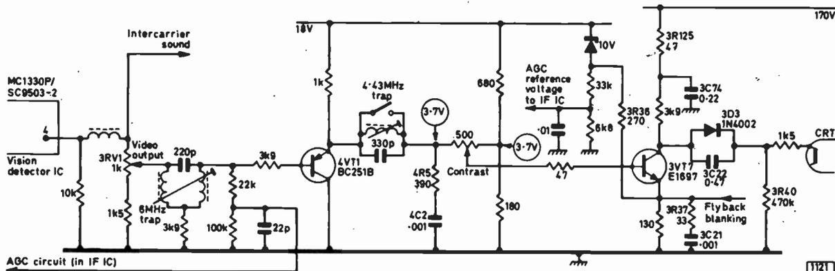
Fig. 5: Video channel used in the RRI A816 chassis, with diode beam limiter 3D3. 3RV1 sets the threshold for the a.g.c. circuit which is in the i.f. i.c. (MC1352P/SC9504P).
