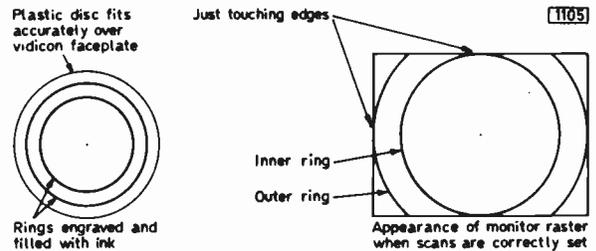
Fig. 5: Setting the scans with an engraved disc.
