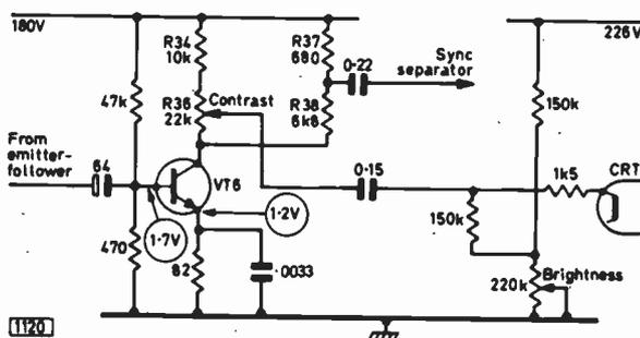
Fig. 4: Video output stage used in the Thorn 1580 chassis. Contrast is controlled by tapping the required degree of c.r.t. drive from the output transistor's collector load circuit.
