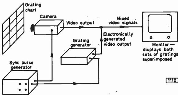
Fig. 10 (above): Setting the camera linearity.
