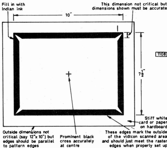
Fig. 8: Scan setting test chart.
