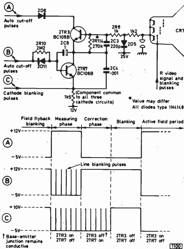
Fig. 1: Automatic grey-scale correction circuit used in the latest Bang and Olufsen colour chassis (red cathode circuit only shown), with associated waveforms beneath. During the measuring phase the cathode current is measured; during the following correction phase a clamping action sets the charge on 2C8. In this way the circuit automatically sets the cathode voltage at the start of each field period.
