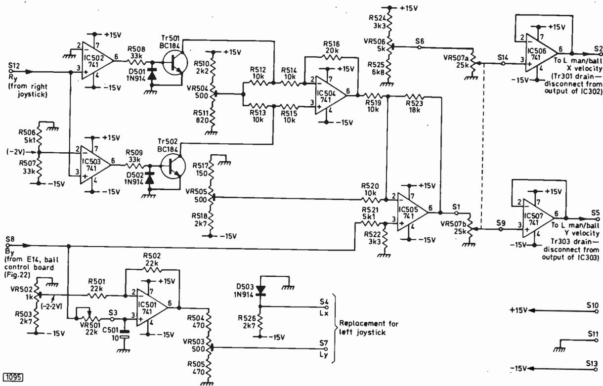
Fig. 33. Circuit for Superman, intended as a plug-in replacement for the left joystick. VR501 and VR507 are front-panel controls for setting the speed of response and kick respectively.
