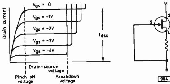
Fig. 3 (left):  $I_d/V_{ds}$  characteristics of an  $n$ -channel junction field effect transistor.
