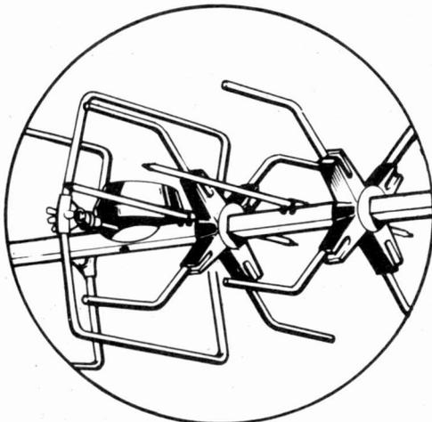
Fig. 1: Close-up showing position of the 'launch directors'.
