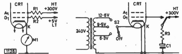
Fig. 1 (left): Basic circuit for emission measurement.
