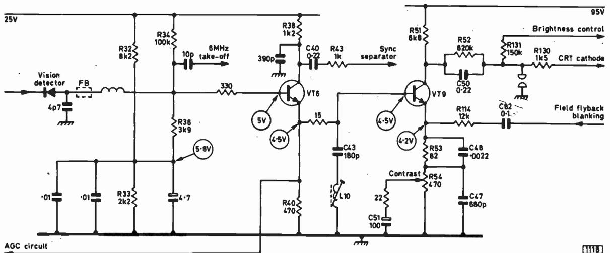
Fig. 2: D.C. coupled video circuit used in the Thorn 1590 chassis. VT6 acts as a sync preamplifier as well as a video buffer/driver stage. The 1591 chassis is the same except for R131 which is 100k $\Omega$ .
