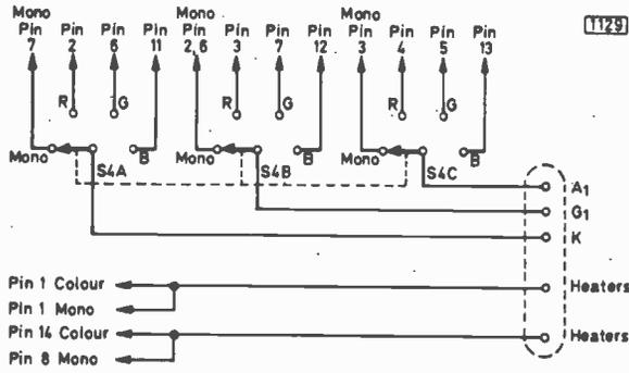
Fig. 5: Switch wiring for the tube base socket assembly.
