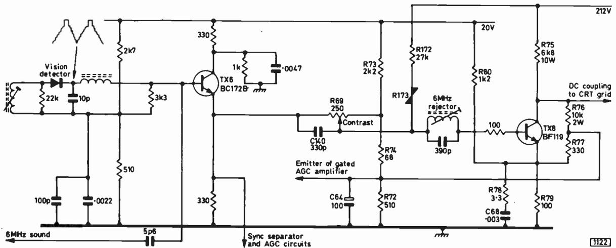
Fig. 6: D.C. coupled video channel used in the ITT VC200 chassis. The output is applied to the c.r.t. grid.
