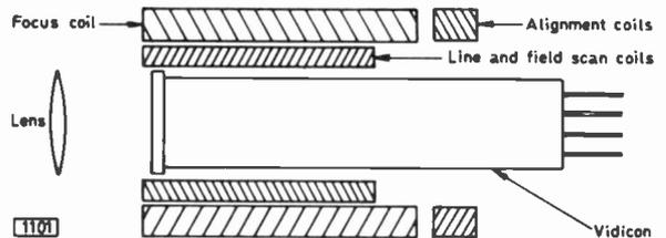
Fig. 1 (above): Cross-section through the vidicon and its associated coils.
