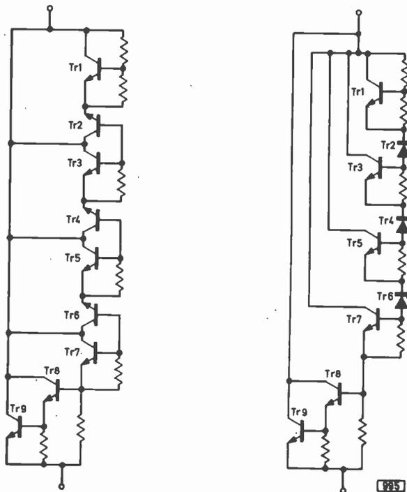
Fig. 5 (left): 35V i.c. stabiliser—internal circuit. Types TAA550 and TBA271.
