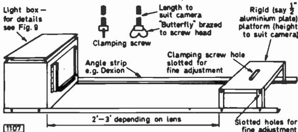
Fig. 7: Camera setting-up jig.
