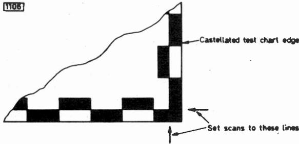
Fig. 6: Scan setting using a commercial test chart.
