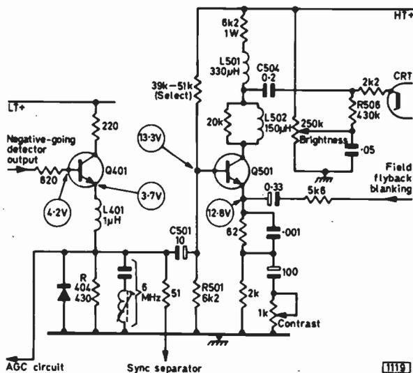
Fig. 3: A.C. coupled circuit used in the Sony Model TV110UK. With a.c. coupling the c.r.t. and the video output transistor can be biased to a midpoint.
