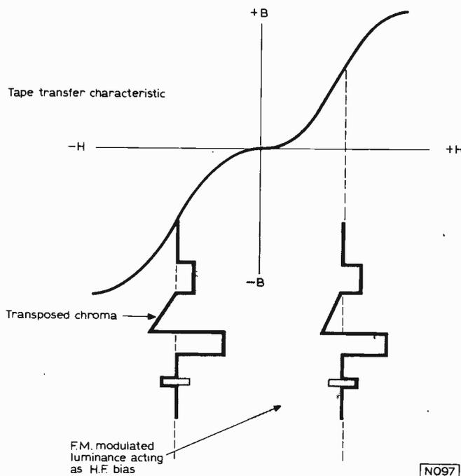
Fig. 8: The f.m. luminance signal acts as h.f. bias for the lower frequency chromance signal on recording.
