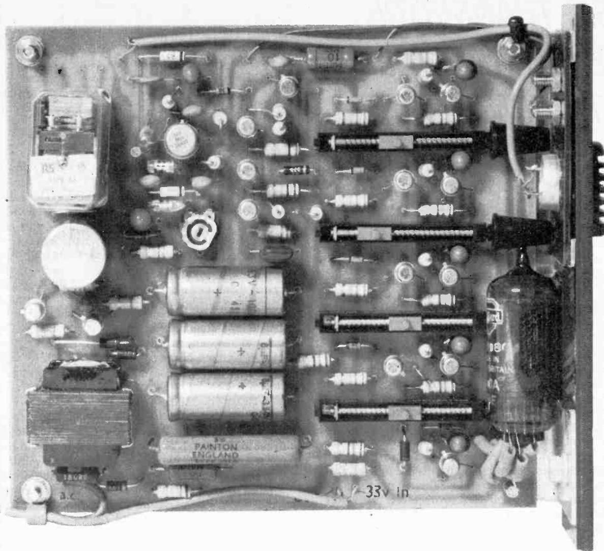
with an oscilloscope on pin 1 of the i.c. About 3V p-p should be obtained with both transducers almost touching, reducing to a few millivolts at normal distance. If an oscilloscope is not available, D5 can be temporarily disconnected and the voltage across C19 monitored with a d.c. voltmeter. Normally VR5 on the receiver will be in the maximum gain position (fully clockwise), but it has been included in case any problem is experienced with interference from any source.
