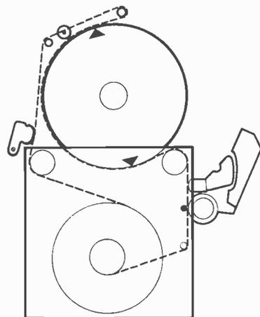
Fig. 4: Tape path with the machine turned on. A loop of tape has been drawn out of the cassette by the tape guide arms and wrapped around the video head drum.
