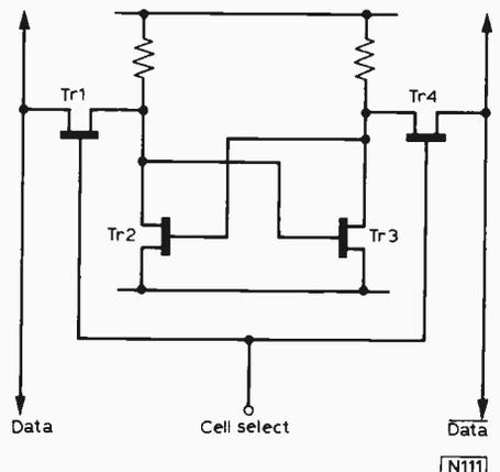
Fig. 23: A typical static memory cell.
