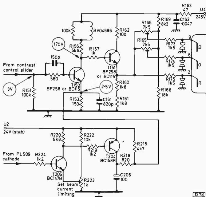
Fig. 3: The luminance output stage and beam limiter circuits. In later versions R165, R166, R168 and R169 are omitted and an AA117 diode is added between the base and emitter of T150, cathode to base; also C206 is changed to 220µF and a 100Ω resistor (R217) is added between the collector of T204 and the junction of C206/R218.
