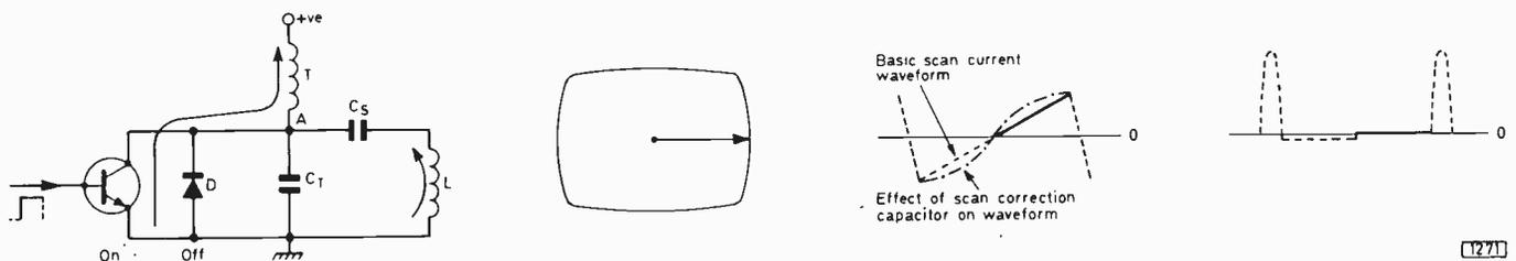
Fig. 5: Conditions during the latter part of the forward scan – completion of beam deflection to the right-hand side of the screen.
