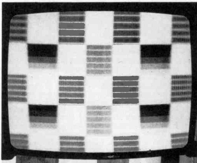
Checkerboard test pattern used by RTVE, RTP, Rhodesia and others. This photo was taken by Doug McFadyen (New Zealand) from a local transmission.
