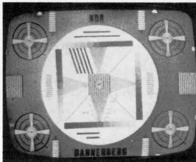
The Telefunken T05 test card, transmitted by Dannenberg NDR-1.
