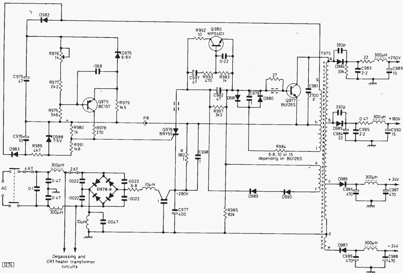
Fig. 3: Blocking oscillator switch-mode power supply circuit used in Tandberg 110° colour sets. Warning to Australian readers: a very similar circuit is used in the EMI (Australia) C211 110° colour chassis!
