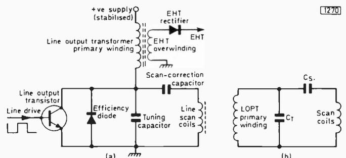
Fig. 1: (a) Basic elements of a transistor line output stage. (b) Equivalent parallel tuned circuit during the flyback period when the transistor and efficiency diode are non-conducting.
