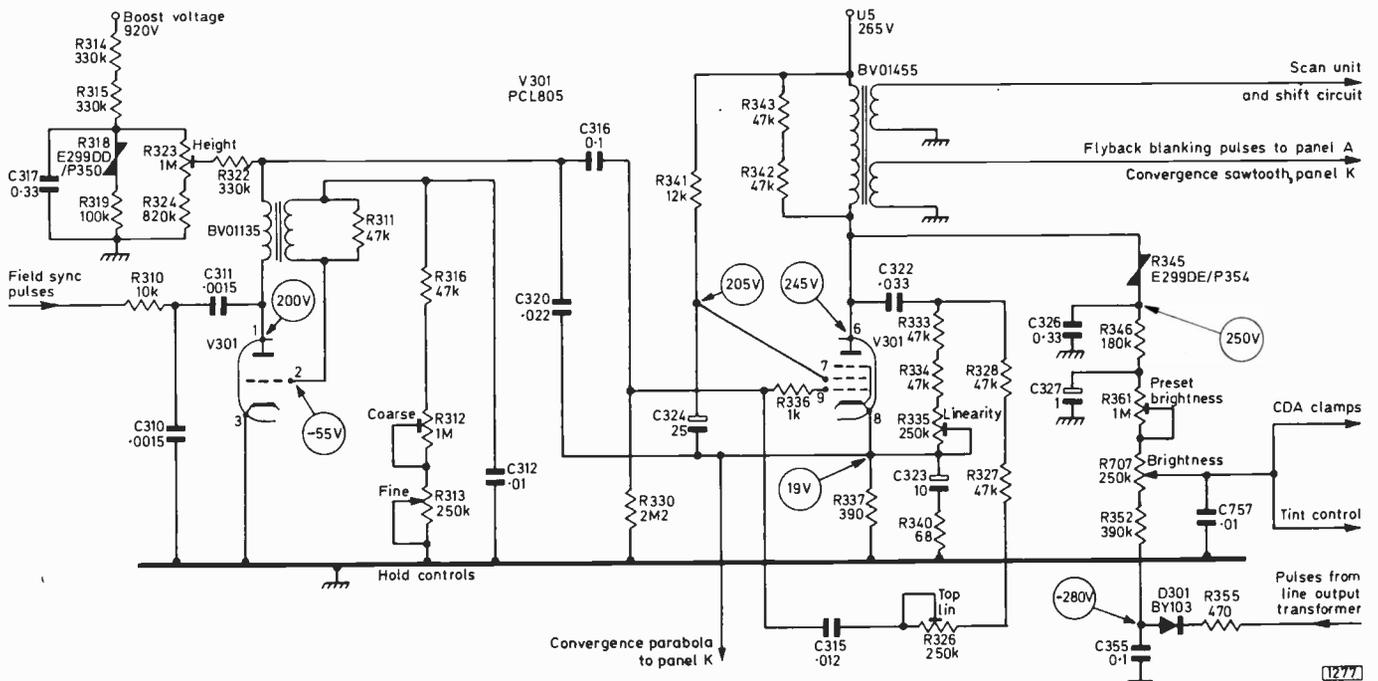
Fig. 2: Field timebase and brightness control circuits. In later production R324 is omitted and the blocking oscillator timing capacitor C312 is changed to 0.015μF.
