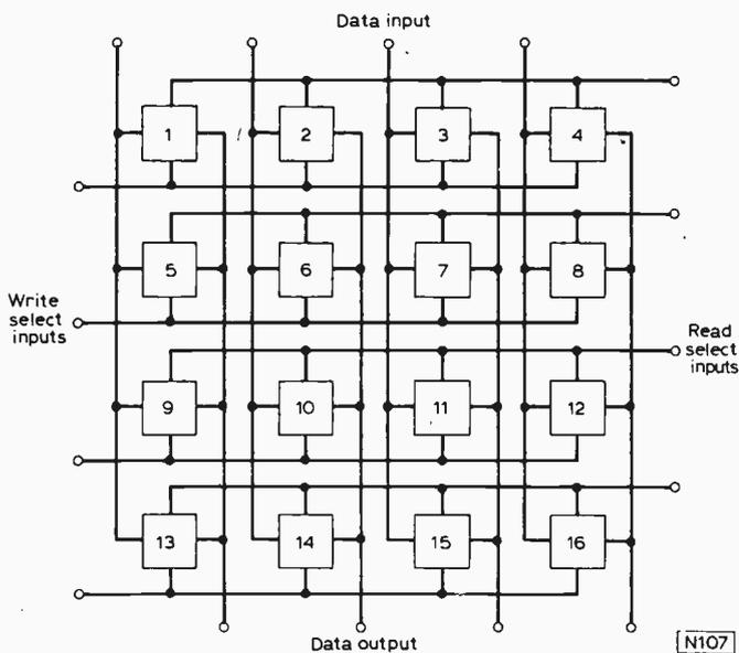
Fig. 19: Connection arrangements for a 16-bit memory array.
