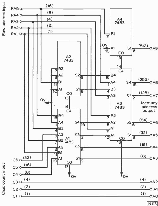
Fig. 25: An address generator circuit.
