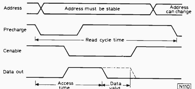
Fig. 22: Timing sequence for the Read cycle of the 1103 memory.
