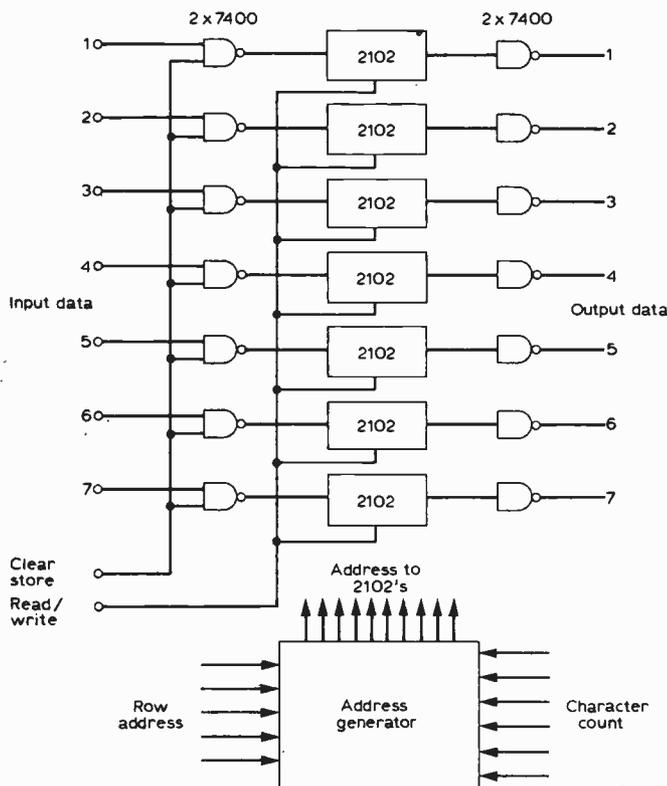
Fig. 24: Block diagram of a Page memory using Intel 2102 RAMs.
