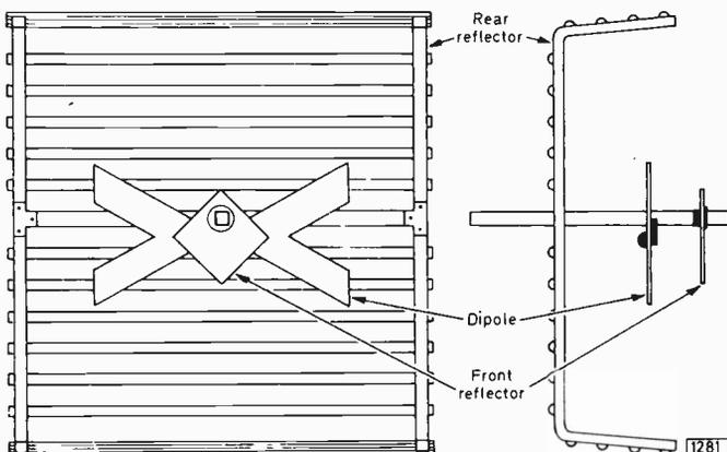
Fig. 1: Front (left) and side views of the Telerection backfire aerial. An add-on director chain is also available.
