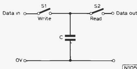
Fig. 17: A capacitor memory cell.
