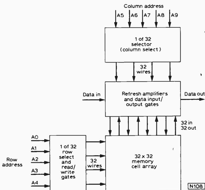
Fig. 20: Overall block diagram of a complete memory i.c.
