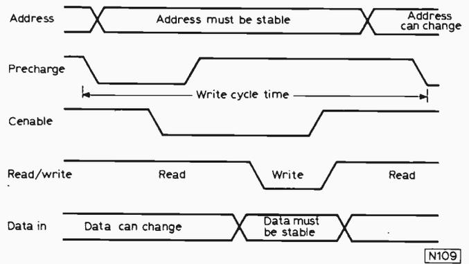
Fig. 21: Timing sequence for the Write cycle of the 1103 memory.
