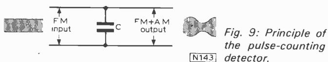
Fig. 9: Principle of the pulse-counting detector.
