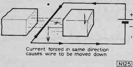
Fig. 5: Relationship between generator and motor effects.
