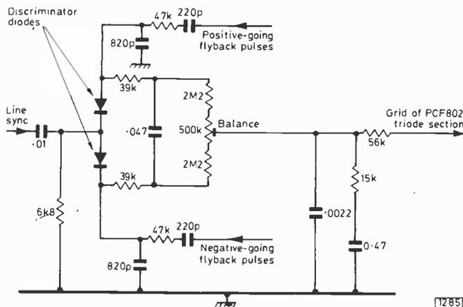
Fig. 1: Flywheel sync circuit used in the Grundig Models R500E/GB, T2002E/GB and P2002E/GB.
