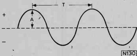
Fig. 10: Defining Peak Amplitude and Periodic Time or Period of a sinewave.
