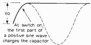
With no load, the capacitor charges up through the rectifier to the peak voltage  $V_o$
