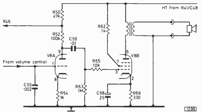
Fig. 2: Audio circuit used in Models DR20/21/23/24.
