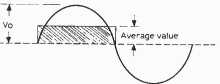
If the rectangle (shaded) has the same area as the half sine wave, then the height of the rectangle is the average value of voltage of the sine wave.
