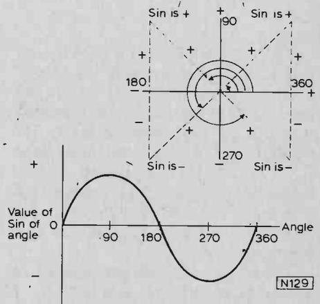
Fig. 9: Plotting the value of  $\sin \theta$  for angles up to  $360^\circ$ .
