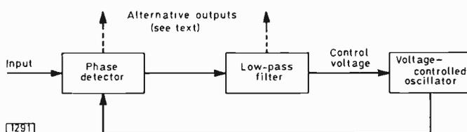
Fig. 3: Detection by means of a phase-locked loop.
