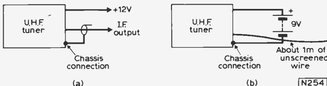
Fig. 1: (a) Transistor u.h.f. tuner connections “as supplied”. (b) Connections required for testing and realignment.
