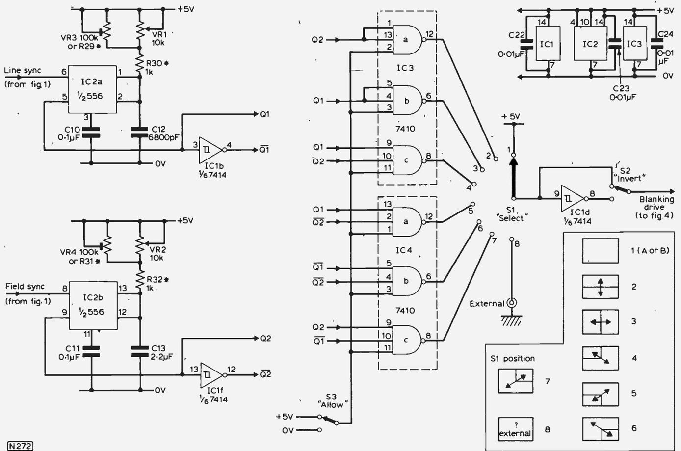
Fig. 2: The timing logic, which generates blanking pulses to drive the video switching circuits of Fig. 4.
