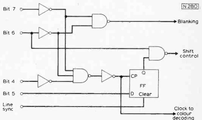
Fig. 57: Shift logic for use with the revised symbol code.
