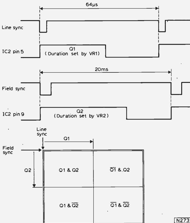
Fig. 3: Waveforms and corresponding screen areas for the timing logic circuit.
