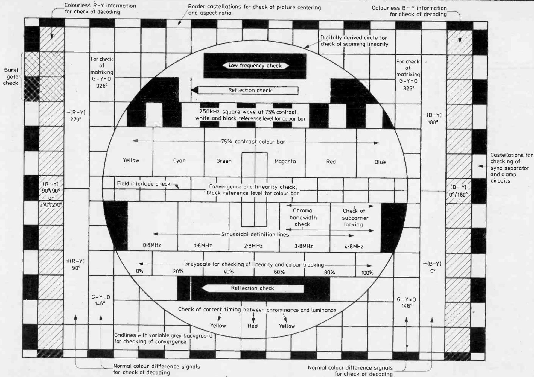
Fig. 1: The basic PM5544 test card, with features identified.
