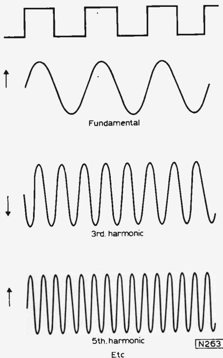
Fig. 2: Analysing a squarewave into a fundamental plus odd harmonics.
