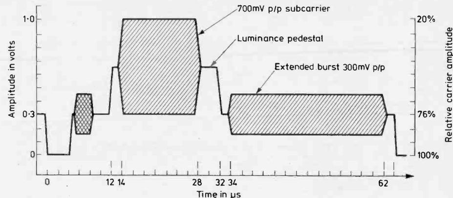
Fig. 6: The signal on line 20, containing only two chroma tests.
