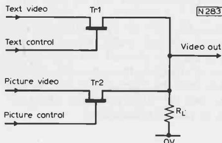
Fig. 60: A video switch using two f.e.t.s.
