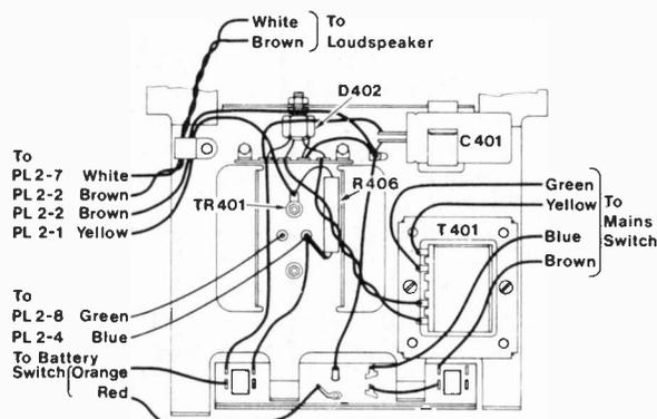
Fig. 1: Layout and wiring of the power unit.
