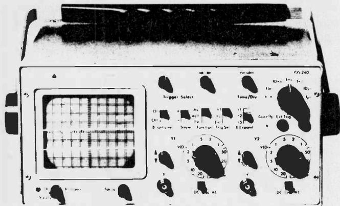
The OS240 is a 10MHz, dual-trace instrument. The smallish 4 in. c.r.t. has been given 10 x 8 graticule divisions by reducing the usual 1cm divisions to 0.8cm. This is just acceptable for fine measurement, provided the brightness is kept within bounds to maintain good focus. A useful X-Y facility is provided, with the Y1 amplifier feeding the X deflection system when X-Y is selected. Provision for Z-modulation is also made via a rear socket.
