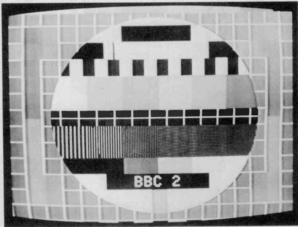
*An off-air photograph of Test Card G. The vertical stripe pattern of the Sony Trinitron tube is clearly visible.*
