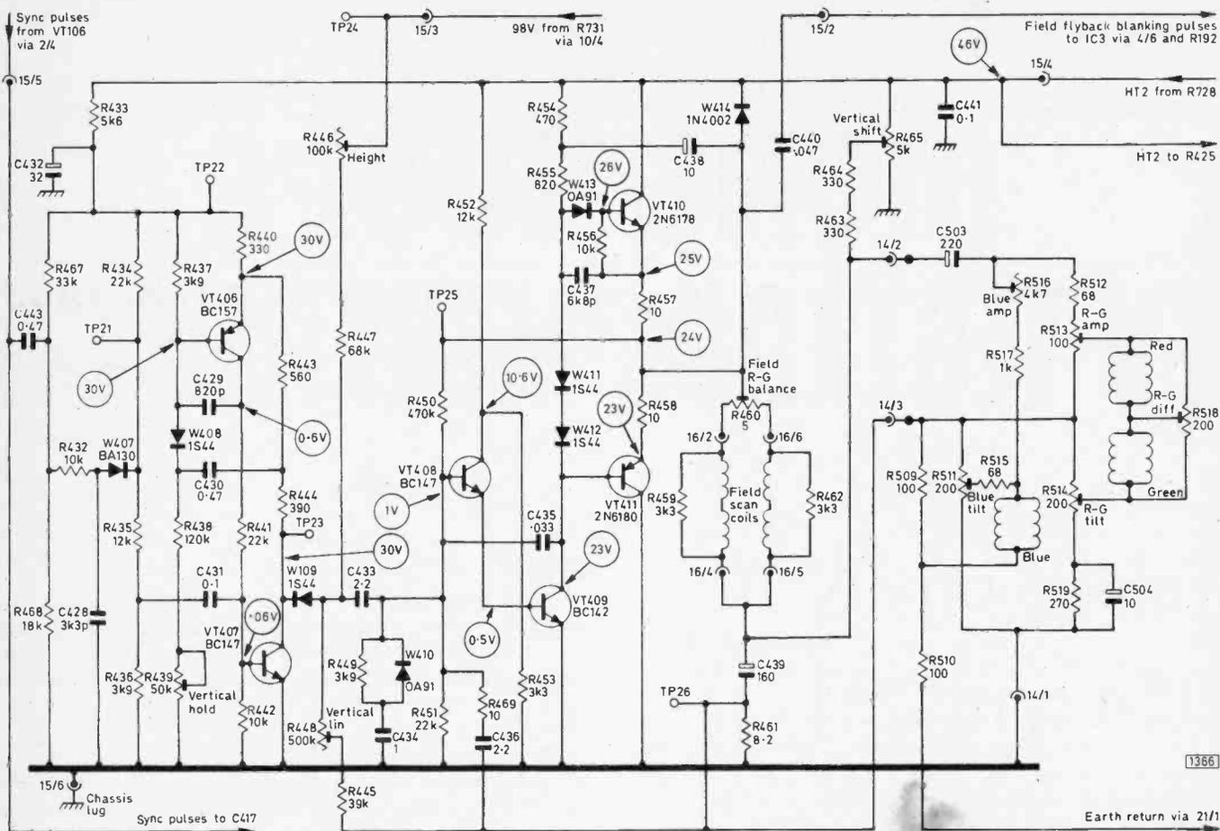
Fig. 1: Field timebase and vertical convergence circuits. C503 is 150µF on the 8000/8000A chassis. C504/R519 were added and W502 (in parallel with R512 and R513) deleted in later production to give improved convergence.
