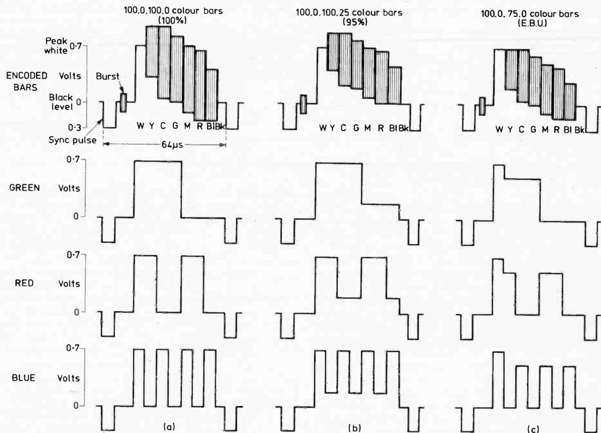
Fig. 3: The three common sets of colour bars:
