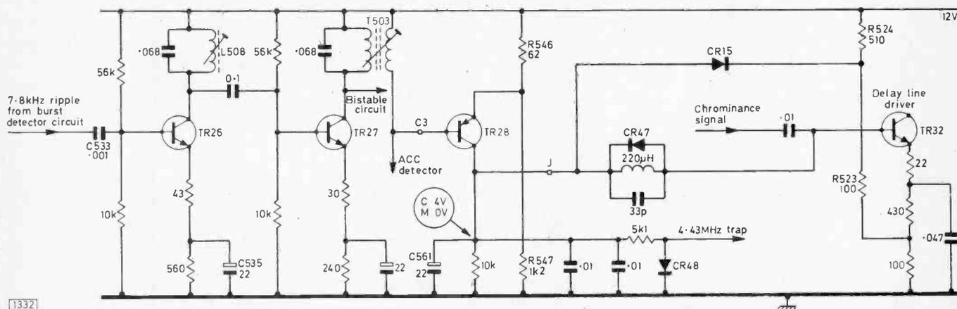
Fig. 1: Ident amplifiers (TR26, TR27) and colour-killer (TR28) stage, Hitachi Model CNP190.
