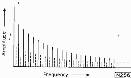
Fig. 5: Fitting another spectrum of signals in. (Frequency interleaving.)
