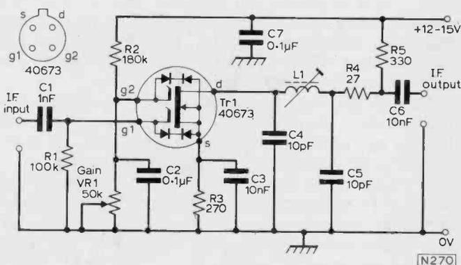
Fig. 1: Circuit diagram of the preamplifier. Although protection diodes are incorporated in the 40673, the usual precautions against build-up of static charge should be taken when handling and installing the device.
