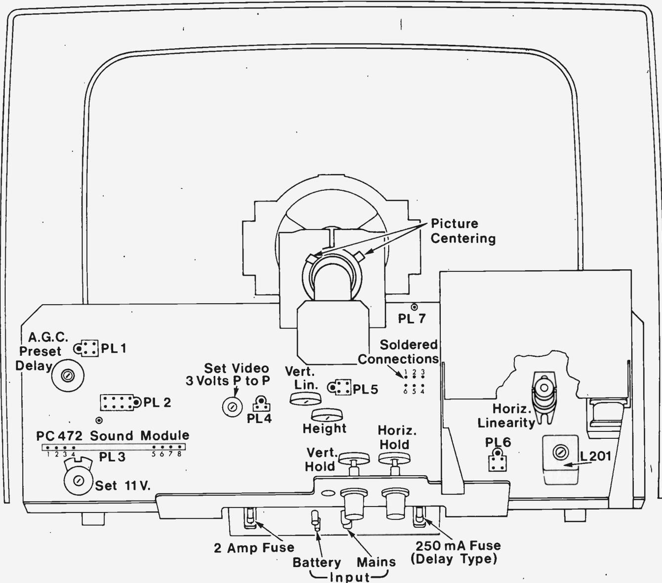
Fig. 3: Rear view of the receiver, with the cabinet back removed.
