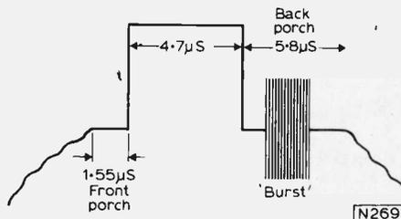
Fig. 8: Timing of the colour sync signal. The "burst" consists of 10 cycles ( $\pm 1$  cycle) of the colour subcarrier.
