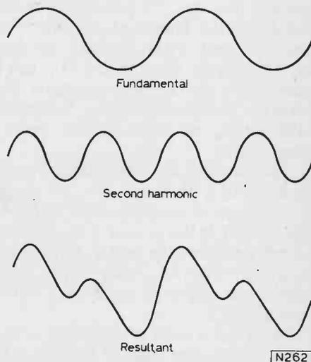
Fig. 1: Result of mixing a fundamental and second harmonic, in phase.
