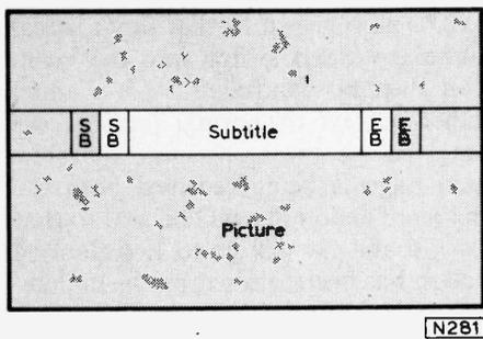
Fig. 58: Arrangement of a subtitle display, showing position of SB (Start Box) and EB (End Box) commands.
