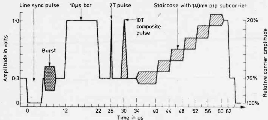
Fig. 5: The signal on line 19, which contains the most tests.
