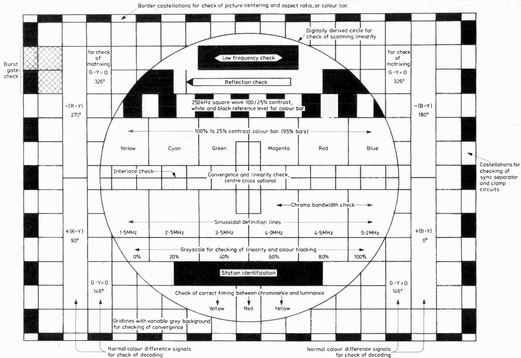
Fig. 2: The modified PM5544 - Test Card G - used by the BBC, with features identified.
