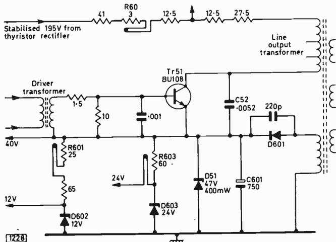
Fig. 8: Line output stage used in the GEC C2110 series.
