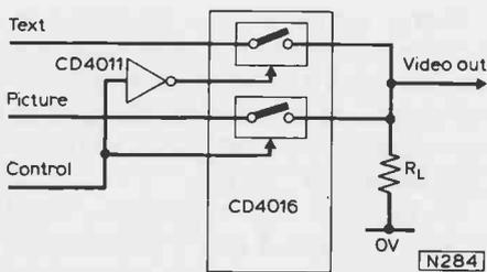
Fig. 61: A video switch using the CD4016 CMOS integrated circuit.
