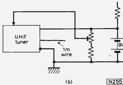
Fig. 2: Tuner with power supply components allowing operation from "valve" h.t. rails. (a) As supplied. (b) Modified ready for testing and realignment.
