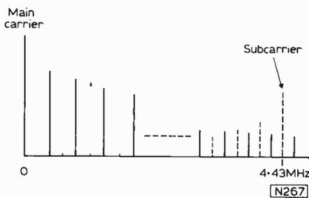
Fig. 6: Colour subcarrier and its spectrum fitted into the main carrier spectrum.
