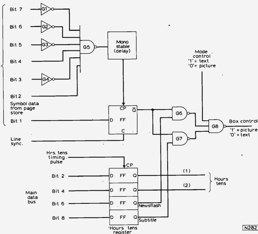
Fig. 59: Box control logic circuitry.
