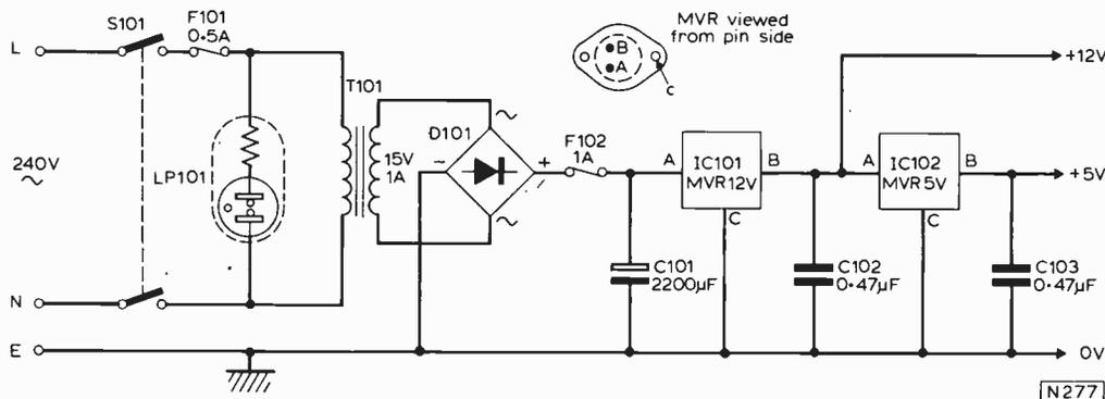
Fig. 6: Circuit diagram of the fader unit, which is electrically separate from the video mixer.
