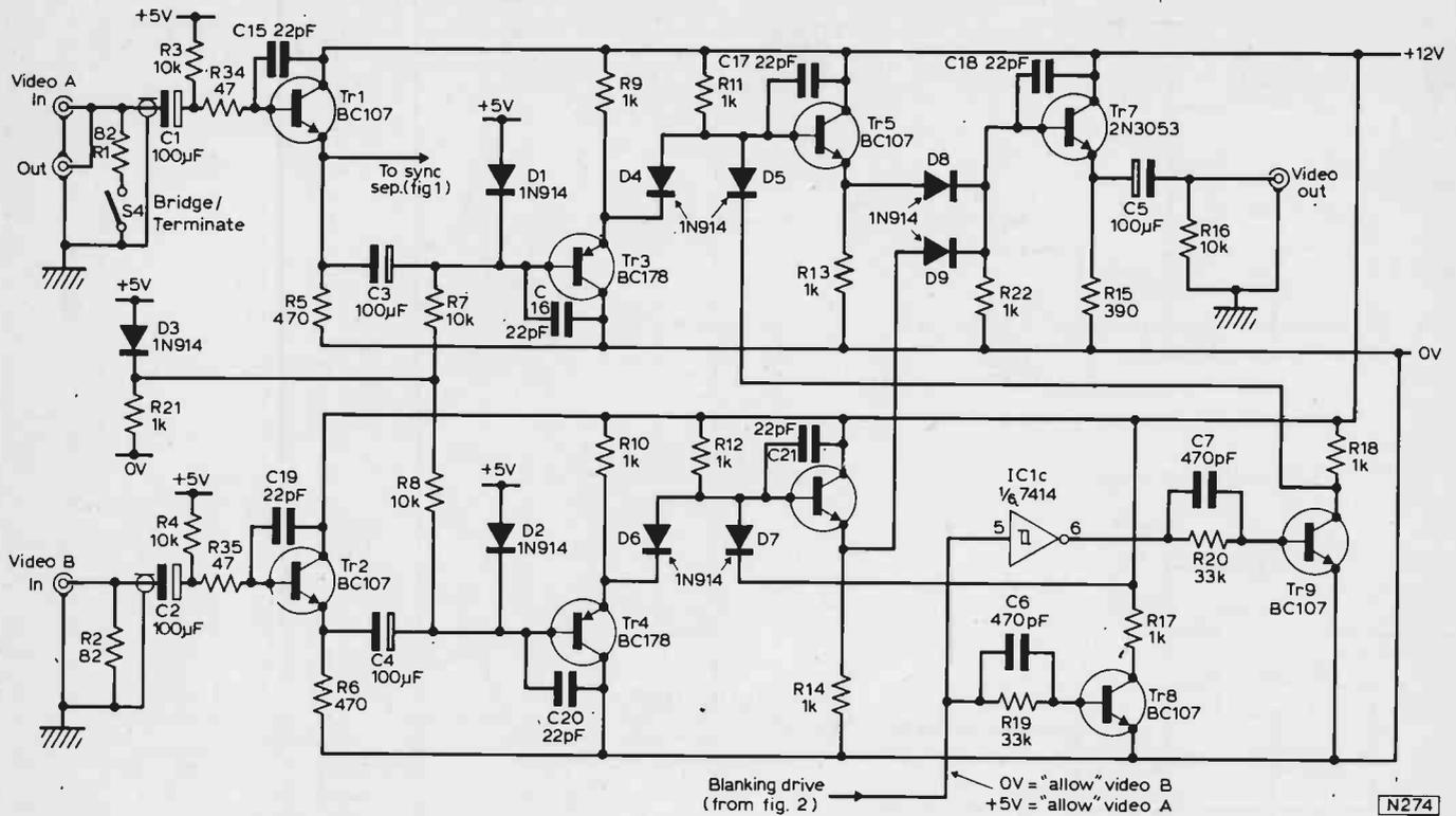
Fig. 4: Circuit of the video mixer, producing an output which is switched between Video A and B, controlled by the timing logic. Note that the feed to D7 cathode should be taken from the collector of Tr8, i.e. the opposite end of R17 to that shown in the drawing.
