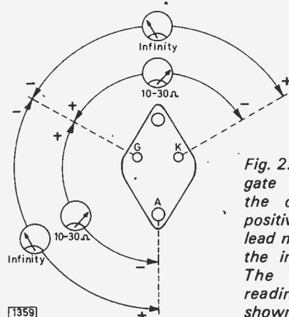
Fig. 2: Ohmmeter checks on a gate controlled switch. Use the ohms  $\times 1$  scale. The positive and negative meter lead markings shown indicate the internal battery polarity. The GCS is defective if readings other than those shown are obtained.
