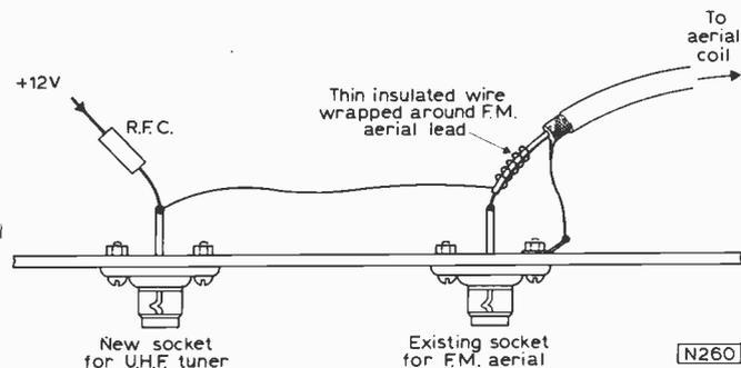
Fig. 7: Coupling the u.h.f. tuner output to the f.m. receiver aerial input circuit.
