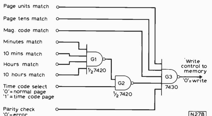
Fig. 55: Decoding logic for time coded type C pages.
