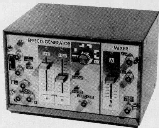
THIS unit is designed for use with two CCTV cameras and provides the following effects:
