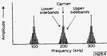
Fig. 3: Spectrum of transmissions with carriers every 100kHz, modulated by frequencies up to a few kilohertz.
