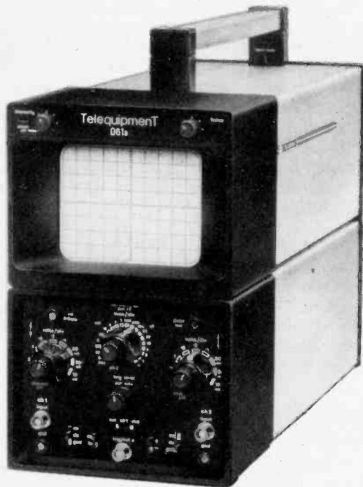
*Editorial Note – The D61 has just been replaced by the D61a (pictured here) in a restyled, more robust case. Technical specifications remain the same, apart from the incorporation of enhanced triggering capabilities and a multi-range power transformer. The price is £155 plus VAT.*
