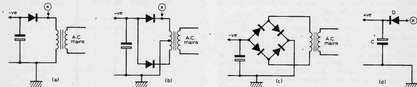
Fig. 5: Three possible basic power supply arrangements for an f.m. receiver with a negative supply rail - (a) half-wave; (b) full-wave; (c) full-wave bridge; (d) Circuit for deriving power for the u.h.f. tuner from the arrangements (a) or (b).
