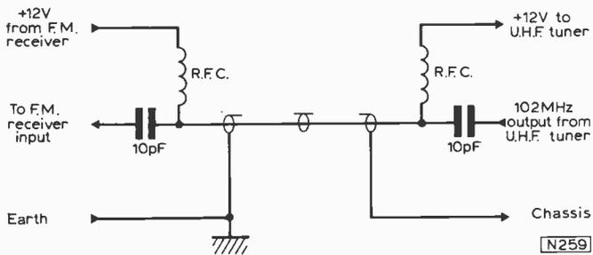
Fig. 6: Circuit arrangement for running power to the u.h.f. tuner via the signal coaxial cable.
