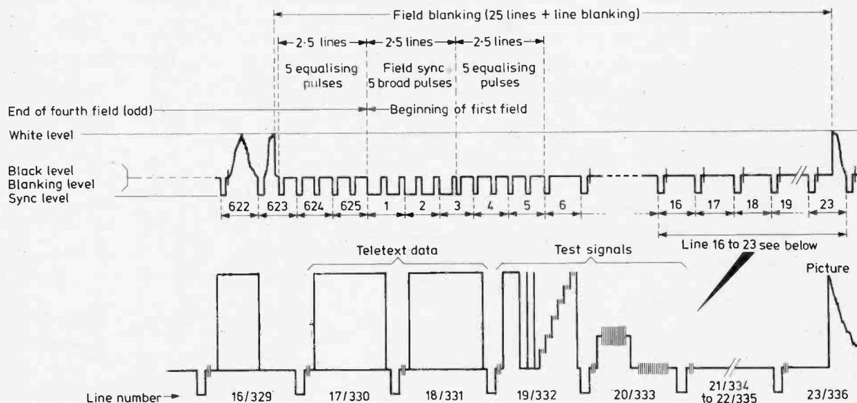
Fig. 4: The field blanking interval, reproduced from the joint BBC/IBA specification. The inset shows in detail the lines used for v.i.t.s. Note that the line count starts from the leading edge of the field sync pulse proper.
