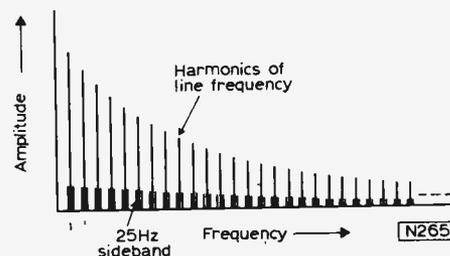
Fig. 4: Spectrum of line-frequency harmonics, each with 25Hz sidebands.
