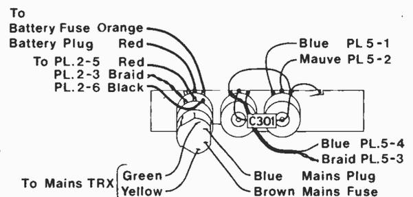
Fig. 2: Connections to the control panel.
