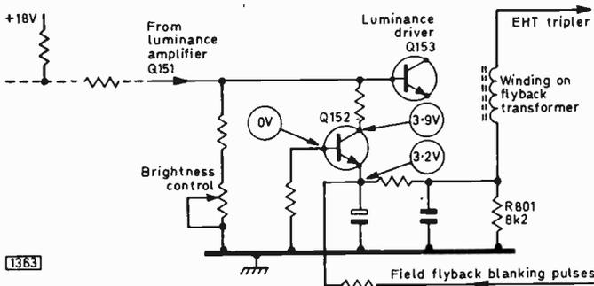
Fig. 7: Simplified circuit of the beam limiter arrangement used in the Sony colour portable Model KV1300UB. Field flyback blanking is also carried out at this point.
