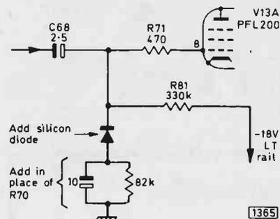
Fig. 1: D.C. restorer circuit suggested by W. R. Hill for use with the Pye group's 368 chassis. This was the final dual-standard monochrome chassis produced by the group.
