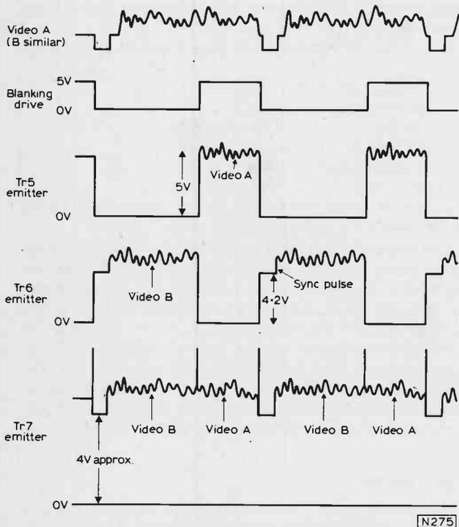
Fig. 5: Typical waveforms for the video mixer circuit.
