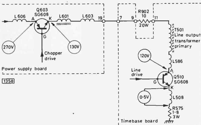
Fig. 1: Path of the 130V line from the power supply regulator GCS Q603 to the line output GCS Q510, Sony Model KV1810UK. Various other feeds are taken off en route.
