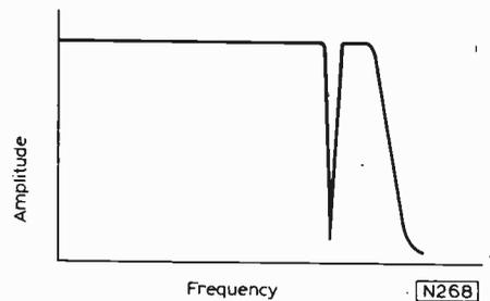
Fig. 7: Response of a receiver video amplifier with 4.43MHz notch filter.
