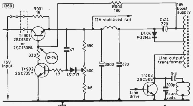
Fig. 3: Basic power supply regulator and line output stage circuitry used in the Elizabethan Model T12. Since the collector of the error sensing transistor Tr902 is fed from the boost rail, via R903, a defunct line output stage will result in the series regulator transistor Tr901 being cut off and the maximum voltage drop being developed across its shunt resistor R901.
