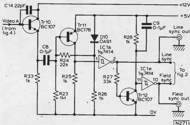
Fig. 1: The sync separator circuit, providing line and field rate pulse trains for internal and external use.
