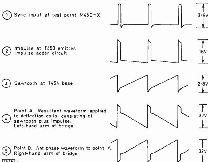
Fig. 2: Field timebase waveforms. The antiphase outputs from the bridge output stage are shown at (4) and (5).
