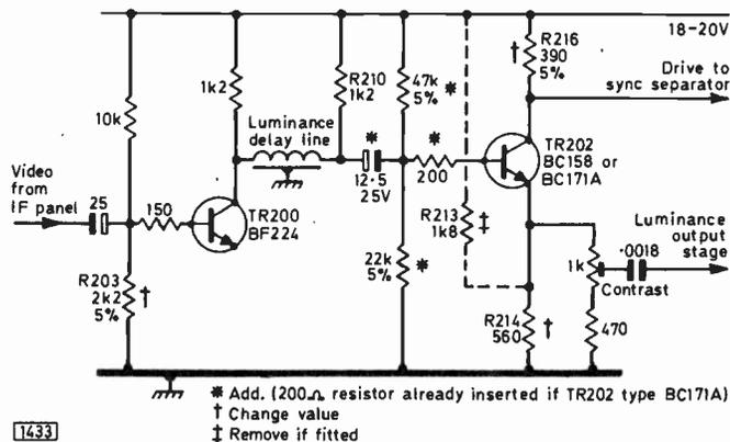
Fig. 4: Modifications in the luminance channel of the Decca CTV25 and related models to deal with field jitter. Applies to models using the following luminance or combined decoder/luminance panels: 550862, 550928 and 550982.
