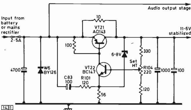
Fig. 2: L.T. stabiliser circuit used in the Thorn 1590, 1591 and 1593 chassis. W6 provides protection against reverse battery connection. C83/R101 provide hum cancellation.
