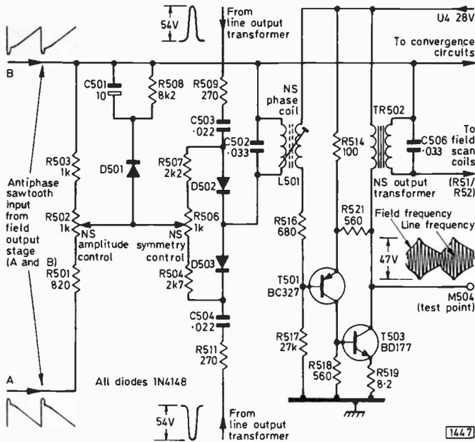
Fig. 3: The north/south raster correction circuit. The diode modulator consists of D502 and D503. The field sawtooth waveforms are modulated at line frequency, the resultant output being applied to the field scan coils. T501 and T503 are the driver and output transistors. A common failure is T503 going short-circuit base to emitter and burning out the emitter resistor R519.
