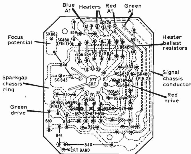
Fig. 2. A typical tube base layout. Ensure that the sparkgaps are uncarbonised. On this layout (Pye 731 chassis) a separate chassis ring is provided for the sparkgaps.
