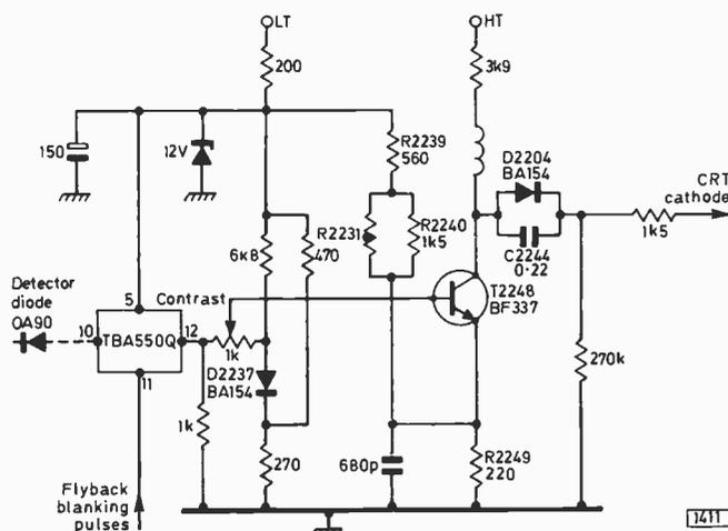
Fig. 1: Circuit of the video channel in the Philips 320 monochrome chassis. A faulty TBA550Q i.c. caused excessive brightness with hardly any picture shortly after switch on.
