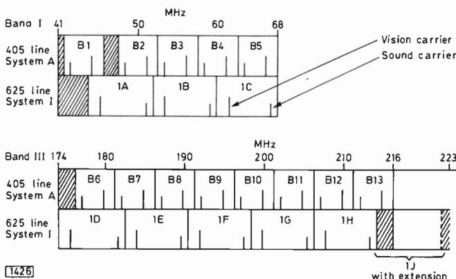
Fig. 1: BBC proposals to the Annan committee for 625-line Band I/III channel allocations. The diagram shows the existing subdivisions of Bands I and III into 5MHz channels for 405-line television and the proposed subdivision into 8MHz channels for 625-line television. The positions of the sound and vision carriers are also shown.
