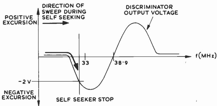
Fig. 2: Response curve of the a.f.c. circuit in the self-seeking tuning system devised by Grundig. The self-seeking action stops as soon as the discriminator voltage sinks to  $-2V$ .
