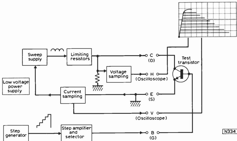
Fig. 1: Simplified block diagram of the Heathkit IT-1121 Semiconductor Curve Tracer. For a pnp transistor, all test signal polarities are reversed, and the display origin moves to the top right-hand corner of the c.r.t.
