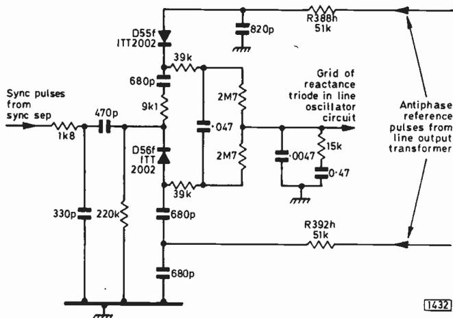
Fig. 3: Flywheel line sync circuit used in the ITT CVC5 and related chassis.
