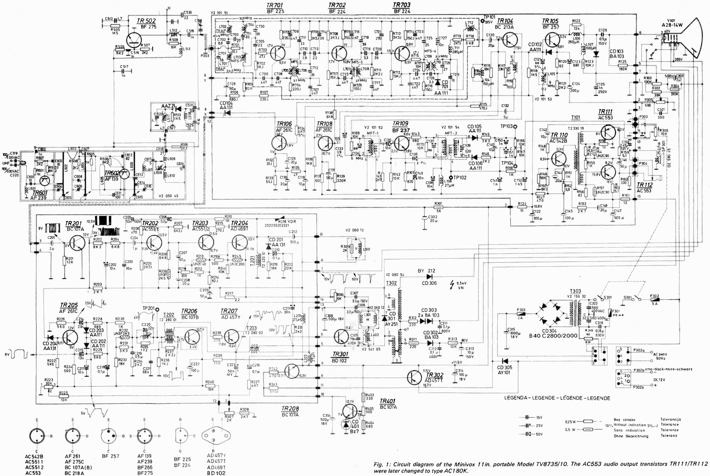
Fig. 1: Circuit diagram of the Minivox 11in. portable Model TV8735/10. The AC553 audio output transistors TR111/TR112 were later changed to type AC180K.
