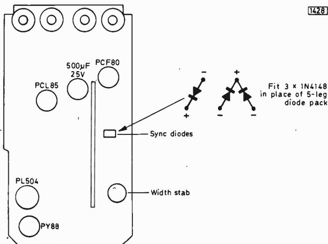
Fig. 1: Rear view of the timebase panel used in the TV141 and later sets.
