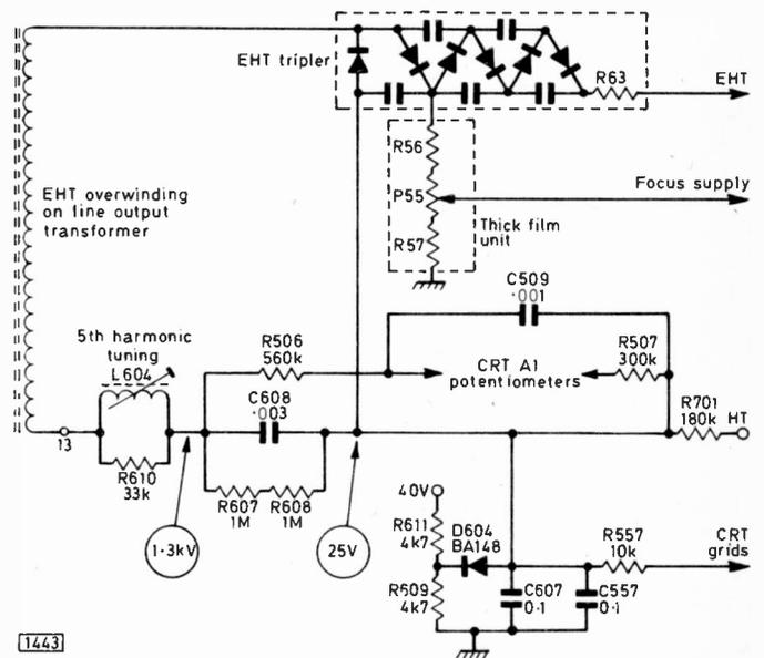
Fig. 3: The e.h.t. and c.r.t. supply circuitry. C608 charges to 1.3kV to provide the first anode supply. D604 monitors the e.h.t. beam current. If the beam current exceeds the bleed current flowing via R609, D604 and R701, D604 will cut off and the voltage at the junction D604/C607 will move negatively, the reduced c.r.t. grid voltage pulling back the beam current. Under normal conditions D604 acts as a clamp diode, clamping the c.r.t. grids at 25V.
