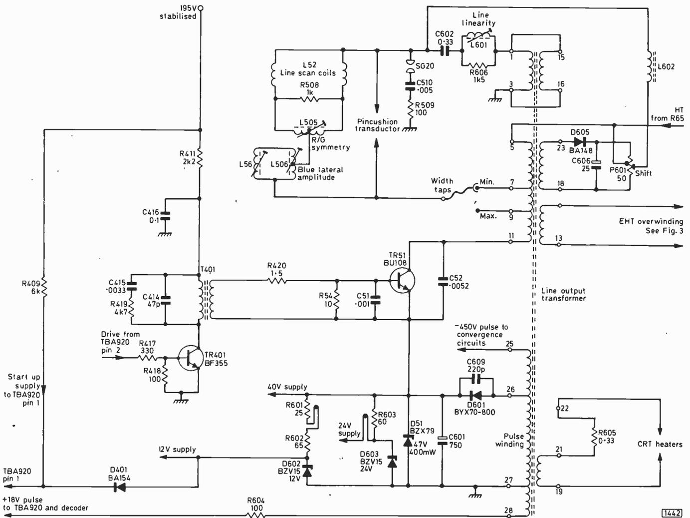
Fig. 2: Circuit of the line output stage. The 47V zener diode D51, a 400mW type, provides circuit protection. Should the 40V line, which is obtained by scan rectification (D601), rise above 47V the zener will go short-circuit, thus removing the l.t. supplies and shutting down the line output stage since there is no line drive.
