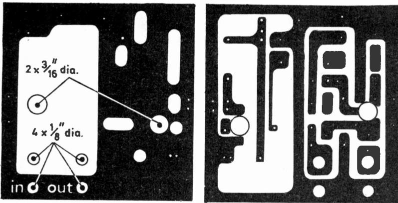
Fig. 2. Printed circuit board details. It is imperative to follow the artwork given very closely, as this will determine the characteristics of the tuning line. For those wishing to buy a ready made board, these are available from Clearline (Bampton), Brook Street, Bampton, Devon, at £1.30 including VAT and postage and packing.
