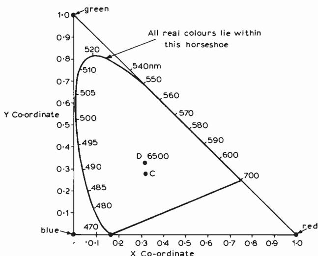
Fig. 3. The C.I.E. chromaticity diagram. The accepted definition of any colour is its X and Y coordinates on this diagram. X relates to the amount of red, Y to the amount of green. Blue (the Z coordinate) is derived from the other two by subtracting their sum from 1 (i.e.  $X + Y + Z = 1$ ). The two common whites, illuminants C and D, are shown in the centre of the diagram.
