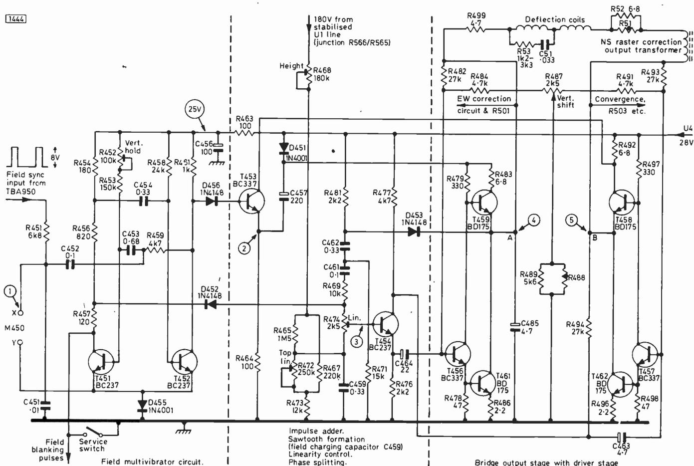
Fig. 1: Complete field timebase circuit. Following the sawtooth waveform charging circuit, the phase-splitter transistor T454 provides antiphase outputs to the driver transistors T456 and T457 which in turn drive, in push-pull, the bridge output transistors T458/T459/T461/T462. To assist with the flyback, a pulse obtained from the collector of T452 is applied via D456 to the impulse adder emitter-follower transistor T453 and is fed via C457 to the output stage.
