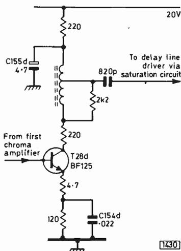
Fig. 1: The second chrominance amplifier stage in the ITT CVC5 and related chassis.
