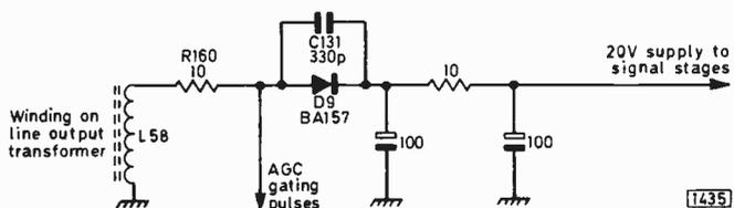
Fig. 6: Method of obtaining an l.t. supply used in the IIT VC200 chassis. D9 rectifies the waveform appearing across L58 during the forward line scan. The negative-going flyback pulses are differentiated, the positive-going spike thus obtained being used to gate the a.g.c. circuit during the sync pulse back porch period.
