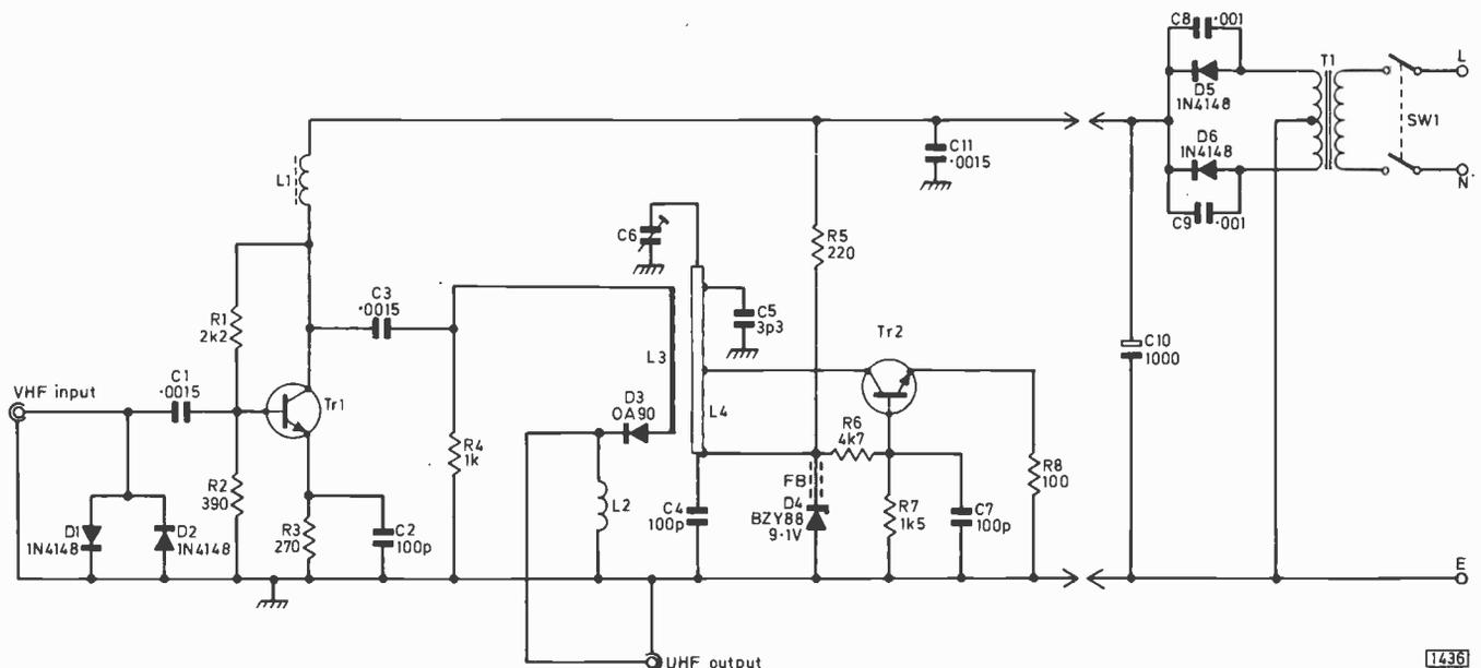
Fig. 1. Complete circuit diagram of the unit. The power supply section is not required if the converter is built into a TV set.
