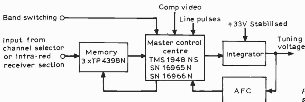
Fig. 1: Block diagram of the Grundig self-seeking tuning system.
