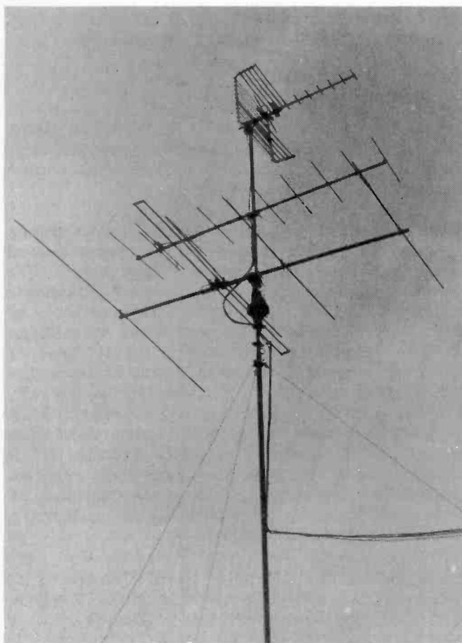
Graham Harrison's aerial mast at St. Leonards. All are wideband arrays: backfire for u.h.f., 10-element for Band III (Telerection), 4-element home constructed unit for Band I.
