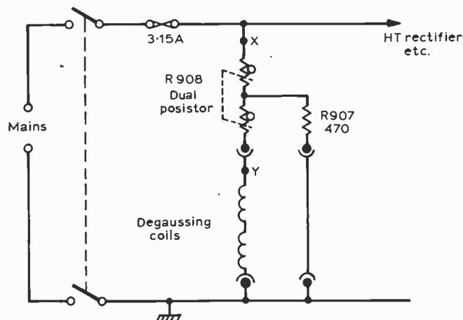
Fig. 1: To check the degaussing circuits, fit a switch at point X (never at Y), display a pure red raster, then impurify it by switching off the bench degausser while held against the tube face. Closing the switch at X will then repurify the displayed raster in a second or two if the circuit is efficient.
