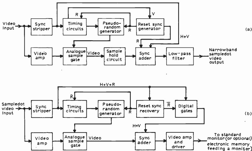
Fig. 3: A simplified block diagram of the Sampledot TV system. (a) Transmitting encoder. (b) Receiving decoder.
