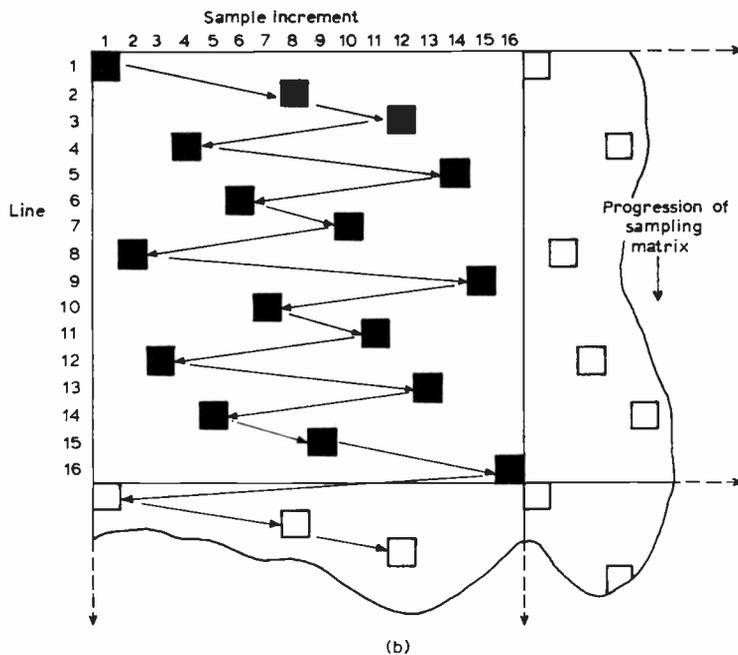
Fig. 2: (a) The Sampledot pseudo-random sampling matrix. (b) An expanded view of segment A, showing a typical pseudo-random sampling code sequence.
