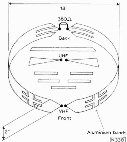
Fig. 2: Basic elements of the aerial system.
