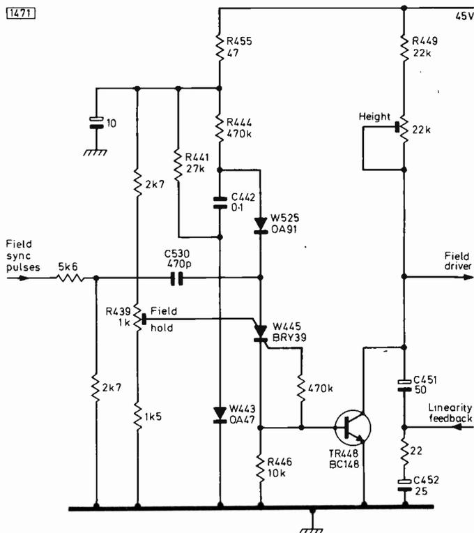
Fig. 6: Silicon controlled switch field oscillator circuit used in the Philips G8 chassis.
