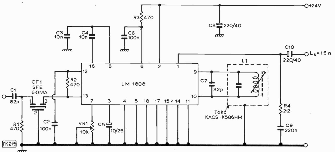
Fig. 1. Circuit diagram of the sound channel unit. See text and Fig. 3 for matching the ceramic filter to the source impedance of the signal input circuit. Since L1 was designed for use at 10.7MHz, C7 is added across it to bring the resonant frequency down to 6MHz.
