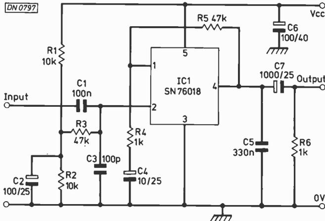
Fig. 6. Circuit diagram of the audio amplifier using the Texas Instruments SN76018 i.c. Changes in the closed loop gain may be made by adjusting the value of R4, see text for calculating the actual value.
