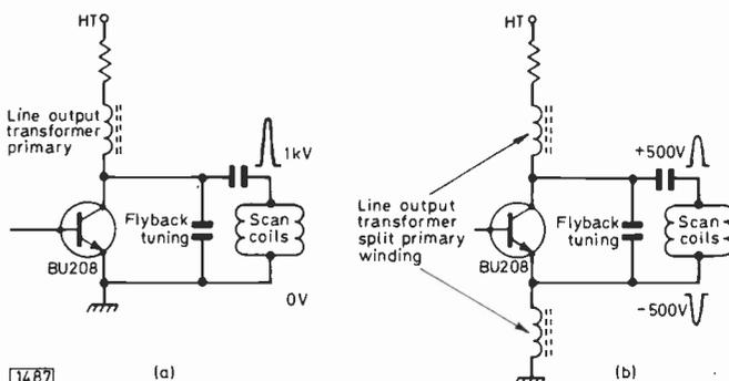
Fig. 1: (a) Conventional unbalanced transistor line output stage configuration. (b) Balanced line output circuit. This arrangement was adopted in the CVC20 chassis to reduce the peak amplitude of the line flyback pulses to a safe level: since the line and field scan coils touch there was the possibility otherwise of arcing.
