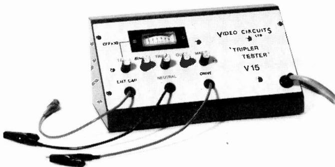
The new tripler tester type V15 from Video Circuits costs £37.40 and can test single-stick rectifiers as well as doublers, triplers and quadruplers with an internally generated 800V pulse. The efficiency is read directly on a meter.
