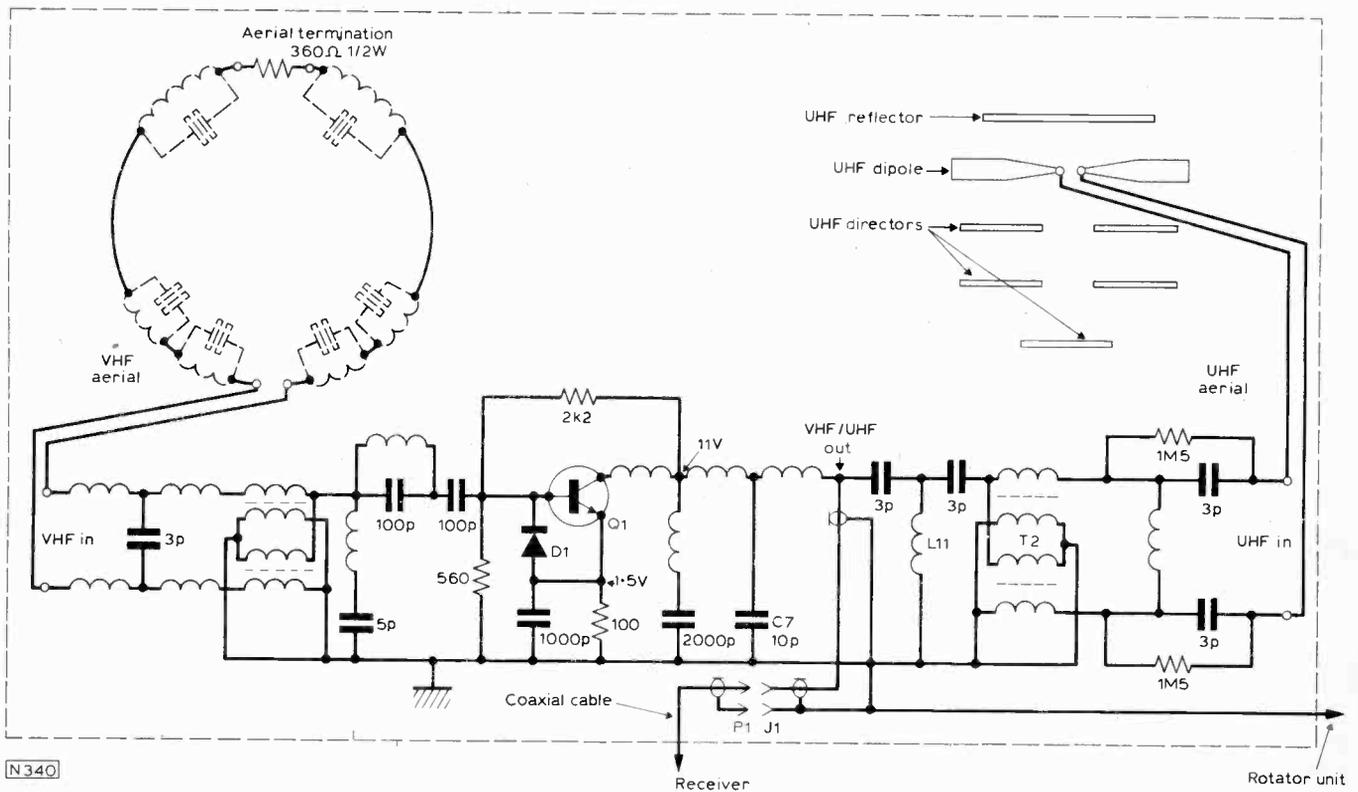
Fig. 4: Circuit diagram of the aeriels and associated amplifier and matching system.
