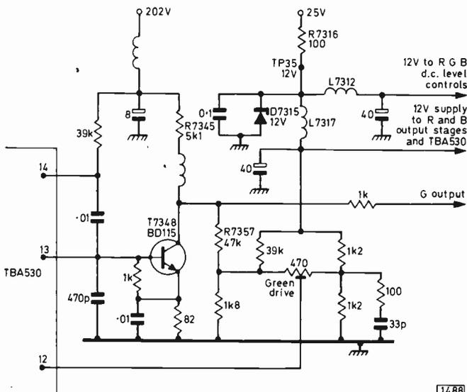
Fig. 1: Circuit of the green output stage. The blue output stage circuit is identical but the red output stage has fixed feedback, i.e. a fixed potential divider replaces the preset drive control. Also showing l.t. feeds in this area.
