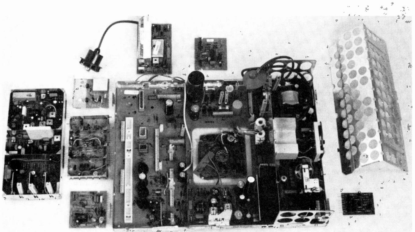
*Fig. 2: General view of the mother board which forms the basis for the CVC20 with the various modules removed. This, coupled with the retention of the "swing-down" service position as used in previous ITT chassis, makes for easy accessibility. Another advantage is the ability of the modules to be plugged onto the reverse side of the mother board so that in-situ module repair is simplified.*
