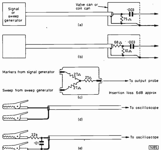
Fig. 8: General purpose probe details. (a) Simple probe suitable for most valve stages. (b) Divide by eight probe to present the low impedance often required when working on transistor circuits: 800μV from the signal generator yields 100μV at the probe end. (c) Mixer unit to enable markers to be added without upsetting the impedance of either feed. (d) Simple take-off probe. (e) Take-off probe with filter to remove spurious beats.
