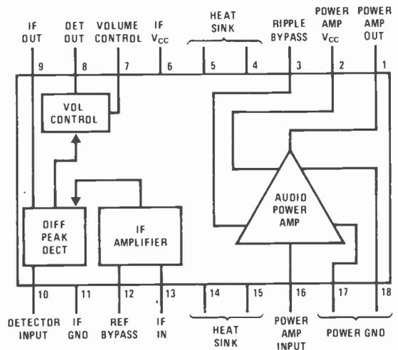
Fig. 4. Functional block diagram of the National LM 1808.
