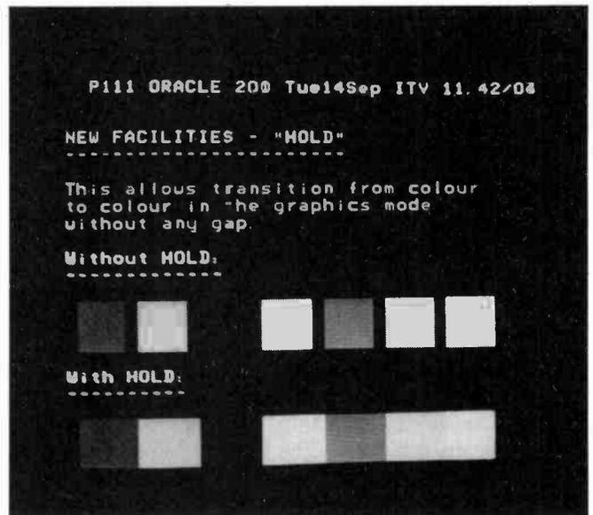
Showing the principle of "hold", which gives colour transitions without a gap between.
