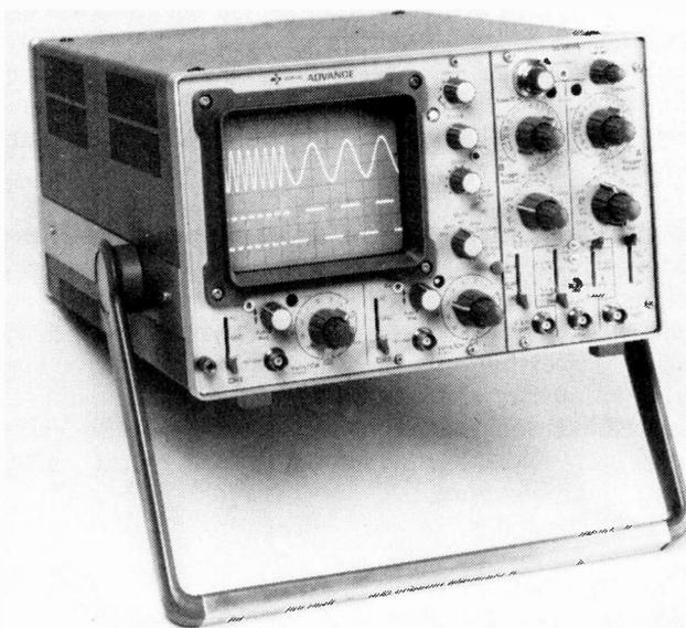
Another newcomer from Gould Advance is the OS3300B; this is a portable 50MHz dual trace unit which is suitable for both laboratory and general servicing use.
