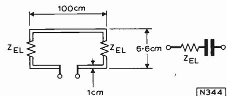
Fig. 8: Experimental miniature unidirectional dipole for Band I TV reception, developed at the Toshiba Research Centre.
