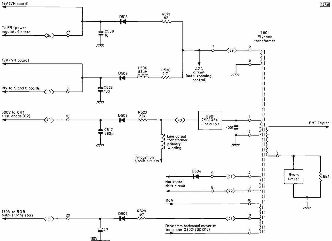
Fig. 3: Supplies derived from the flyback transformer in the Sony Models KV1310UB and KV1330UB. Diodes D503, D504, D507, D508 and D513 are all on the VH board. The 12V line oscillator supply is dropped from the 18V output from D513/C558 – there is a kick-start circuit, powered from the 110V h.t. supply, in order to get the line oscillator working before the line timebase comes into full operation.
