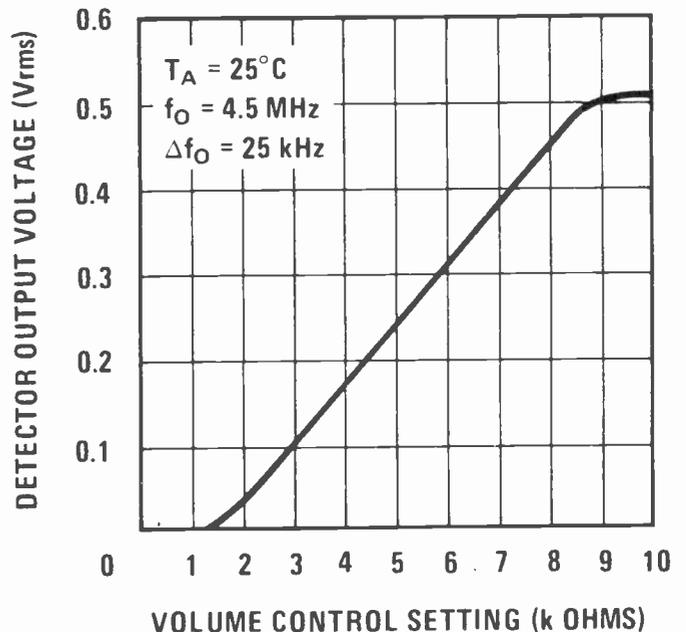
Fig. 5. Volume control characteristic of the LM 1808.
