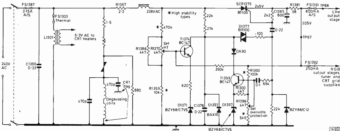
Fig. 2: The power supply circuit. This is the current circuit – variations will be found in earlier versions.
