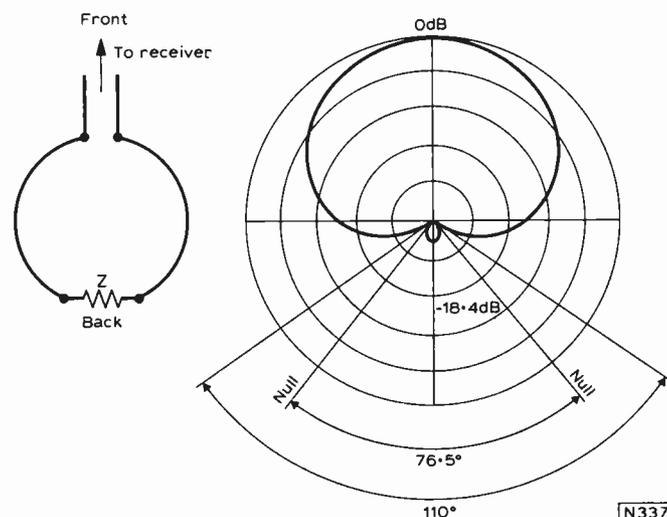
Fig. 1: The terminated loop aerial and its associated polar response.
