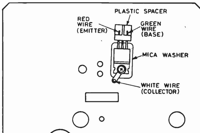
Fig. 1: Fitting a 2N5296 or TIP31 transistor in place of the AD161 20V supply regulator transistor in the ITT CVC5 and later chassis in the series.
