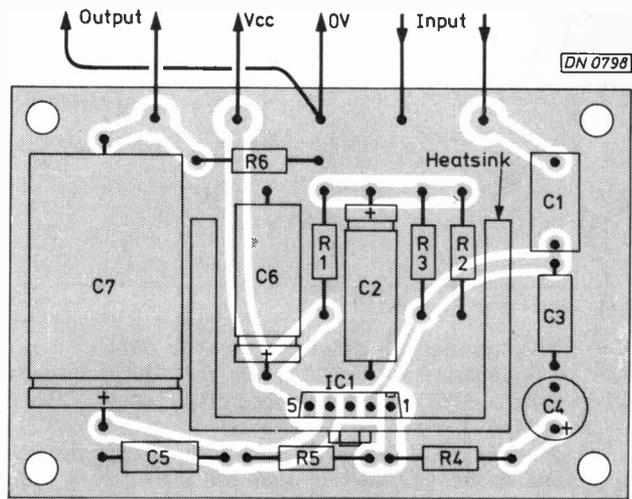
Fig. 7. P.c.b. details and component layout diagram for the audio amplifier circuit. The i.c. and heatsink (type TV35) are available from A. Marshall (London) Ltd, 42 Cricklewood Broadway, London NW2 3ET. Both this board and the p.c.b. for the sound channel circuit are available from Readers PCB Services Ltd, PO Box 11, Worksop, Notts.
