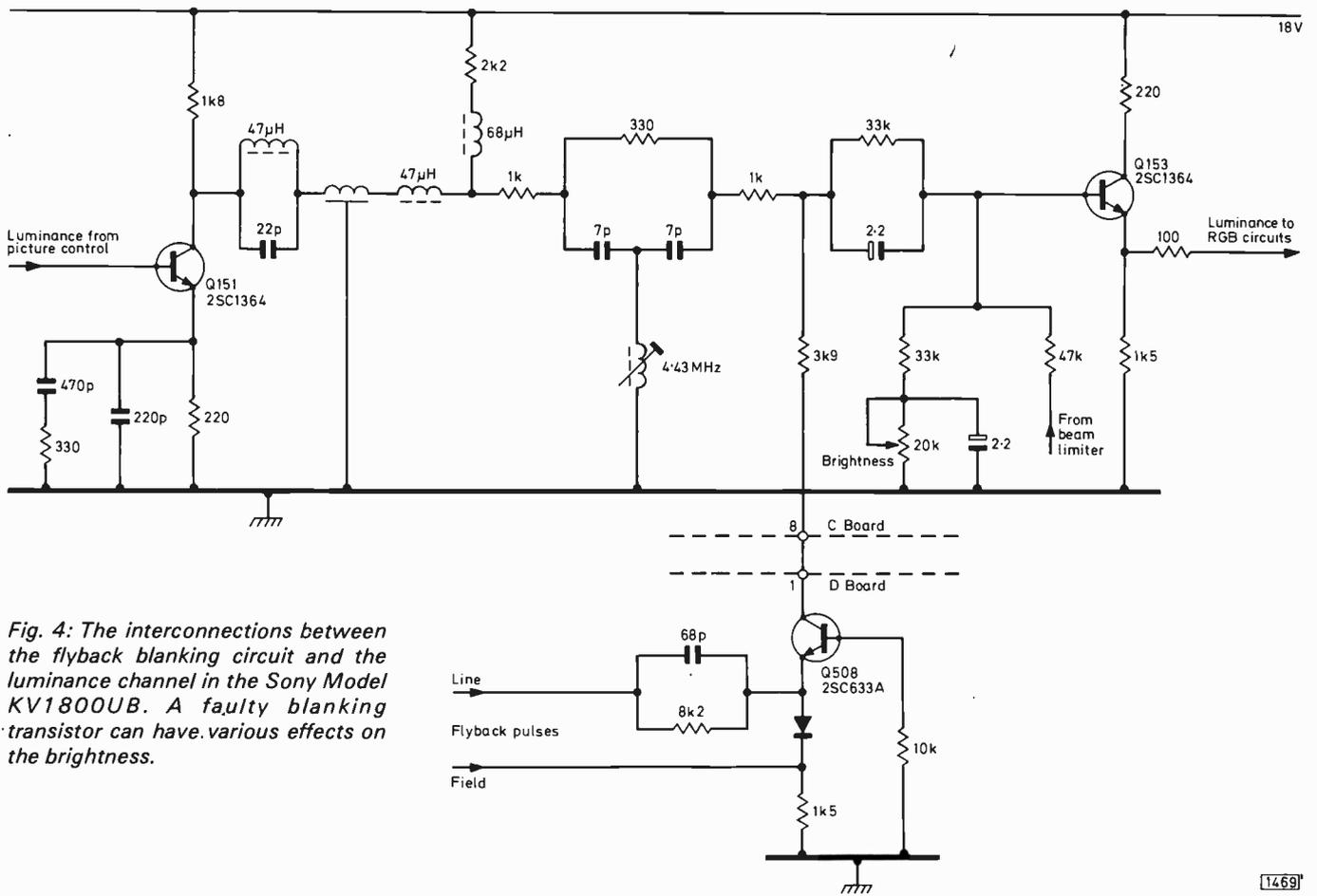
Fig. 4: The interconnections between the flyback blanking circuit and the luminance channel in the Sony Model KV1800UB. A faulty blanking transistor can have various effects on the brightness.
