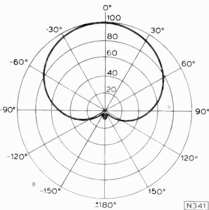
Fig. 5: Typical Band I response.
