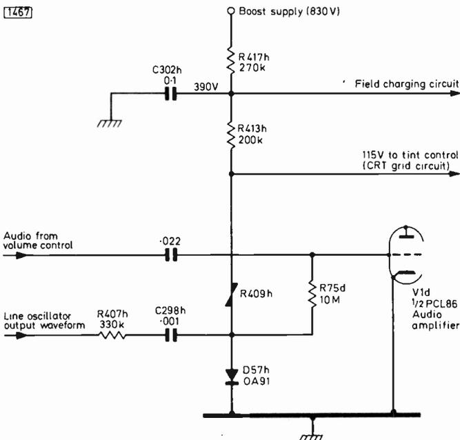
Fig. 2: This circuit links the boost, field charging, audio and tint control circuits in the CVC5 and subsequent ITT chassis.
