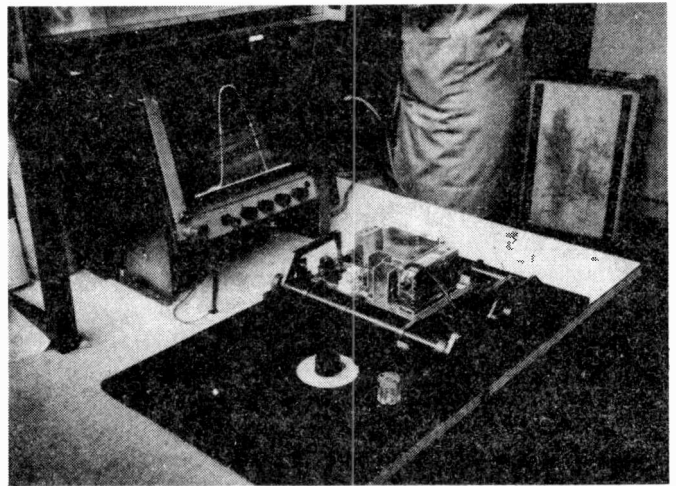
The modern method of factory alignment, with the i.f. board mounted on a pin jig through which signals are injected and extracted and power supply connections made. The large knob on the left is the signal attenuator. Each step is selected by a push button. As the monitor screen shows, a text book i.f. trace is obtained every time! (Courtesy Pye, Lowestoft.)
