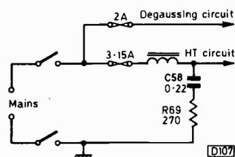
Fig. 1: Snubber network (C58, R59) connected between the junction of the mains filter coil and the anode of the thyristor mains rectifier to chassis to protect the thyristor against peak voltages. The type of capacitor used is important.
