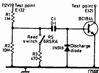
Fig. 1: Automatic VCR switch-off modification. The reed relay is operated by a magnet cemented to the counter pulley. A suitable magnet is the RS type 349-052.
