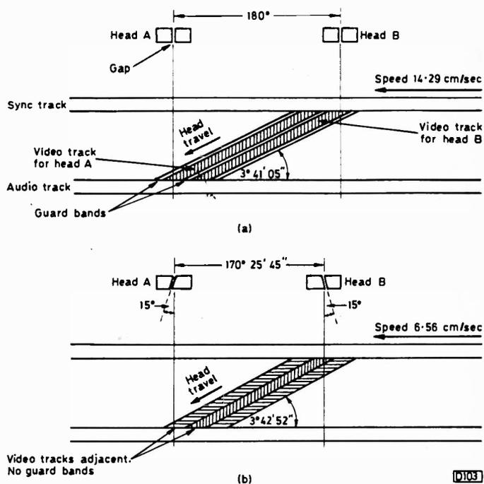
Fig. 1: Comparison of the basic N1500 (a) and N1700 (b) systems. In the 1500 the video track width is 130µm, the distance between tracks 57µm and the distance between track centres 187µm. In the 1700 the video track width is 85µm, the tracks are adjacent and in consequence the distance between track centres is also 85µm. The track length is 16.5cm in both systems.
