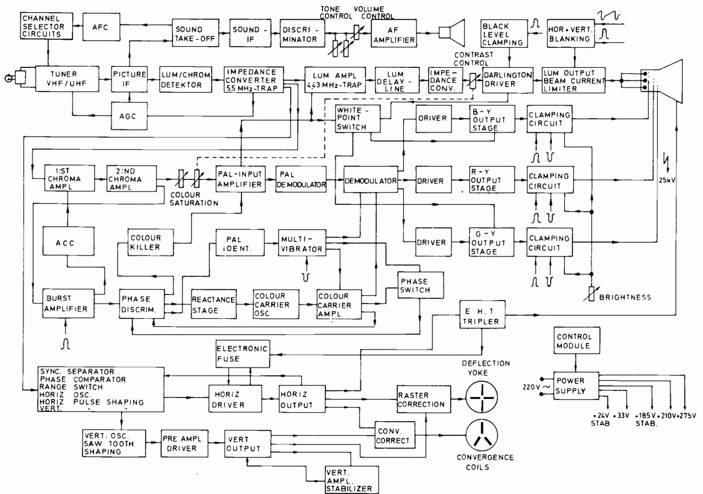
Fig. 3: Block diagram of the receiver.
