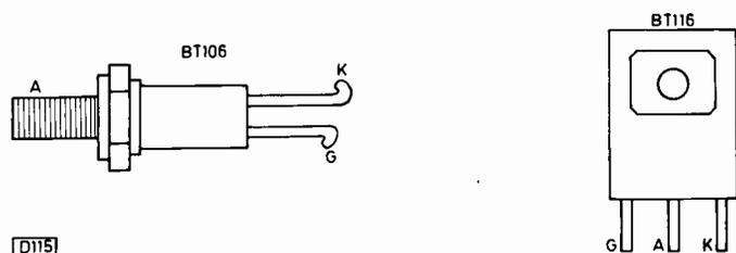
Fig. 6: Specimen thyristors. To test whether a thyristor is operational, connect the black probe to the anode and the red probe to the cathode: there should be no reading until the gate is shorted to the anode.
