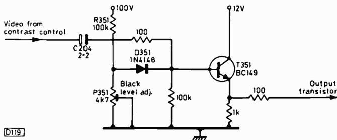
Fig. 4: Diode D351 acts as a d.c. restorer to set the black level following a.c. coupling via C204 in the GEC 3133 series.
