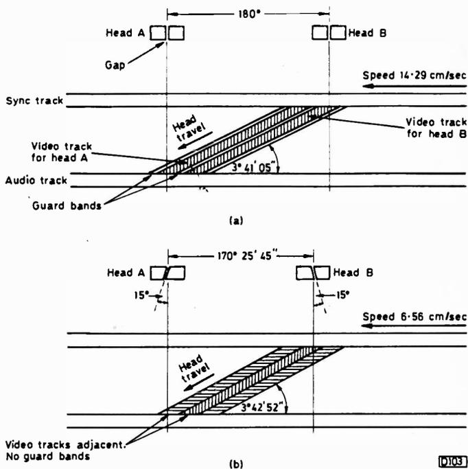
Fig. 1: Comparison of the basic N1500 (a) and N1700 (b) systems. In the 1500 the video track width is  $130\mu\text{m}$ , the distance between tracks  $57\mu\text{m}$  and the distance between track centres  $187\mu\text{m}$ . In the 1700 the video track width is  $85\mu\text{m}$ , the tracks are adjacent and in consequence the distance between track centres is also  $85\mu\text{m}$ . The track length is 16.5cm in both systems.
