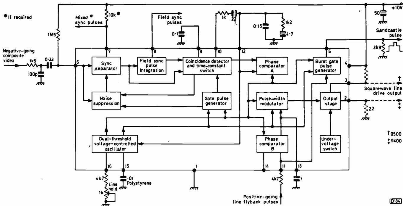
Fig. 2: Block diagram of the TDA9400/9500 sync separator/line generator i.c., also showing the peripheral circuitry.
