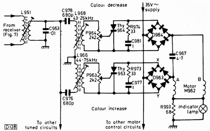
Fig. 8: The motor control system for colour change.
