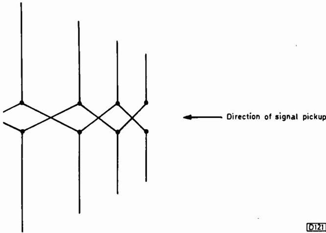
Fig. 1: Basic principle of the log-periodic aerial, showing the cross-connections (not to scale).
