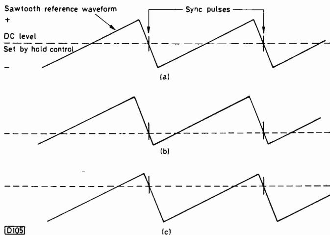
Fig. 1: Action of a flywheel line sync discriminator circuit. Note how the areas above and below the d.c. level vary when the reference sawtooth is early (b) or late (c), giving rise to a positive- or negative-going output respectively after integration by the filter circuit.
