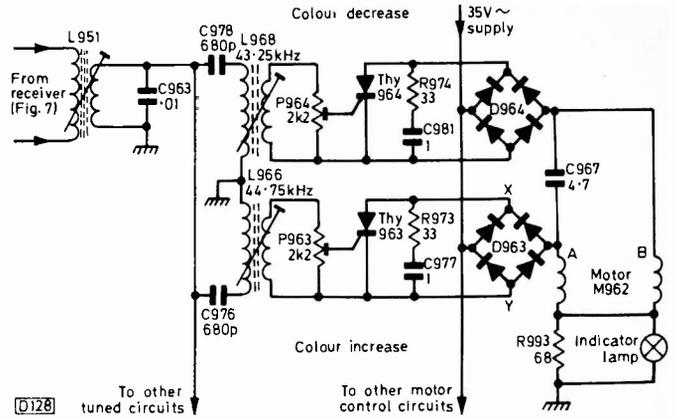
Fig. 8: The motor control system for colour change.
