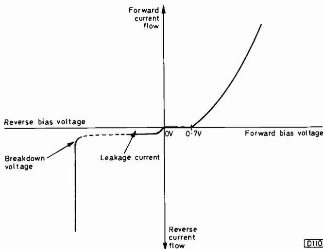
Fig. 1: Silicon diode characteristics. With a germanium diode, forward conduction starts at a lower forward bias voltage, typically 0.3V. The breakdown voltage varies for different types of diode.
