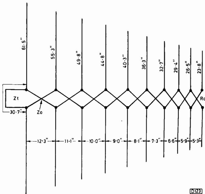
Fig. 3: Ten-element log-periodic aerial design by D. Browne, covering the same bandwidth as before but with a gain of 8.25dBi. Dipoles 1, 2 1in.; 3  $\frac{7}{8}$ in.; 4, 5  $\frac{3}{4}$ in.; 6, 7  $\frac{5}{8}$ in.; 8-10  $\frac{1}{4}$ in. Boom two 2in. tubes spaced as before and with stub as before. Boom length 6.3ft.
