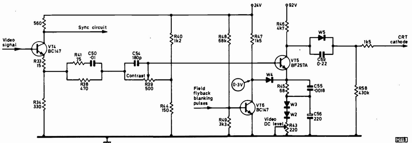
Fig. 3: Video circuitry used in the Thorn 1613 chassis.
