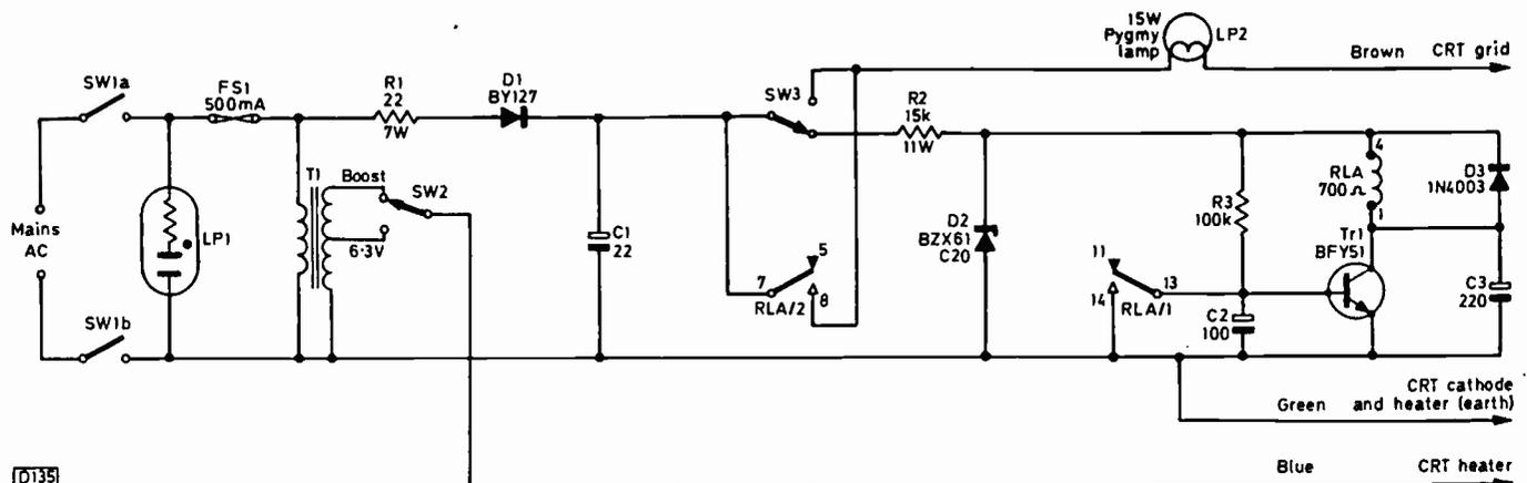
Fig. 1: Circuit diagram of the unit. SW3 shown in the pulsed operation position.
