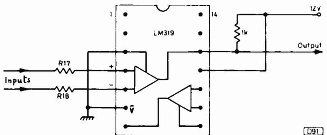
Fig. 4: Using an LM319 dual-comparator i.c. as a video slicer. Only one half of the i.c. is used.
