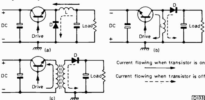
Fig. 1: Basic switch-mode power supply circuits. (a) Series circuit – the chopper transistor's inductive reservoir  $L$  is in series with the load. (b) Parallel circuit, with the inductive reservoir in parallel with the load. (c) Showing how a parallel circuit can provide mains isolation.
