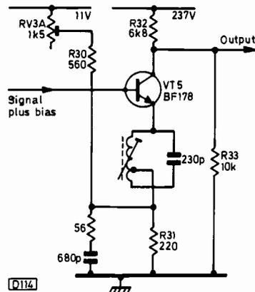
Fig. 5 (right): The video output stage in the Pye 173 chassis. R33 limits the voltage at the collector of VT5 when the transistor is not conducting. The current flowing through R31 is the sum of the currents flowing through the transistor and resistors R30/RV3A. If the transistor is not conducting there will still be voltage readings across R31 and R32 therefore.
