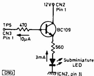
Fig. 3: Adding a colour signal indicator light to the Sony Model VO2850P U-matic editing machine.
