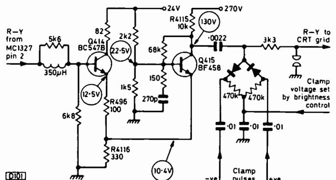
Fig. 2: The colour-difference signal channels are unusual, consisting of an emitter-follower driving a common-base transistor output stage. The R-Y channel is shown above.
