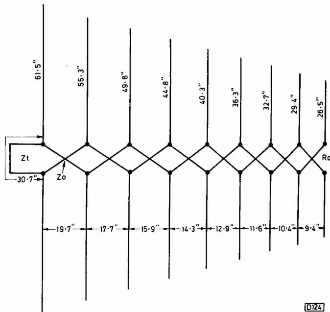
Fig. 4: Nine-element log-periodic aerial design by D. Browne, covering 48-68MHz. Gain 8.6dBi. Dipole 1 1in.; 2, 3  $\frac{7}{8}$ in.; 4  $\frac{3}{4}$ in.; 5, 6  $\frac{5}{8}$ in.; 7, 8  $\frac{1}{4}$ in.; 9  $\frac{3}{8}$ in. Boom and stub as Fig. 3.
