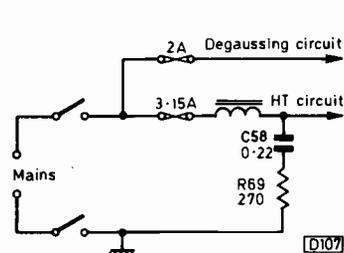
Fig. 1: Snubber network (C58, R59) connected between the junction of the mains filter coil and the anode of the thyristor mains rectifier to chassis to protect the thyristor against peak voltages. The type of capacitor used is important.
