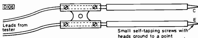
Fig. 2: Suggested probe for use with the in situ transistor tester featured in our October 1976 issue.
