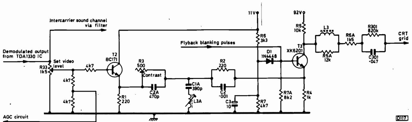
Fig. 2: Video channel, with common-base output stage, used in the ITT VC400 chassis.
