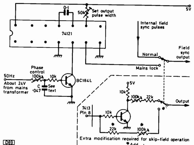
Fig. 2: Adding a mains lock circuit to overcome the problem of recorded tapes with unreadable field sync pulses.
