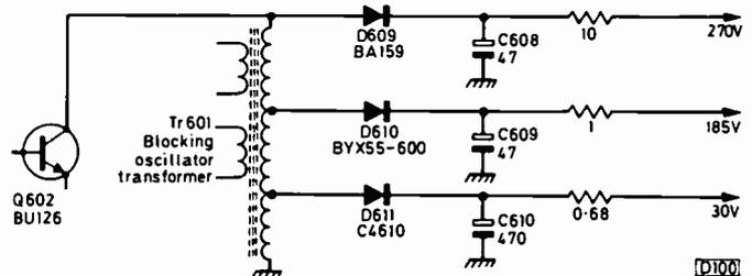
Fig. 1: The parallel switch-mode power supply uses the BU126 chopper transistor Q602 in a blocking oscillator circuit. The primary winding of the blocking oscillator transformer Tr601 acts as the inductive reservoir, feeding three half-wave rectifiers.
