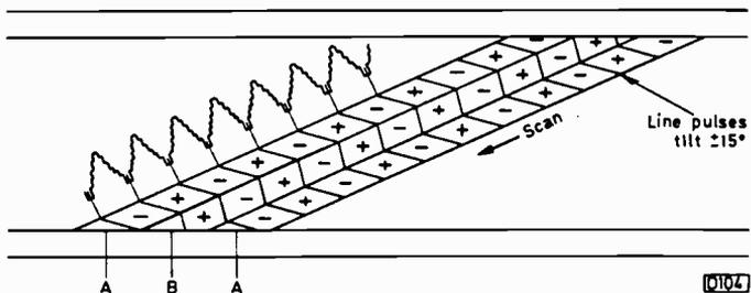
Fig. 2: Schematic (not to scale — head A's field contains 311.5 lines and head B's 313.5 lines) showing how lines with identical colour phases are laid beside each other.
