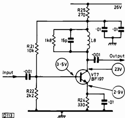
Fig 4 (left): The final i.f. amplifier stage in the Thorn 1500 chassis. R21/R22 provide forward bias for the base. If the voltage across the emitter resistor R24 is correct the transistor is operating normally.
