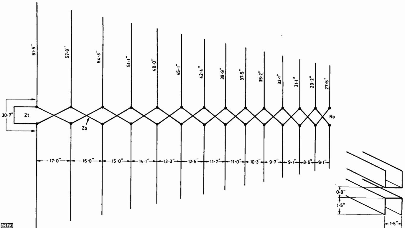
Fig. 2: Log-periodic aerial design by D. Browne, covering 48.25-85.25MHz with a gain of 9.25dBi. Dipole tubing diameters are as follows: 1, 2 1 in.; 3, 4 7/8 in.; 5-7 3/4 in.; 8-11 5/8 in.; 12-14 1/4 in. The boom can be 2in. tubes spaced 2.5in. between centres, or two lengths of U channelling as shown, with the stub Zt shorted 15.3in. from the final dipole. Boom length 13.2ft.
