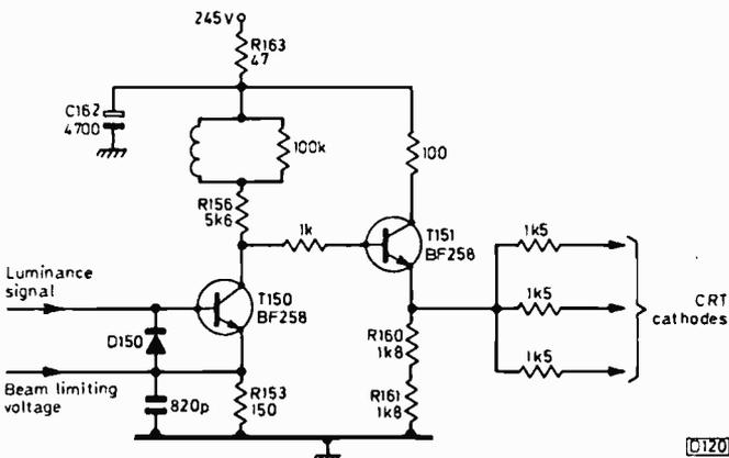
Fig. 5: Luminance output stage used in Korting hybrid sets, with an emitter-follower driving the c.r.t. cathodes.
