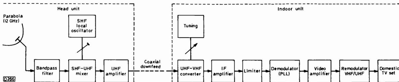
Fig. 1: Block diagram of a double-superhet receiving system developed by Mullard.
