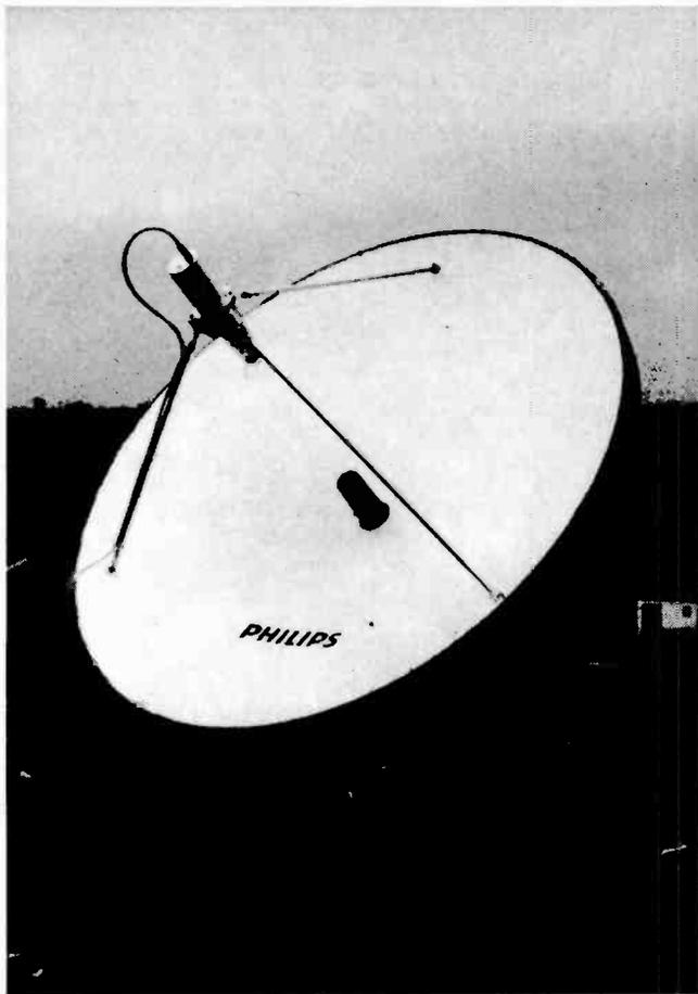
*Philips 1.2m dish/head end used for the Canadian CTS satellite experiments.*
