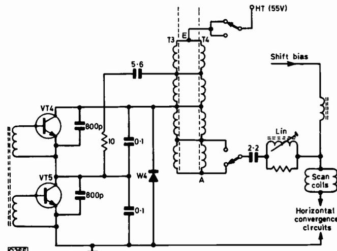
Fig. 3: Line output stage circuit (simplified) used in the Thorn 2000 chassis. The raster correction circuit is connected across points E and A. Note that there are three "LOPTs" in all in the 2000 chassis. One is used in the separate e.h.t. generator circuit. The other two (T3/4) are connected in parallel in the line output stage.
