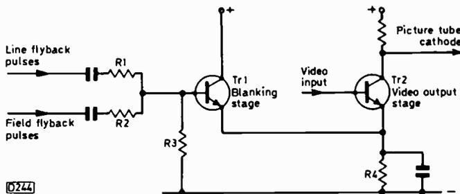
Fig. 4: One method of achieving flyback blanking.
