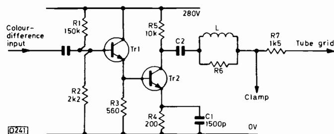
Fig. 1: Essentials of a colour-difference signal amplifier.
