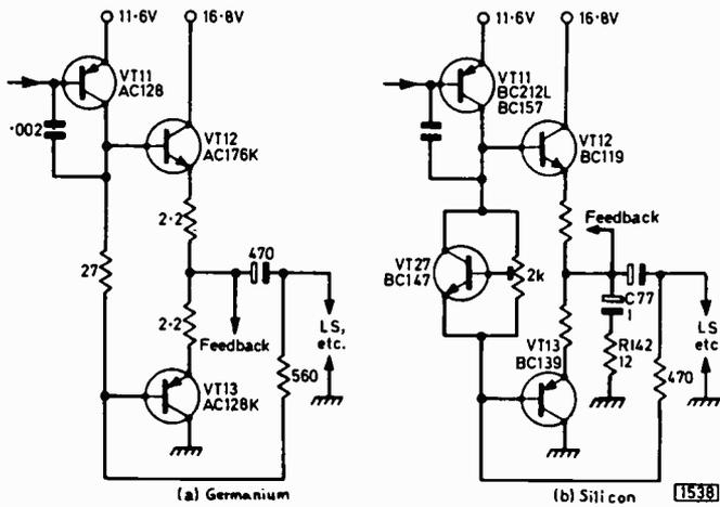
Fig. 2: Audio circuit modifications when silicon devices are used in the output and driver stages. The network C77, R142 was added to improve the audio stability.
