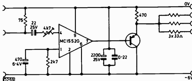
Fig. 2: Alternative version of the circuit for use as a pulse distribution amplifier.
