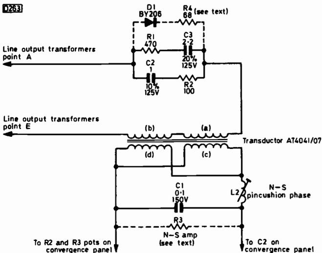
Fig. 1 Raster correction circuit.
