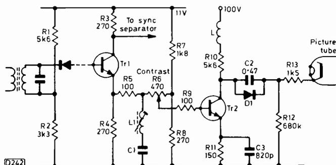
Fig. 2: Video driver and output stage circuits for a monochrome portable set.
