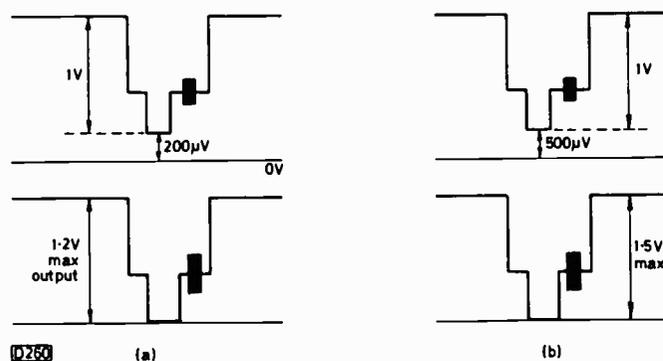
Fig. 3: Output waveforms obtained from the video distribution amplifier circuit. (a) Standard 6V circuit. (b) Circuit with 6V supply and 22kΩ resistor added between pin 1 of IC1 and chassis (across the 470µF capacitor).
