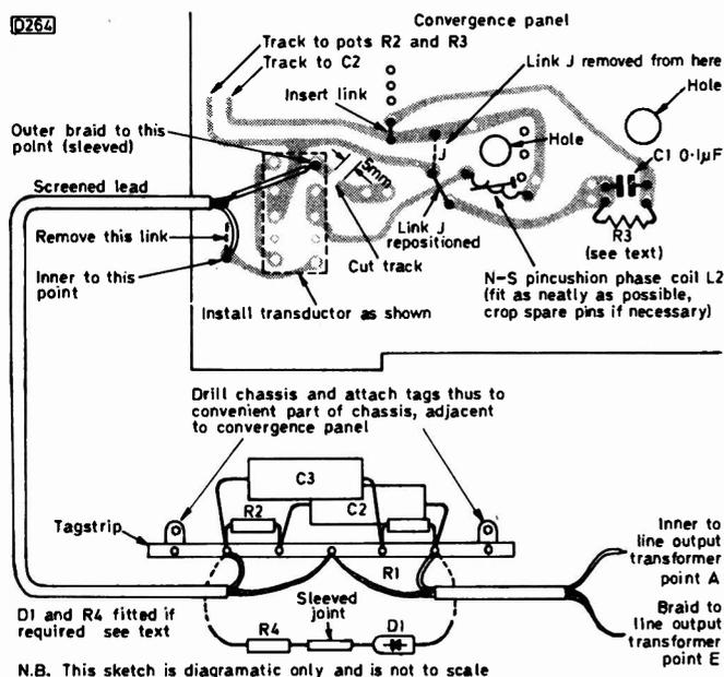
Fig. 2: Physical layout of the modification.
