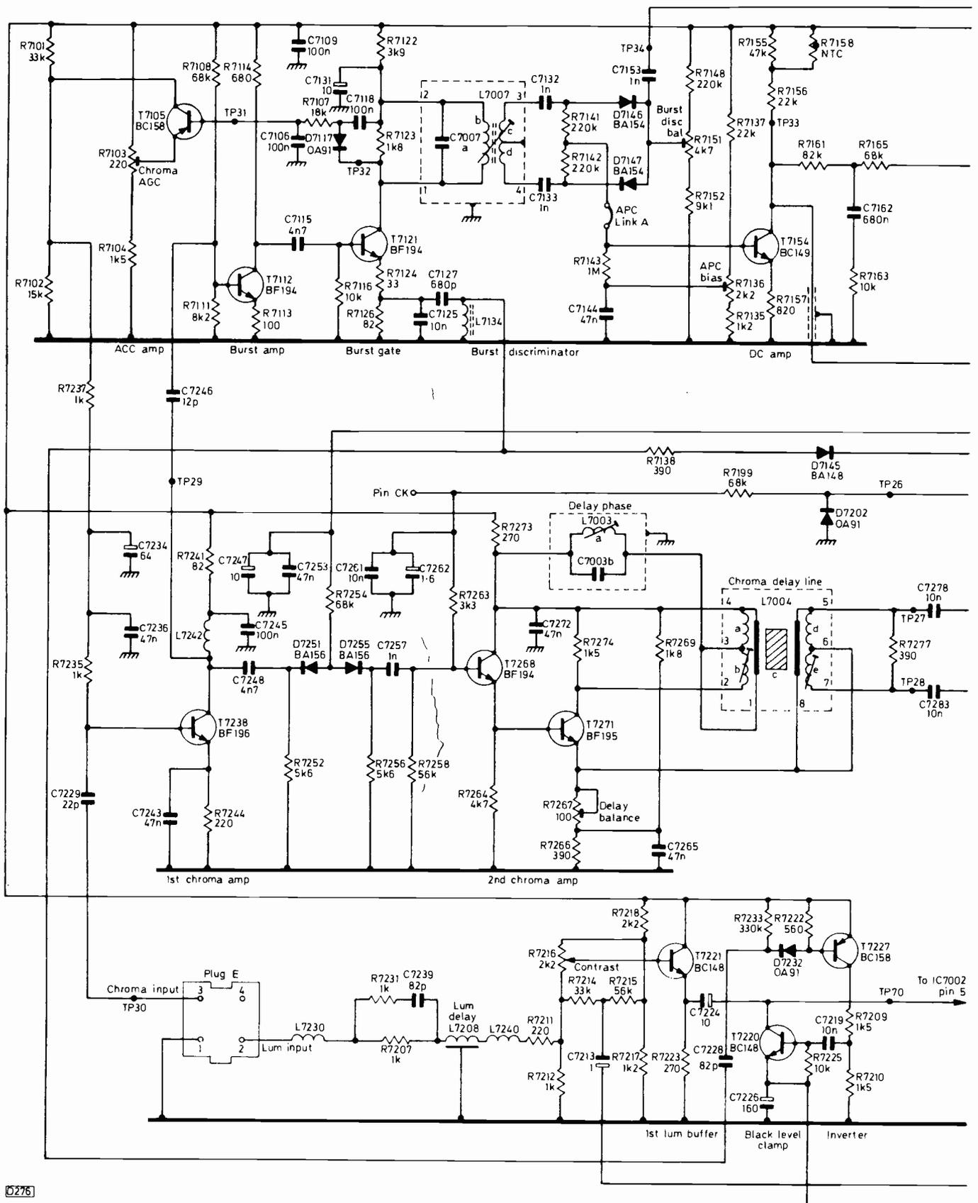
Fig. 9: Circuit of the two-i.c. decoder
