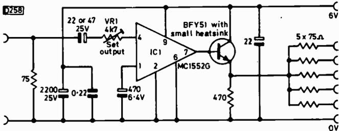
Fig. 1: Steve Beeching's video distribution amplifier circuit. Adding a 22kΩ resistor between pin 1 of IC1 and chassis alters the output as shown in Fig. 3(b).
