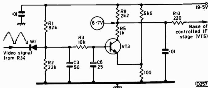
Fig. 3: A.G.C. circuit used in the Thorn 1500 chassis.
