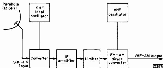
Fig. 2: Block diagram of an s.h.f./f.m. video receiver developed by NKH, Tokyo.
