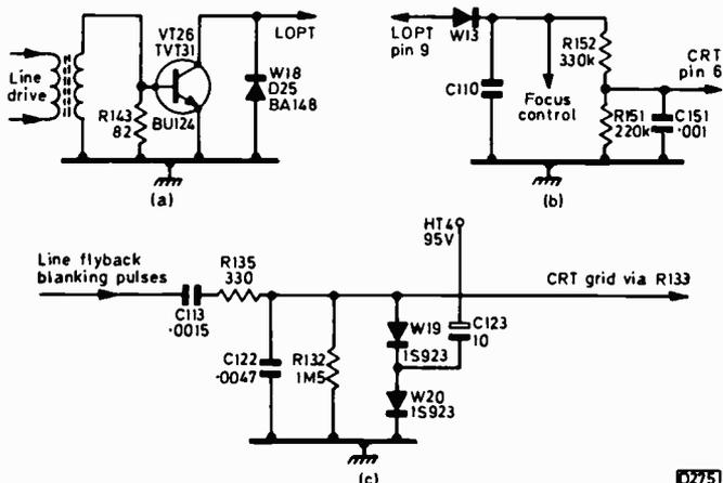
Fig. 3: Recent modifications. (a) Use of silicon line output transistor. (b) Revised c.r.t. first anode supply with c.r.t. type TMT31-102. (c) Spot-quench circuit.
