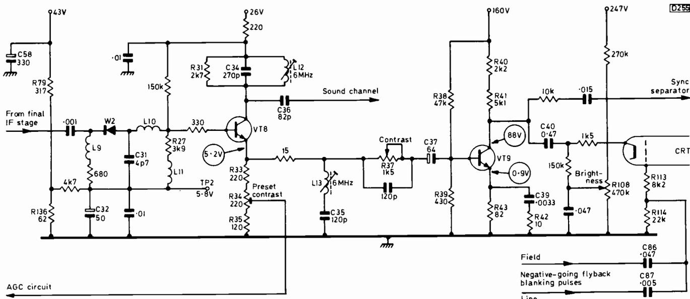
Fig. 1: Video circuitry used in the Thorn 1500 chassis.
