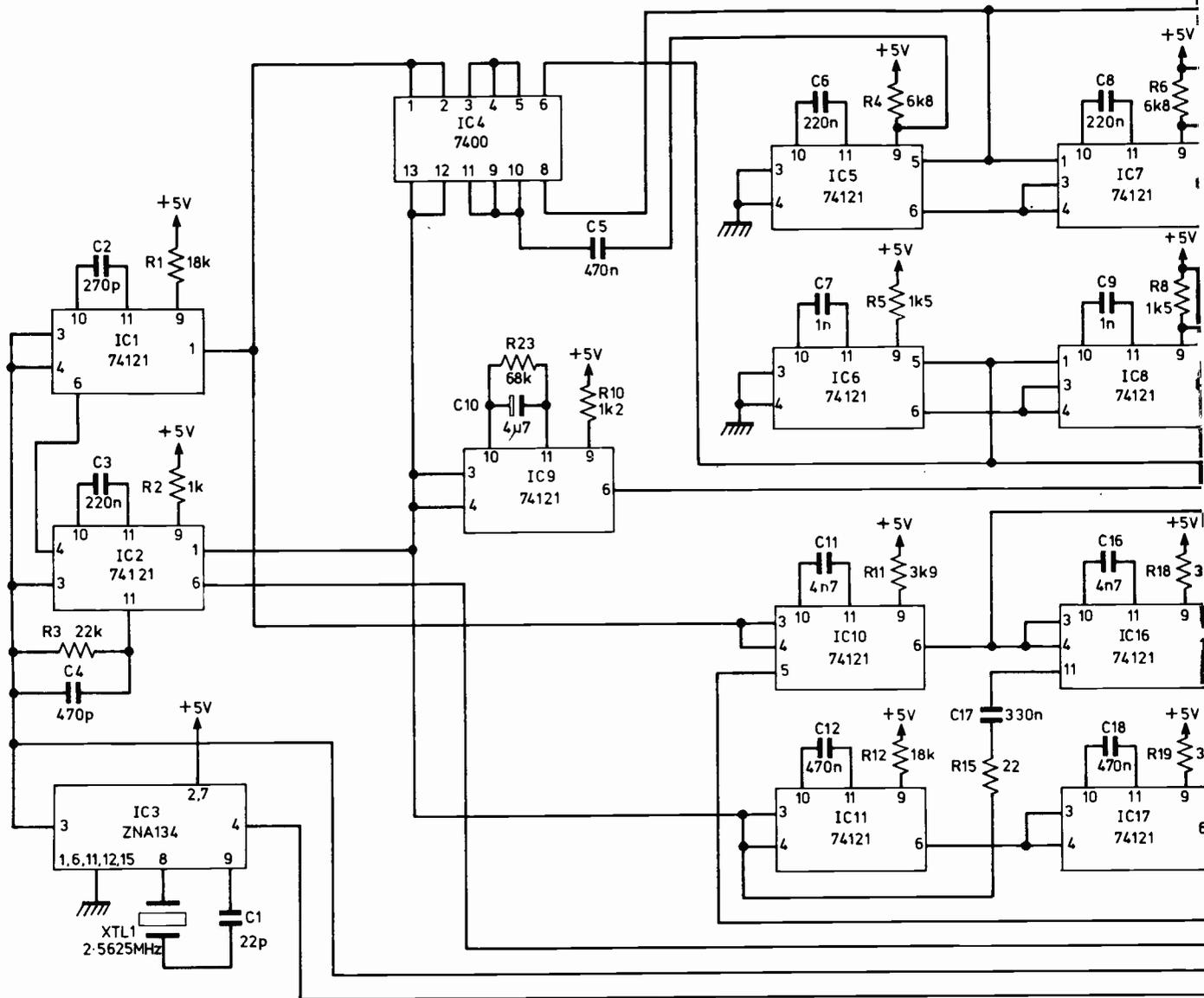
Fig. 3: Circuit of the diagnostic pattern generator. With external compatible source or via CR network
