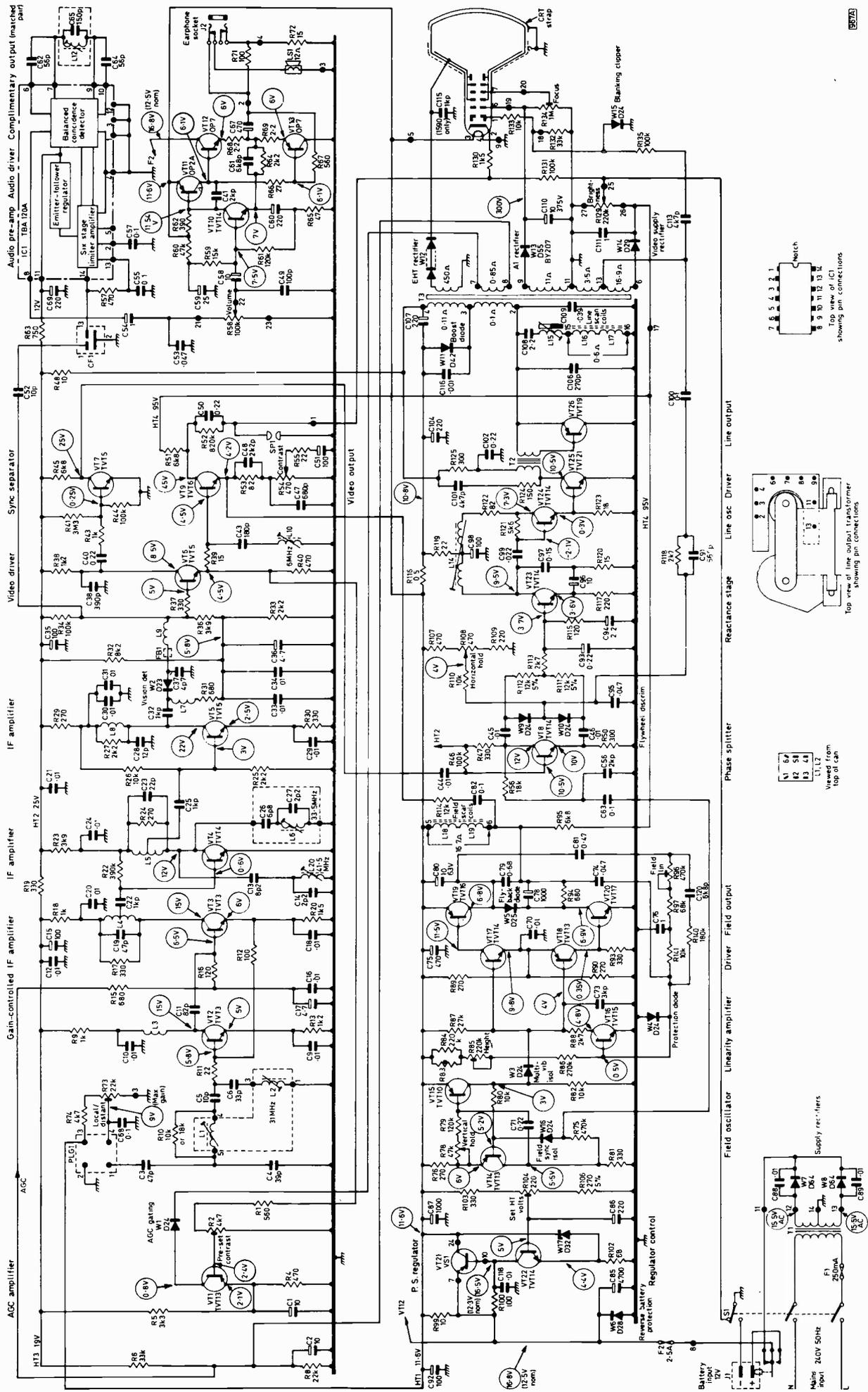
Fig. 1: Circuit diagram, including minor component value changes. In the 12in. chassis (1590) R131 is 150kΩ and C106 0.0039μF. C115 was fitted on earlier 12in. models only. In later production R48 is a safety resistor - see modifications over page. The 560Ω resistor added across L15 in later production is R126. See Fig. 2 for later audio circuitry.
