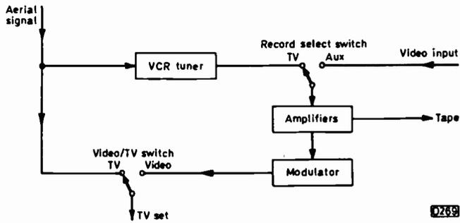
Fig. 1: Input/output switching.
