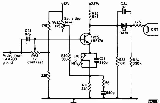
Fig. 2: Video circuit used in the Pye 169/569/173 chassis.
