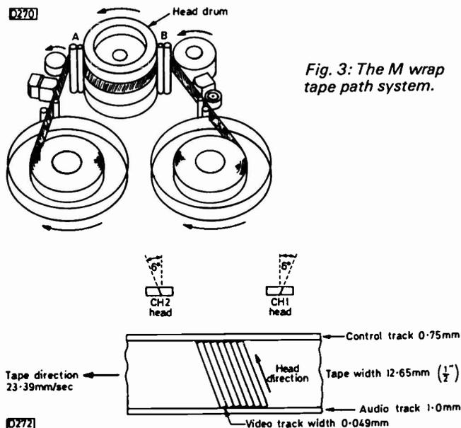
Fig. 4: Head/tape format details.
