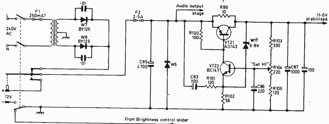
Fig. 1: Power supply with series voltage regulator circuit. Used in the Thorn 1590/1/3 series portable chassis.
