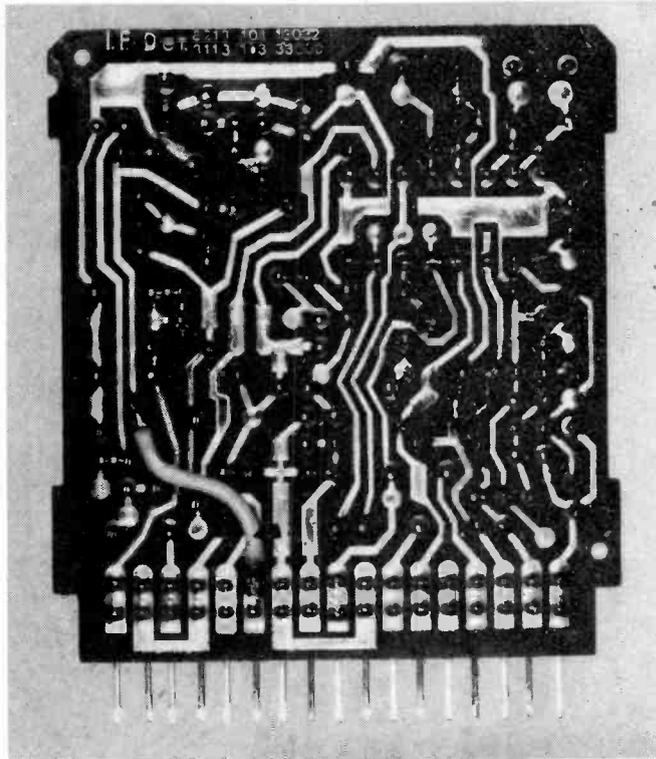
Fig. 1 (above left): The Philips vision detector module, with the screening can and base removed. R654 (arrowed) has to be removed.
