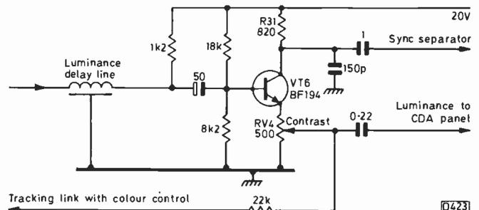
Fig. 2: The "phase splitter" stage in the luminance channel of the Pye group hybrid chassis.
