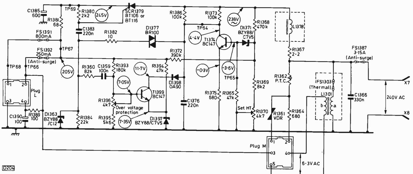
Fig. 2: Use of a thyristor to provide voltage stabilisation. Circuit used in early versions of the Philips G8 chassis.
