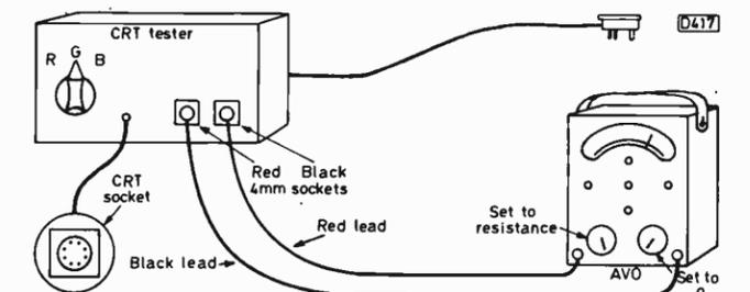
Fig. 3: Physical arrangement of the tester.
