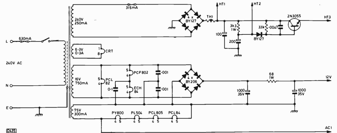
Fig. 3: Power supply circuitry. The 2N3055 transistor acts as an active filter, providing a very smooth h.t. supply.
