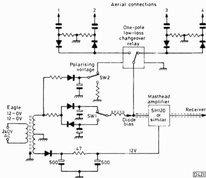
Fig. 2: Thoughts on a possible aerial switching unit.
