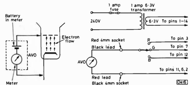
Fig. 1 (left): Electron flow from cathode to grid when the c.r.t. is biased by the meter's internal battery.
