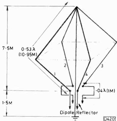
Fig. 1: Basic switchable quad aerial, with legs 1 and 4 acting as the active element (dipole) and legs 2 and 3, with the extra phasing sections, acting as a reflector.
