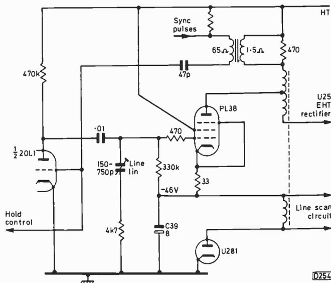
Fig. 3: Simplified circuit of the unusual line oscillator and output stage, with its -46V boost rail.
