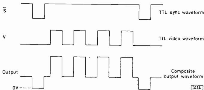
Fig. 1: The input and output waveforms.
