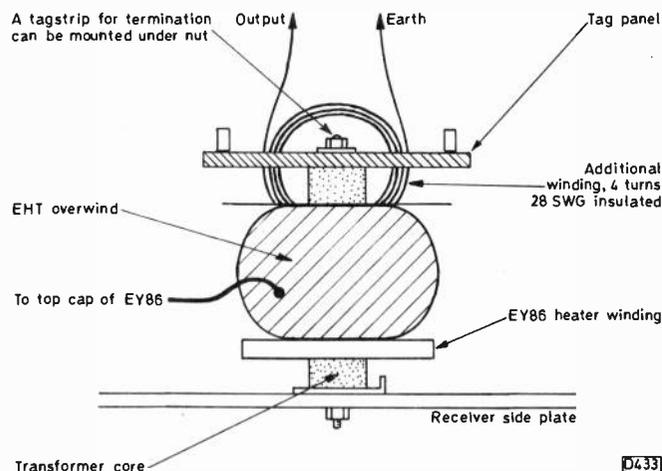
Fig. 1: The position of the extra winding required on the line output transformer. Viewed from the top.
