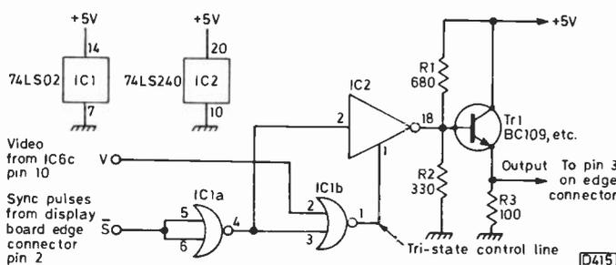
Fig. 2: Improved signal combining circuit.
