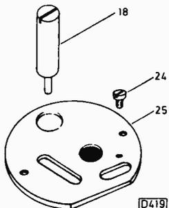
Fig. 1: Resetting the cutout – simplified view of the cutout table (25). Screw 24 and pillar 18 should be slackened and the table turned slightly clockwise. Then tighten the screw and pillar. See text above for further details if the cutout is then too sensitive.
