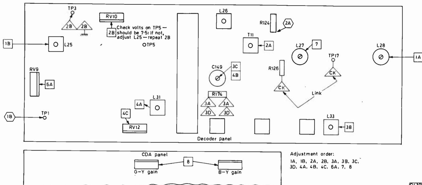
Fig. 11: Aligning the Pye hybrid chassis decoder.
