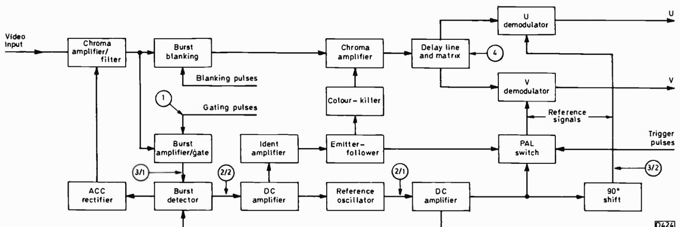
Fig. 3: Block diagram of a typical decoder. The numbers in circles correspond with the alignment procedure given later.
