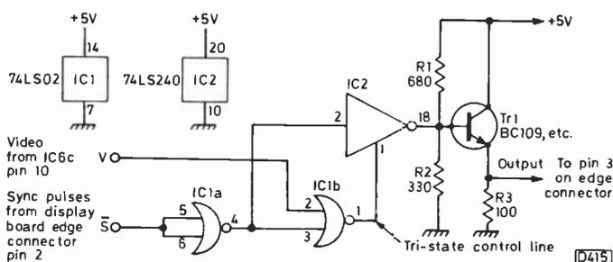
Fig. 2: Improved signal combining circuit.
