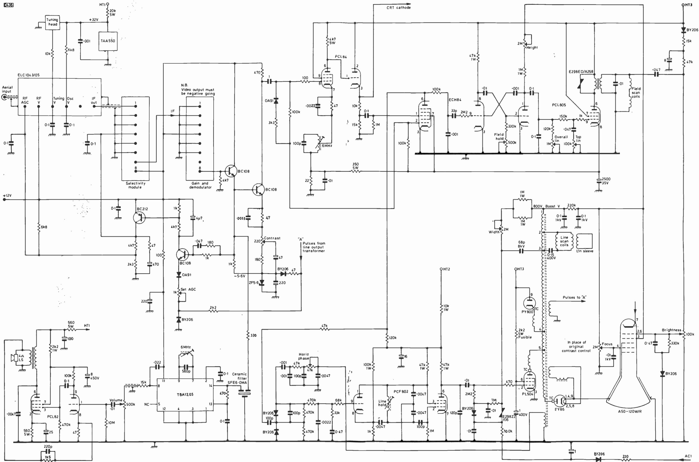
Fig. 4: The signal and timebase circuits of the latest version of the 625-line receiver, incorporating the r.f./i.f. circuitry used in the Television monochrome portable project.
