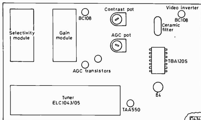
Fig. 2: Suggested layout for the tuner, i.f. components, etc. The tuner, i.f. modules and other components can be arranged on a piece of Veroboard.
