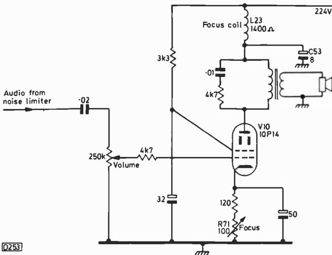
Fig. 2: The sound output stage also provided the current for the focus coil.
