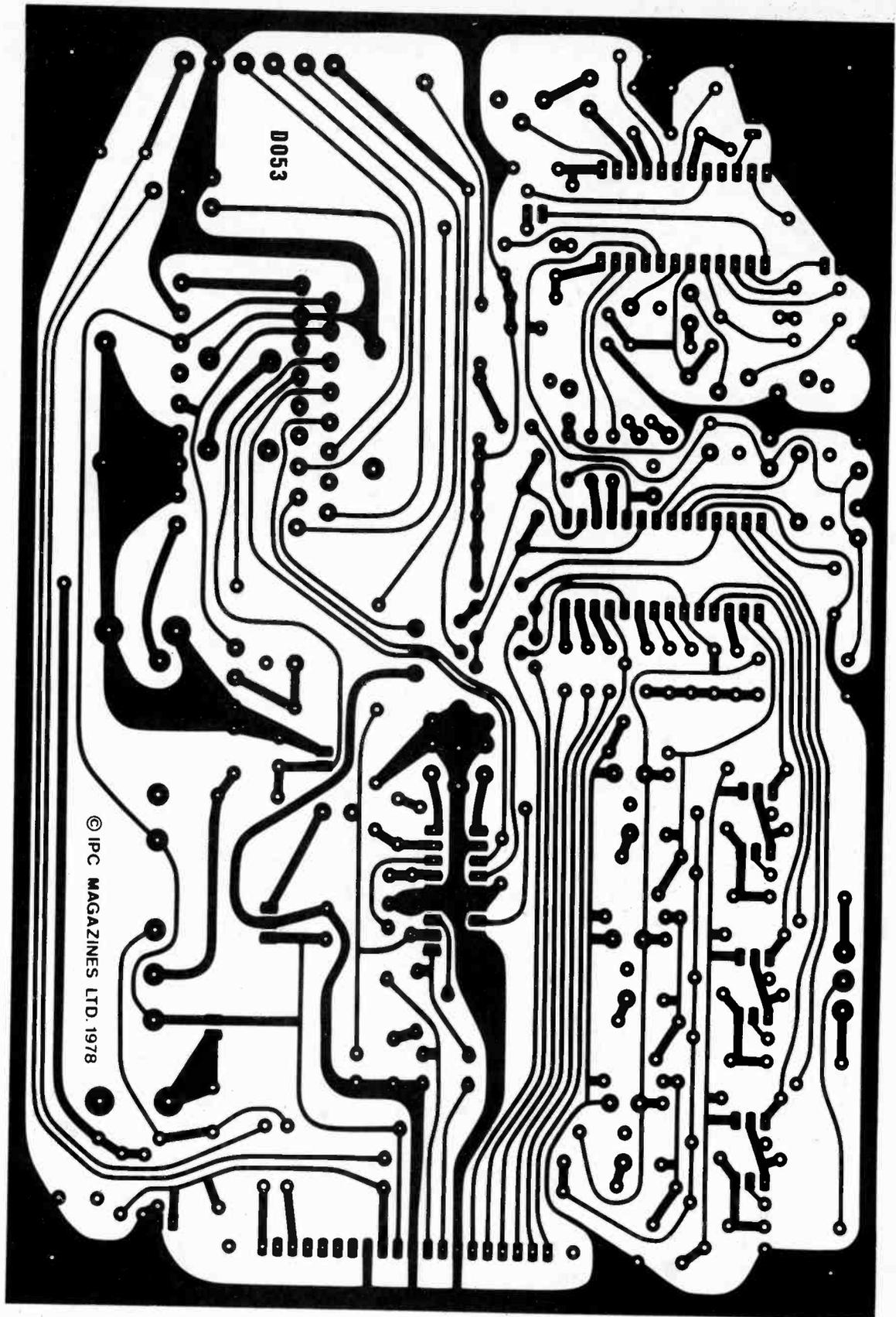
Fig. 3 (above): Copper track pattern for the signals board. Scale 1:1.
