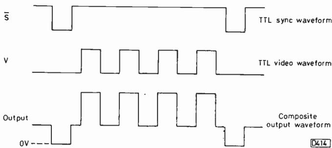
Fig. 1: The input and output waveforms.
