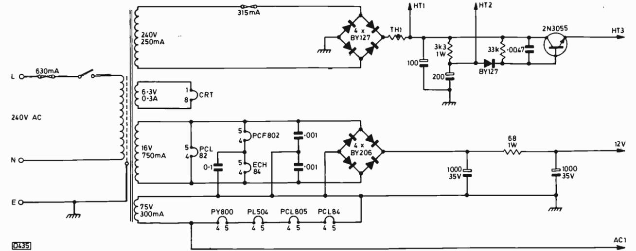
Fig. 3: Power supply circuitry. The 2N3055 transistor acts as an active filter, providing a very smooth h.t. supply.
