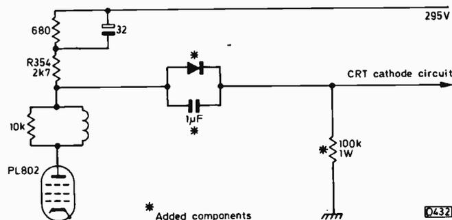
Fig. 10: Adding a beam limiter in the feed to the c.r.t. cathodes. Components shown as in the Pye hybrid chassis.
