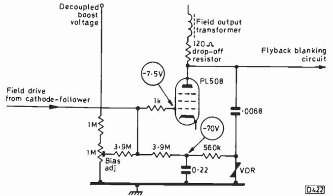
Fig. 1: The field output stage bias circuit used in the Philips G6 chassis, incorporating VDR stabilisation.
