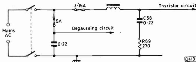
Fig. 3: Mains input circuit used in the GEC C2110 series chassis. The filter network C58/R69 was added to later versions to provide extra protection for the thyristor.
