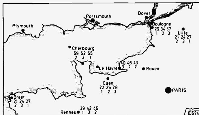
Fig. 1: French TV transmitters which can be received in the UK. Those marked with an asterisk provide a strong signal in good reception conditions only. Cherbourg, Le Havre and Boulogne have an e.r.p. of 100kW, all others an e.r.p. of 1MW. Rouen is also a 1MW transmitter, but the channels are the same as Crystal Palace. The network number is shown beneath the channel number.
