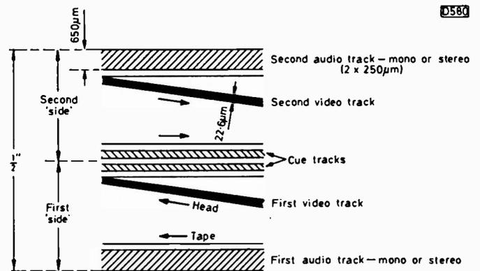
Fig. 1: Arrangement of the tracks on the tape.
