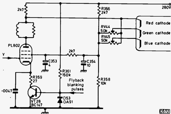
Fig. 3: A typical pentode luminance output stage. In some receivers there are preset controls in all three c.r.t. cathode circuits. The luminance signal is a.c. coupled to the PL802's control grid, and the brightness control acts here via a d.c. restorer. Beam limiting is also generally carried out at this point in hybrid colour receivers.
