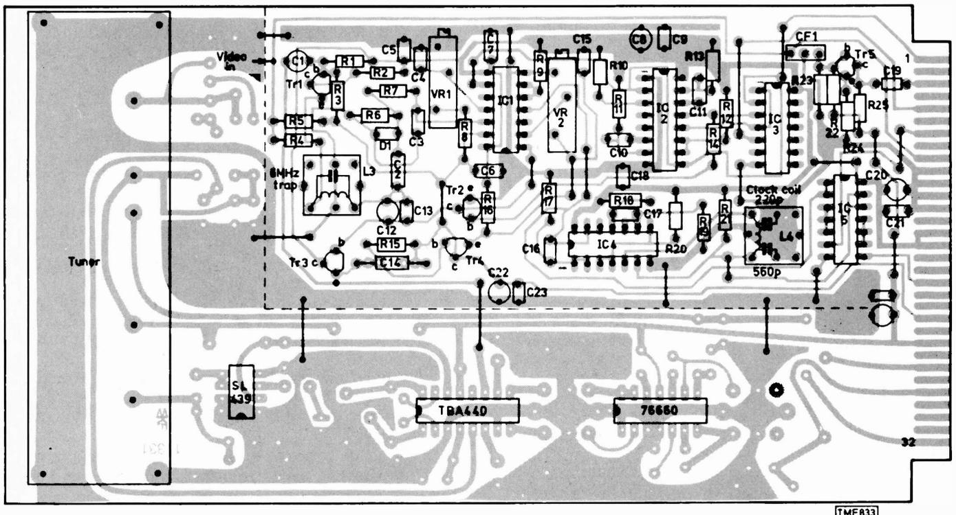
Fig. 2: Component location diagram of the new signal board. The component location diagram for the i.f. section is given in the October 1977 issue.
