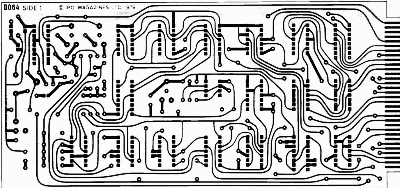
Fig. 5: Underside copper pattern for the teletext options card (see last month), ref. D064.
