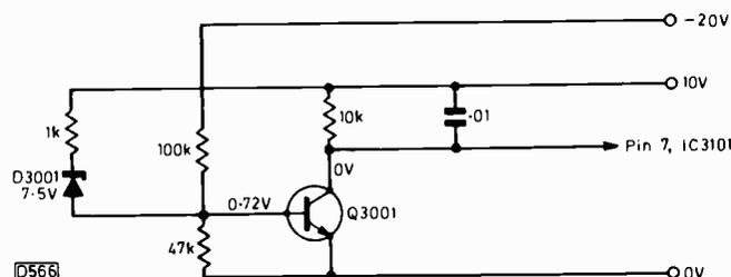
Fig. 1: Timer i.c. reset circuit.
