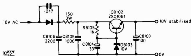
Fig. 2: 10V supply circuit.
