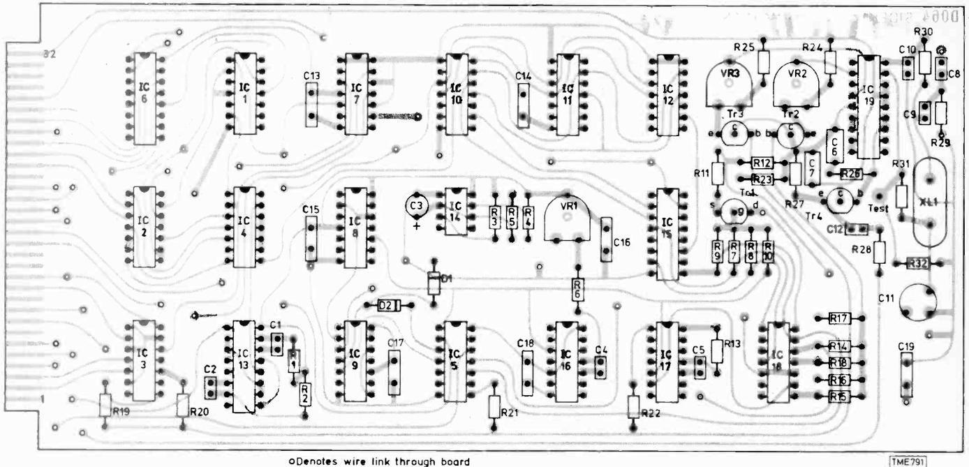
Fig. 7: Component location diagram for the options board.
