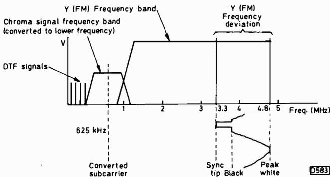
Fig. 4: The signal positions within the bandwidth.
