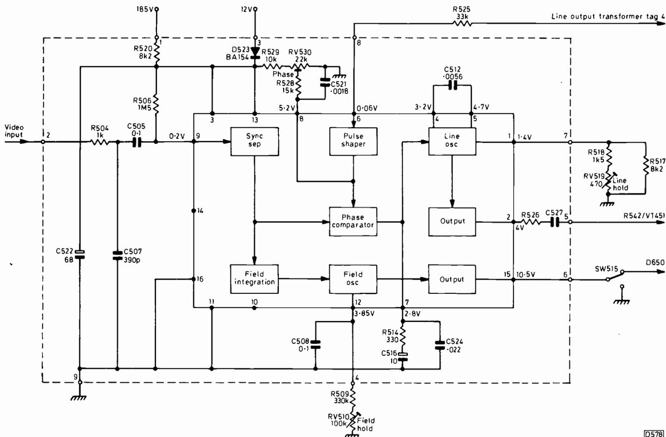
Fig. 3: The 731 chassis uses an SN76544N07 i.c. as the sync separator and line and field oscillator. It's mounted, along with certain associated components, on a subpanel, as shown above. R526 and C527 values as in Fig. 1.
