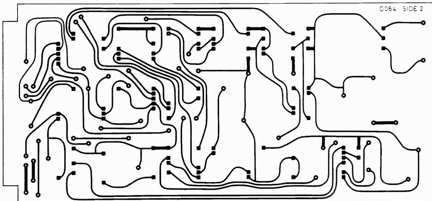
Fig. 6: Topside copper track of the options card D064. Note that the actual board size is 438mm x 205mm.
