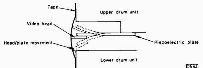
Fig. 3: The heads are mounted on servo-controlled piezoelectric elements to provide dynamic track following.
