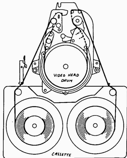
Fig. 2: The M-wrap tape path in the recorder.
