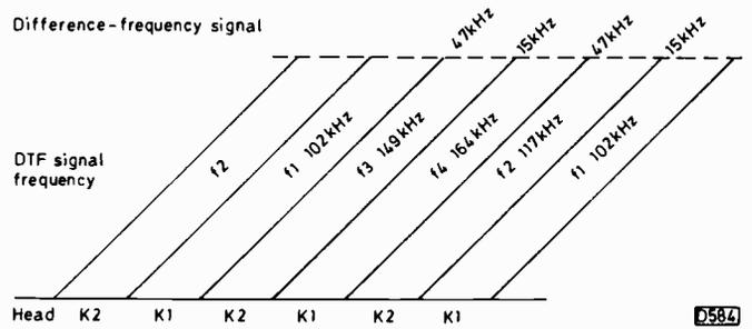
Fig. 5: The sequence of the dynamic track following signals. Read from the right, this is f1, f2, f4, f3.
