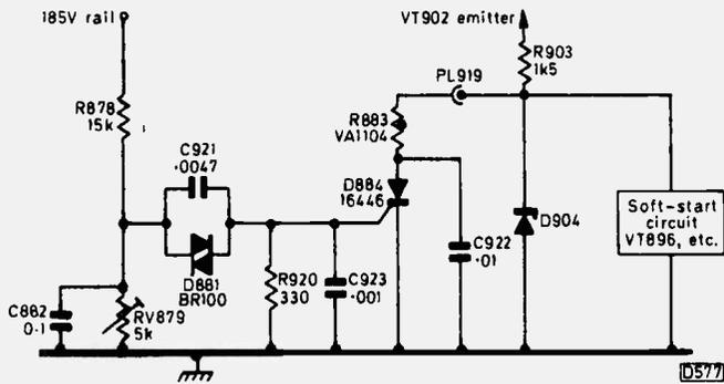
Fig. 2: The over-voltage protection circuit used in early models. On very early versions, PL919 is taken to the cathode of the mains rectifier thyristor: this gives a crowbar action, blowing the mains fuse in the event of excessive h.t. voltage.
