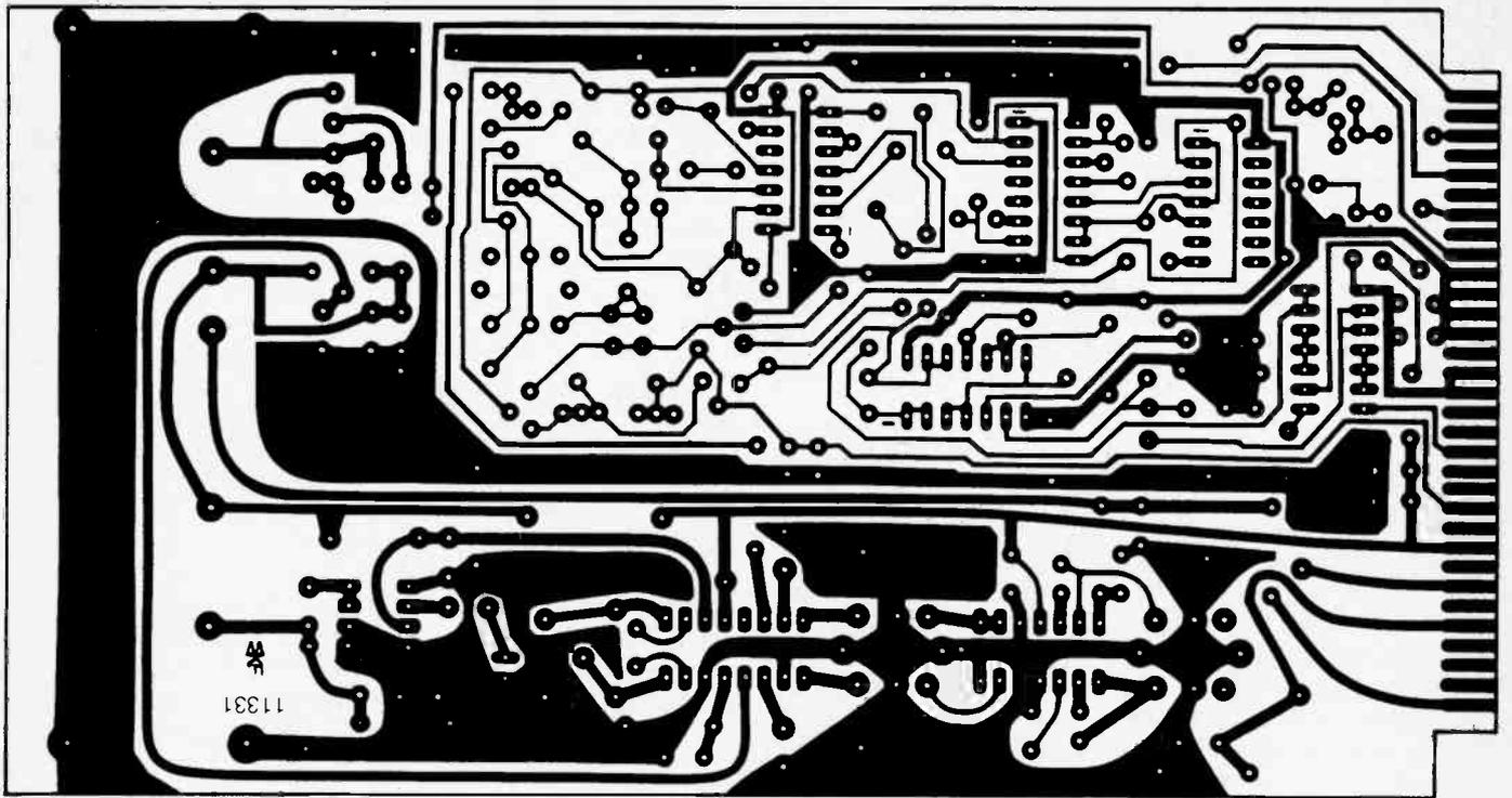
Fig. 3: Copper pattern of the new signal board. The board is available from our Readers PCB Services, reference 11331. Note that the actual size of the board is 386mm x 205mm.
