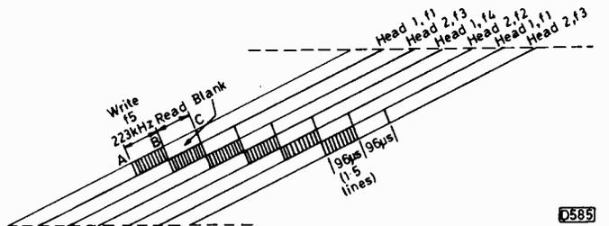
Fig. 6: For dynamic head position correction during recording, a signal is laid down during a 96µsec period while the field flyback is occurring. Recording ceases during the following 96µsec period, the head then reading the crosstalk signal from the previous track. The resultant signal initiates the servo control action.
