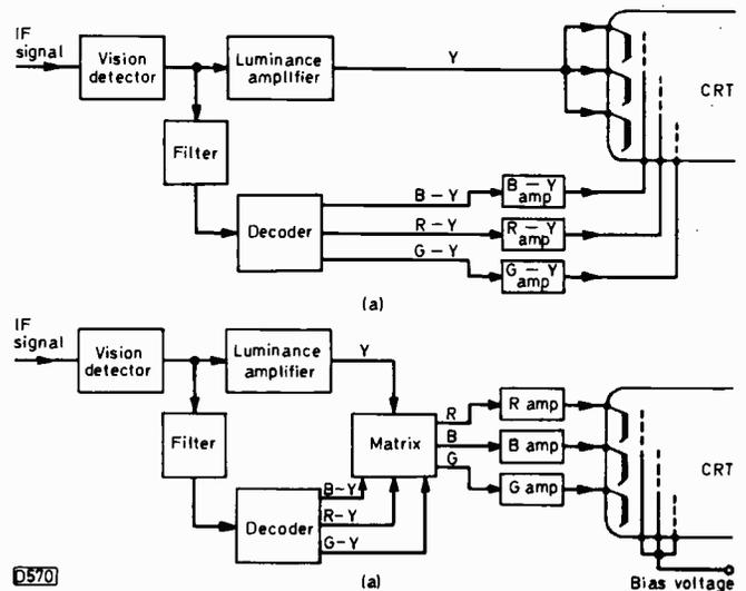
Fig. 1: Methods of driving a colour tube. (a) Colour-difference drive, with the luminance signal (Y) applied to the three cathodes and the three colour-difference signals applied to the grids. The tube then carries out the RGB matrixing, the phosphor screen being activated by the three primary-colour signals. (b) RGB drive. In this case matrixing is carried out prior to the tube, the RGB signals being applied (almost always) to the three cathodes.
