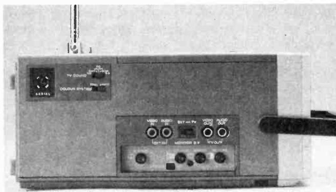
Side view, showing the TV sound and colour system switching and the audio/video input/output sockets.
