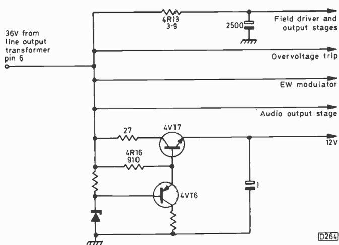
Fig. 3: 36V supply feeds in the Rank T20 chassis.
