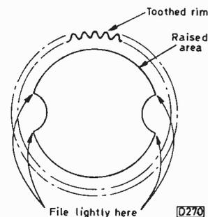
visible. Switch off the mains supply. (4) File the gear, switch on the mains supply and watch for the second filing point. Switch off, file, switch on and allow the machine to unlace. The machine can now be reassembled. **D.S.**
