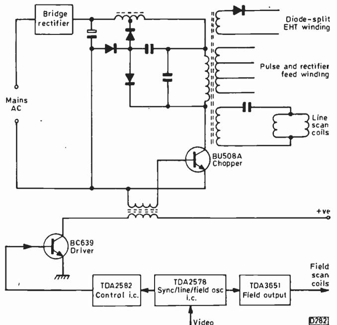
Fig. 1: The Mullard/Philips S<sup>2</sup>P<sup>2</sup> power supply/timebase configuration for use in small-screen colour sets.
