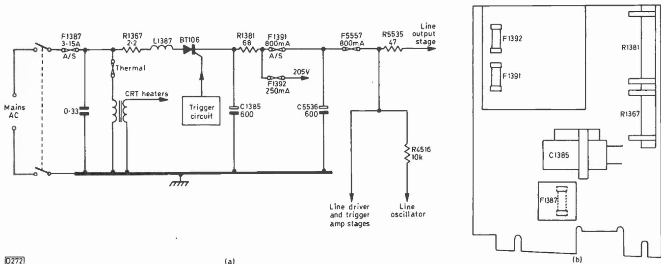
0272 (a) Fig. 1: Mains power supply arrangements (simplified circuit) used in the Philips G8 chassis (a). Positions of the fuses and dropper resistor sections on the power supply panel (b). Components suffixed "1" are on the power supply panel, those suffixed "5" are on the line scan panel, while R4516 is on the timebase panel.
