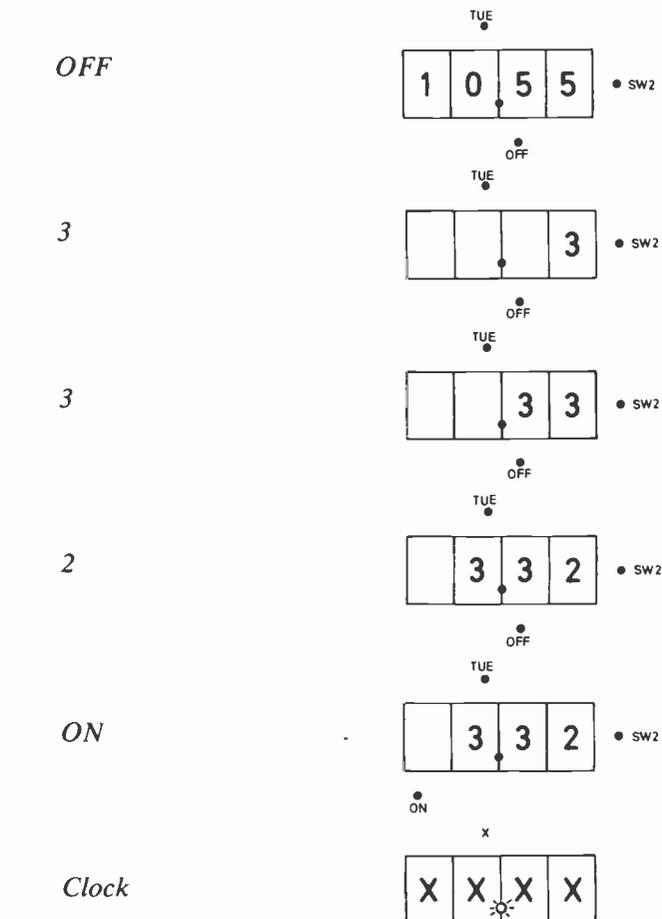
**Direct ON and OFF** (e.g. to turn switch 1 ON directly)
