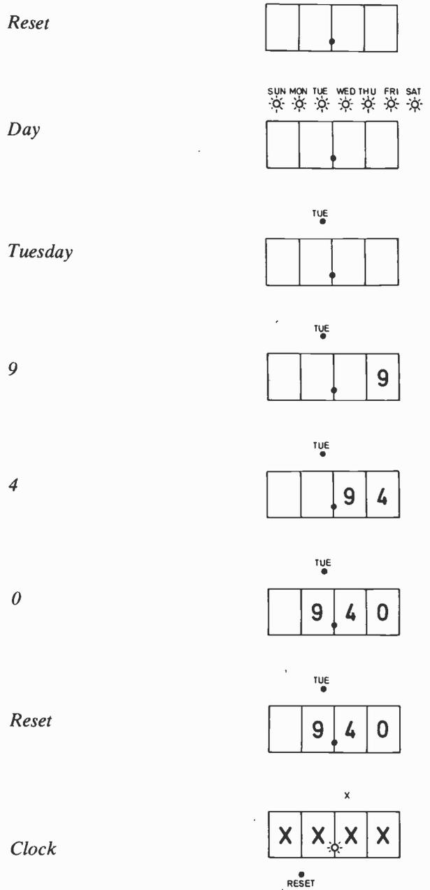
The clock will run until Tuesday 9.40 when it will reset. If continuous reset is selected it will automatically reset to Sunday 00.00 and start counting again. If non-continuous reset is selected it will reset to Sunday 00.00 with the display flashing up zeros and wait until a start command is given. On pressing the start button the clock will commence counting from Sunday 00.00 until the reset point is reached again.
