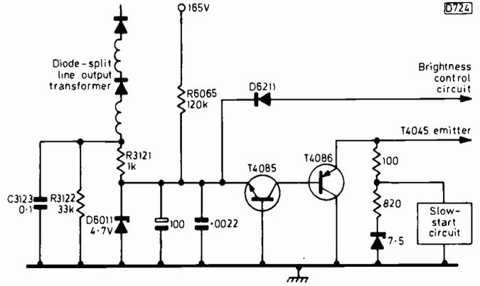
Fig. 7: The circuit used in the Pyel/Philips G11 chassis has two modes of operation (see text).
