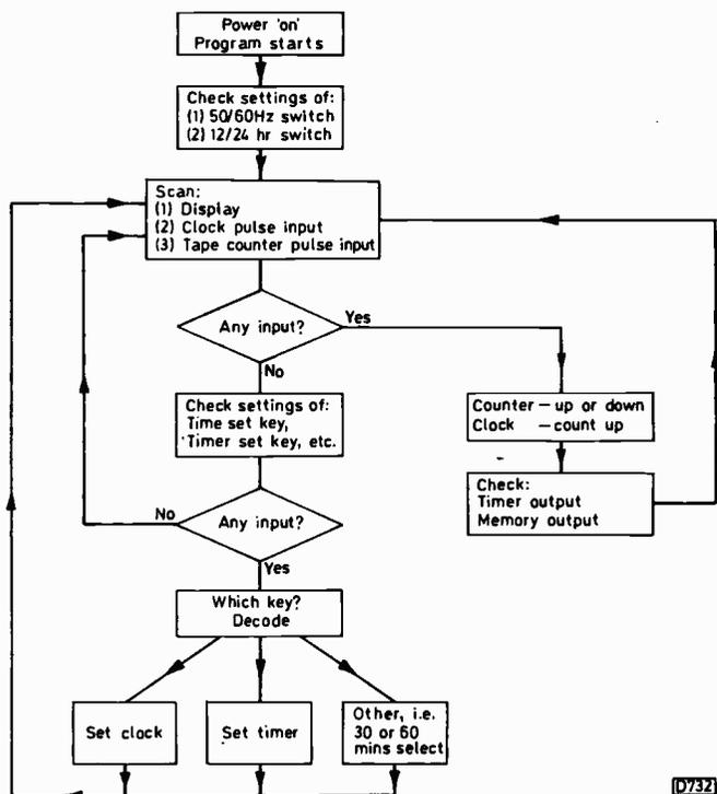
Fig. 4: Flow chart of the TMS1070 microcomputer's programme. The microcomputer starts at the top, then carries out each operation in turn. The whole cycle takes less than  $1 \times 10^{-3}$  seconds.
