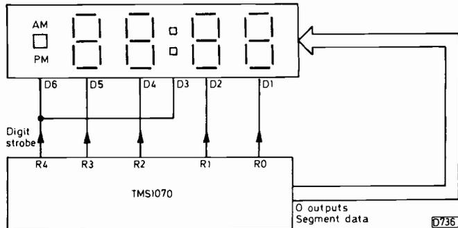
Fig. 8: Driving the fluorescent display.
