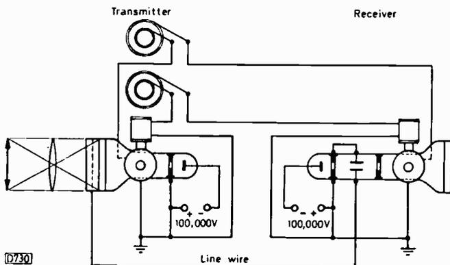
Fig. 1: A. A. Campbell Swinton’s 1912 scheme for an electronic TV system. The main problem was that a camera “plate” to convert the picture into an electronic signal was not at the time available – the development of an effective camera tube was in fact the key to modern television.
