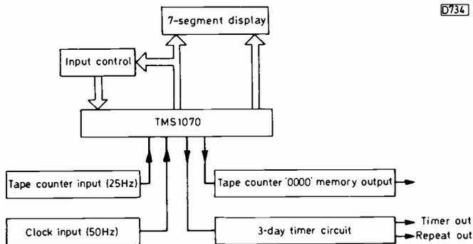
Fig. 6: Use of the TMS1070 in the Sanyo VTC9300P VCR.
