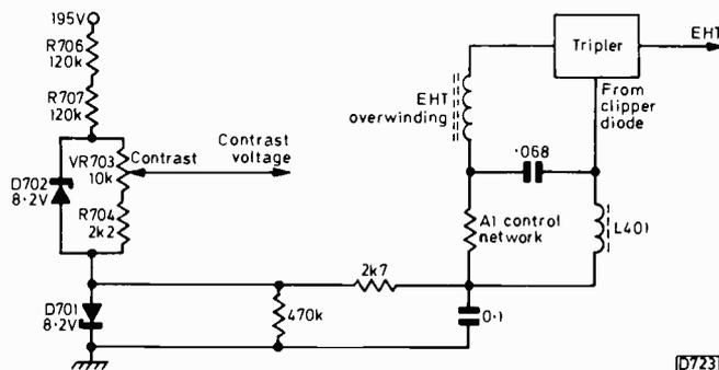
Fig. 6: Use of a zener diode for beam sensing in the Decca 70 series chassis.
