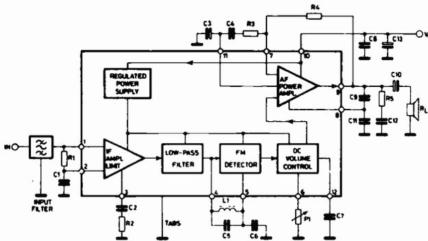
Fig. 1: Functional block diagram of the TDA1190Z with peripheral components.
