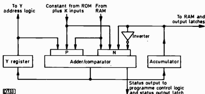
Fig. 5: The arithmetic logic unit's inputs and outputs.
