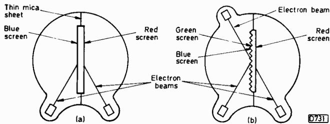
Fig. 2: The basic principles of Baird's Telechrome colour display tube, which he patented in 1940 and demonstrated to the press in 1941. (a) Arrangement of the phosphor coatings for a two-colour version. (b) Use of a rigid back to the screen to provide two surfaces for a three-colour system.
