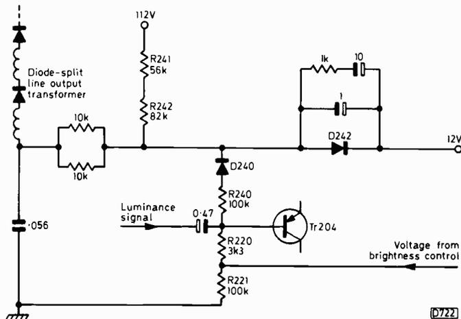
Fig. 5: Circuit used in the Rank-Toshiba T24E chassis.
