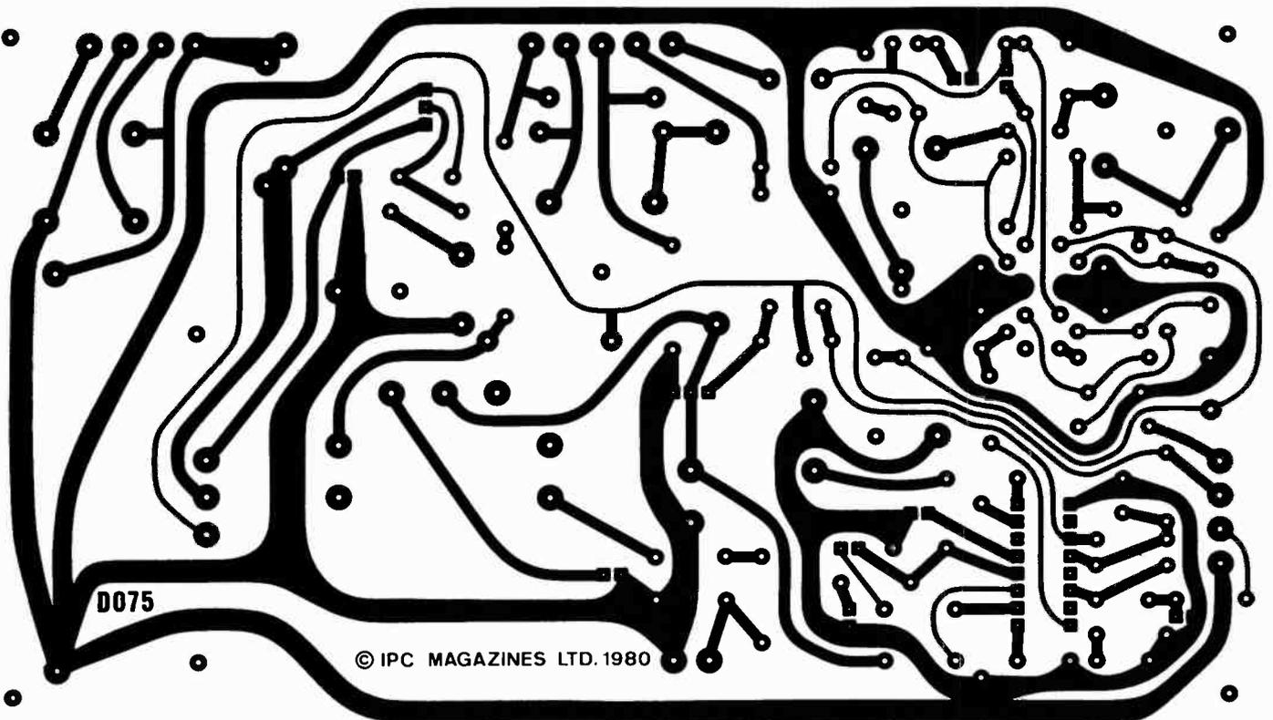
Fig. 3: Track pattern, timebase/power supply board. The overall board size is  $7\frac{3}{8} \times 4\frac{1}{4}$  in.
