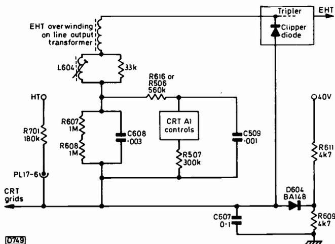
Fig. 1: CRT first anode supply and beam limiting circuits, GEC C2110 series. The factory preset L604 provides fifth harmonic tuning. Several resistors in this area can cause problems. R506/616 (depending on which board it's mounted on) going high in value reduces the brightness, as does R701 since the beam limiter then operates at a lower beam current level. R607/8 can fall in value quite dramatically, producing smoke and fuse blowing.
