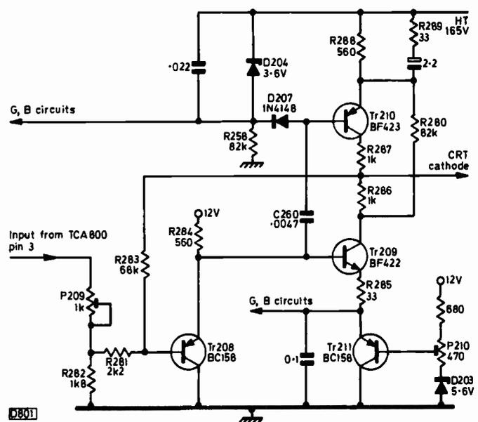
Fig. 4: A practical example of the complementary-symmetry class AB video output stage, as used in the GEC C2201H, C2217H and similar models (decoder panel PC719). P210 forms an output bias control, and is set for a reading of 150V d.c. at the output. A simplified circuit using BF469 and BF470 transistors is employed in the later GEC chassis with PIL tube (panel PC786/7).
