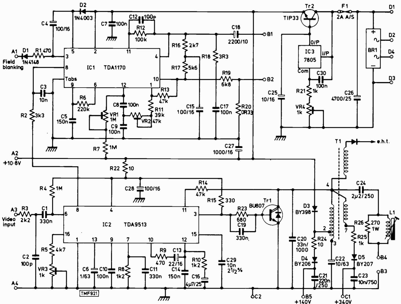
Fig. 1: Circuit diagram of the timebase/power supply board.
