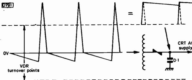
Fig. 5: Using a VDR to rectify an asymmetrical waveform – the line scan/flyback waveform. The VDR hardly conducts in the area between the dotted lines, but passes the positive-going spikes above its turnover point.
