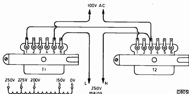
Fig. 2: Method of obtaining a 100V a.c. mains supply using two autotransformers from the Thorn 900/950 chassis. Note that the pinning of some transformers differs.
