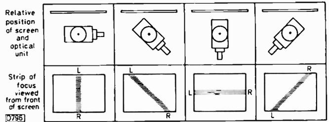
Fig. 3: Focusing chart for projection TV sets.
