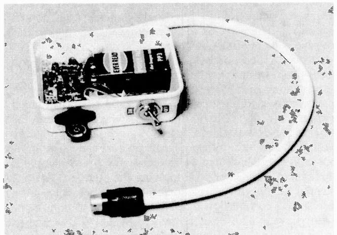
View of the Electronic Mailorder B45/High Gain preamplifier with the snap-on top cover removed.
