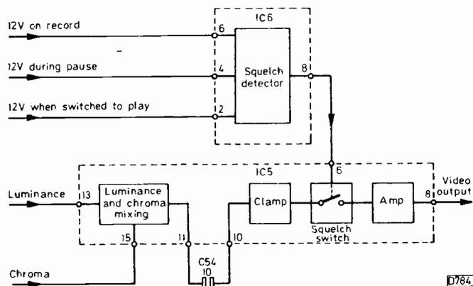
Fig. 1: Block diagram of the video muting system used in the JVC HR3300 videocassette recorder.
