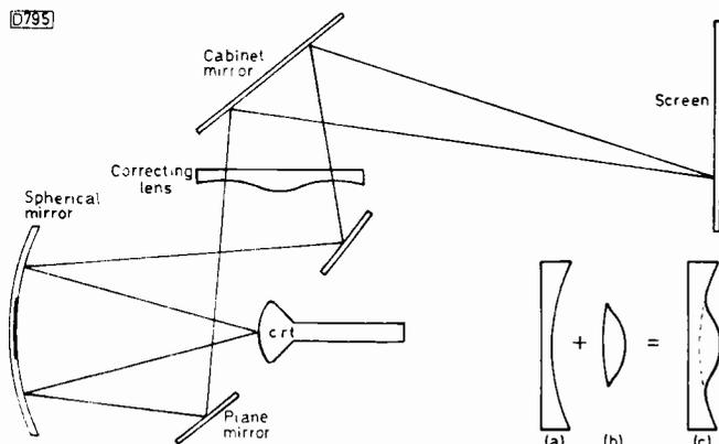
Fig. 1: Arrangement of the Schmidt "folded" optical system used in projection TV systems. The c.r.t. was a 2½in. one produced by Mullard (type MW6-2).
