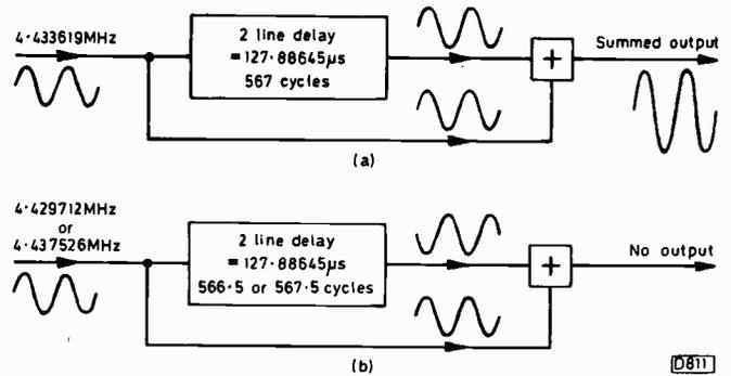
Fig. 9: Delay line system used in Sony Betamax machines. (a) Wanted chroma signals add. (b) Unwanted chroma crosstalk signals cancel. The head A replay intermediate frequency is 5.119165MHz, so the head B crosstalk is 5.119165 - 0.689453 = 4.429712MHz. The head B replay intermediate frequency is 5.123072MHz, the head A crosstalk being 5.123072 - 0.685546 = 4.437526MHz.
