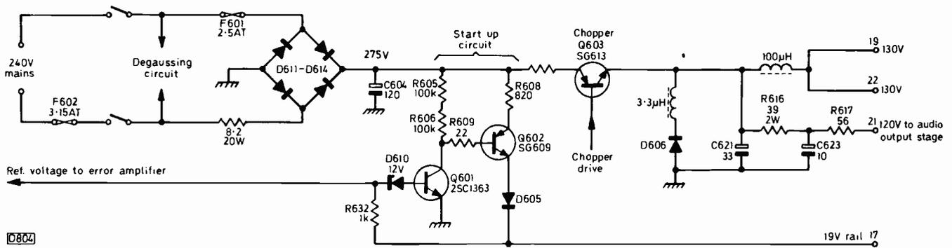
Fig. 1: Simplified circuit showing the mains input, chopper, start-up and h.t. filter circuits in the Sony Model KV1810UB Mk. II. Once the set starts up, the 19V supply is derived from the line output stage.
