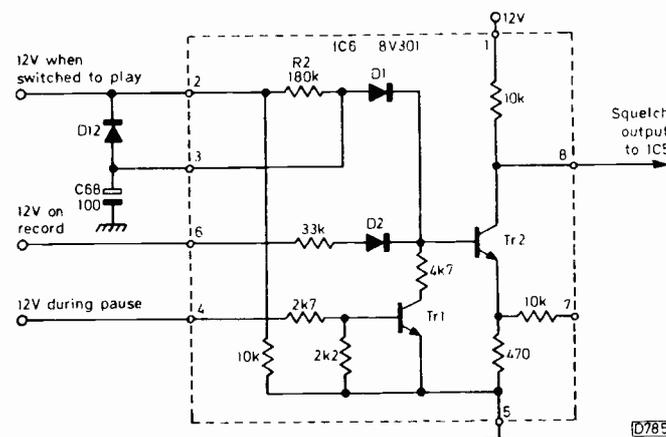
Fig. 2: The squelch detector circuit.
