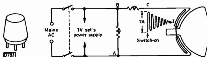
Fig. 7: The action of the dual-posistor degaussing circuit.
