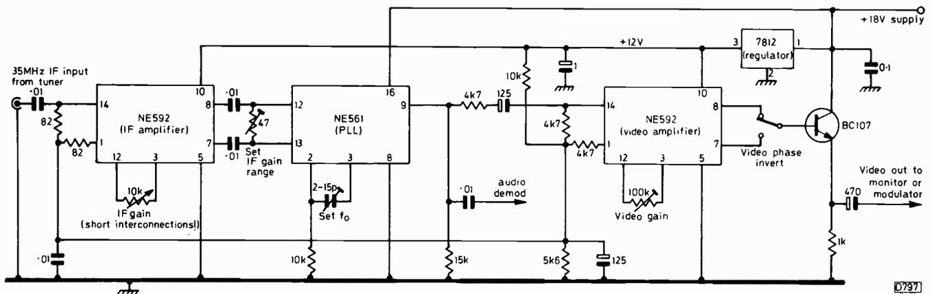
Fig. 1: Steve Birkill's i.f. strip for satellite TV reception. A phase-locked loop is used to demodulate the f.m. video.
