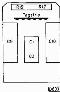
Fig. 3 (above): Layout of the power resistor/main electrolytic plate, which is at the bottom centre of the chassis.
