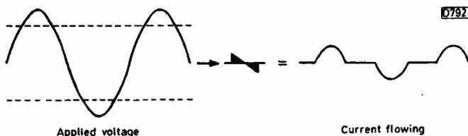
Fig. 6: A VDR will distort a current waveform by conducting on only the voltage peaks.
