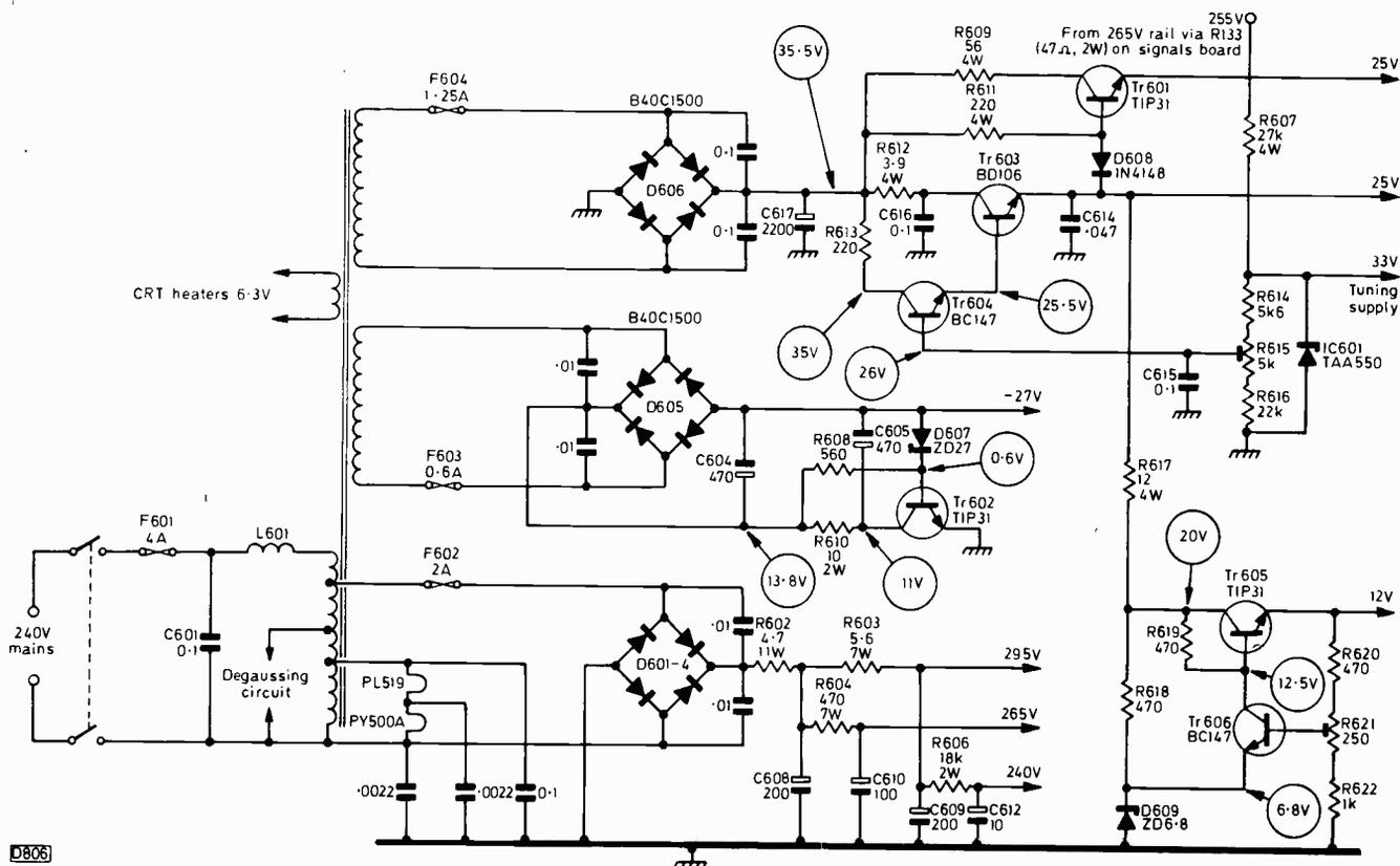
Fig. 1: The power supply circuits in the Kuba Florence.
