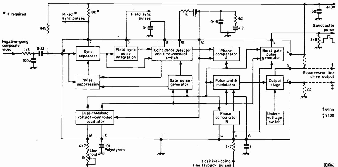
Fig. 4: Block diagram of the TDA9400/9500 series line processor i.c.
