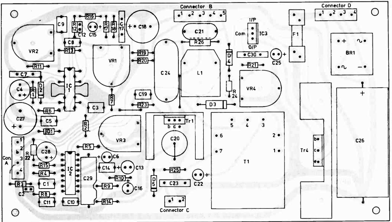
Fig. 2: Component layout, timebase/power supply board. The board is slightly larger than shown here.
