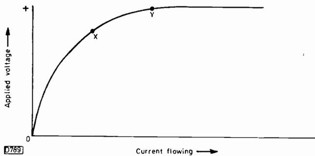
Fig. 3: Voltage-dependent resistor characteristic. At point X (the turnover point) the current begins to increase significantly. At point Y the voltage is virtually clamped to a fixed value – given in data books as the point at which the resistance falls to about a fifth of the cold value.
