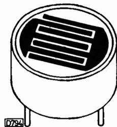
Some continental sets use these devices as opto-isolators to transfer an a.g.c. or a.f.c. voltage from its generating source on a d.c. pedestal to a tuner. The control voltage modulates a LED, which alters the resistance of the LDR. There are now better ways of doing this.
