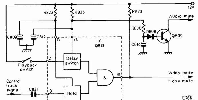
Fig. 3: The signal muting circuit used in the Sanyo VTC9300P, a Betamax format VCR.
