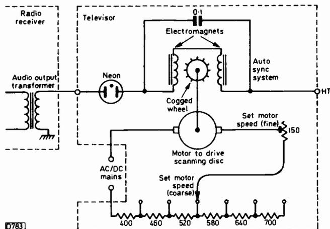
Fig. 1: Circuit diagram of the world's first commercially produced TV receiver – the Baird Televisor.
