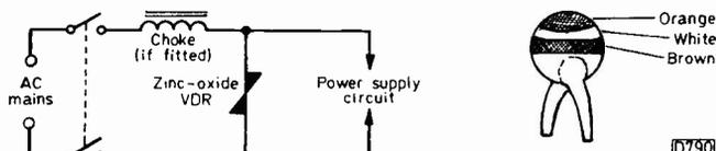
Fig. 4: Using a zinc oxide VDR to provide protection against mains surges. The device conducts only on mains spikes over 300V, protecting the set against fuse blowing etc. If the set incorporates an anti-radiation choke, this should be on the mains side of the VDR.
