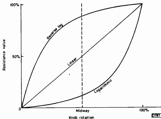
Fig. 1: Variable resistor tracking laws.
