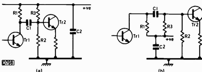
Fig. 1: (a) A.C. coupling between stages by means of an RC network. Note that from a d.c. point of view R2 and R3 are connected in series. (b) Circuit redrawn to bring out the a.c. conditions. From the a.c. point of view, R1, R2, R3 and the input impedance of Tr2 are all in parallel (with C2 in series with R1 and R3).
