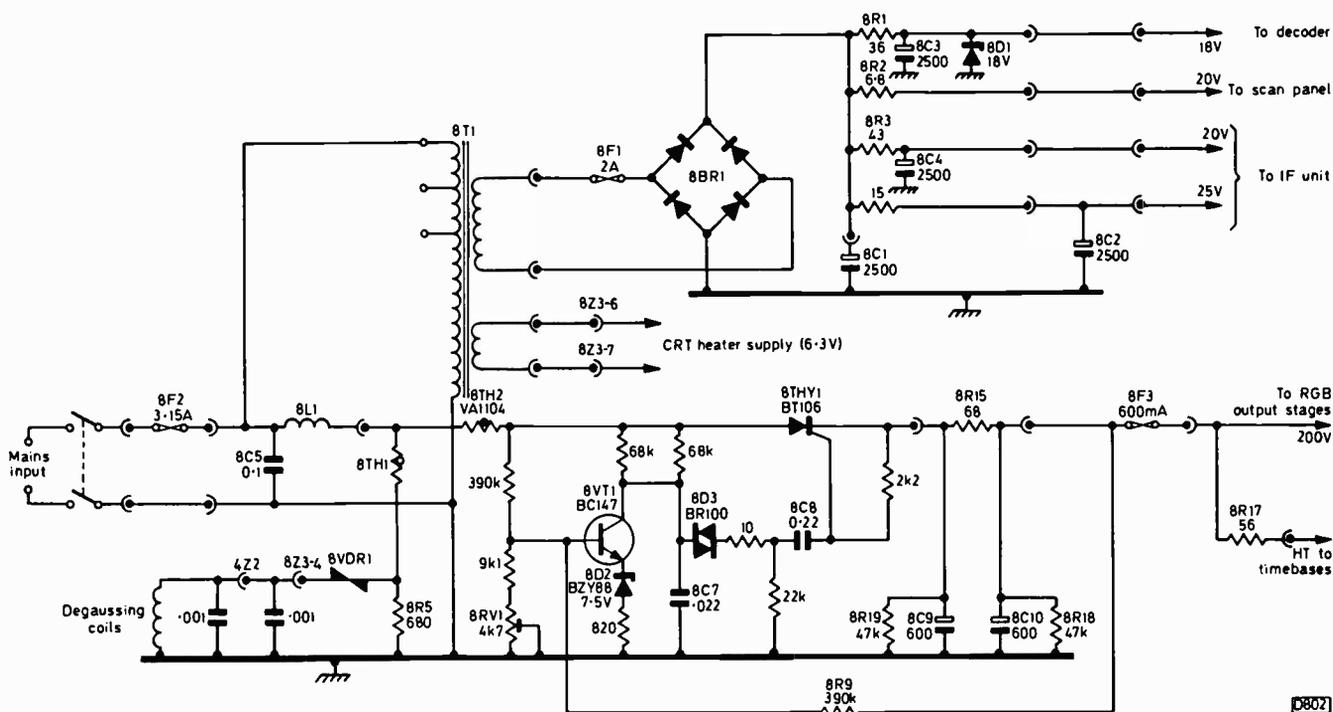
Fig. 1: Power supply circuitry, Rank A823 chassis. Note that there were several minor modifications to this circuit.
