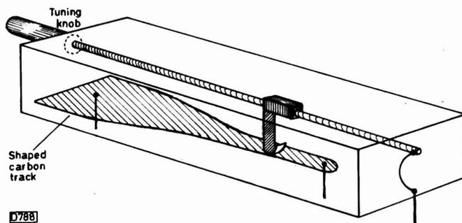
Fig. 2: A special tracking law, neither logarithmic nor linear but in between, is required for the multiturn potentiometers used to tune varicap tuners.
