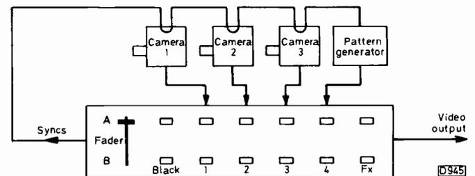
Fig. 1: Fader, switches and general arrangement of the inputs. Position 4 can be used for a pattern generator or a fourth camera.
