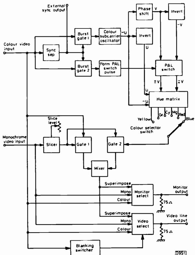
Fig. 2: Simplified block diagram of the Sony HVS2000P effects unit, which also provides regulated power supplies for the two cameras.
