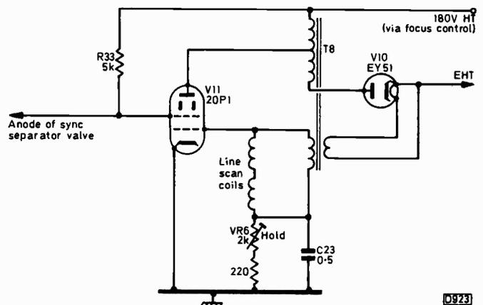
Fig. 1: The single valve line timebase used in the Baird Everyman. In addition to driving the scan coils, the secondary winding on the line output transformer T8 provides feedback to the 20P1's control grid. The self-oscillating circuit was synchronised by applying the line sync pulses to the valve's screen grid. There was no efficiency diode in this early form of line timebase, the output valve conducting throughout the scan while the flyback energy was dissipated as heat.
