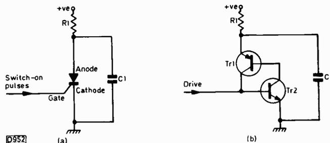
Fig. 1: Analogy between a thyristor (a) and a complementary transistor switch (b). Both operate in the same manner, the thyristor acting like a pair of pnp/npn transistors with their bases and collectors d.c. coupled. The discrete transistor circuit gives greater flexibility in application.
