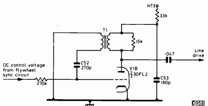
Fig. 1: The line blocking oscillator circuit used in the Thorn 1500 chassis. The weak spot here is the charging capacitor C53, which can cause intermittent line tearing when leaky.
