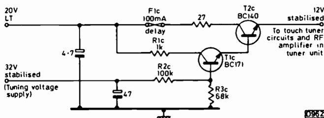
Fig. 1: The 12V stabiliser circuit on the Feathertouch tuning panel used in some versions of the ITT CVC9 chassis. When F1c goes open-circuit there's still some voltage on the 12V rail, via R1c, T1c and the base-emitter junction of the series regulator transistor T2c. This can cause misleading symptoms. There are two fuses with the reference number F1c in these sets, the other one being the mains fuse.
