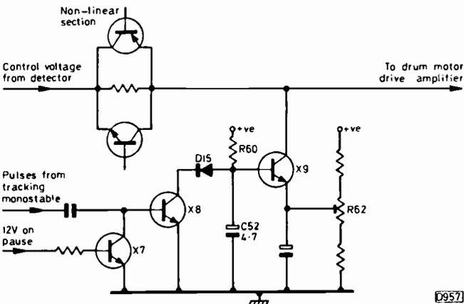
Fig. 1: Part of the pause circuit in the JVC portable Model HR4100. During a pause transistor X9 switches on, clamping the drum servo voltage at the level set by R62.
