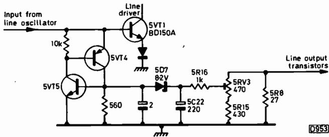
Fig. 2: Use of a complementary transistor switch circuit as an overload trip in the Rank Z718 chassis. In the event of excessive current being drawn by the line output stage, the trip operates to remove the input to the line driver stage.
