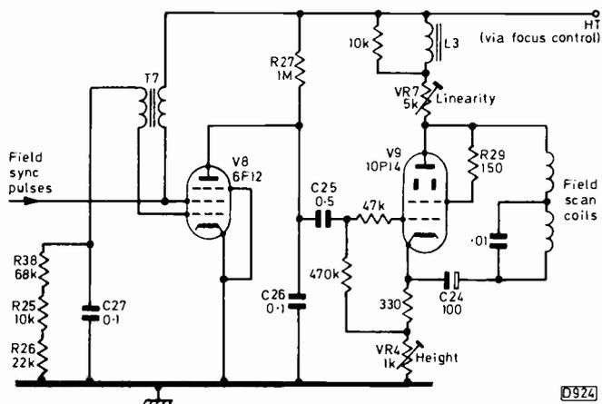
Fig. 2: The Baird Everyman's field timebase circuit. The network R38/25/26 forms a fixed field hold control, resistors being shorted out as required. The output valve is operated as a triode, with the scan coils a.c. coupled via C24.
