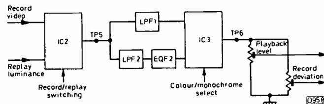
Fig. 2: Luminance signal path in the JVC Models HR3330 and HR3660.
