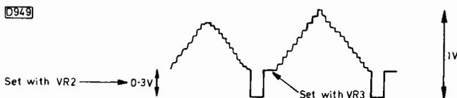
Fig. 5: Setting up the sync and black level controls.
