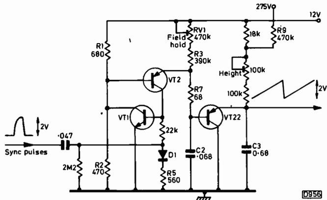
Fig. 5: Use of a complementary transistor switch (VT1/2) as the field oscillator in the Rank Z718 chassis. The circuit is timed by C2 in conjunction with RV1 and R3. The field sawtooth is generated in the following stage, as C3 charges from the 275V h.t. rail via R9 and the height control etc.
