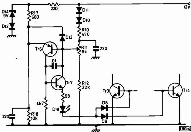
Fig. 3: The complementary transistor switch circuit Tr6/7 in the Panasonic Model TC333G 13in. battery/mains colour portable comes into operation when the voltage from the battery falls to a low level.
