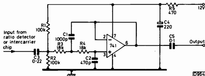
Fig. 2: Practical circuit, using a 741 i.c. The filter components R3/C1/R4/C2 give a corner frequency of 12.6kHz. If the impedance being fed is less than 50kΩ, the value of C5 should be increased to 4.7µF.
