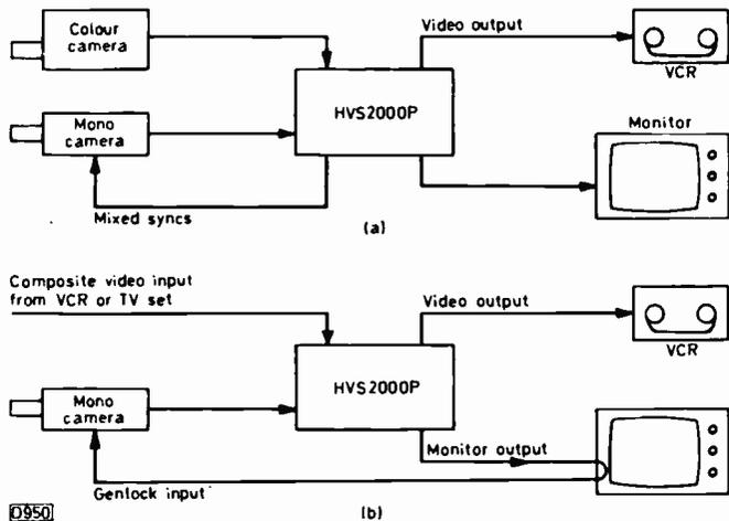
Fig. 1: Using the Sony HVS2000P effects unit. (a) Normal use. (b) Alternative ways of using the unit.
