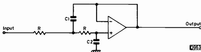
Fig. 1: Two-pole active low-pass filter, using an operational amplifier i.c.
