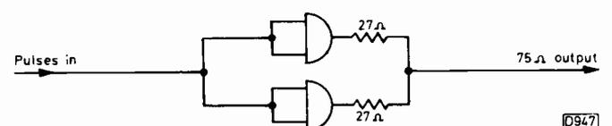
Fig. 3: Use of extra gates to obtain 75Ω outputs.
