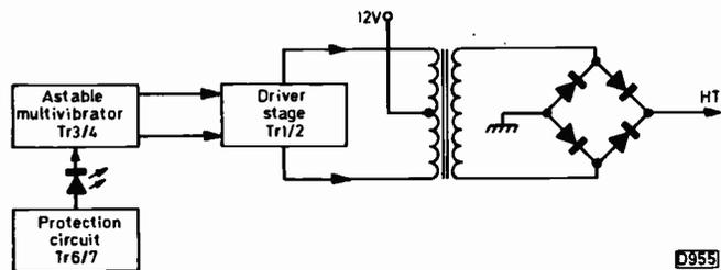
Fig. 4: Block diagram of the battery power supply arrangement used in the Panasonic Model TC333G. In the event of the 12V battery voltage falling to a low level, the protection circuit shuts down the multivibrator oscillator.
