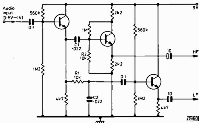
Fig. 1: Pseudo-stereo sound filter circuit – C1/R2 and R1/C2 filter out the h.f. and l.f. components of the sound.
