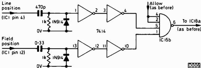
Fig. 9: Modified circuitry giving a movable spot.
