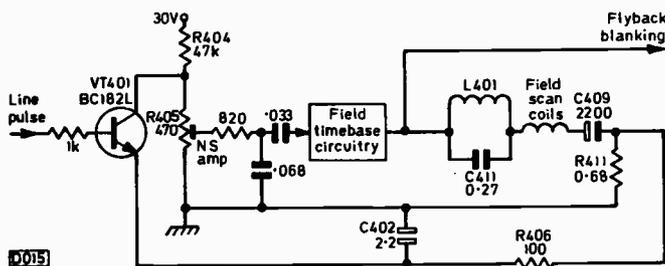
Fig. 5: Simplified circuit showing the way in which NS raster correction is carried out in the Thorn 4000 chassis. The signal developed across R411 is also used as feedback in the field timebase and is fed to the convergence circuits.
