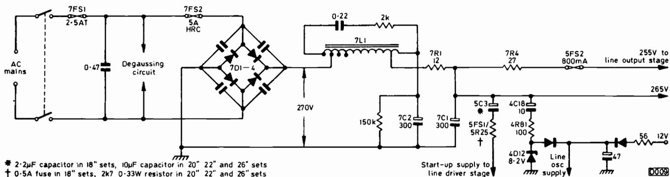
Fig. 2: The mains input, h.t. and start-up circuits used in the Rank Z718 solid-state colour chassis. The mains bridge rectifier 7D1-4 produces the h.t. supply, stabilisation being carried out via the EW modulator circuit.
