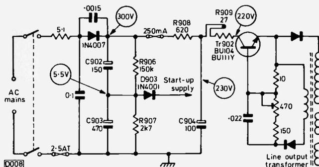
Fig. 1: Power supply arrangements used in the Indesit T12LGB monochrome portable, showing the mains input and rectifier, the start-up circuit and the pump transistor Tr902.
