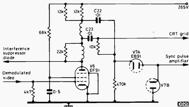
Fig. 1: The video output and diode sync separator stages used in the CN370.
