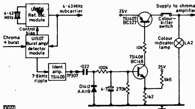
Fig. 1: Ident/colour-killer arrangement used in the Philips N1500 VCR.
