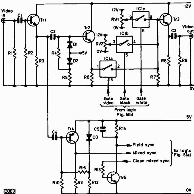
Fig. 6: Circuitry on the video board.
