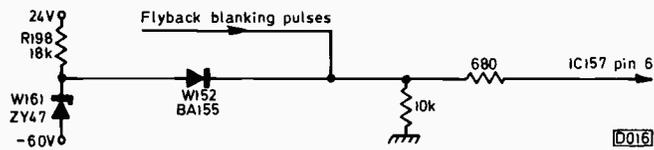
Fig. 6: Circuit used to provide tube protection in the event of line output stage failure. The anode of diode W152 is reverse biased by the network R198/W161, which is connected between 24V and -60V supplies. Since the -60V supply is obtained from the line output transformer, via a voltage doubler circuit, failure of the line output stage will remove this supply. W152 will then be forward biased via R198 and a positive voltage will appear at pin 6 of IC157, removing the c.r.t. drive signals.
