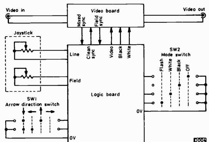
Fig. 7: Interconnections between the video and logic boards.
