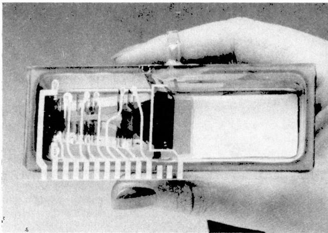
One of the Sinclair flat-screen tubes produced on the pilot production line at St. Ives, Cambridgeshire.
