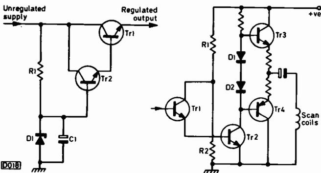
Fig. 1 (left): Darlington pair of transistors in a simple voltage regulator circuit without feedback. The output is stabilised at 1.4V less than the voltage, set by zener diode D1, at the base of Tr1. The circuit acts as an active filter, since the value of C1 is much less than would otherwise be necessary to provide smoothing.
