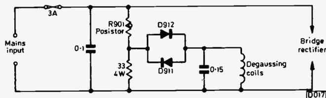
Fig. 1: Degaussing circuit used in the Electrohome monitor.
