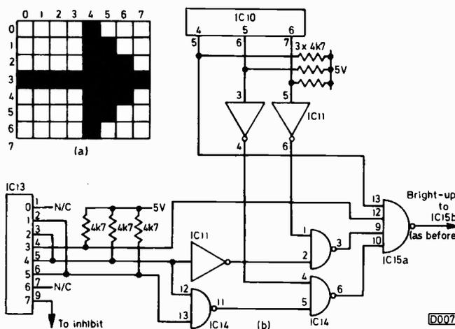
Fig. 10: Decoding circuit for an arrow with a closed head.
