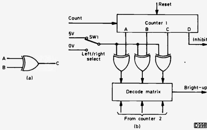
Fig. 3 (above): (a) NEV gate symbol. (b) Modification to the basic system to give left/right pointing arrows.
