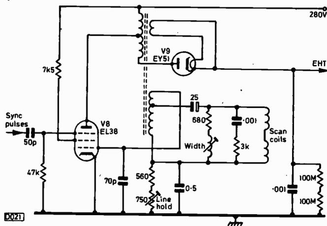
Fig. 2: The single-valve (plus e.h.t. rectifier) line timebase circuit used in the CN390 series.
