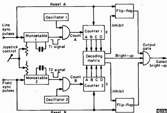
Fig. 2: Simplified diagram showing the logic required to produce a right-pointing arrow.
