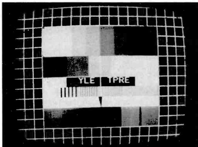
Fubk test pattern used by Finland, with Tampere identification (ch. E2). Photo from Petri Pöppönen.
