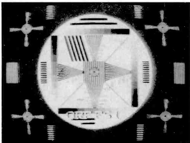
The Telefunken T05 test card used by ORF (Austria). Received on ch. E2a by Andrew Tett (Caversham) using a 7ft. dipole!
