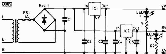
Fig. 8: Power supply circuit.
