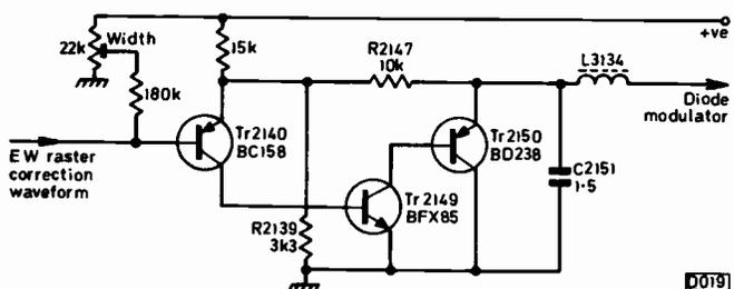
Fig. 3: A triple Darlington configuration, with pnp and npn transistors, used to provide the EW modulator drive with a 20AX tube (Philips G11 chassis).
