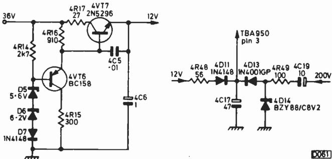
Fig. 4 (left): The 12V regulator circuit.
