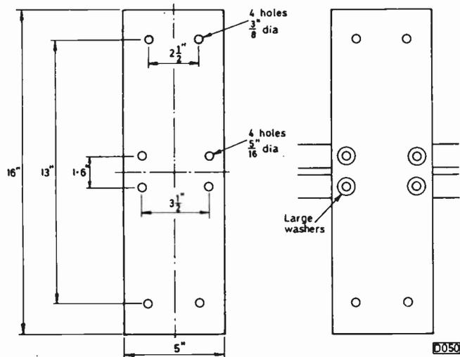
Fig. 5: Centre support/mounting plate.
