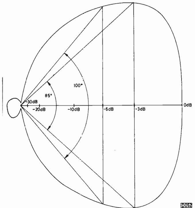
Fig. 7: Polar response at 94.9MHz.
