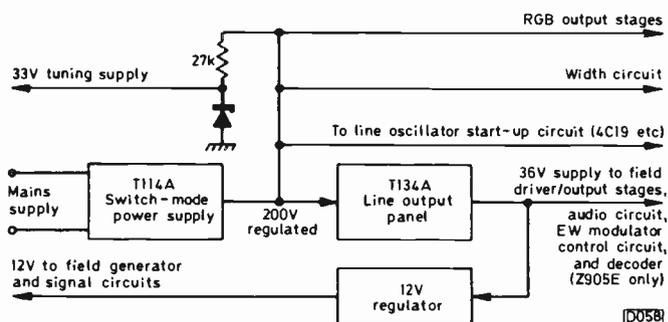
Fig. 1: Power supply arrangements, Rank T20/T22 chassis.
