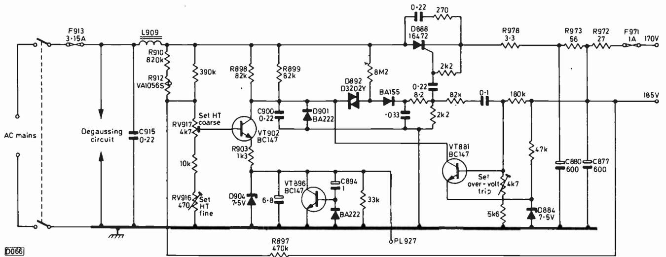
Fig. 3: Regulated power supply circuit used in the Pye 725 etc. chassis. If the zener diodes need to be replaced, use type BZX79C7V5. To reduce drift and improve the regulation, the following modifications were introduced in late production: R898/899 changed to 56k $\Omega$ , 1W; R910/R912 deleted; R897 changed to 330k $\Omega$  and R903 to 680 $\Omega$ ; an 82k $\Omega$ , 1W resistor (R929) added between the collector of VT896 and the cathode of the thyristor D888.
