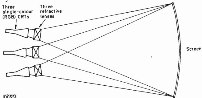
Fig. 3: Use of three tubes with refractive lenses.
