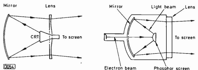
Fig. 1 (left): The basic Schmidt optical system.
