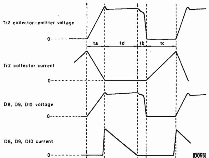
Fig. 1: Self-oscillating switch-mode power supply waveforms.
