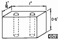
Fig. 4 (right): Boom shorting block.
