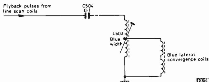
Fig. 1: The blue lateral convergence circuit used in the Thorn 9800 chassis.
