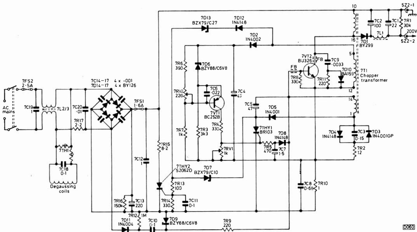
Fig. 1: Circuit of the self-oscillating switch-mode power supply (type T114A).
