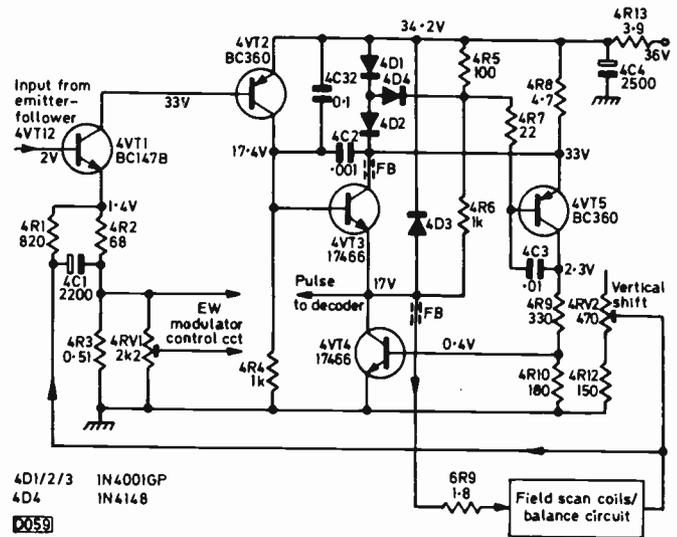
Fig. 2: field driver and output stage circuit.
