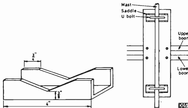
Fig. 6: Method of clamping the aerial to the mast.
