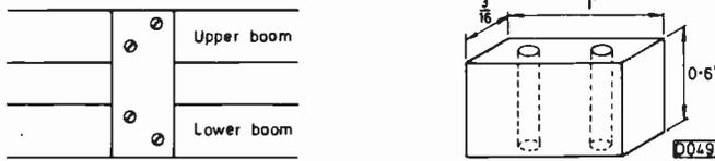
Fig. 3 (left): Boom spacing, with pieces of Paxolin at each side, towards the front and back of the aerial.
