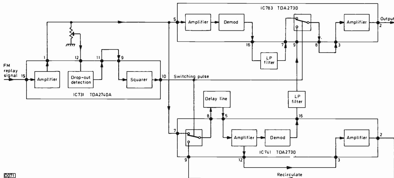
Fig. 1: The luminance playback/drop-out compensation system used in the Grundig 2 x 4 VCR. When a drop-out occurs, the f.m. playback signal envelope collapses. This is detected by IC731, which produces a switching signal at pin 10 to operate the electronic switches in IC783 and IC741. As a result, the signal is obtained from the 64µ sec delay line. In the event of a sustained drop-out (longer than one line), the signal is recirculated via pins 12, 3, 2, 9 and 8 of IC741.
