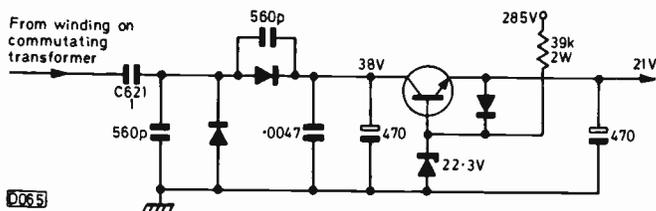
Fig. 2: 21V regulator circuit, Grundig 5010/6010 series.
