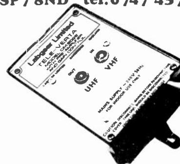
The Labgear CM6022/RA 'Televerta' is a wideband 40-220MHz VHF to UHF up-converter intended for use on relay systems (VHF) or for VHF coverage with a UHF only TV receiver. The 'Televerta' – which needs no tuning – enjoys considerable popularity with TVDXers.
