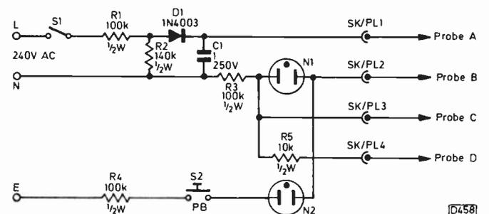
Fig. 1: Modified capacitor tester circuit.
