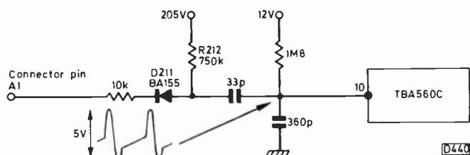
Fig. 1: Burst gating/black-level clamping pulse delay circuit used in later versions of the Philips G8 chassis.
