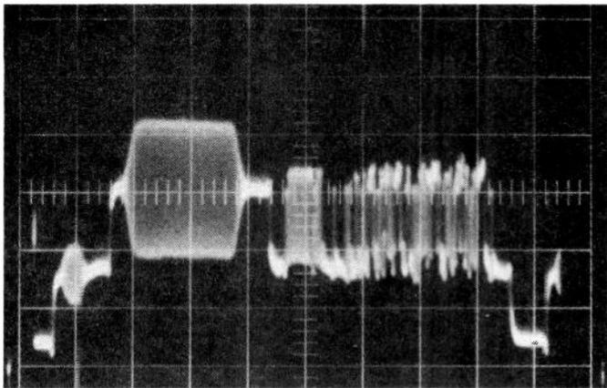
Fig. 2: BBC line 20, the second half of which provides a teletext eyeheight display.
