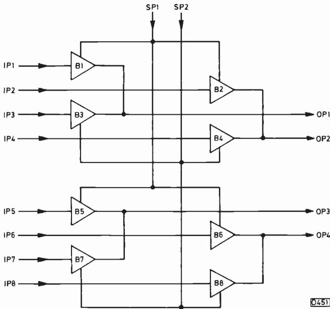
Fig. 6: Multiplexing system using bus buffers.
