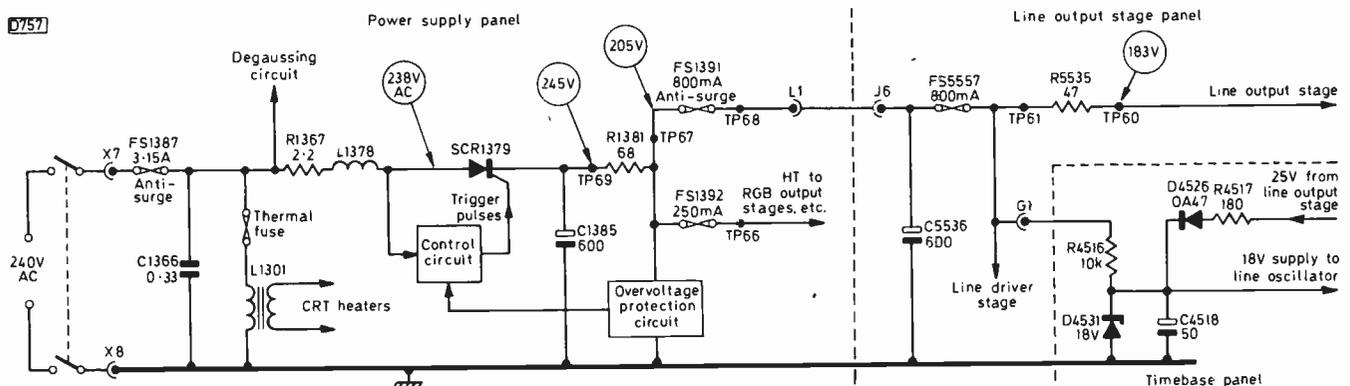
Fig. 1: H.T. supply arrangements used in the Philips G8 chassis.
