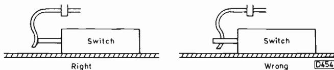
Fig. 53: Audio switch actuator arrangement.
