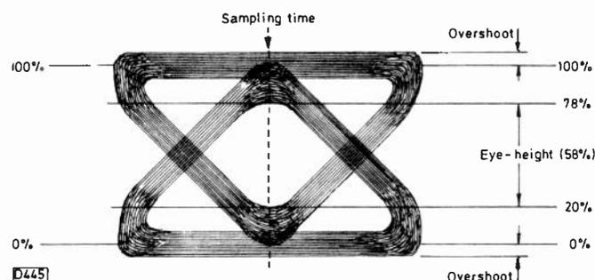
Fig. 1: A typical eyeheight display. The individual ellipses represent separate 0 and 1 pulses and are overlaid to give average and worst-case conditions.
