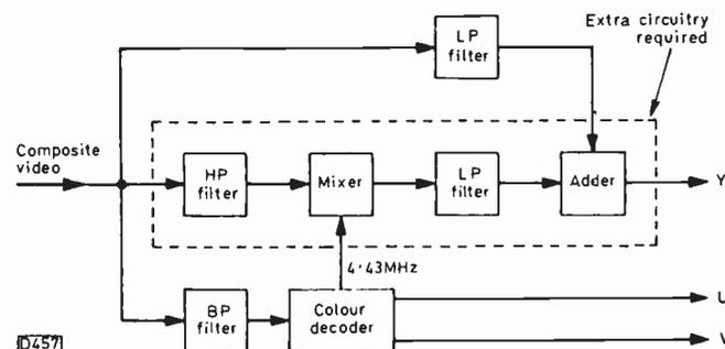
Fig. 2: Decoder arrangement for extended PAL reception.
