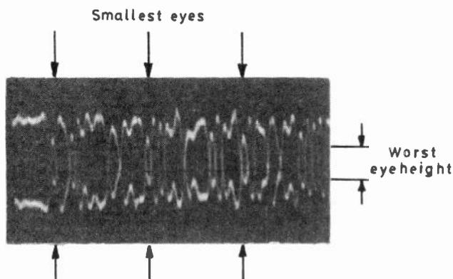
Fig. 4: An expanded portion of the trace shown in Fig. 3, with examples of worst eyeheight arrowed.
