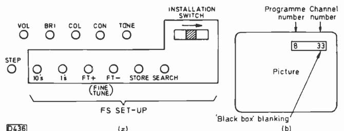
Fig. 2: Layout of the tuning and other controls behind the bottom flap (a); on-screen display (b).
