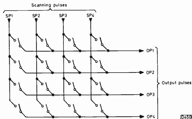
tions from the user (keyboard scanning) usually takes the form shown in Fig. 5. The microcomputer continually generates scanning pulses each of which lasts from about
