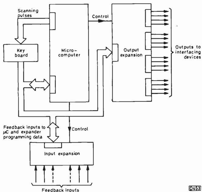
Fig. 8: Block diagram of a microcomputer VCR control system.
