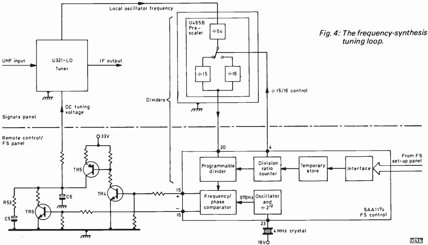
Fig. 4: The frequency-synthesis tuning loop.
