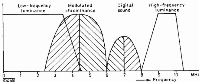
Fig. 1: Extended PAL signal spectrum.
