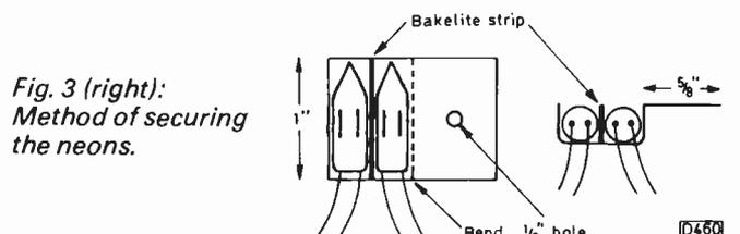
Fig. 3 (right): Method of securing the neons.
