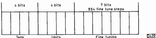
Fig. 6: The coding system used for holding channel information in the stores. Note that a four-bit system has sixteen possible states: only the first ten are used.
