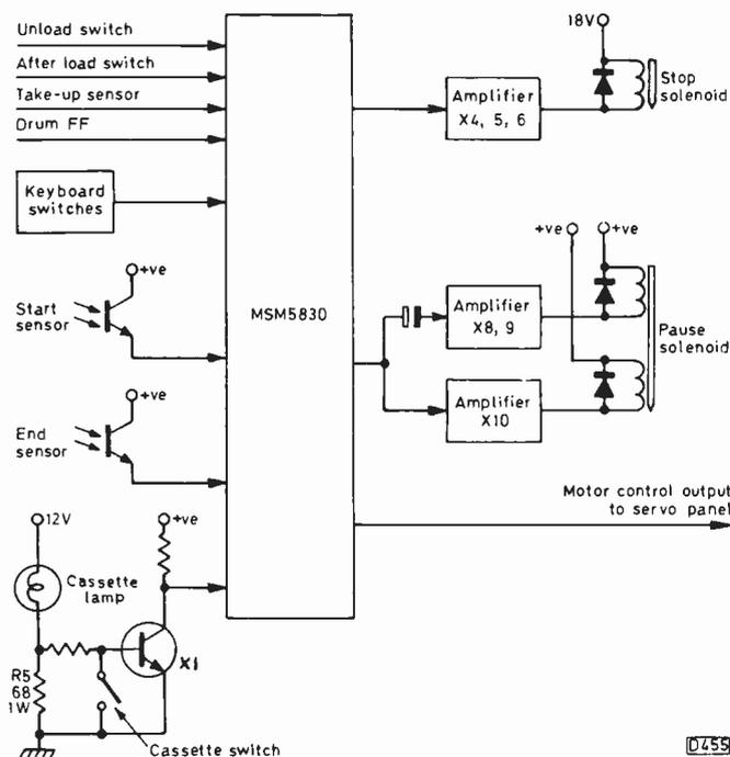
Fig. 54: The mechanism control system.
