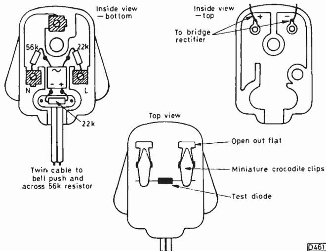
Fig. 4: Constructional details of the zener diode checker.
