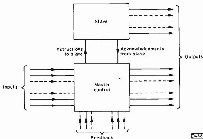
Fig. 3: Master/slave control arrangement.
