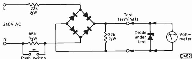
Fig. 5: Zener diode checker circuit.
