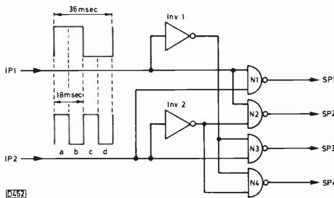
Fig. 7: Keyboard scanning economy arrangement used in the Philips VR2020 VCR.
