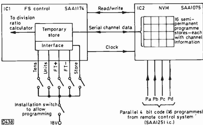
Fig. 5: Links between the FS control and non-volatile memory i.c.s.
