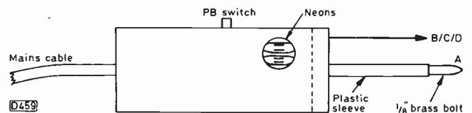
Fig. 2: Method of housing the capacitor tester.
