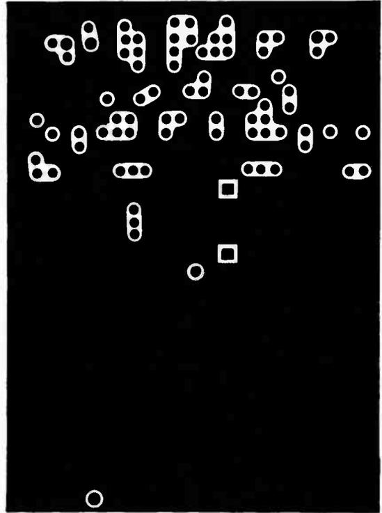
Fig. 4: Print pattern, component side.
