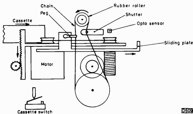
Fig. 76: Cassette housing, shown in the up position.
