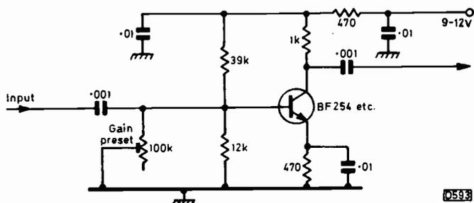
Fig. 1: Simple i.f. preamplifier circuit. A BF254, BF314 or equivalent transistor can be used.
