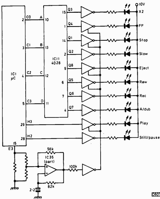
Fig. 74: Function LED drive circuit.
