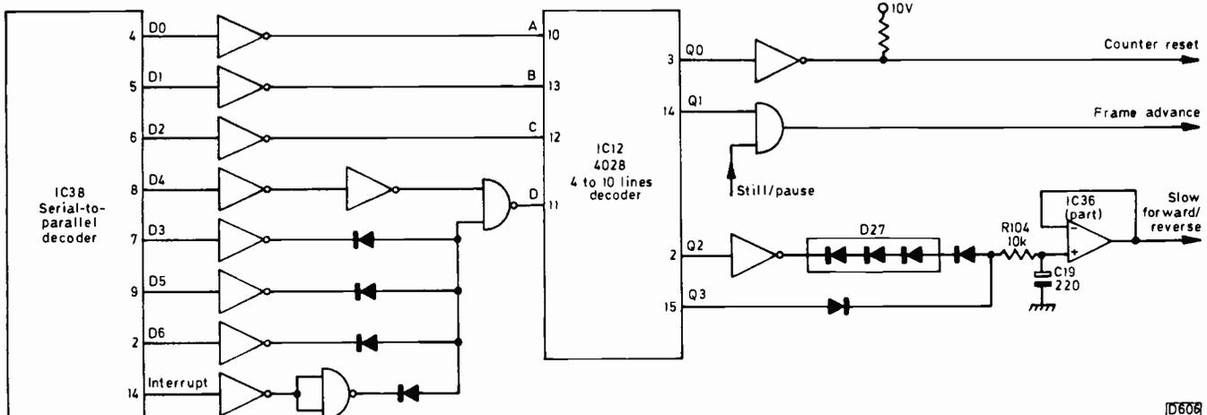
Fig. 73: Counter reset, frame advance and slow forward/reverse control.
