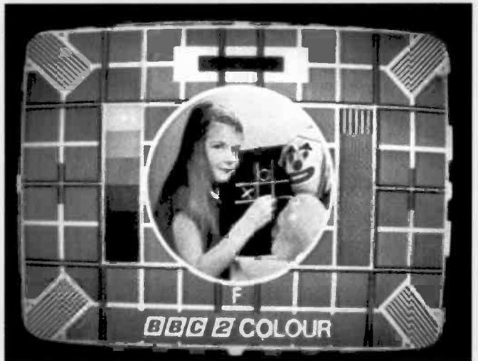
(10) Effect produced when the head preamplifier  $Q$  and resonance adjustments are incorrect.
