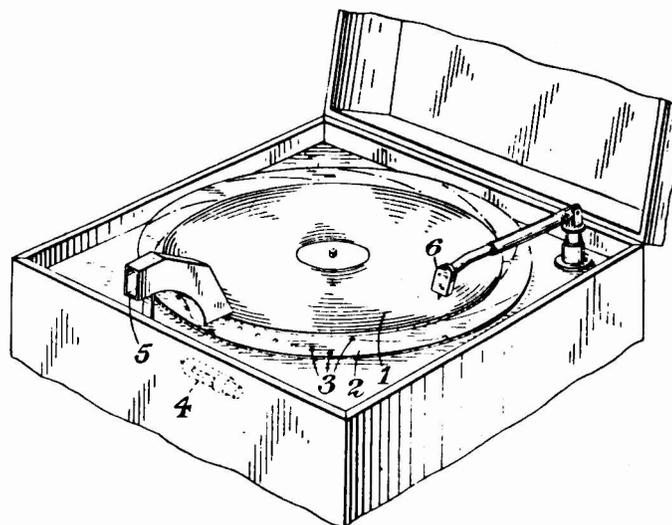
Fig. 2: Baird's 1928 idea for a combined disc player and television. (1) Disc. (2) Combined turntable/Nipkow disc. (3) Scanning holes. (4) Modulated neon light source. (5) Viewing lens. (6) Pick-up.
