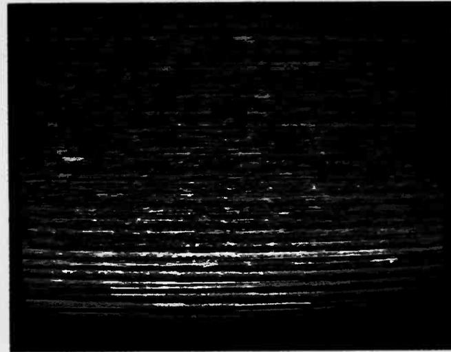
(16) When the drum speed is too far out the result is line slip as shown here.
