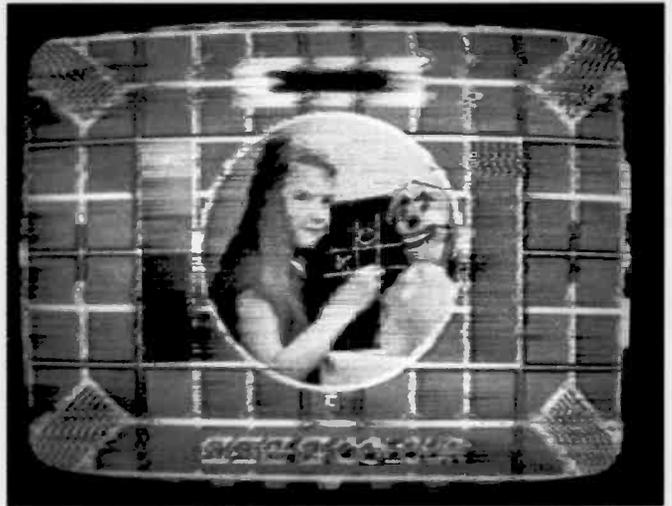
(8) If the limiting is inadequate or the f.m. is noisy the result is "spaghetti" as shown here.
