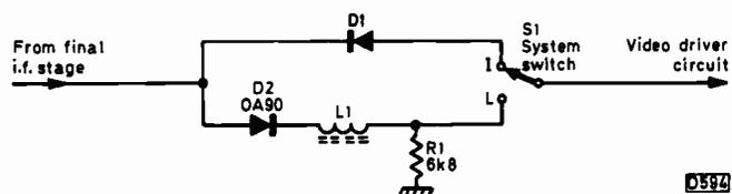
Fig. 2: Switched video detector circuit for the Thorn 1690 chassis.
