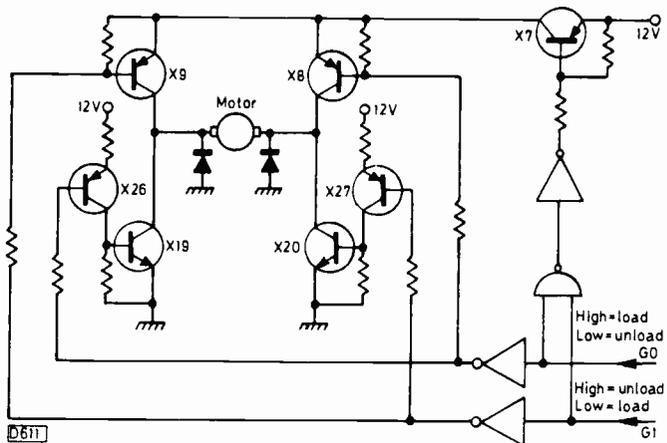
Fig. 78: Tape loading motor drive circuit.
