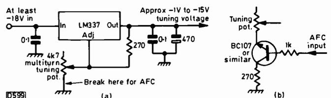
Fig. 2: (a) Method of obtaining a stable negative bias supply for tuning the microwave oscillator. (b) Method of applying a.f.c. to the bias supply.
