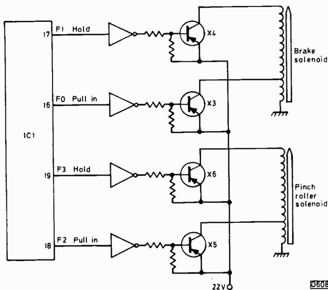
Fig. 75: Brake and pinch roller solenoid control.
