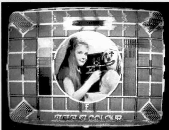
(11) Effect produced when the f.m. record current is excessive – noisy playback, possibly with spaghetti.
