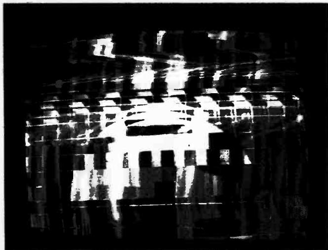
(3) The effect produced by minor drop-outs on a V2000 system machine.
