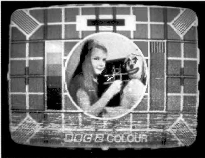
(7) Noise bar at the bottom of the picture due to a tape path fault on the take-up side.
