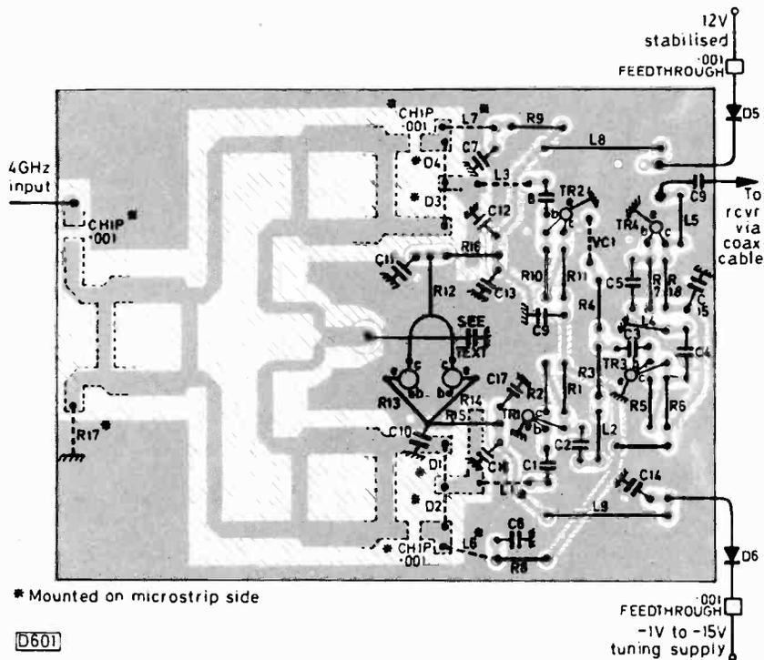
Fig. 5: Component layout. VC1 can be mounted on either side of the board.
