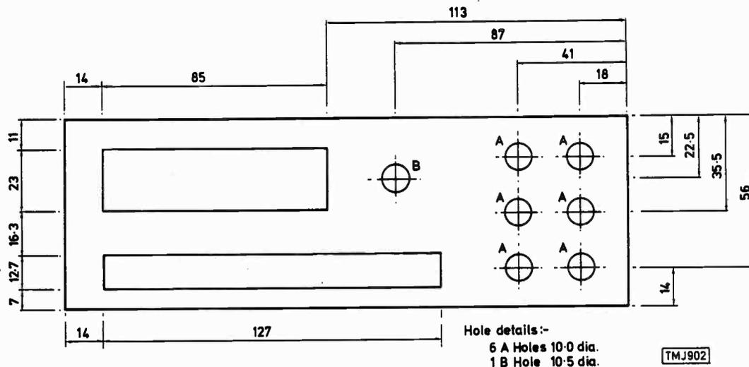
Fig. 8: Front panel cut-outs - dimensions in mm.
