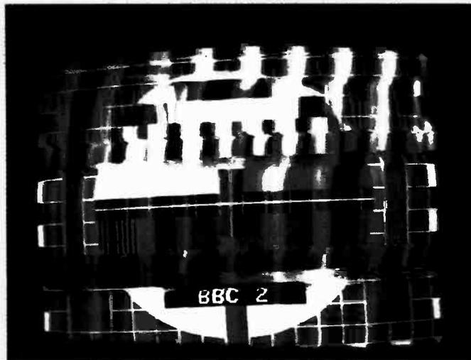
(4) Effect when the dynamic track following system is not working on fast search with a V2000 machine.
