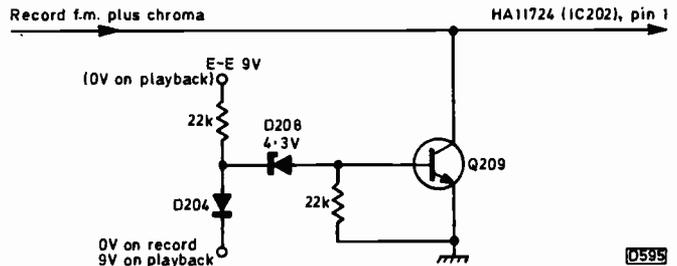
Fig. 1: Record signal muting circuit used in the Ferguson Model 3V29. The circuit is inoperative on playback.
