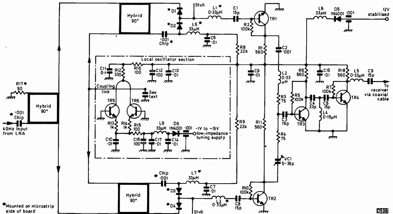
Fig. 1: Complete circuit of the converter.
