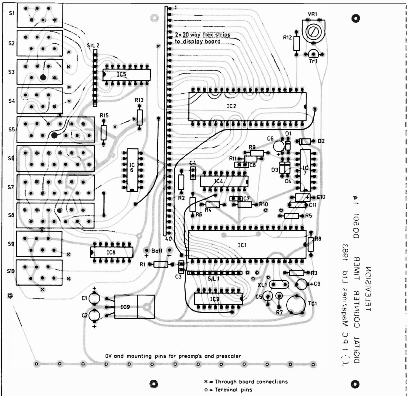
Fig. 7: Main panel component layout.
