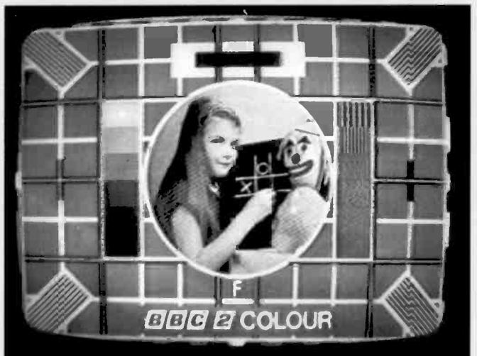
(12) Effect produced when the chroma record current is excessive – patterning, not excessive saturation.
