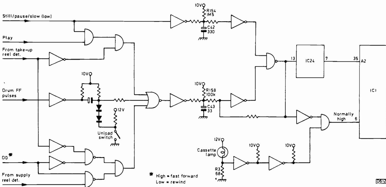
Fig. 79: The tape guard system.
