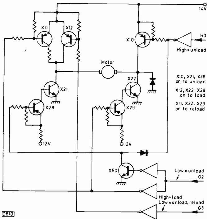
Fig. 77: Cassette loading motor drive circuit.
