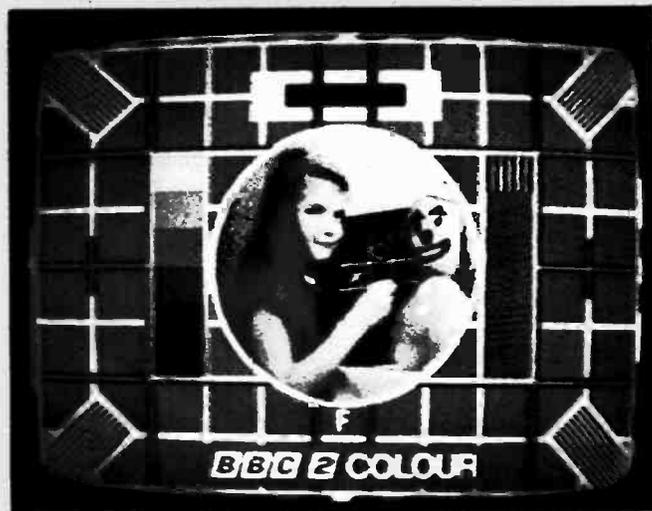
(15) Chroma displaced with respect to the luminance, due in this case to incorrect head phase control.
