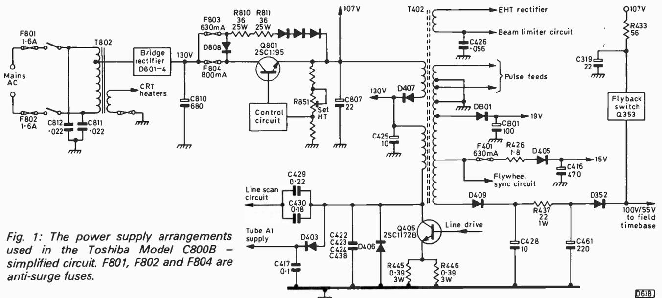
Fig. 1: The power supply arrangements used in the Toshiba Model C800B - simplified circuit. F801, F802 and F804 are anti-surge fuses.
