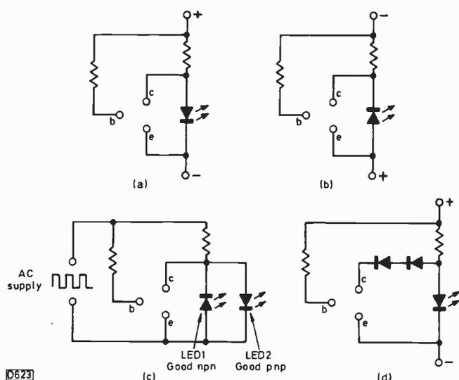
Fig. 1: Basic principles. (a) Arrangement for npn transistors. (b) Arrangement for pnp transistors. (c) Arrangement for testing both types automatically. (d) Addition of two diodes to ensure that only the low saturation voltage of a good transistor will extinguish the LED.
