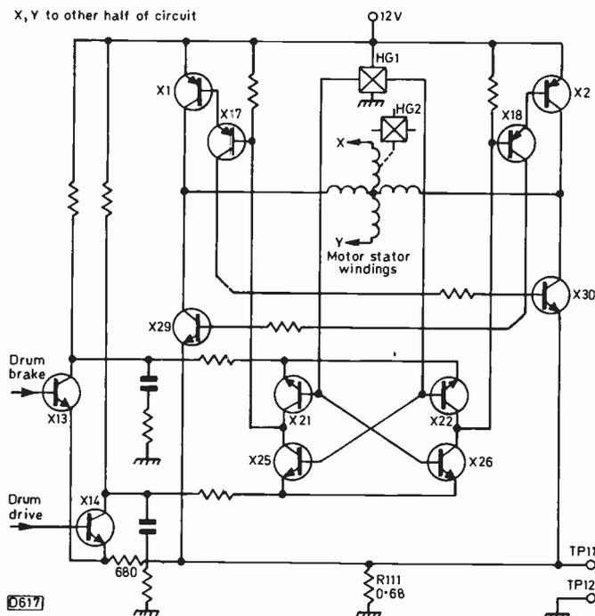
Fig. 84: Motor drive amplifier circuit.
