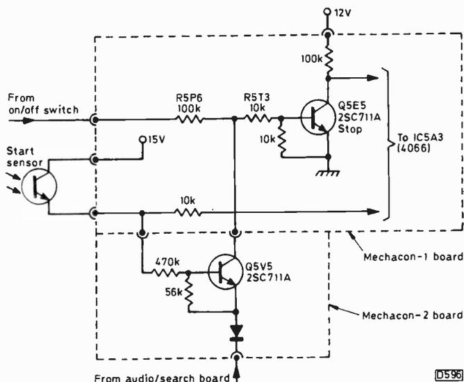
Fig. 2: Start sensor circuit, Mitsubishi HS300B.
