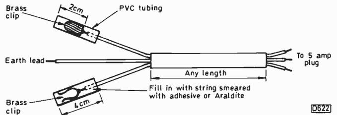
Fig. 2: DIY adaptor for converting a 13A plug for operation from a 5A socket.
