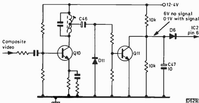
Fig. 1: Sound muting circuit, Ferguson 3V29.
