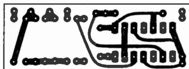
Fig. 3: Printed board layout - 1:1 scale.
