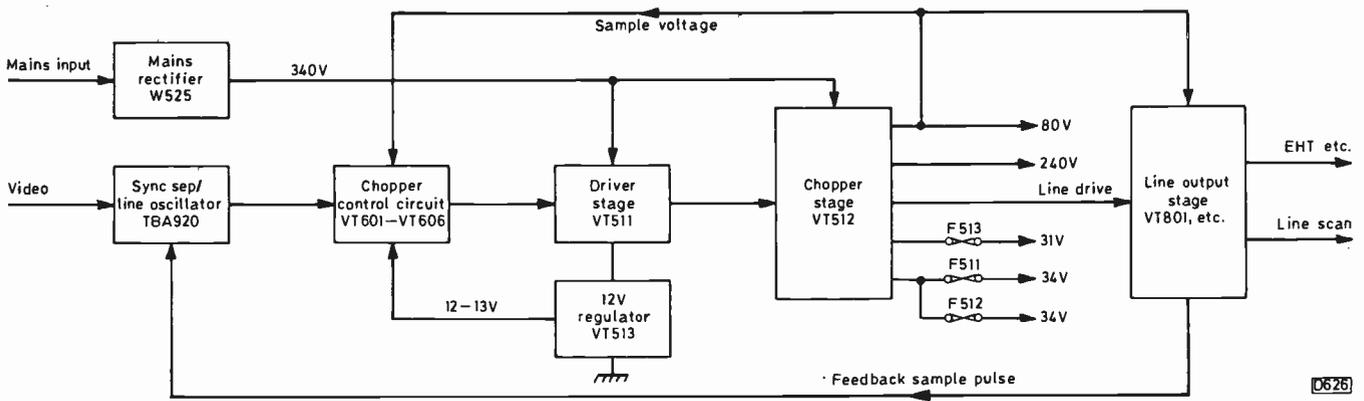
Fig. 1: Power supply/line timebase arrangement used in the Thorn 9600 chassis.
