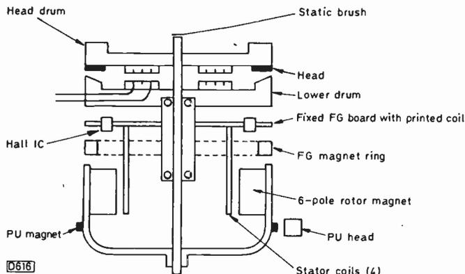
Fig. 83: The head drum/motor assembly.
