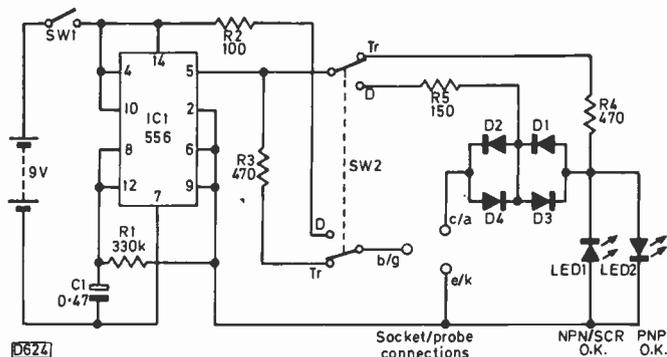
Fig. 2: Complete circuit. Diodes are tested by being connected across the collector-emitter terminals.
