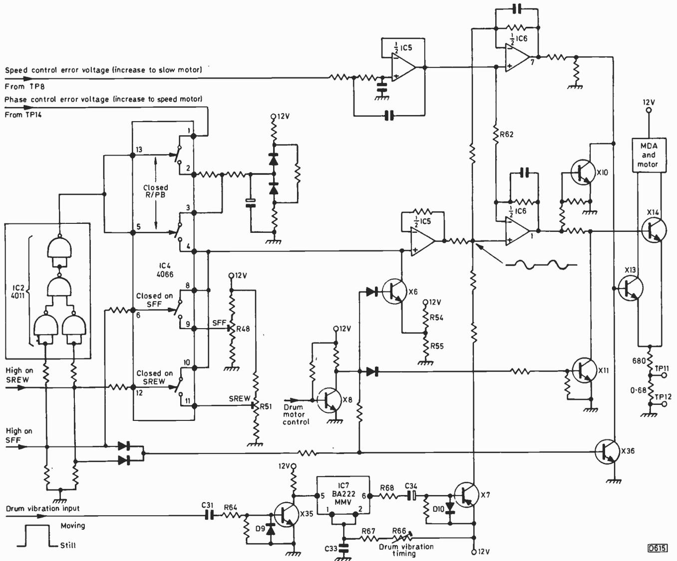
Fig. 82: Drum motor control arrangements.
