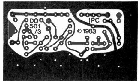
Fig. 13: Preamplifier board pattern.
