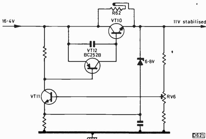
Fig. 1: Series regulator circuit used in the Bush Ranger Model BM6514. With a light load and VT10 non-conductive the output remained at 11V.
