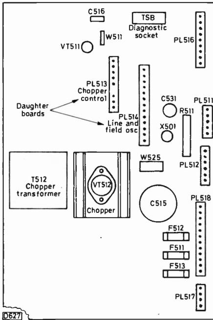
Fig. 2: Items on the right side power supply panel.
