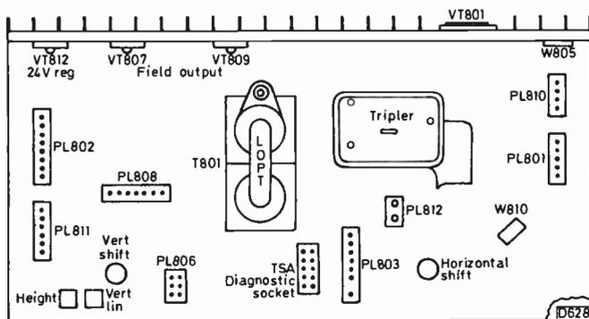
Fig. 3: Main items on the centre horizontal panel, which houses the field and line output stages.
