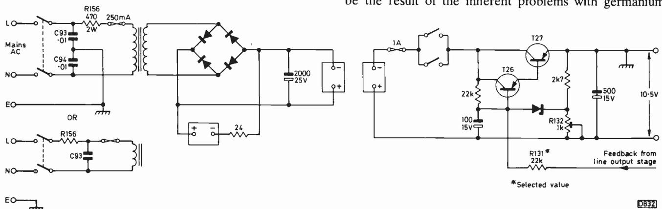
Fig. 1: Mains unit, with battery charging socket, and the earlier two-transistor series regulator circuit.
