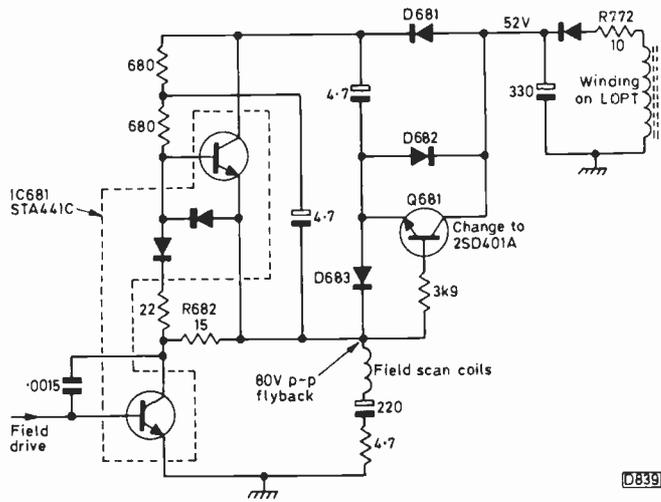
Fig. 1: Field output circuit, Hitachi CPT1471/CPT1473.
