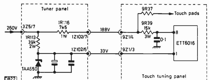
Fig. 1: Supplies to the touch tuning panel.
