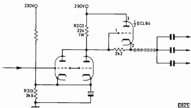
Fig. 3: Modification to remove teletext signals.
