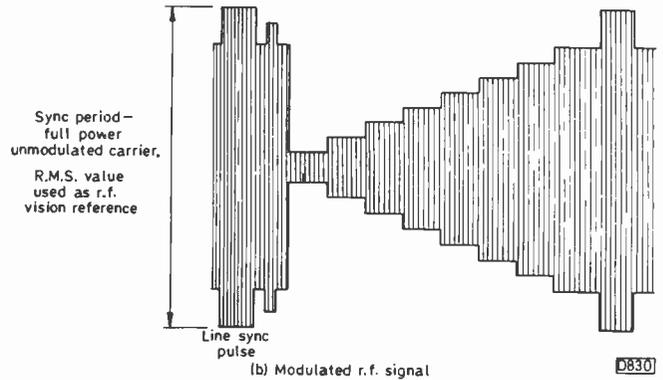
**Fig. 2:** The sync pulse is the reference point to which all signal levels are referred. Note that 1mV r.m.s. = 2.83mV peak-to-peak seen on an oscilloscope.
