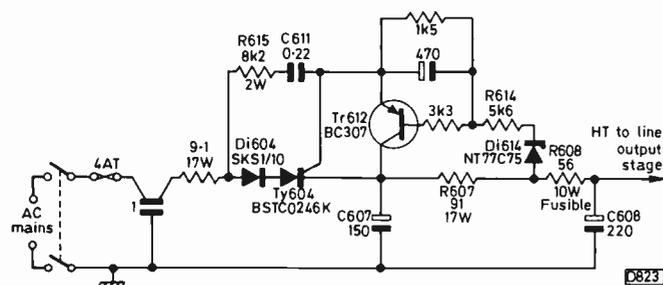
Fig. 1: H.T. rectifier circuit, Grundig 1510 series.
