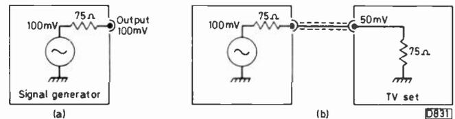
**Fig. 3:** Signal generators usually indicate their output as an e.m.f. at a certain impedance, as shown at (a). In use, the generator will be terminated by the TV set. The e.m.f. then becomes a voltage of half the value (-6dB) stated on the generator.
