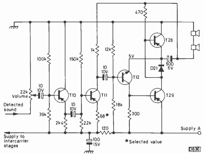
Fig. 5: The audio circuit.
