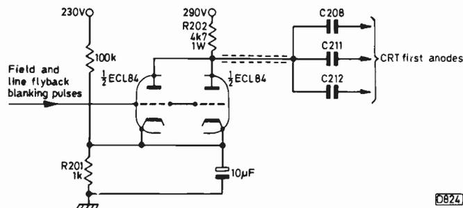
Fig. 2: Flyback blanking in the B and O 2600/3200 chassis.
