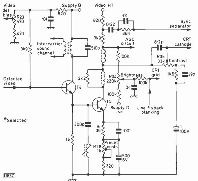
Fig. 6: Video driver and output stages.
