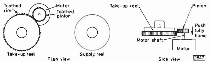
Fig. 2: Pinion wheel trouble with the Mitsubishi HS700.
