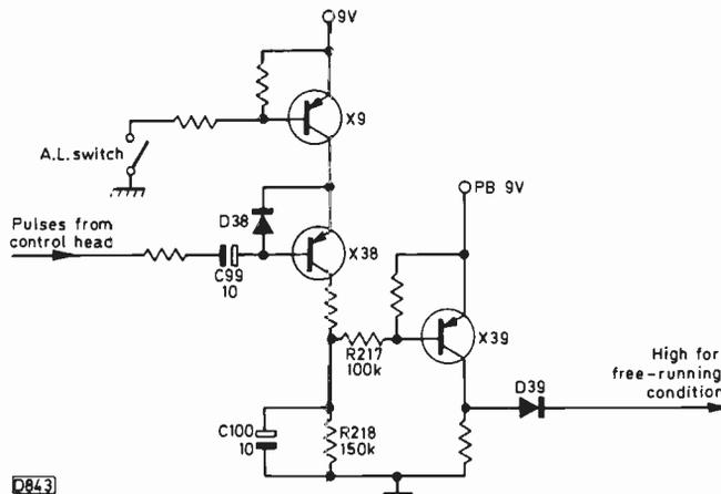
Fig. 123: The control pulse detector circuit.
