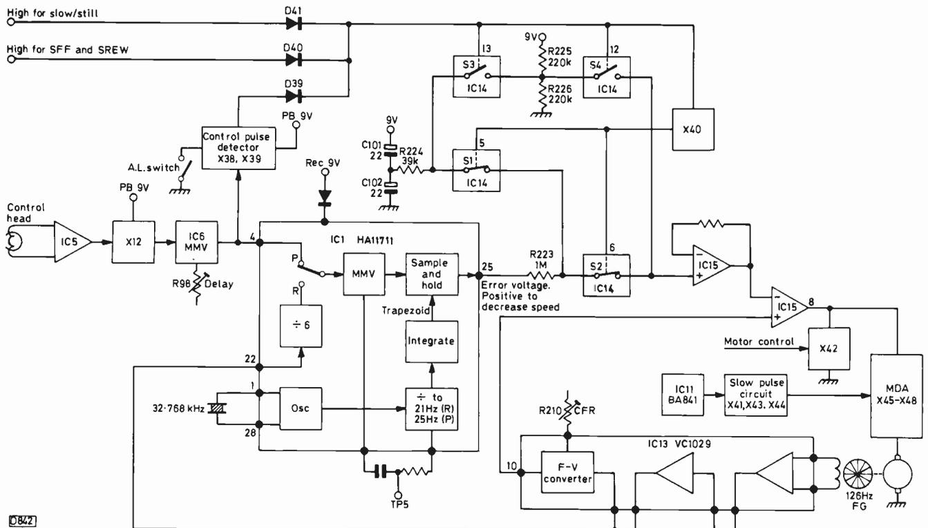
Fig. 122: Block diagram of the capstan servo.
