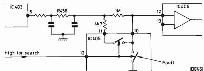
Fig. 1: Picture search fault, Ferguson 3V36.
