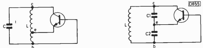
Fig. 2 (left): Basic form of Hartley oscillator.
