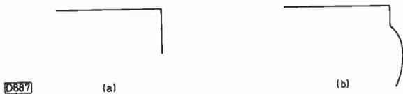
Fig. 12: Testing a diode-thyristor combination. (a) Diode test only. (b) Thyristor turned on.
