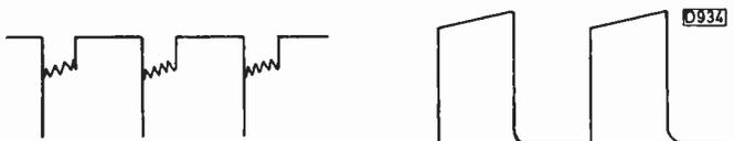
Fig. 6 (left): Drive waveform at the base of Q901.
