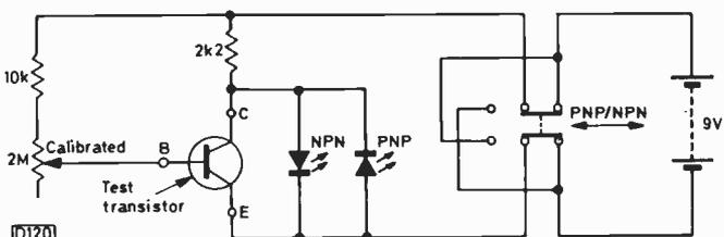
Fig. 6: Simple transistor gain checker. Adjust the potentiometer until one LED is just extinguished: read gain at this point off calibrated potentiometer.
