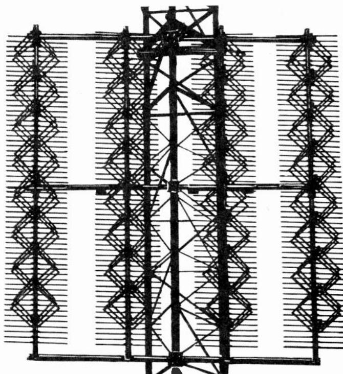
Zig-zag curtain aerial: four-stack array mounted on a lattice mast. Produced by Lindsay, Horsham, Pa, USA.
