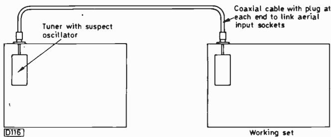
Fig. 2: Using a tuner as a u.h.f. oscillator.
