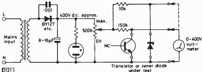
Fig. 7: Non-destructive breakdown tester for transistors and zener diodes. Turn control to zero, insert device being checked then turn up control until the meter gives a stable reading – voltage shown is the breakdown or zener voltage.
