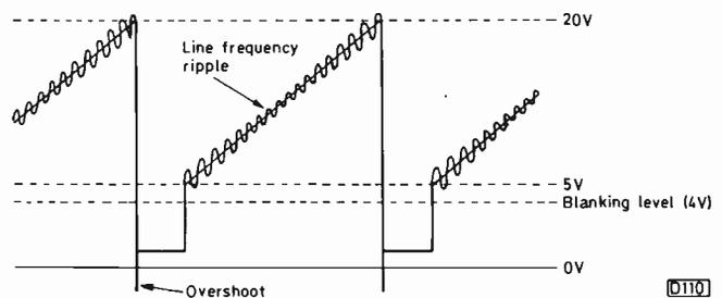
Fig. 1: Correct waveform at the emitter of T43 in the G9's field output stage.
