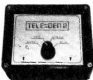
Telegen 2 is a colour bar generator at a very modest price and yet is extremely effective, stable and durable. It is the perfect complement to Telegen 1, giving colour bars arranged in the following sequence: white, yellow, cyan, green, magenta, red, blue and black. The unit provides a signal in the UHF band approx. Channel 35 and requires a supply of 14 to 18 volts D.C.
