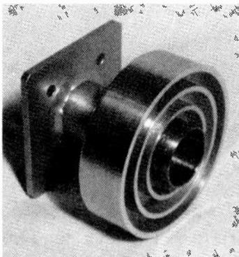
Fig. 1 (left): Typical scalar feedhorn. Note that the rings are adjustable with respect to the waveguide pipe, which is shown protruding slightly. The LNALNC is bolted to the rear flange.
