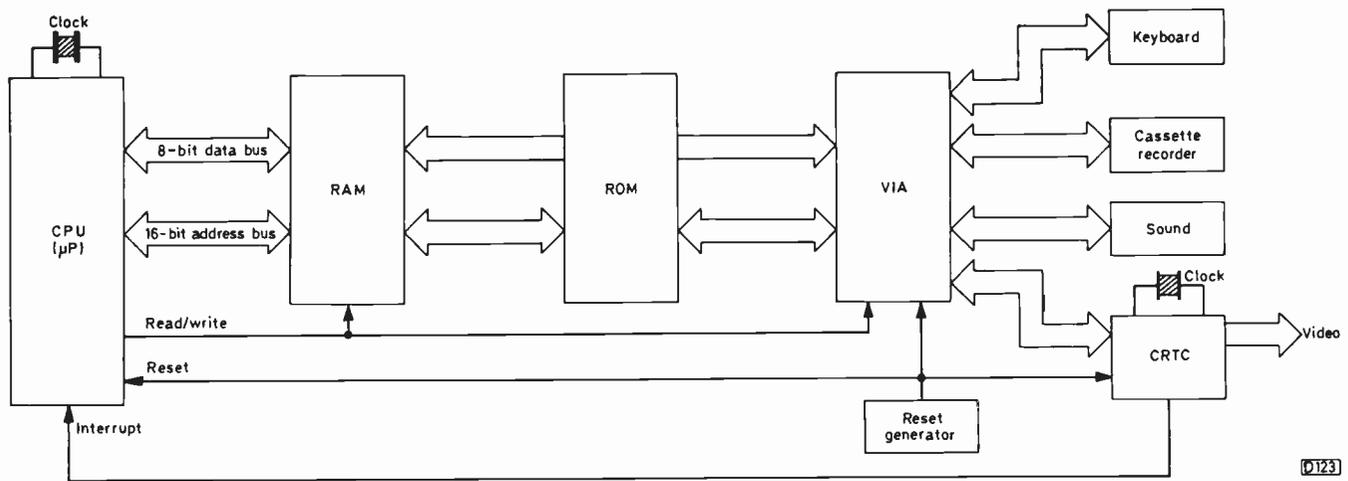
Fig. 1: Basic microcomputer block diagram.
