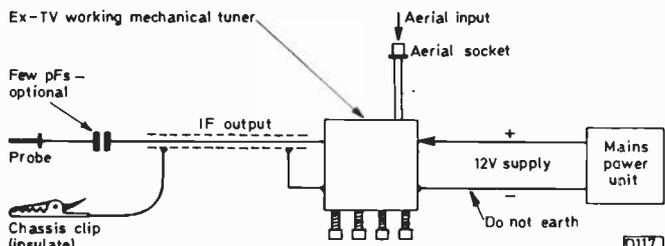
Fig. 3: Tuner substitution set-up. Connect as shown: take care as the metalwork in some chassis is at half mains potential (fit in box). No varicap tuning voltage is required with a mechanical tuner.
