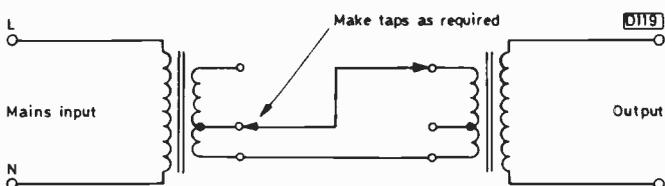
Fig. 5: Use of two transformers to give mains isolation. Small to moderate loads can be connected. Provides 1:1 or other ratios of mains voltage.
