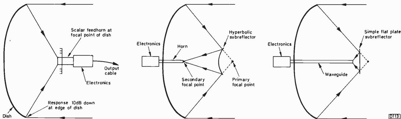
Fig. 3 (left): Parabolic dish aerial with the feedhorn and electronics mounted at the focal point (prime-focus feed).
