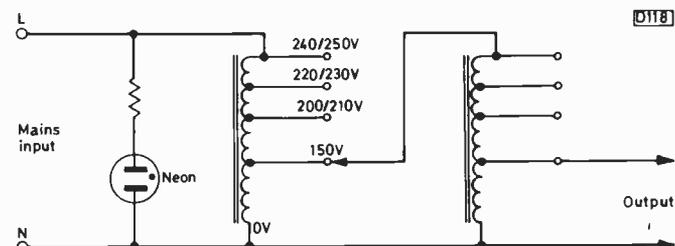
Fig. 4: Poor man's variac: use of two old Thorn autotransformers to give a supply ranging from about 88V up to full mains potential. Isolation is not provided. Output is determined by the various combinations of taps. Take care not to overload.
