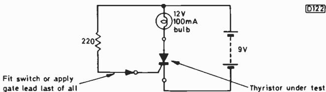
Fig. 8: Simple thyristor tester. Short the anode and cathode connections to check the bulb.
