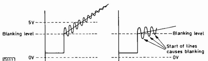
Fig. 2 (left): Incorrect waveform – d.c. conditions wrong.
