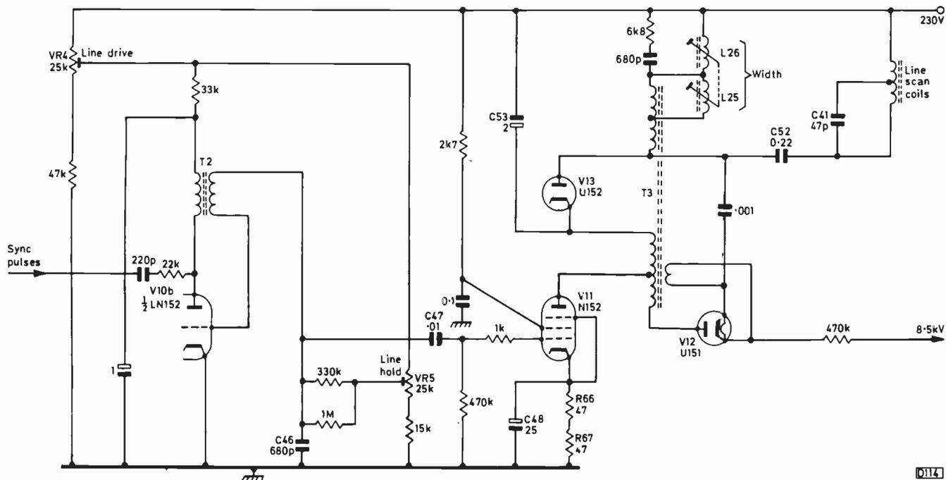
Fig. 1: Line timebase circuit used in the Marconiphone Models VT59DA and VC59DA.
