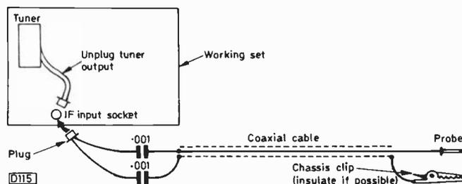
Fig. 1: Tuner/i.f. signal tracer using a working TV set with its tuner disconnected.
