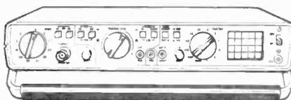
The new Thandar SC110A represents a break-through in oscilloscope development. The SC110A is ONLY TWO INCHES thick and weighs under two pounds, yet retains the standard features and controls of a bench oscilloscope. **FITS IN A BRIEFCASE**
