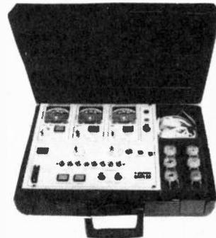
Regenerates picture tubes even better - Also IN-LINE - Removes short-circuits, even between cathode and filament - Measures beam current, emission current, life expectancy, etc.
