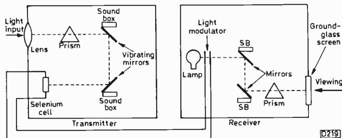
Fig. 1: Basic principle of the telectroscope.
