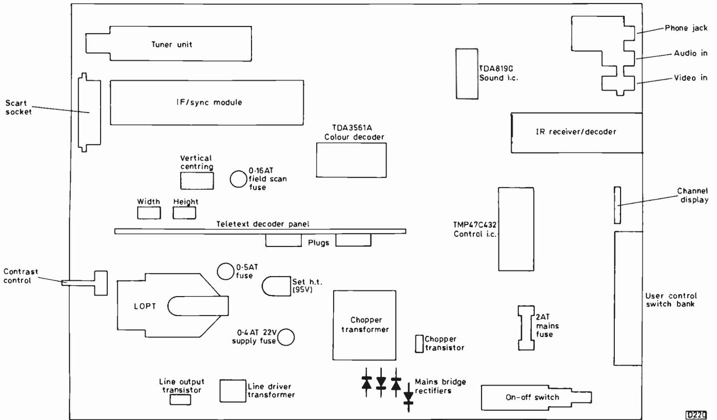
Fig. 1: Basic layout of the Philips CP90 chassis, showing the main components.
