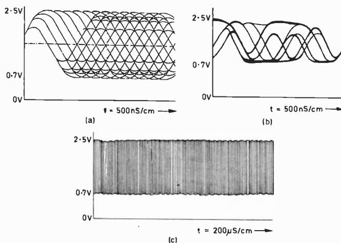
Fig. 2: Off-disc r.f. waveforms. (a) Observed during a passage of music. The d.c. level and peak voltage may differ from model to model. (b) Observed while reading the table of contents or between tracks. (c) Observed during a passage of music, but this time at a slower timebase speed. Instead of seeing the individual increase/decrease of the reflected beam intensity you can see a much larger sample of data.
