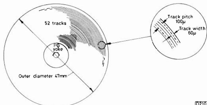
Fig. 2: The disc track arrangement
