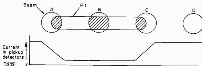
Fig. 1: Laser beam traversing a pit, showing the effect of the pit on the output current waveform.
