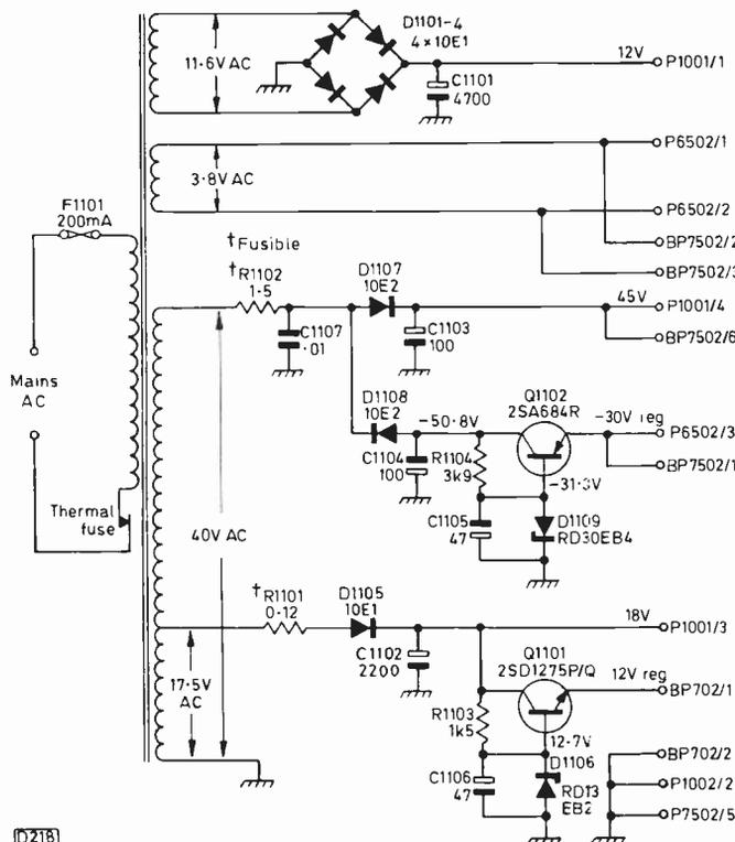
Fig. 2: The mains transformer/rectifier PCB circuit, Model NV370.
