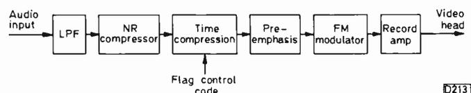
Fig. 5: Block diagram of the audio recording system.
