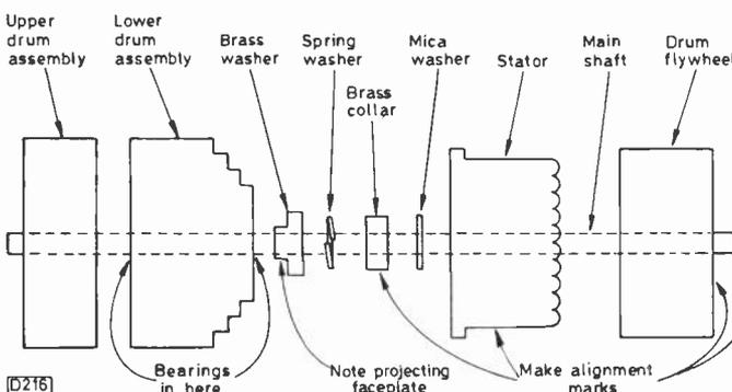
Fig. 3: The various items that comprise the drum assembly in the Panasonic NV333 VCR.
