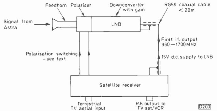
Fig. 1: Simplified block diagram of a receiver system for Astra transmissions.
