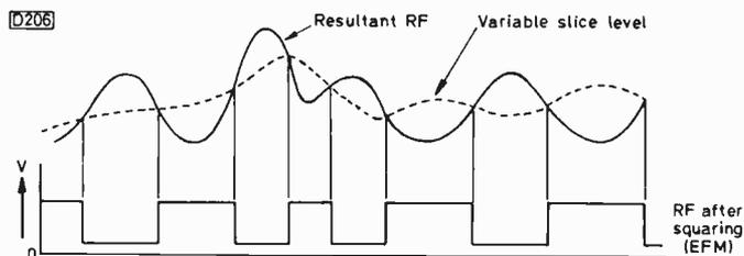
Fig. 4: The waveform squaring process carried out by the auto asymmetry control section of the circuit.
