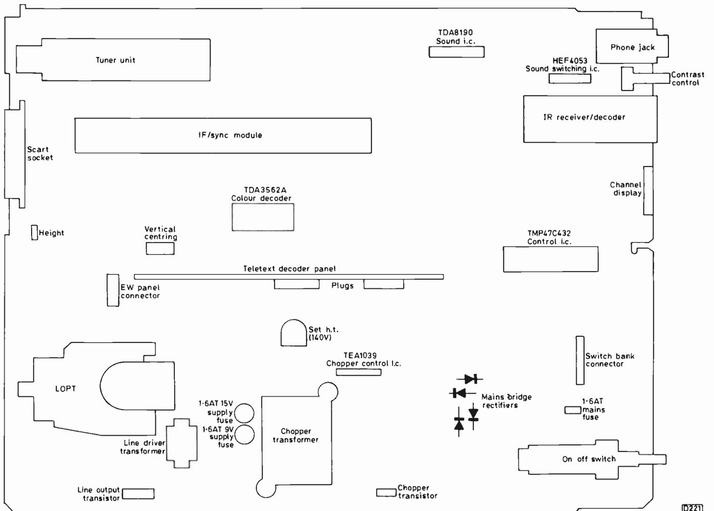
Fig. 2: Basic layout of the Philips CP110 chassis, showing the main components.
