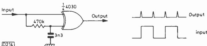
Fig. 1: Use of an exclusive-or gate to obtain substitute field sync pulses from the head switching waveform in a VCR.
