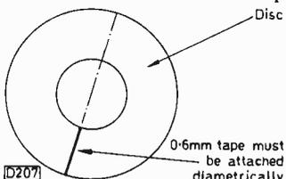
Fig. 5: A simple test disc can be made from a one-hour commercial recording and PCB artwork tape (RS Components order code 555 370 for example).
