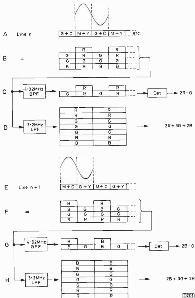
Fig. 1: The way in which the signal samples (pixels) are processed to produce separate luminance and  $2R - G/2B - G$  colour signals on alternate lines with the earlier system that uses filtering and matrixing.
