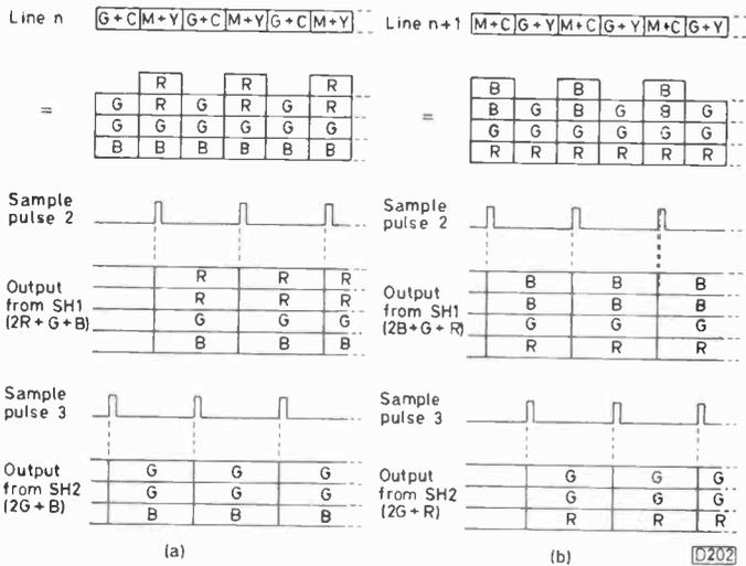
Fig. 2: Equivalent conditions with the later high-resolution system that uses sampling instead of simple filtering to separate the h.f. components of the output from the image sensor. (a) Line n; (b) Line n + 1.
