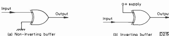
Fig. 2: An exclusive-or gate can be used as a non-inverting buffer (a) or an inverting buffer (b) depending on the way in which it is wired.
