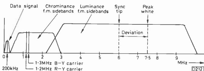
Fig. 4: Frequency spectrum of the recorded signals.
