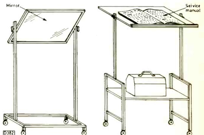
Fig. 3 (left): Mobile mirror. Easily pushed aside and with a pivot action to cater for different screen sizes. The back can be used to mount test and colour charts or focus patterns for camcorder servicing.
