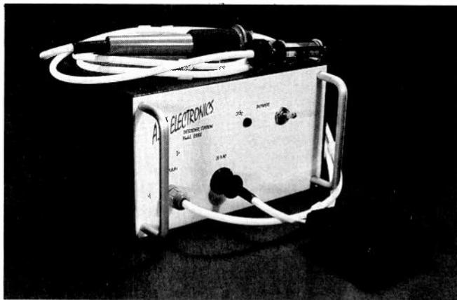
The AK Electronics RA100 desoldering station.
