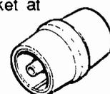
**Co-Axial Chassis Mounting Socket.** Plastic body.
